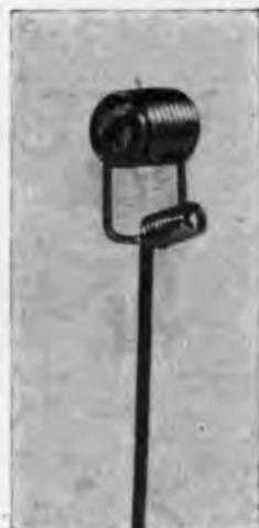
Fig. 74.—Storage Electrode for High-pressure Lamps (Osram, Berlin).
