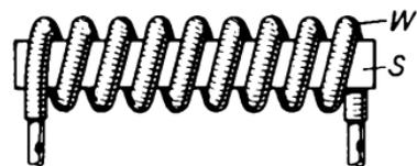
Fig. 66.—Example of a Storage Cathode.
