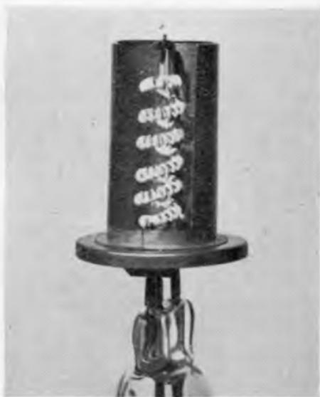
Fig. 68.—Directly Heated Double Spiral Cathode with Heat Shield Used in High-voltage Rectifiers (part of shielding cylinder cut away). (Current density 0.2 amp./cm.<sup>2</sup>; AEG G 10/4d;  $\frac{2}{3}$  natural size.)
