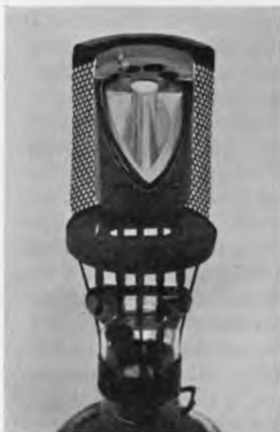
Fig. 69.—Hull's Multicellular Cathode: (a) Schematic Cross-section; (b) Commercial Cathode. (Current density 0.3 amp./cm.<sup>2</sup>; AEG S 15/40;  $\frac{2}{3}$  natural size.)
