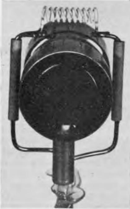
Fig. 67.—Directly Heated Spiral Cathode of a Low-voltage Rectifier. (Current density 3 amp./cm.<sup>2</sup>; AEG N 190/10;  $\frac{3}{4}$  natural size.)
