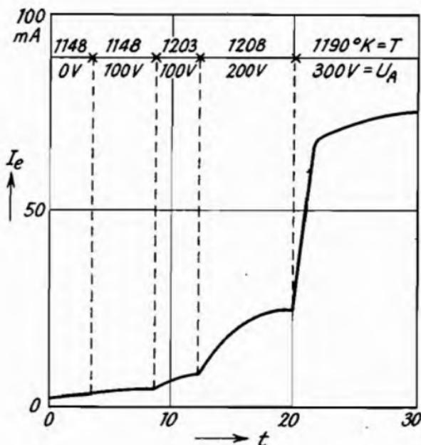
Fig. 133.—Variation of the Emission Current  $I_e$  during an Activation by Drawing Current from a Combined BaO Cathode (Espe<sup>1</sup>).
