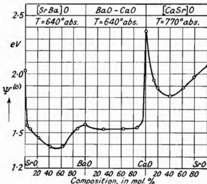
Fig. 112.—Work Function  $\Psi$  as a Function of Composition of Mixtures of Alkaline Earth Oxides (Huber<sup>1</sup>).
