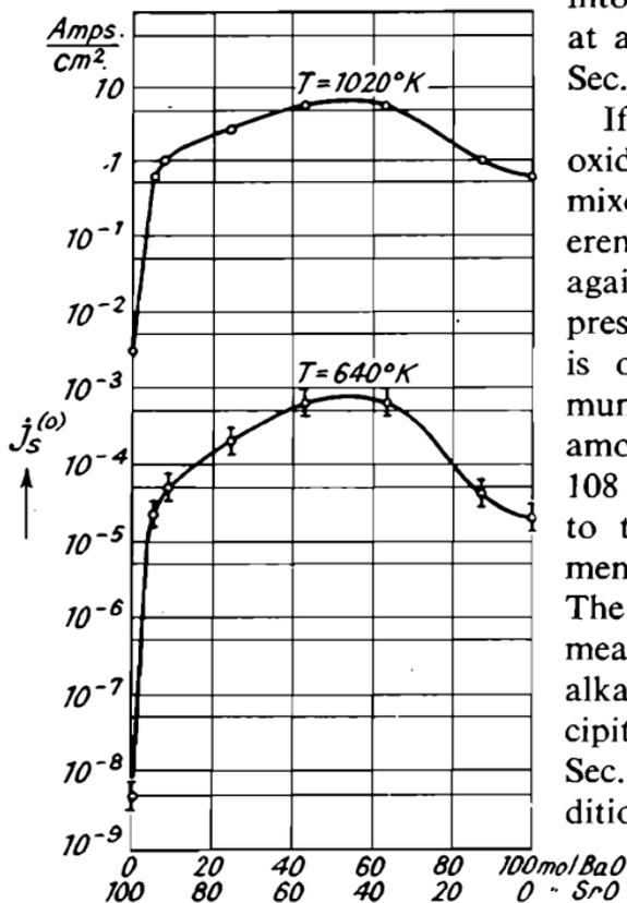
Fig. 108.—Density  $j_s$  of the Saturated Current of an Oxide Cathode, consisting of Mixed Crystals [BaSr]O, as a Function of Composition (Huber<sup>1</sup>).
