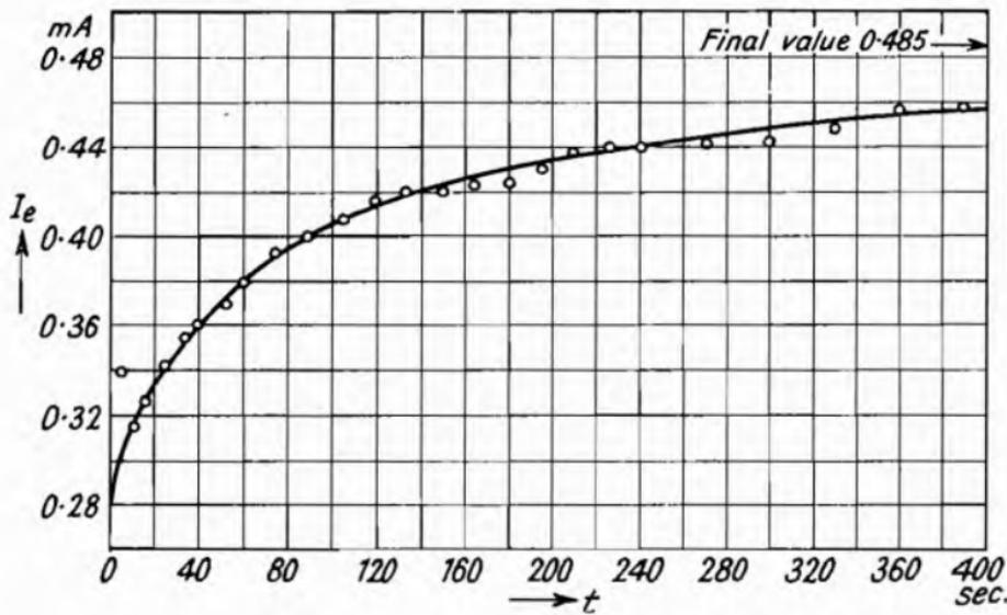
Fig. 134.—Variation of the Emission Current  $I_e$  after decreasing the Cathode Temperature (Davisson and Germer<sup>1</sup>).
