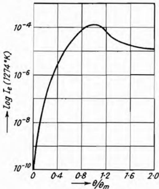
Fig. 34.—Electron Emission of the W-Th Cathode as a Function of the Fraction  $\theta$ , covered with Th (Brattain and Becker<sup>1</sup>).
