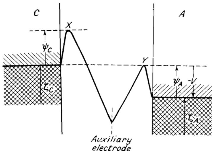
Fig. 58.—Potential Distribution in the Experimental Set of Goss and Henderson.<sup>1</sup>
