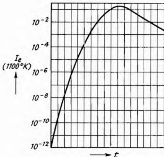
Fig. 84.—Variation of the Emission Current of a Tungsten Ribbon during the Heating of an Oxide Cathode, arranged opposite to the Ribbon (Becker<sup>1</sup>).
