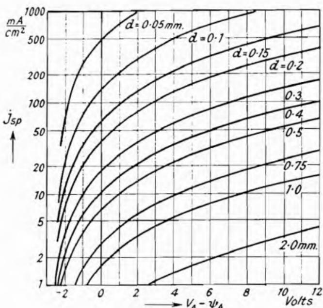
Fig. 22.—Density  $j_{sp}$  of Space-charge Current as a Function of the Difference  $V_A - \psi_A$  between Anode Voltage and Work Function of the Anode (Distance  $d$  between Cathode and Anode as Parameter) (Liebmann<sup>1</sup>).
