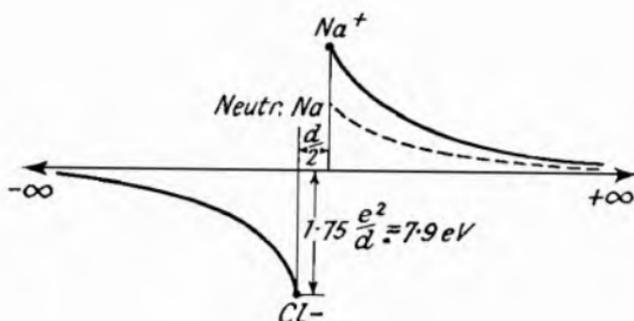
Fig. 67.—Variation of the Potential of the Electrons during the Formation of Sodium Chloride (Schematic).
