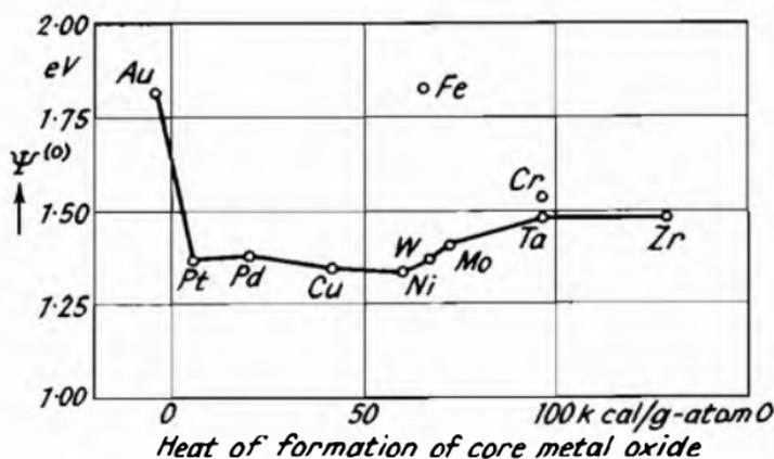
Fig. 149.—Relation between Work Function  $\Psi^{(0)}$  and Heat of Formation of the Core Metal Oxide, for Cathodes with Different Core Metals (Liebold <sup>1</sup>) (the Work Functions shown are calculated from the Emission Equation).
