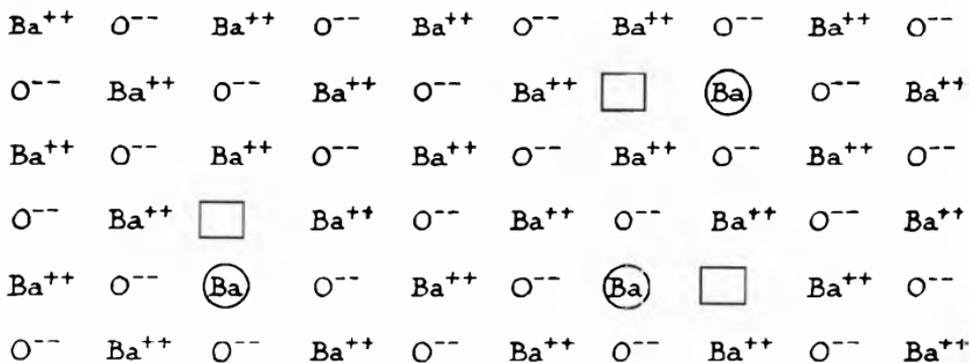
Fig. 88.—Configuration of Excess Barium in the Crystal Lattice of a Barium Oxide Cathode.
