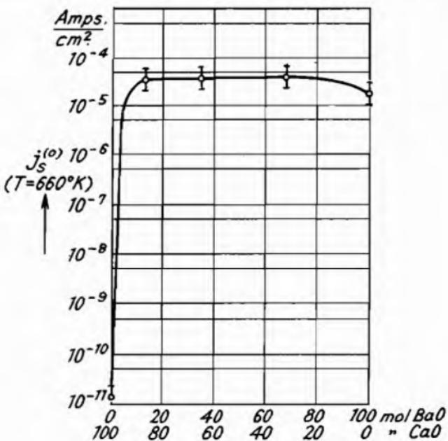
Fig. 110.—Density  $j_s$  of the Saturated Current of an Oxide Cathode, consisting of a  $\text{BaO}-\text{CaO}$  Mixture, as a Function of Composition (Huber<sup>1</sup>).
