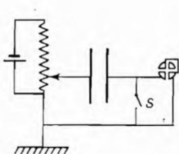
Fig. 51.—Circuit for Measuring the Contact Potential according to Lord Kelvin (Gericke<sup>1</sup>).
