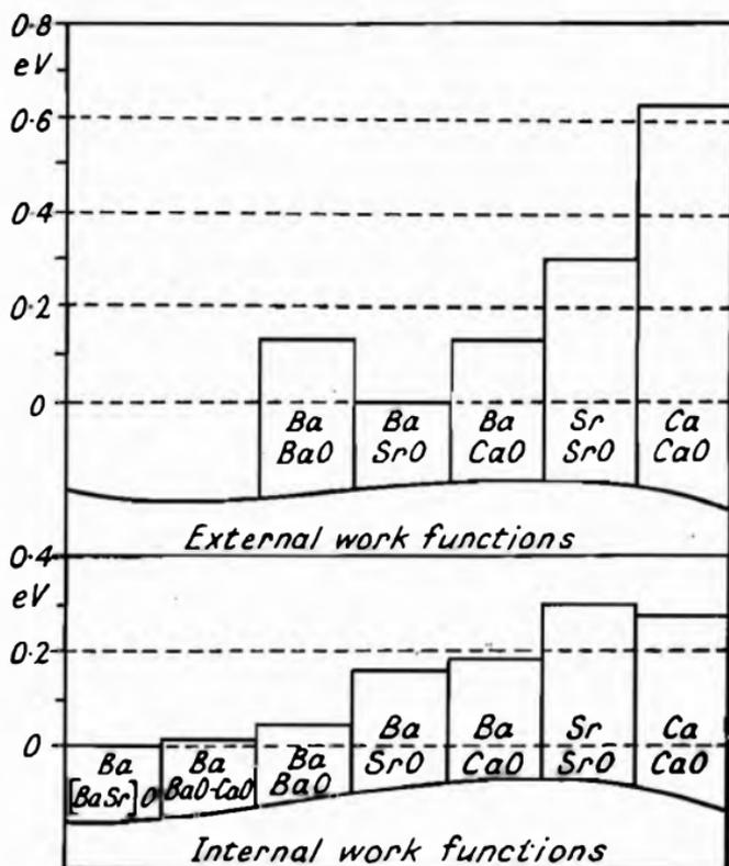
Fig. 123.—Differences between Internal and External Work Functions of differently composed Oxide Cathodes according to Huber.<sup>1</sup>
