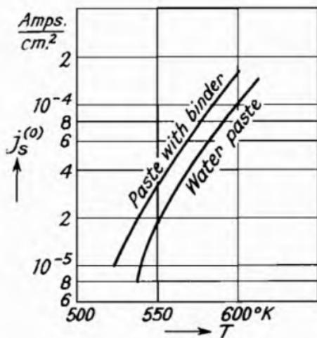
Fig. 127.—Saturated Currents of Oxide Coatings prepared with and without Organic Binder as a Function of Temperature (Liebold<sup>1</sup>).
