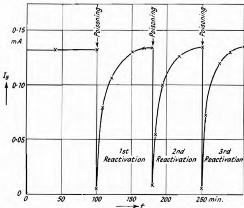
Fig. 139.—Variation of the Saturated Current during the Reactivation after Poisoning by Oxygen (Metson<sup>2</sup>).
