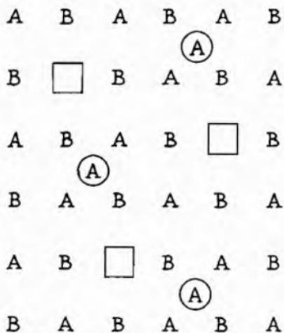
Fig. 60.—Frenkel Defects.
