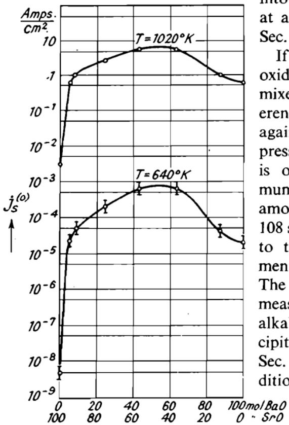
Fig. 108.—Density  $j_s$  of the Saturated Current of an Oxide Cathode, consisting of Mixed Crystals [BaSr]O, as a Function of Composition (Huber<sup>1</sup>).
