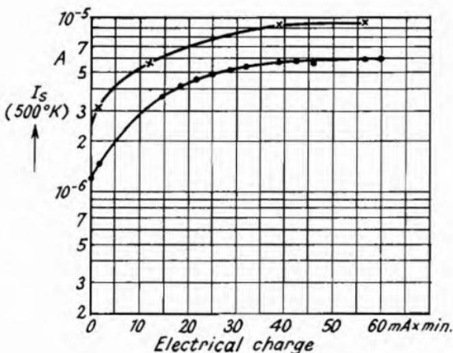
Fig. 87.—Variation of the Saturated Current of an Oxide Cathode during Repeated Electron Bombardments (Becker and Sears<sup>2</sup>).
