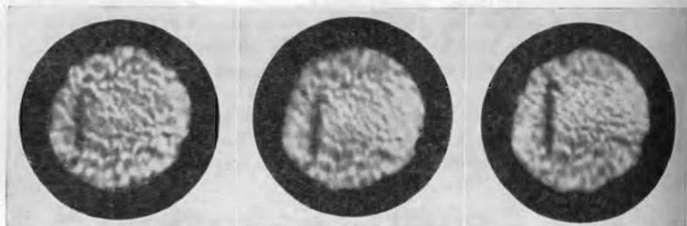
Fig. 99.—Electron Images of an Oxide Cathode taken during Further Activation (mag.  $\times 30$ ): (a)  $I_s = 10^{-6}$  amp.; (b)  $I_s = 2 \times 10^{-3}$  amp.; (c)  $I_s = 2 \times 10^{-2}$  amp. (Heinze and Wagener<sup>2</sup>).
