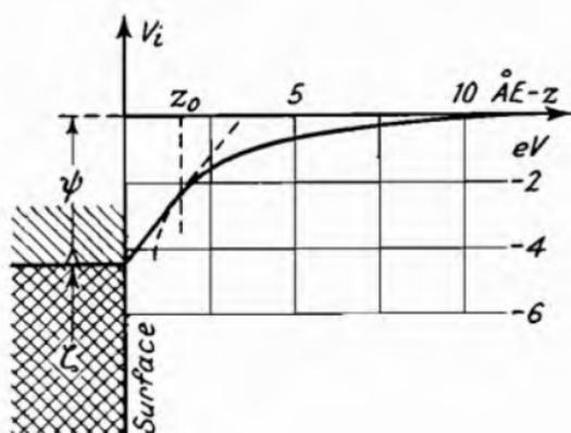
Fig. 8.—The Potential  $V_i$  associated with the Image Force.
