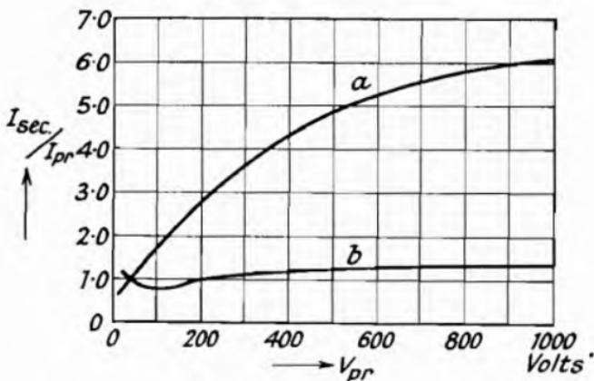
Fig. 106.—Coefficient of Secondary Emission ( $I_{\text{sec}}/I_{\text{pr}}$ ) of an Oxide Cathode as a Function of Primary Voltage  $V_{\text{pr}}$ : (a) activated, (b) poisoned (Bruining and de Boer<sup>1</sup>).
