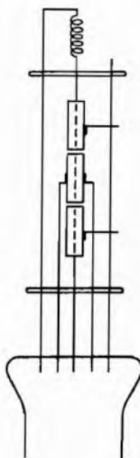
Fig. 46.—Assembly for Measurement of the Work Function.
