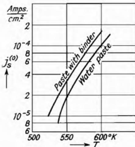
Fig. 127.—Saturated Currents of Oxide Coatings prepared with and without Organic Binder as a Function of Temperature (Liebold<sup>1</sup>).
