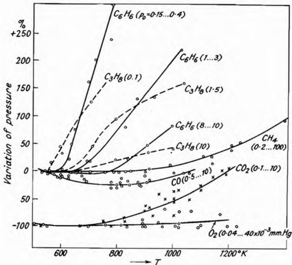
Fig. 147.—Variation of Gas Pressure during 10 Minutes Poisoning of an Oxide Cathode by Different Gases as a Function of the Temperature of the Cathode (Herrmann and Krieg<sup>2</sup>).
