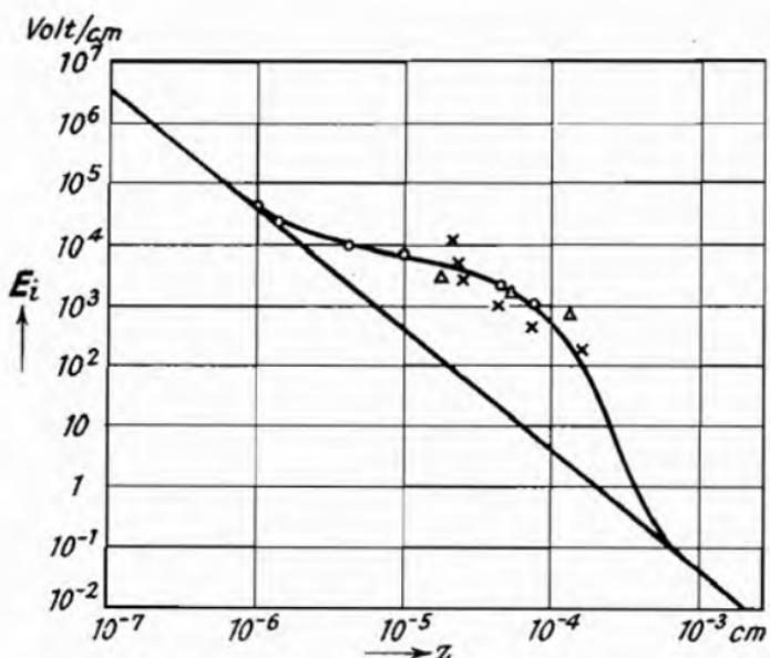
Fig. 41.—The Internal Field  $E_i$  as a Function of the distance  $z$  from the Surface (Linford<sup>1</sup>).
