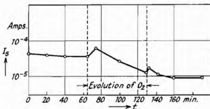
Fig. 143.—Variation of the Saturated Current of an Oxide Cathode when setting free Small Quantities of Oxygen from a Second Cathode with Iron Core (Liebold<sup>1</sup>).
