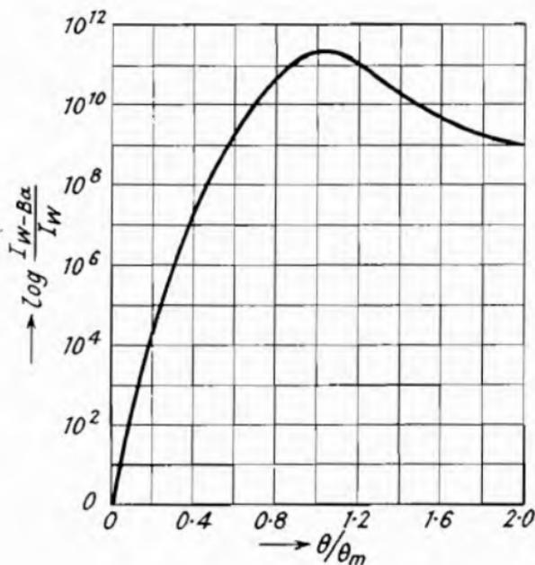
Fig. 33.—Emission Current of a W-Ba Cathode as a Function of the Fraction  $\theta$  covered with Barium (Becker <sup>4</sup>).
