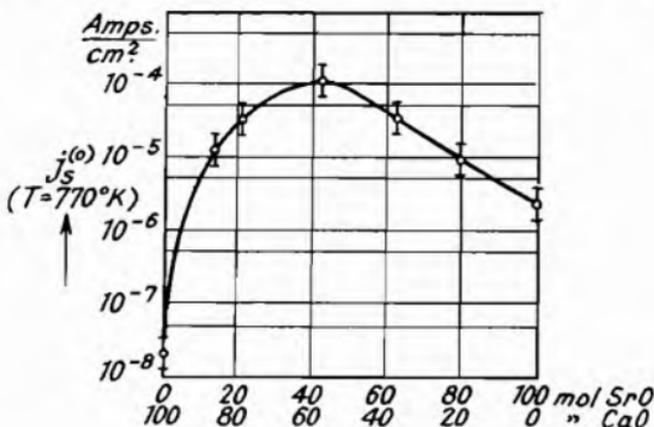
Fig. 109.—Density  $j_s$  of the Saturated Current of an Oxide Cathode, consisting of Mixed Crystals [SrCa]O, as a Function of Composition (Huber <sup>1</sup>).
