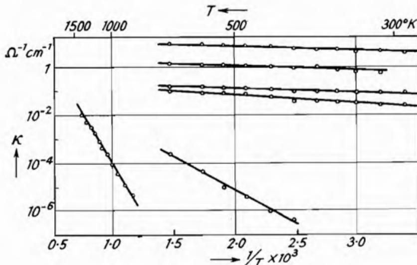
Fig. 79.—The Conductivity  $\kappa$  of a Semi-conductor as a Function of Temperature for Different Densities of Excess Atoms :  $\text{TiO}_2$  (Meyer<sup>2)</sup>).
