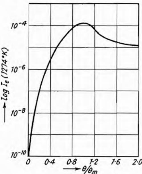
Fig. 34.—Electron Emission of the W-Th Cathode as a Function of the Fraction  $\theta$ , covered with Th (Brattain and Becker<sup>1</sup>).
