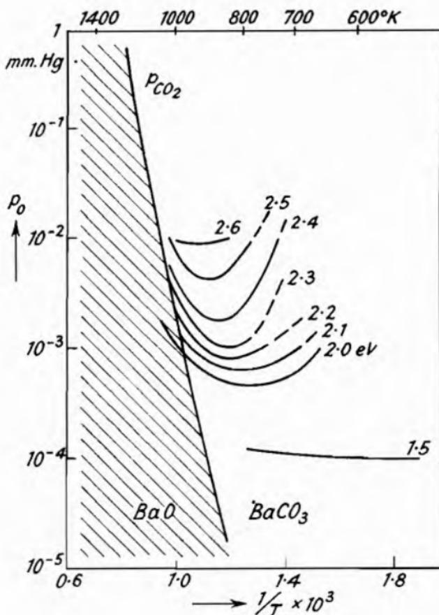
Fig. 144.—Pressure-Temperature Diagram showing Curves of Equal Work Function for Poisoning by Carbon Dioxide after 10 Minutes Exposure. The Dashed Line represents the Dissociation Pressure of  $\text{BaCO}_3$  (Herrmann and Krieg<sup>2)</sup>.
