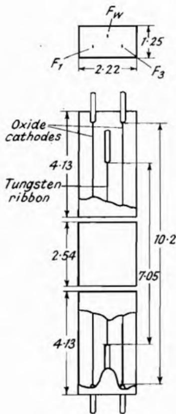
Fig. 85.—Experimental Arrangement of Becker<sup>1</sup> (dimensions in cm.).
