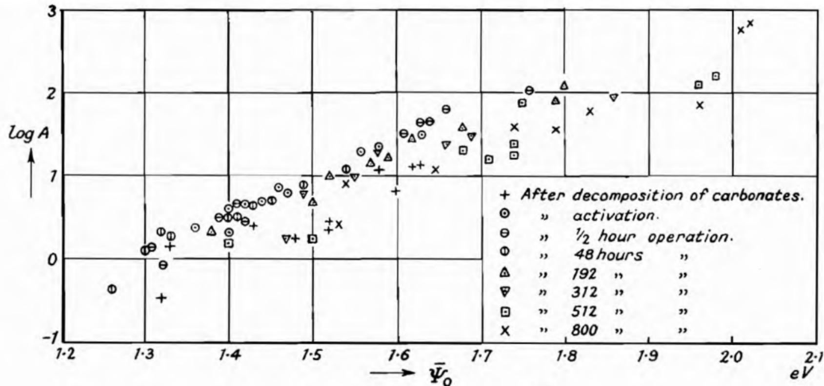
Fig. 95.—Relationship between Emission Constant  $A$  and Work Function  $\bar{\Psi}_0$  of Oxide Cathodes (Veenmans<sup>1</sup>).
