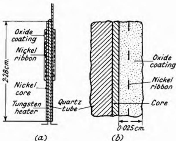
Fig. 100.—Sectional View of an Experimental Cathode for measuring the Conductivity of the Coating: (a) Total View; (b) Enlarged Section (Becker and Sears<sup>2</sup>).
