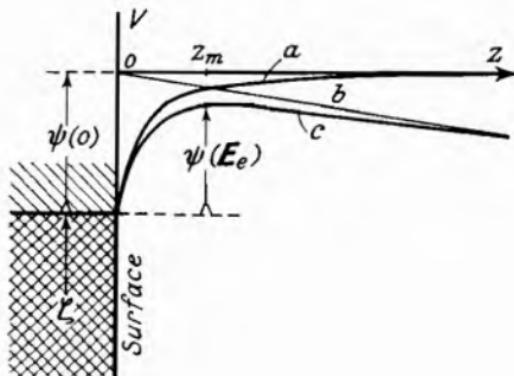
Fig. 9.—Superposition of Image Potential and External Potential.
