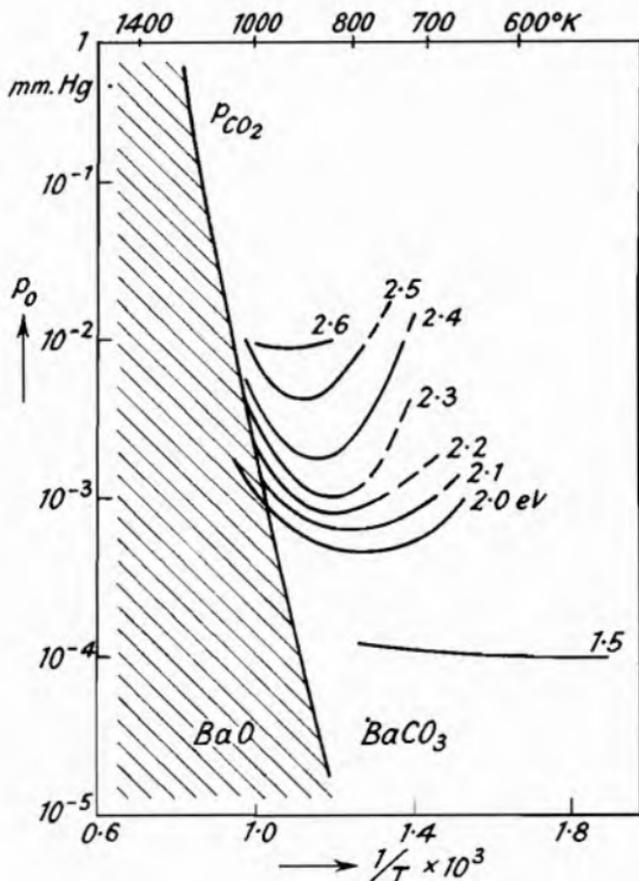
Fig. 144.—Pressure-Temperature Diagram showing Curves of Equal Work Function for Poisoning by Carbon Dioxide after 10 Minutes Exposure. The Dashed Line represents the Dissociation Pressure of  $\text{BaCO}_3$  (Herrmann and Krieg<sup>2</sup>).
