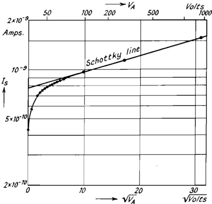
Fig. 27.—Measured and Calculated Values of the Saturated Current as a Function of Anode Voltage ( $T=1434^{\circ}$  K.) (Nottingham<sup>1</sup>).
