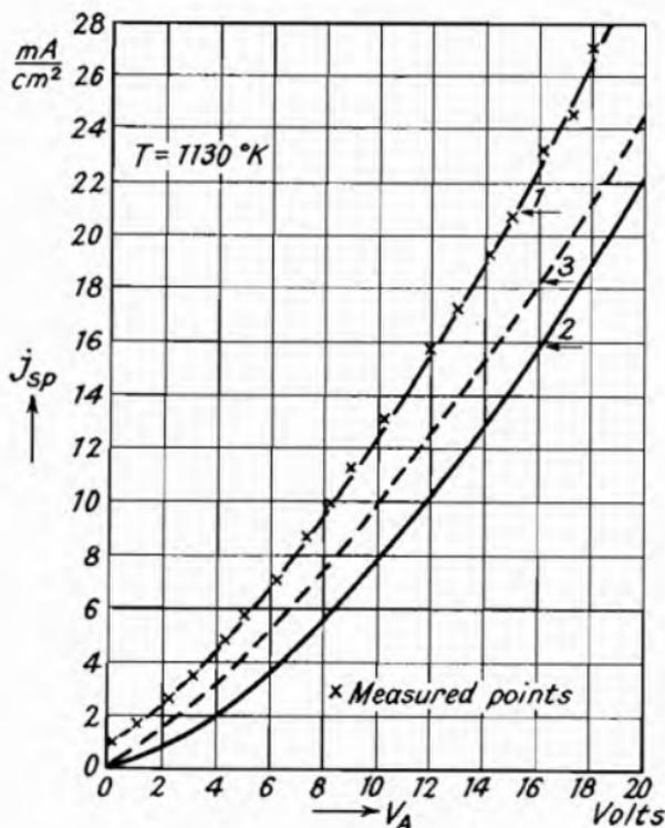
Fig. 23.—Comparison of Measured and Calculated Values of the Space-charge Current. 1. Calculated according to (65). 2. Calculated according to (60). 3. Calculated according to (65), the correction term  $\Delta$  being neglected (Kleen<sup>1</sup>).
