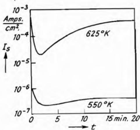
Fig. 140.—Variation of the Saturated Current during Poisoning by Oxygen (Initial Pressure  $3 \times 10^{-5}$  mm.) (Herrmann and Krieg<sup>2</sup>).
