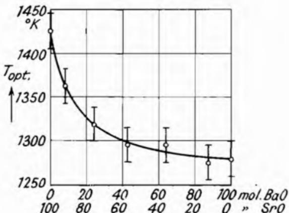
Fig. 131.—Optimum Activation Temperature  $T_{opt}$  as a Function of the Composition of a  $[BaSr]O$  Mixture (Huber<sup>1</sup>).
