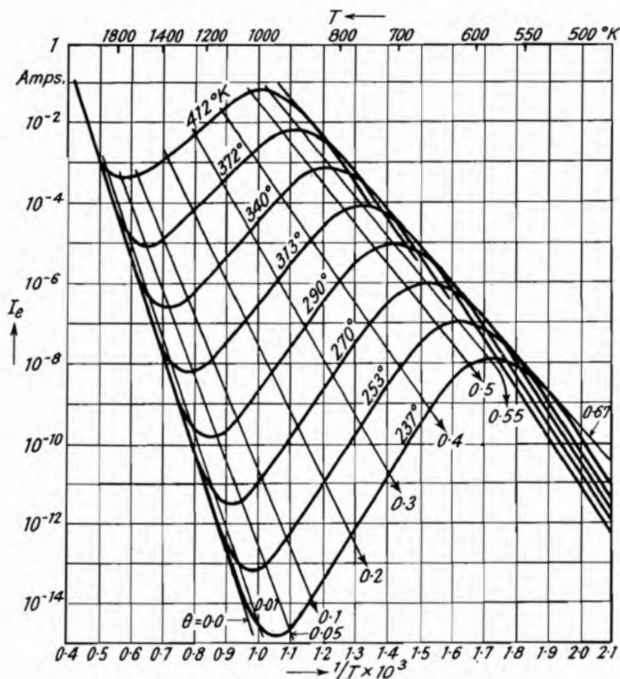
Fig. 30.—Electron Emission of the W-Cs Cathode as a Function of Temperature (Temperature of the Valve as Parameter) (Langmuir and Taylor<sup>8</sup>).
