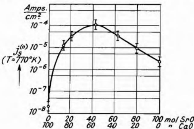
Fig. 109.—Density  $j_s$  of the Saturated Current of an Oxide Cathode, consisting of Mixed Crystals  $[\text{SrCa}]O$ , as a Function of Composition (Huber<sup>1</sup>).
