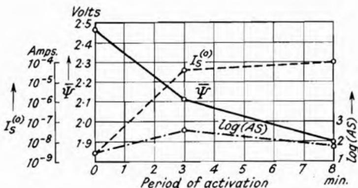
Fig. 97.—Variation of Work Function  $\bar{\Psi}$  and Saturated Current  $I_s^{(0)}$  of an Oxide Cathode during the Activation (Heinze and Wagener<sup>4</sup>).
