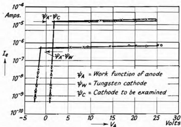
Fig. 54.—Determination of the Contact Potential by the Intersection Method (Heinze and Wagener<sup>3</sup>).
