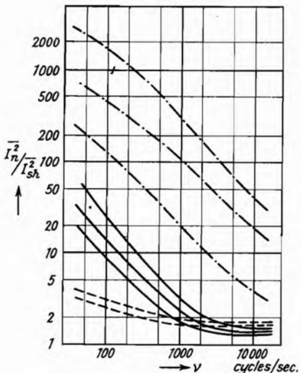
Fig. 153.—Ratio between Mean Square of Noise Current  $\bar{I}_n^2$  and Mean Square of Shot Current  $\bar{I}_{sh}^2$  of Oxide Cathodes as a Function of Frequency  $\nu$  (Graffunder<sup>1</sup>).
