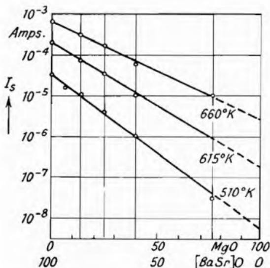
Fig. 111.—Saturated Current of Oxide Cathodes, made of Mixtures of [BaSr]O and MgO, as a Function of Composition (Herrmann<sup>1</sup>).
