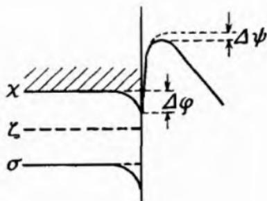
Fig. 93.—Depression of Energy Levels of a Semi-Conductor produced by an External Electrical Field (Morgulis<sup>2</sup>).
