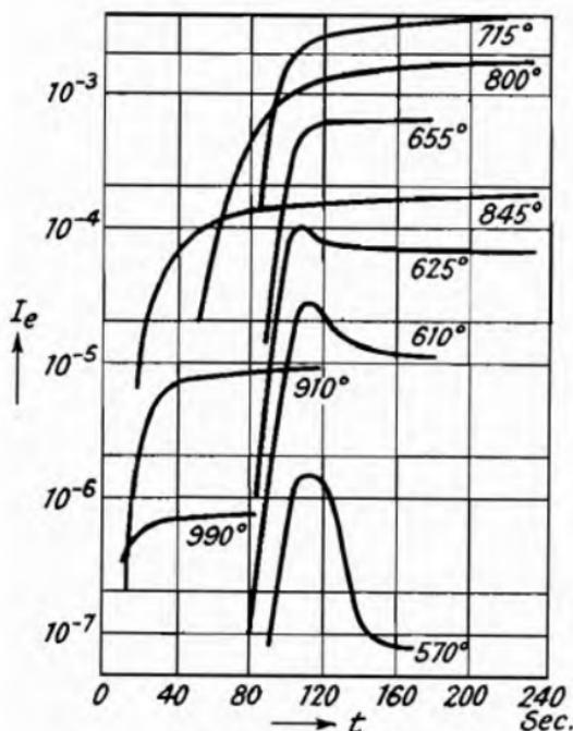
Fig. 31.—Activation of a W-Cs Cathode (Cathode Temperature as Parameter) (Becker<sup>1</sup>).
