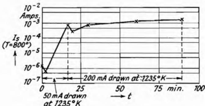
Fig. 129.—Variation of the Saturated Current during the Activation by Drawing Current of a Cathode with Platinum Core previously poisoned with Oxygen (Heinze and Wagener <sup>1</sup>).
