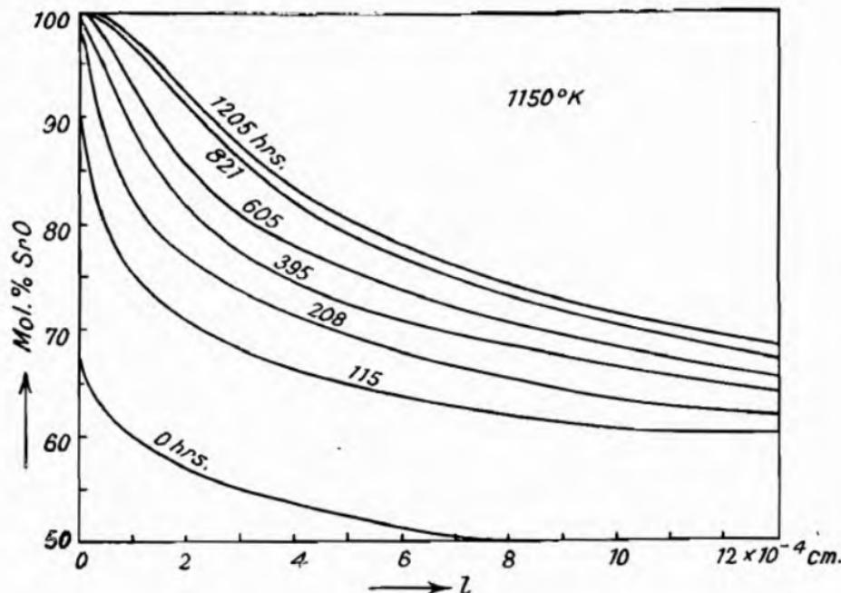
Fig. 114.—Percentage of Strontium Oxide in a [BaSr]O Cathode as a Function of Distance  $l$  from the Surface (Eisenstein<sup>1</sup>) (operating time as parameter).
