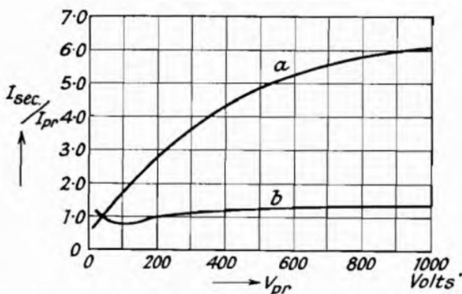
Fig. 106.—Coefficient of Secondary Emission ( $I_{sec}/I_{pr}$ ) of an Oxide Cathode as a Function of Primary Voltage  $V_{pr}$ : (a) activated, (b) poisoned (Bruining and de Boer<sup>1</sup>).
