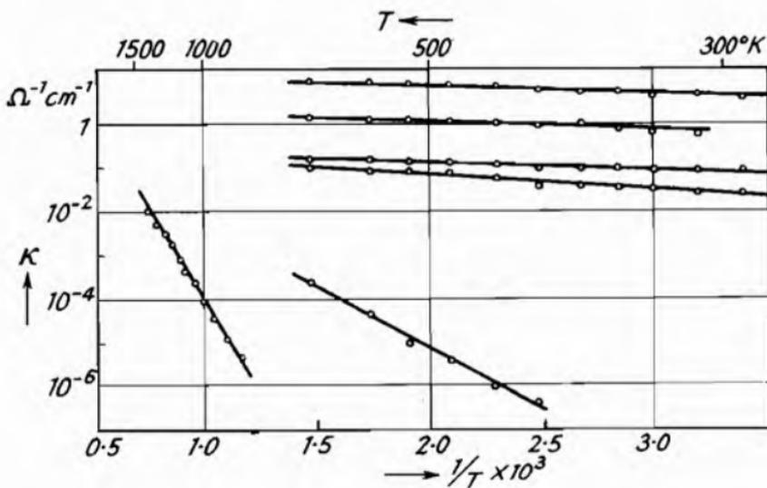
Fig. 79.—The Conductivity  $\kappa$  of a Semi-conductor as a Function of Temperature for Different Densities of Excess Atoms : TiO<sub>2</sub> (Meyer <sup>2</sup>).
