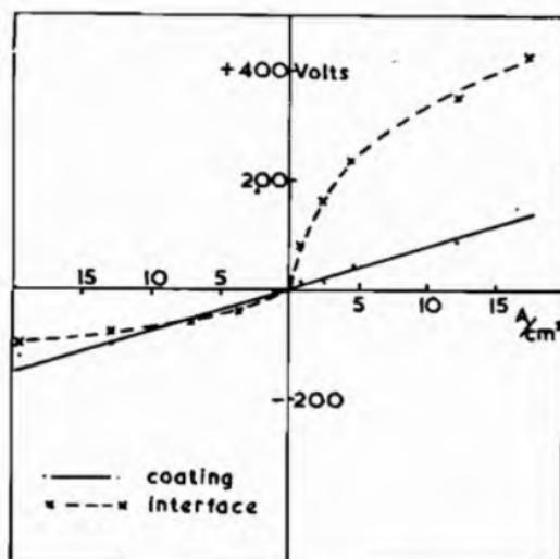
Fig. 150.—Voltage-current characteristic of a  $[BaSr]O$  coating on  $Ni + 5\%$  Si-core metal, and of the interface layer between coating and core ( $T = 1135^\circ K$ , curves obtained by  $5 \mu$  sec. pulses) (Mutter<sup>1</sup>).
