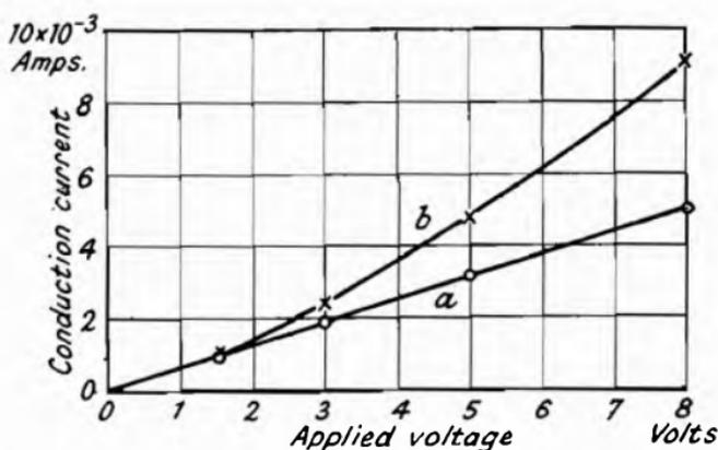
Fig. 101.—Relationship between Conduction Current through the Coating and Applied Voltage (Becker and Sears<sup>2</sup>).
