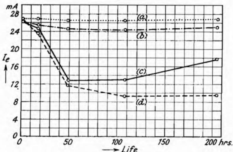
Fig. 152.—Variation of the Emission Current  $I_e$  during Life at a Cathode Temperature of  $800^\circ\text{K}$ .
