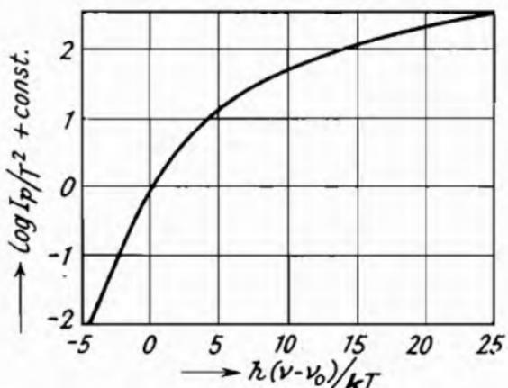
Fig. 57.—Plot of the Photo-electric Current according to Fowler (Du Bridge and Roehr<sup>3</sup>).
