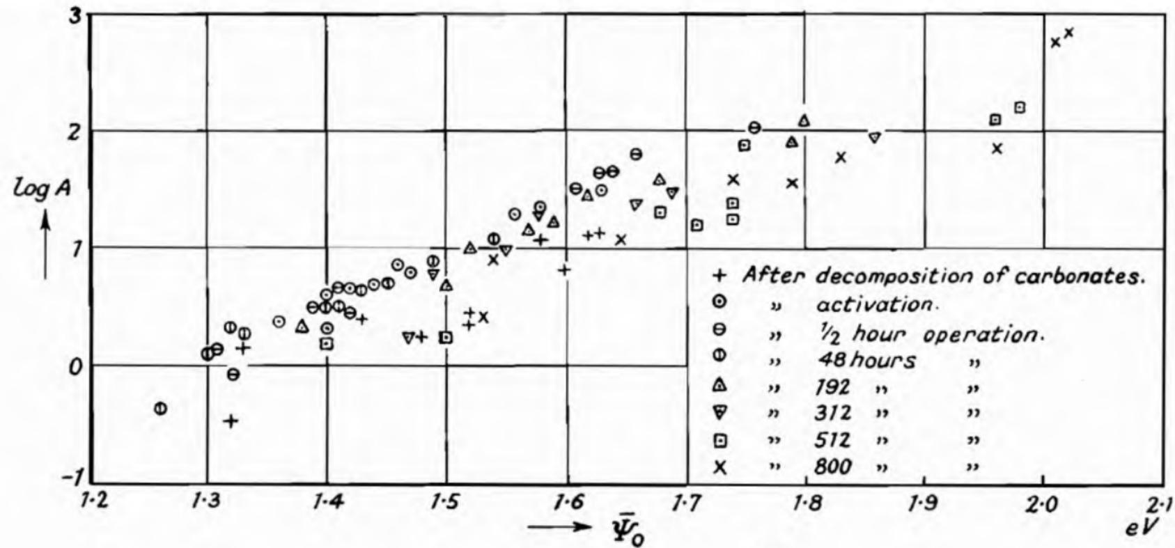
Fig. 95.—Relationship between Emission Constant  $A$  and Work Function  $\bar{\Psi}_0$  of Oxide Cathodes (Veenemans<sup>1</sup>).
