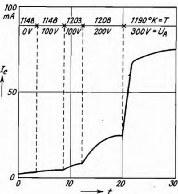
Fig. 133.—Variation of the Emission Current  $I_e$  during an Activation by Drawing Current from a Combined BaO Cathode (Espe<sup>1</sup>).
