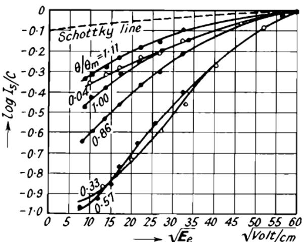
Fig. 43.—Saturated Current of a W-Th Cathode as a Function of Square Root of the Applied Field Strength for Different Densities of Adsorbed Material (Becker<sup>5</sup>).
