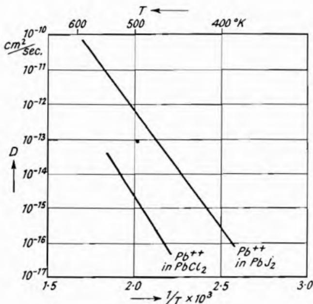
Fig. 65.—Diffusion Coefficient  $D$  of  $\text{PbCl}_2$  and  $\text{PbI}_2$  as a Function of Temperature (Hevesey and Seith,<sup>1</sup> Seith<sup>2</sup>).
