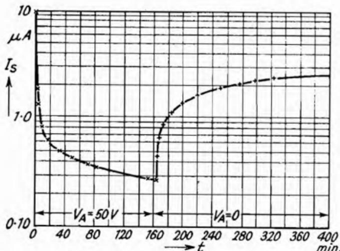
Fig. 135.—Fall and Rise of the Saturated Current  $I_s$ , when operating the Cathode with and without Anode Voltage (Becker<sup>1</sup>).
