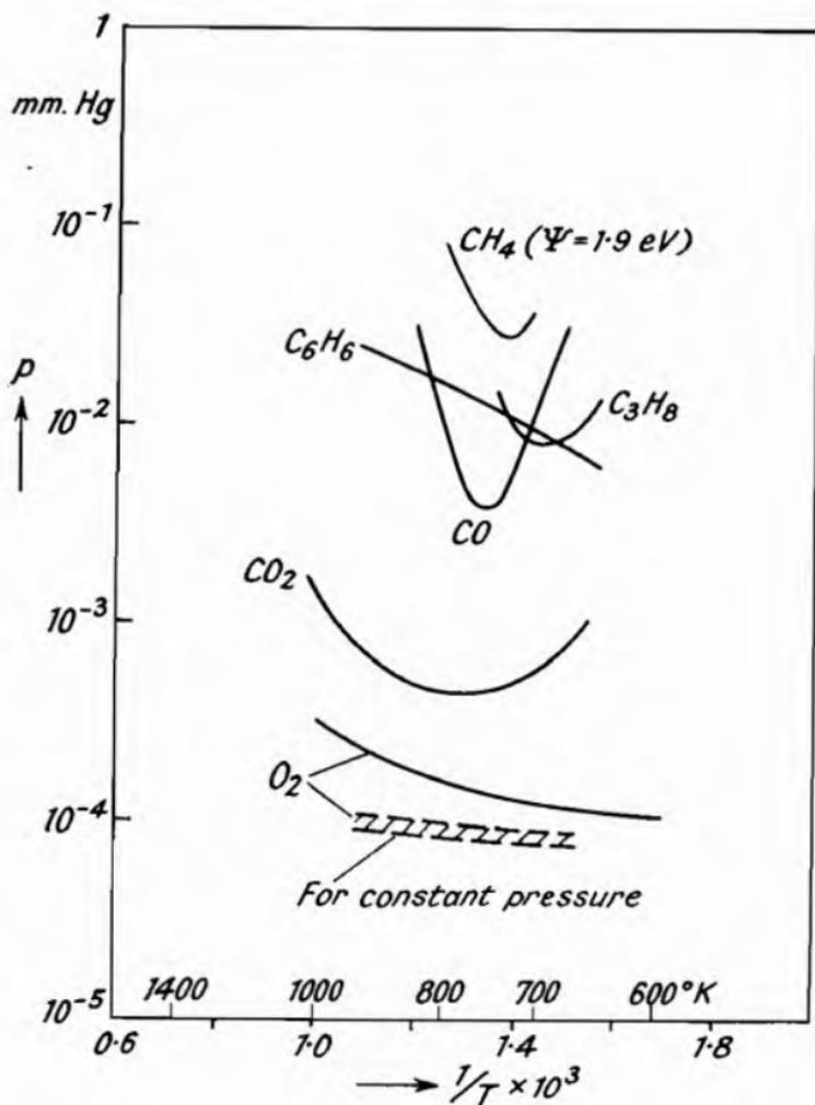
Fig. 146.—Pressure-Temperature Diagram showing Curves of Equal Work Function ( $\Psi = 2.0 \text{ eV}$ ) for Poisoning by Different Gases after 10 Minutes Exposure. The Dashed Curves refer to Poisoning by Oxygen with Constant Pressure. (Herrmann and Krieg<sup>2</sup>).
