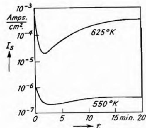
Fig. 140.—Variation of the Saturated Current during Poisoning by Oxygen (Initial Pressure  $3 \times 10^{-5}$  mm.) (Herrmann and Krieg<sup>2</sup>).
