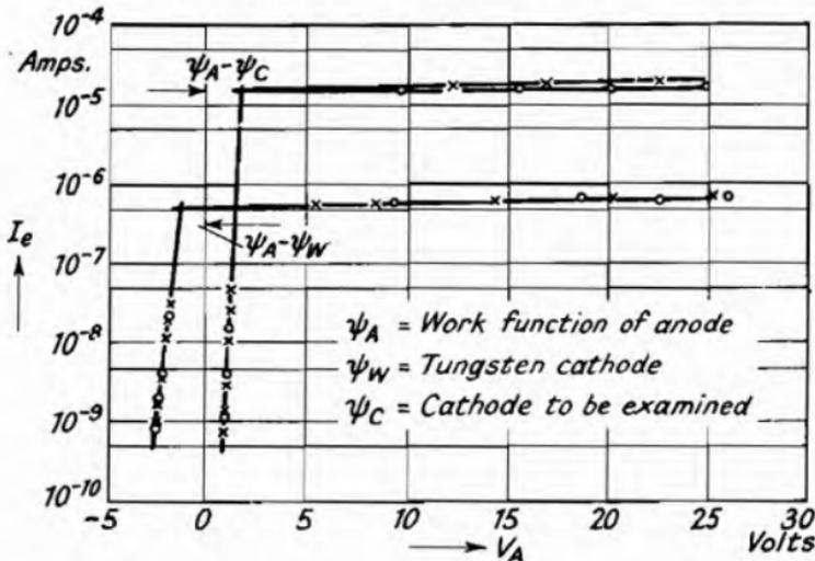
Fig. 54.—Determination of the Contact Potential by the Intersection Method (Heinze and Wager<sup>3</sup>).
