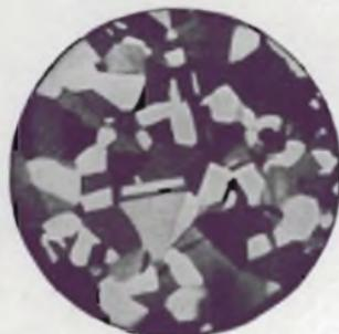
Fig. 39.—Electron Images of a Ni-Cs Cathode (mag.  $\times 5$ ) (Brueche<sup>2</sup>).
