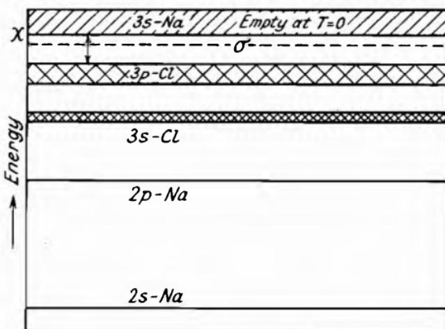
Fig. 68.—Energy Bands of Sodium Chloride.
