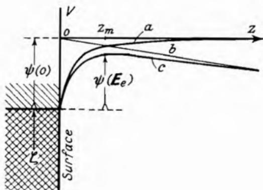
Fig. 9.—Superposition of Image Potential and External Potential.
