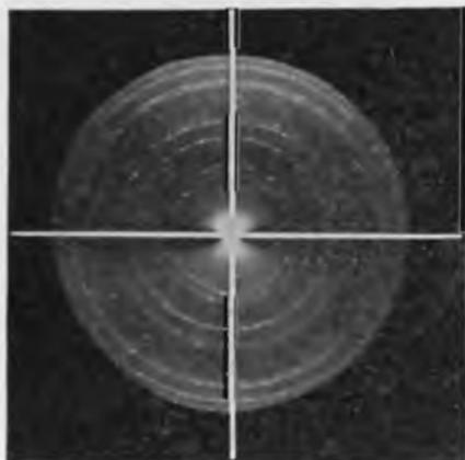
Fig. 113.—Electron Diffraction Patterns of an Oxide Cathode coated by SrO on the One Side and by [BaSr]O on the Other Side (Huber and Wagener<sup>2</sup>).
