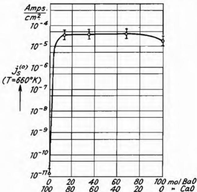
Fig. 110.—Density  $j_s$  of the Saturated Current of an Oxide Cathode, consisting of a BaO–CaO Mixture, as a Function of Composition (Huber <sup>1</sup>).
