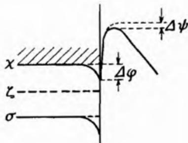
Fig. 93.—Depression of Energy Levels of a Semi-Conductor produced by an External Electrical Field (Morgulis<sup>2</sup>).
