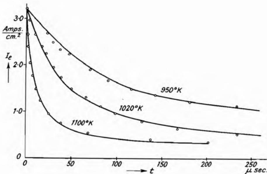
Fig. 137.—Variation of the Emission Current obtained by applying a pulsed Anode Voltage (Sproull<sup>1</sup>).
