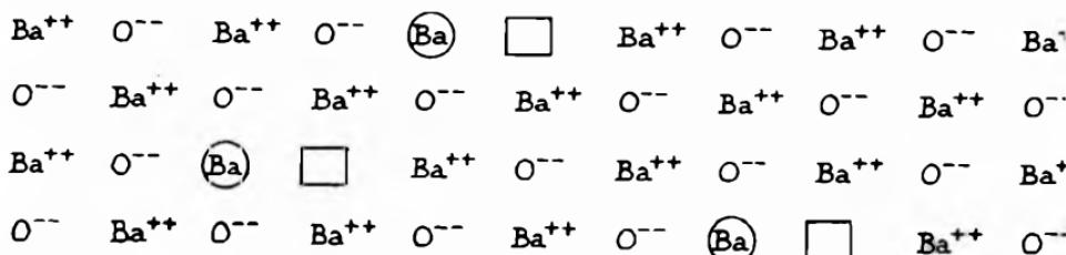
Fig. 105.—Composition of the Surface of a Barium Oxide Coating.
