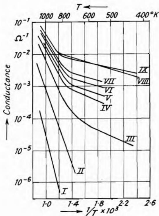
Fig. 104.—Electrical Conductance of a [BaSr]O Coating as a Function of Temperature for Different States of Activation (Range of Medium and Low Temperatures) (Vink<sup>1</sup>).
