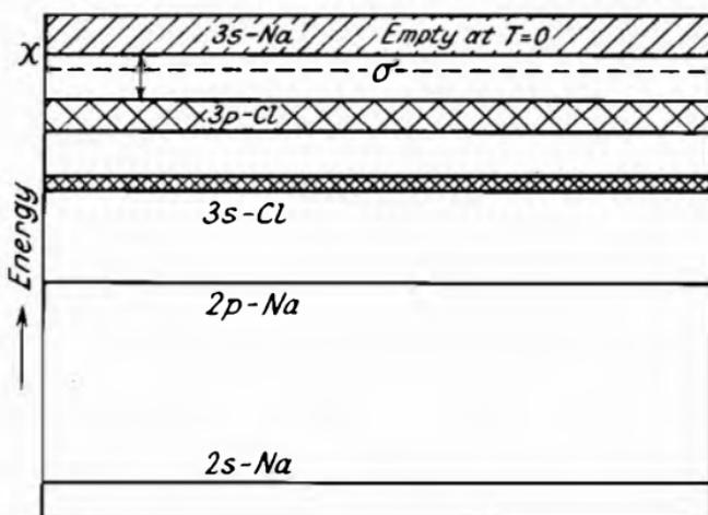
Fig. 68.—Energy Bands of Sodium Chloride.
