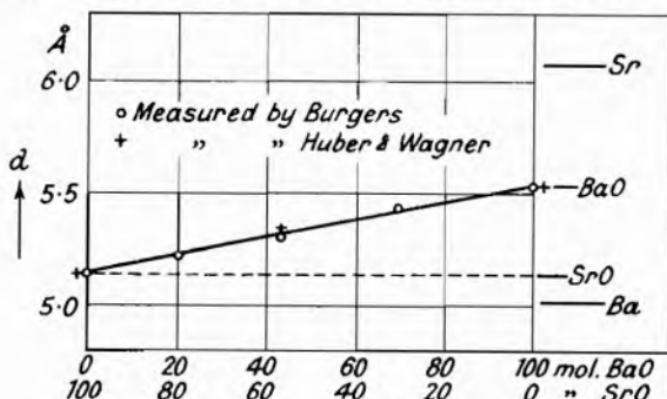
Fig. 107.—Lattice Constant  $d$  of Mixed Crystals [BaSr]O as a function of Composition (Burgers,<sup>1</sup> Huber and Wagener<sup>2</sup>).
