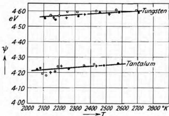
Fig. 59.—Temperature Dependence of the Work Functions  $\psi$  of Tungsten and Tantalum (Krueger and Stabenow<sup>2</sup>).
