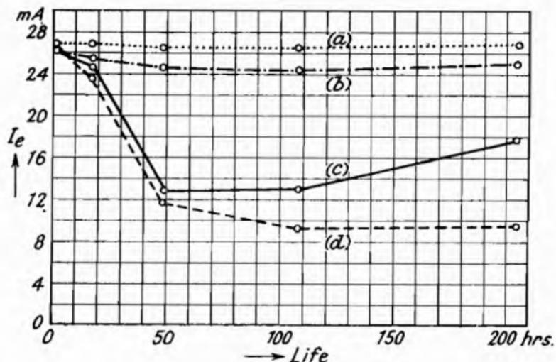
Fig. 152.—Variation of the Emission Current  $I_e$  during Life at a Cathode Temperature of  $800^\circ$  K.
