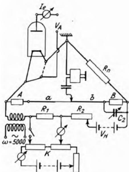
Fig. 50.—Principal Circuit for Measuring the Cooling Power.
