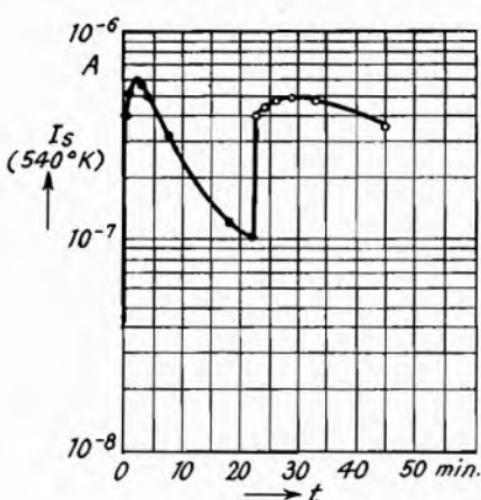
Fig. 86 that the emission current of an oxide cathode not only depends on the qualities of the surface of the coating but also on the qualities of the interior, especially on the number of excess barium atoms in the interior.
