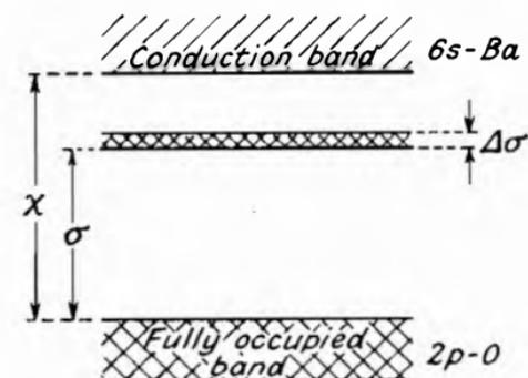
Fig. 89.—Energy Bands of the BaO Lattice with Excess Ba built in.
