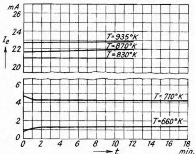
Fig. 136.—Variation of the Emission Current  $I_e$  of a well activated Cathode after switching on the Anode Voltage.
