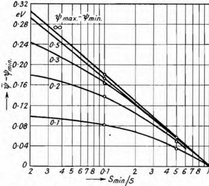
Fig. 44.—Difference between the Mean Value  $\bar{\psi}$  of the Work Function and the smallest Work Function  $\psi_{min}$  as a Function of the Fraction  $S_{min}/S$  of Highly Emitting Surface (Heinze and Wagener<sup>1</sup>).
