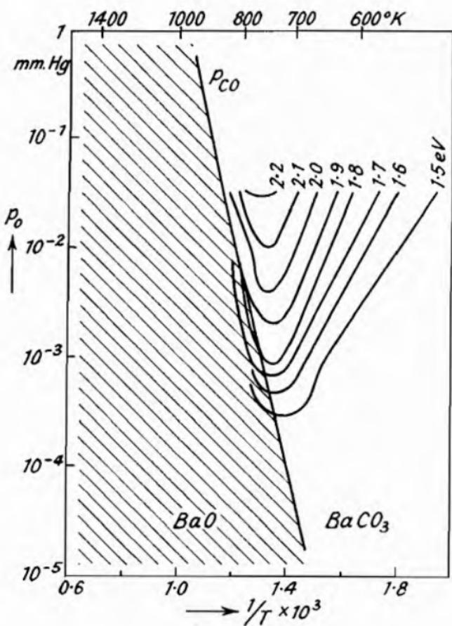
Fig. 145.—Pressure-Temperature Diagram showing Curves of Equal Work Function for Poisoning by Carbon Monoxide after 10 Minutes Exposure. The Dashed Line represents the Equilibrium between  $\text{BaO}$  and  $\text{CO}$  (Herrmann and Krieg<sup>2</sup>).
