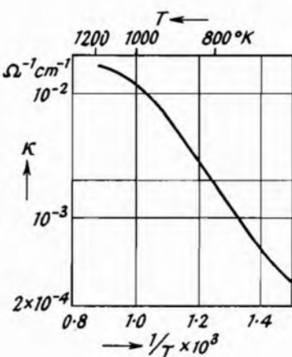
Fig. 76.—Conductivity of ZnO as a Function of Temperature (Miller<sup>1</sup>).
