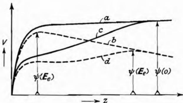
Fig. 42.—Schematic Plot of the Potential of an Electron in front of a Metal Surface
