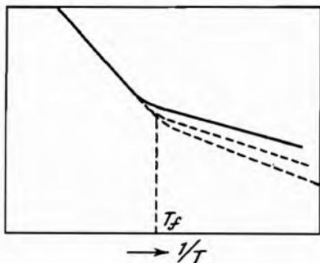
Fig. 66.—Ionic Conductivity as a Function of Temperature (Schematically)
