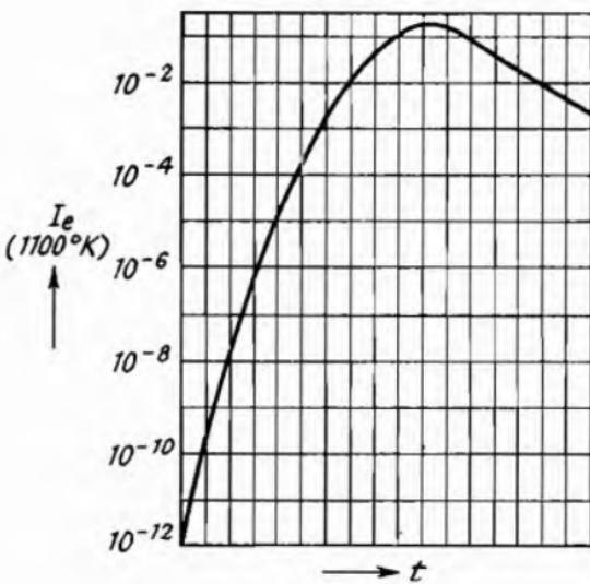
Fig. 84.—Variation of the Emission Current of a Tungsten Ribbon during the Heating of an Oxide Cathode, arranged opposite to the Ribbon (Becker<sup>1</sup>).
