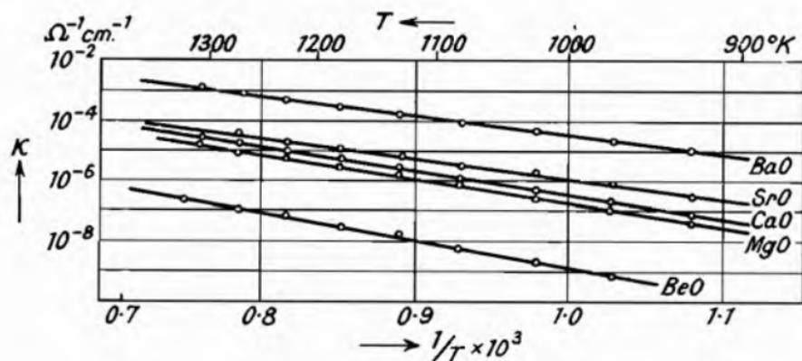
Fig. 102.—Electrical Conductivity of Different Alkaline Earth Oxides as a Function of Temperature (Spanner<sup>1</sup>).
