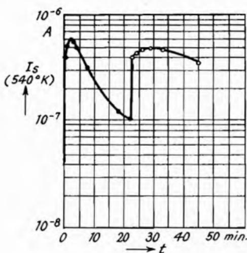
Fig. 86.—Variation of the Saturated Current of an Oxide Cathode during Bombardment by Electrons and Subsequent Heating at  $800^\circ$  K. (Becker<sup>1</sup>).
