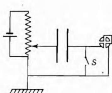
Fig. 51.—Circuit for Measuring the Contact Potential according to Lord Kelvin (Gericke<sup>1</sup>).
