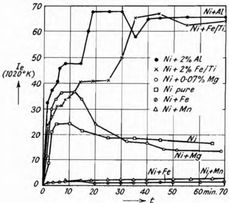
Fig. 130.—Variation of the Emission Current during the Activation by Reduction of Cathodes with Nickel Cores alloyed with Different Materials in Small Quantities (Benjamin<sup>2</sup>).
