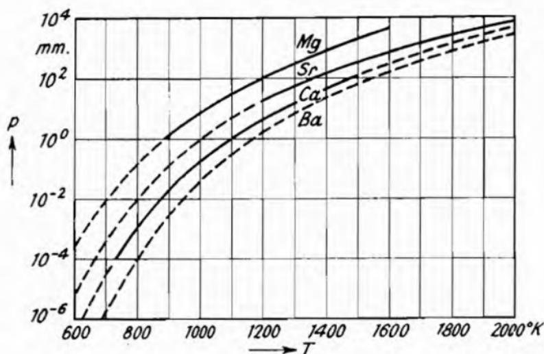
Fig. 82.—Vapour Pressure  $p$  of Alkaline Earth Metals as a Function of Temperature.*Crystallographic Properties of Alkaline Earth Carbonates*
