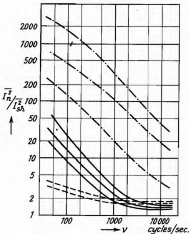
Fig. 153.—Ratio between Mean Square of Noise Current  $\overline{I_n^2}$  and Mean Square of Shot Current  $\overline{I_{sh}^2}$  of Oxide Cathodes as a Function of Frequency  $\nu$  (Graffunder<sup>1</sup>).
