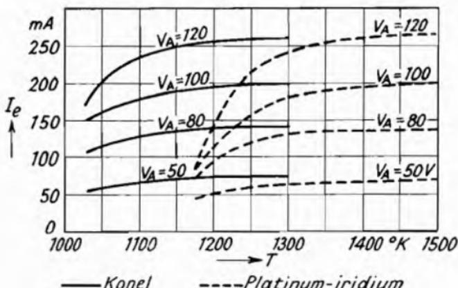
Fig. 148.—Emission Current of Oxide Cathodes with Platinum-Iridium Core or with Konel Core as a Function of Temperature (Lowry<sup>1</sup>).
