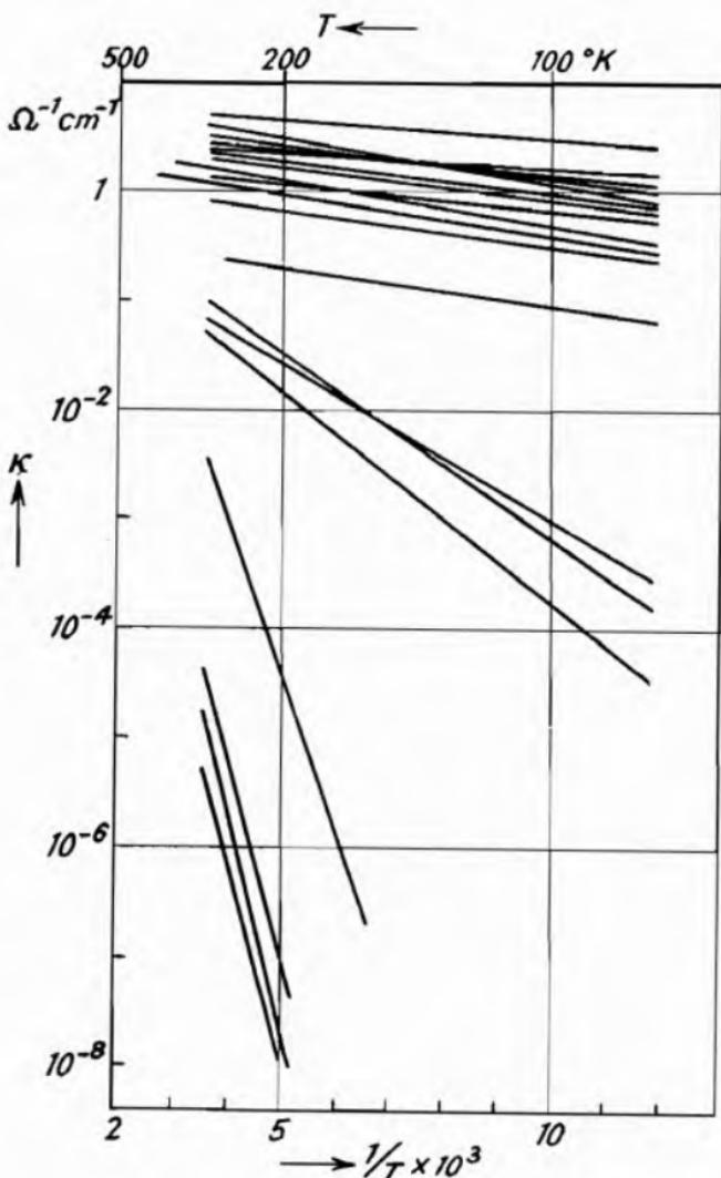
Fig. 80.—The conductivity  $\kappa$  of a Semi-conductor as a Function of Temperature for Different Densities of Excess Atoms: ZnO (Fritsch<sup>1</sup>).
