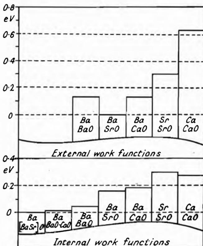
Fig. 123.—Differences between Internal and External Work Functions of differently composed Oxide Cathodes according to Huber.<sup>1</sup>
