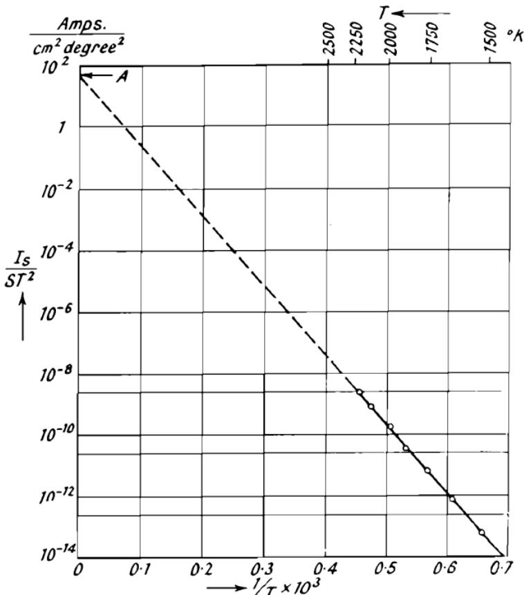
Fig. 48.—Richardson Line for Tungsten.
