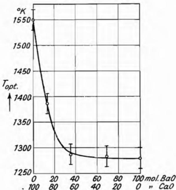
Fig. 132.—Optimum Activation Temperature  $T_{opt}$  as a Function of the Composition of a BaO-CaO Mixture (Huber<sup>1</sup>).
