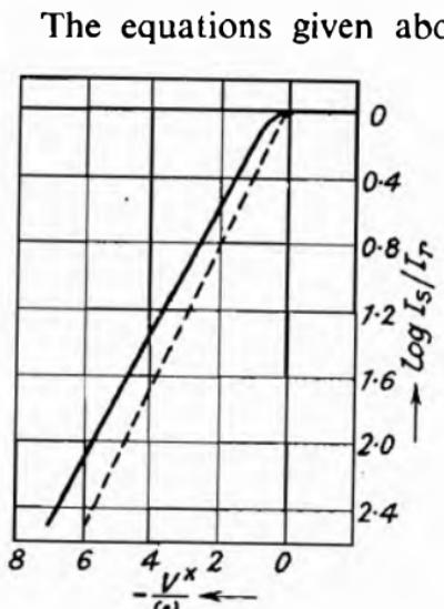
Fig. 18.—Calculated Retarding Field Current in a Cylindrical (full line) and a Plane Field (dashed line). (Rothe-Kleen, Vol. I, Fig. 5.)
