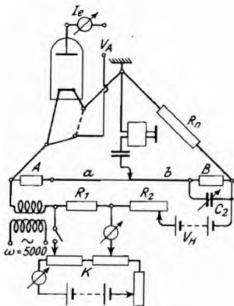
Fig. 50.—Principal Circuit for Measuring the Cooling Power.
