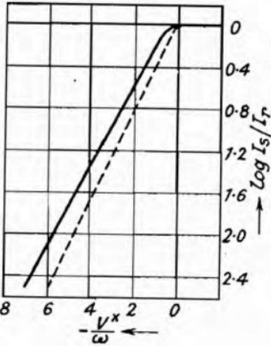
Fig. 18.— Calculated Retarding Field Current in a Cylindrical (full line) and a Plane Field (dashed line). (Rothe-Kleen, Vol. I, Fig. 5.)
