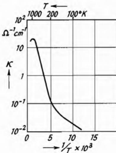
Fig. 81.—Conductivity  $\kappa$  of Silicon Carbide as a Function of Temperature (Busch<sup>1</sup>).
