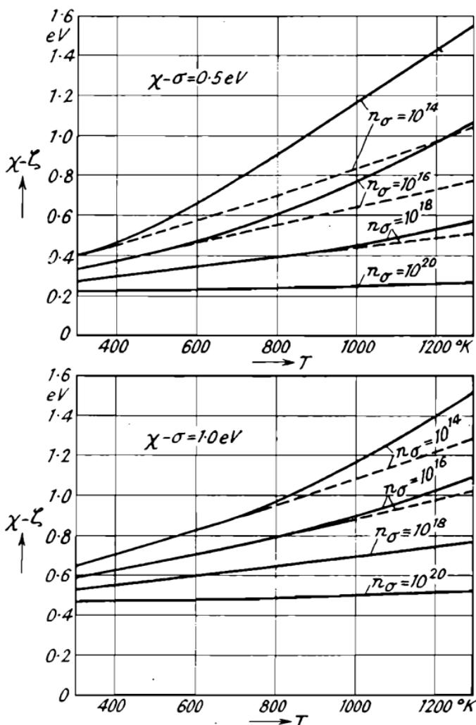
Fig. 75.—Internal Work Function  $\chi - \zeta$  of a Semi-conductor as a Function of Temperature. Exact Values full lines, Approximate Values, broken lines.
