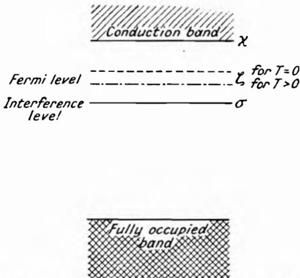
Fig. 74.—The Highest Energy Bands and Levels in an excess Semi-conductor.
