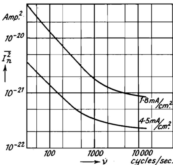
Fig. 154.—Mean Square of Noise Current as a Function of Frequency for Different Densities of the Saturated Current (Graffunder<sup>1</sup>).
