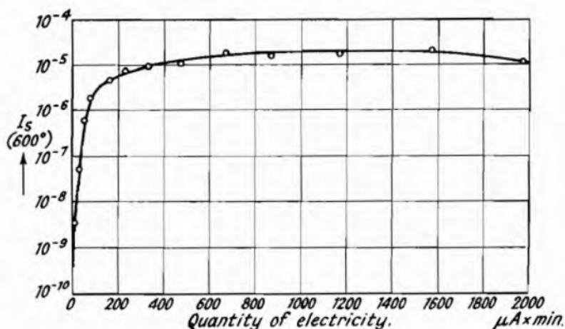
Fig. 151.—Variation of the Saturated Current of a SrO Cathode during Bombardment by Electrons (Becker<sup>1</sup>).
