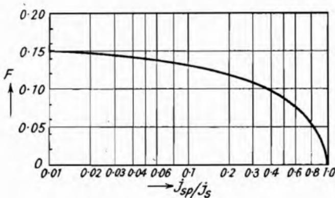
Fig. 21.—Factor  $F$ , necessary for Evaluation of the Distance between Cathode and Potential Barrier due to Space Charge.
