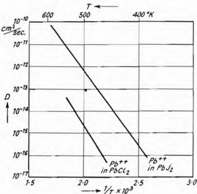
Fig. 65.—Diffusion Coefficient  $D$  of  $\text{PbCl}_2$  and  $\text{PbI}_2$  as a Function of Temperature (Hevesey and Seith,<sup>1</sup> Seith<sup>2</sup>).
