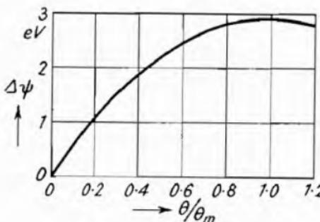
Fig. 32.—Variation  $\Delta\psi$  of the Work Function of a W-Cs Cathode as a Function of the Fraction  $\theta$  covered with Cæsium (Langmuir and Taylor<sup>8</sup>).
