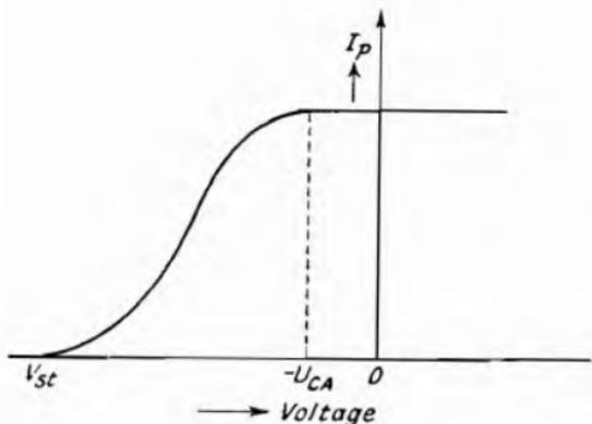
Fig. 55.—Photo-electric Current as a Function of a Retarding Voltage (Schematic).
