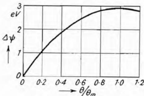
Fig. 32.—Variation  $\Delta\psi$  of the Work Function of a W-Cs Cathode as a Function of the Fraction  $\theta$  covered with Caesium (Langmuir and Taylor<sup>8</sup>).
