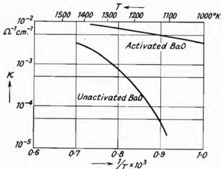
Fig. 103.—Electrical Conductivity of BaO as a Function of Temperature for Different States of Activation (High-Temperature Range) (Meyer and Schmidt<sup>1</sup>).
