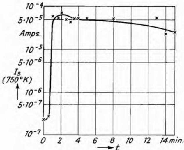
Fig. 122.—Variation of the Saturated Current of a SrO Cathode, when Evaporating Barium on the Surface (Huber<sup>1</sup>).
