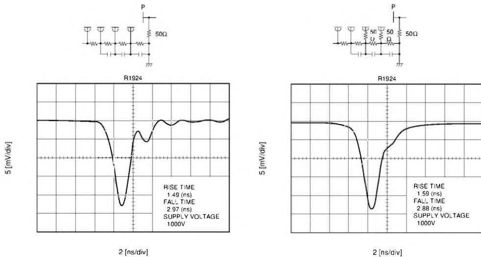
**Figure 5-13: Effect of damping resistors on ringing**
