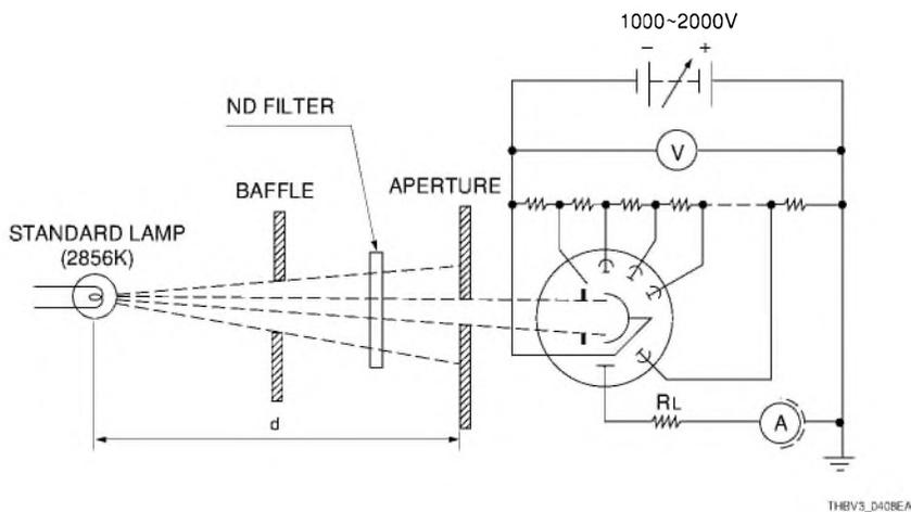
Figure 4-8: Anode luminous sensitivity measuring diagram
