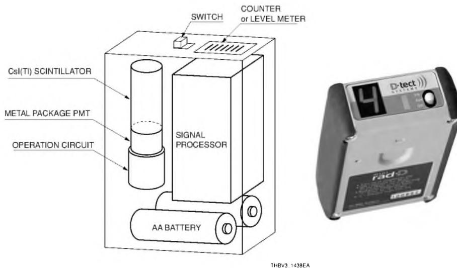
Figure 14-38: Structural view of a handheld radiation monitor
