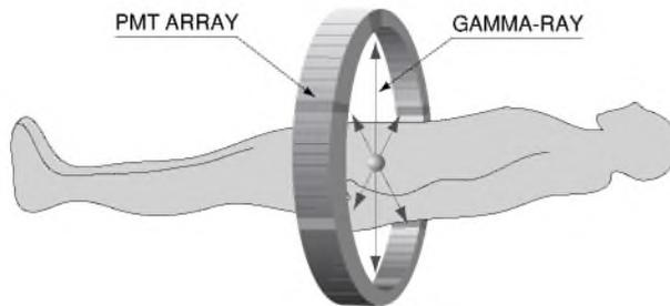
Figure 14-8: Concept view of a PET scanner
