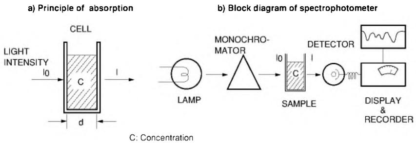
**Figure 14-2: Principle and block diagram of a spectrophotometer**
