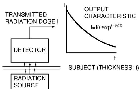
**Figure 14-40: Principle of a transmission-mode thickness gauge**
