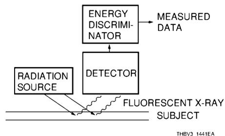
**Figure 14-41: Principle of a fluorescent X-ray thickness gauge**
