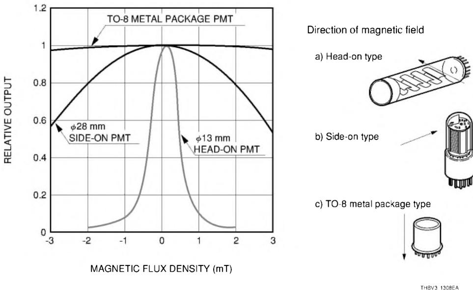
**Figure 13-8: Magnetic characteristics of typical photomultiplier tubes**
