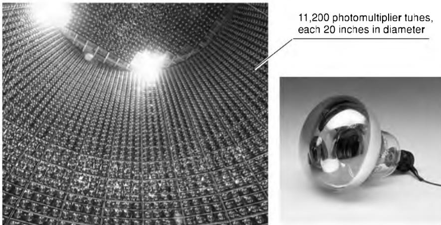
Figure 14-31: Interior of Super-Kamiokande detector tank lined with 20-inch PMT
