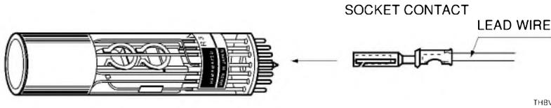
**Figure 5-47: Connecting the lead pins to the socket contacts**
