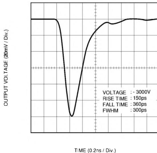
Figure 10-6: Pulse response waveform of MCP-PMT (R3809U-50)
