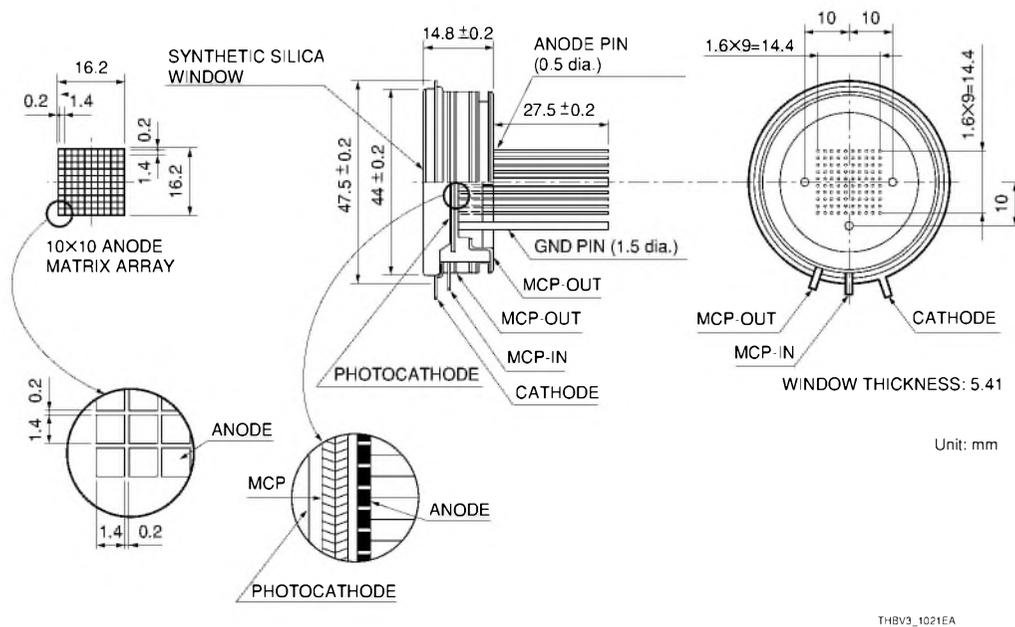
Figure 10-21: Multianode MCP-PMT with 10x10 anode format
