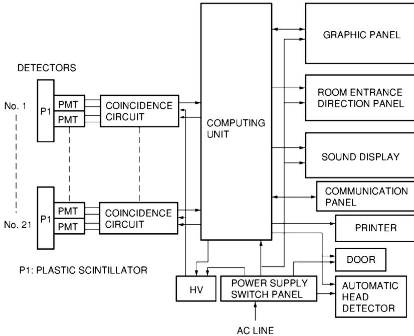
Figure 14-39: Block diagram of a door monitor
