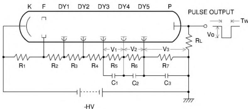
Figure 5-8 (1): Divider circuit with serial-connected decoupling capacitors
