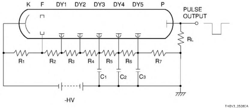
**Figure 5-8 (2): Voltage-divider circuit with parallel-connected decoupling capacitors**
