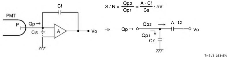
Figure 5-34: Influence of input distribution capacitance
