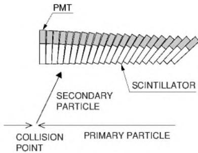
Figure 14-29: Calorimeter setup
