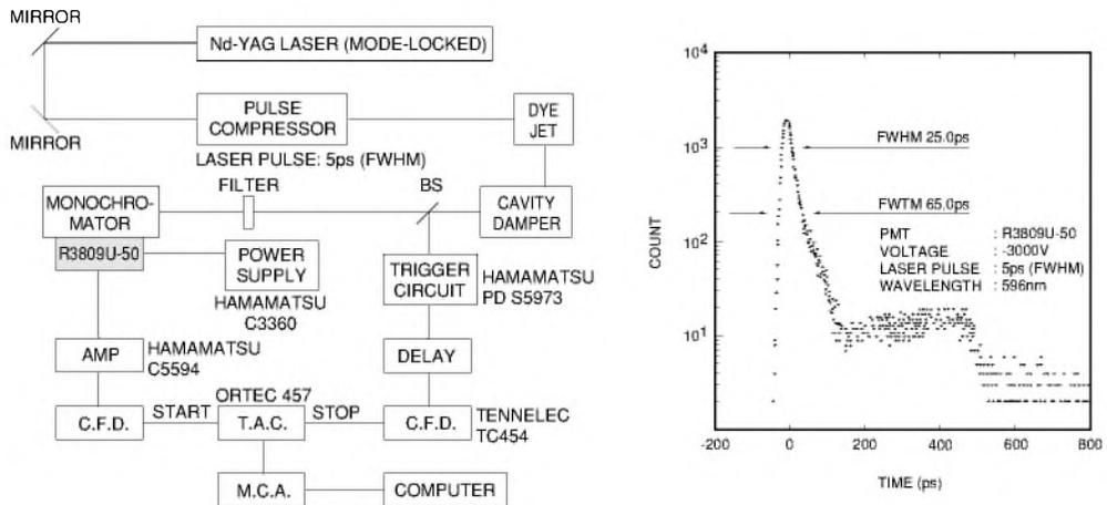
Figure 10-8: Accurate TTS measurement of MCP-PMT (R3809U-50)
