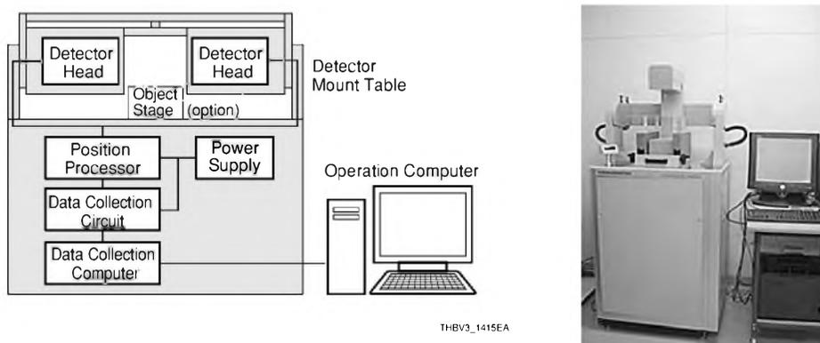
Figure 14-15: Block diagram and external view of a planar imaging device
