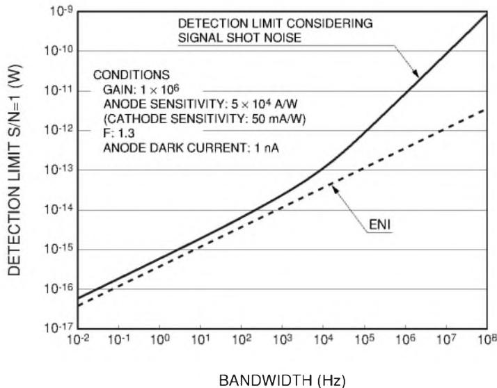
Figure 4-44: Detection limit considering signal shot noise component
