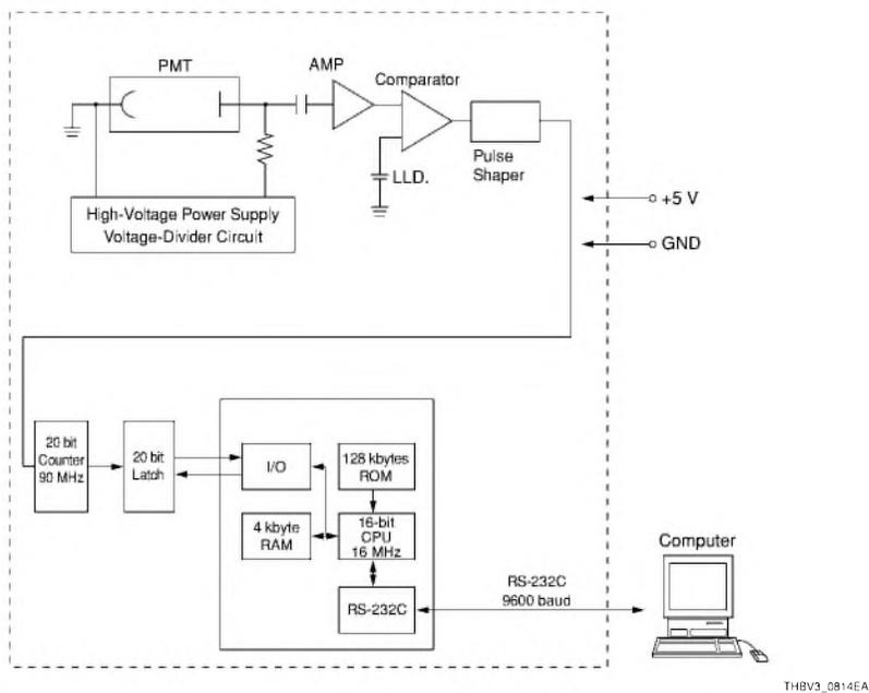
Figure 8-14: Block diagram of photon counting type module
