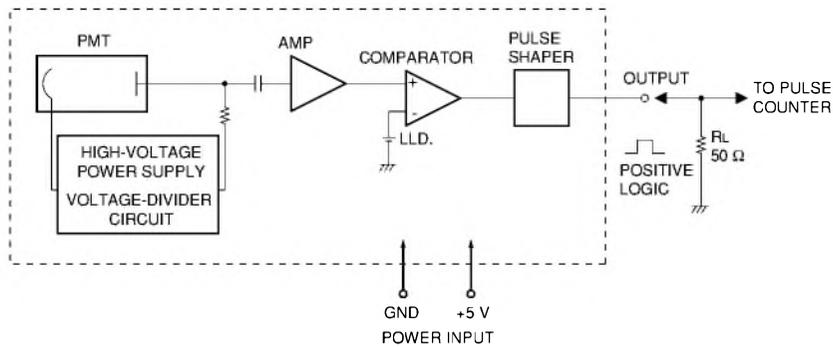
Figure 8-8: Block diagram of photon counting head
