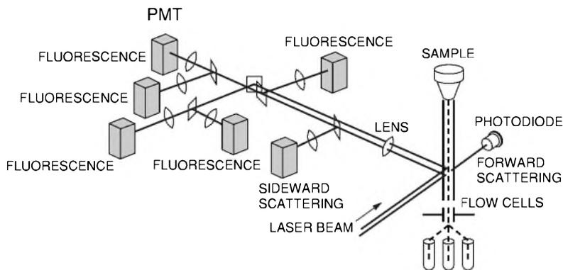
Figure 14-22: Major components of a flow cytometer
