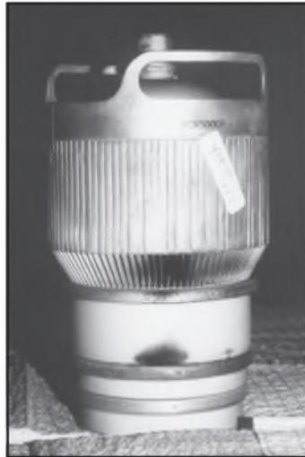
**Figure 9.19** The interior elements of a 4CX15000A tube that had gone to air while the filament was lit. (*Courtesy of Econco.*)
