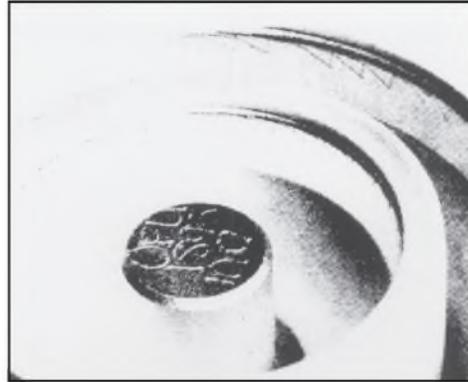
**Figure 9.11** Damage to the grid contact of a power tube caused by insufficient fingerstock pressure. (Courtesy of Varian.)
