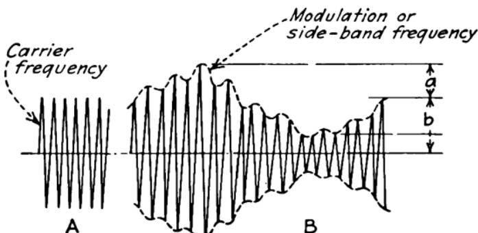
FIG. 257.—Carrier and modulation frequencies.
