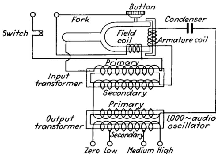
FIG. 209.—Circuit of audio-frequency oscillator.
