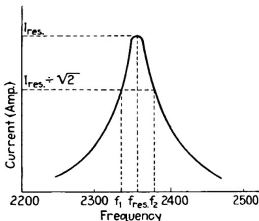
FIG. 35.—Typical resonance curve.
