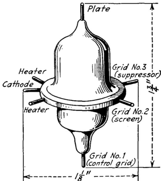
FIG. 128.—Midget pentode tube (type 954).
