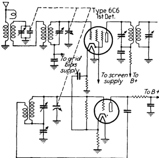
FIG. 407.—Typical all-wave superheterodyne oscillator circuit.
