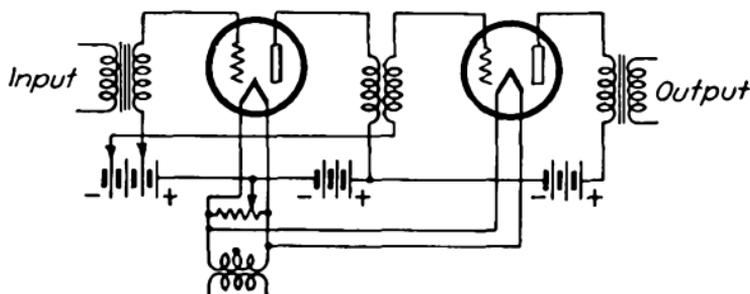
FIG. 375.—Transformer-coupled amplifier.
