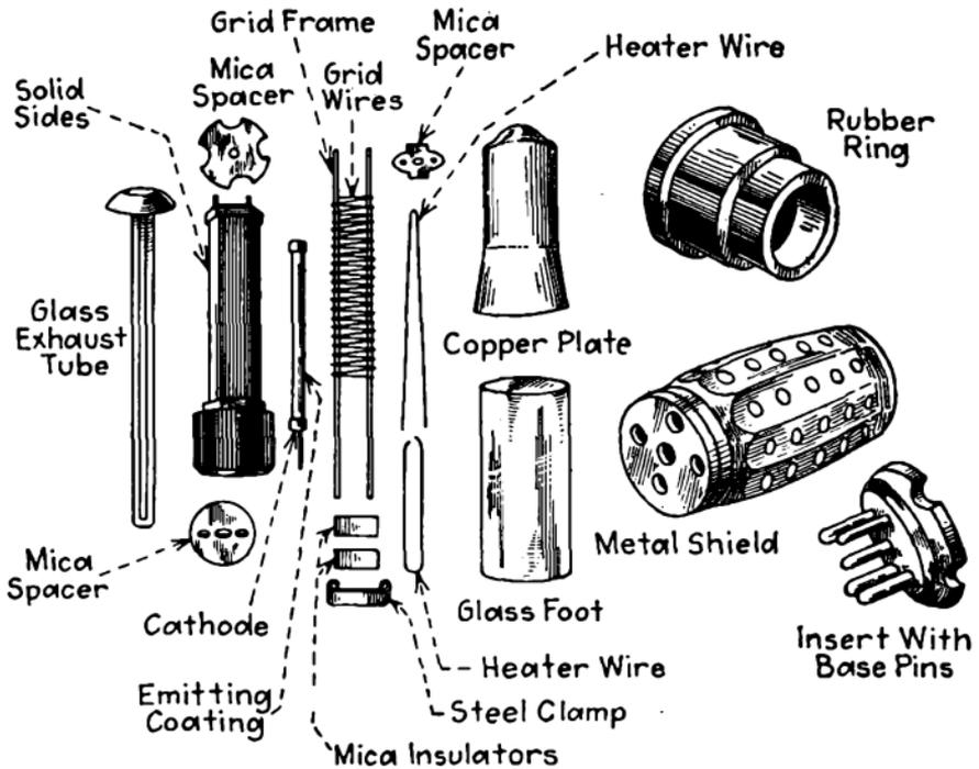
FIG. 107.—Parts of Catkin metal screen-grid tube.
