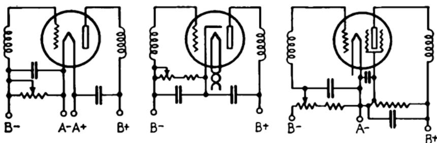
FIG. 251.—Grid-bias voltage variation for volume control.
