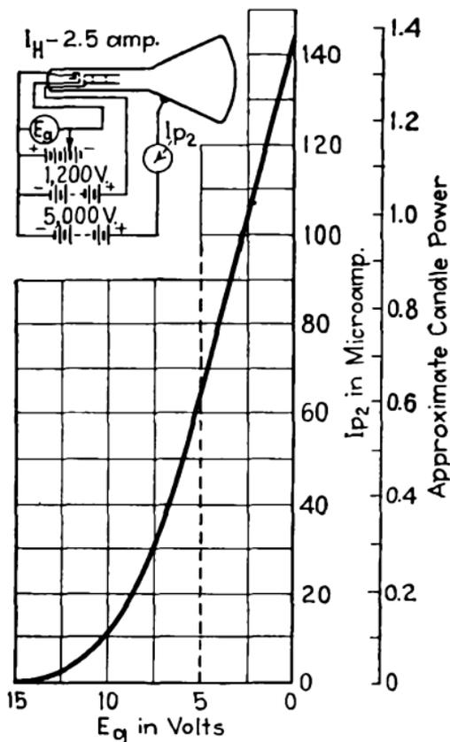
FIG. 441.—Characteristic curve of kinescope.
