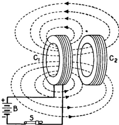
FIG. 31.—Mutual induction between two coupled coils.
