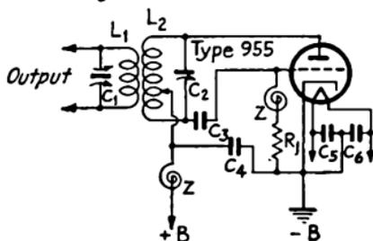
$L_1 C_1, L_2 C_2 =$  Depend on frequency range desired.
