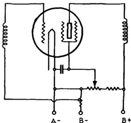
FIG. 253.—Volume-control arrangement using screen-grid voltage variation.
