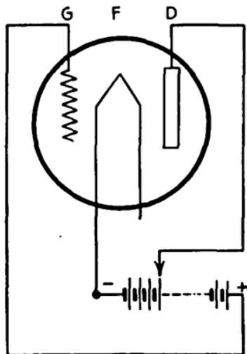
FIG. 185.—Dynatron connection for a three-element tube.
