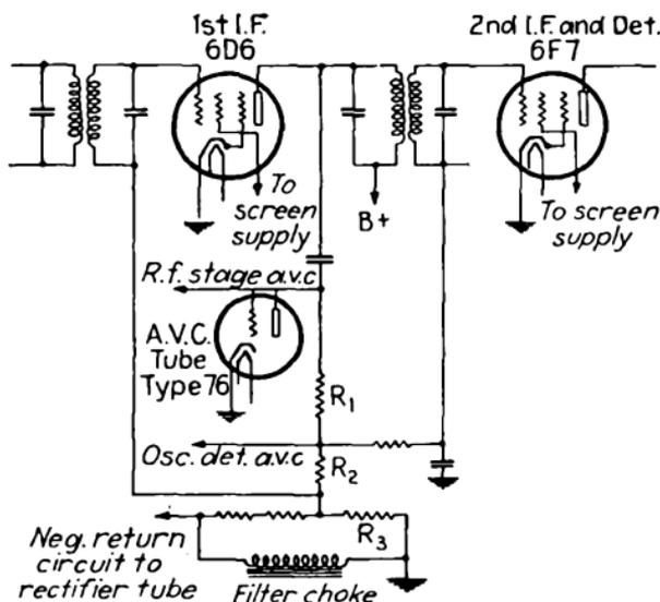
FIG. 358.—Retroactive circuit for automatic volume control.
