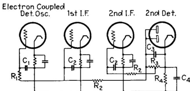
FIG. 361.—Circuit providing grid-bias voltage for automatic volume control on intermediate-frequency stages.
