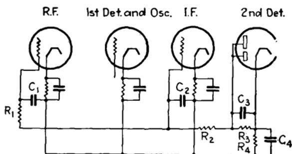
FIG. 359.—Circuit details for automatic volume control.
