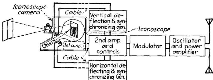
FIG. 438.—Iconoscope transmitting equipment.
