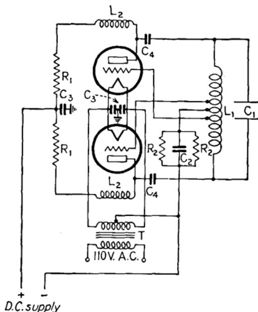
FIG. 415.—Oscillating push-pull circuit for three-electrode tubes.
