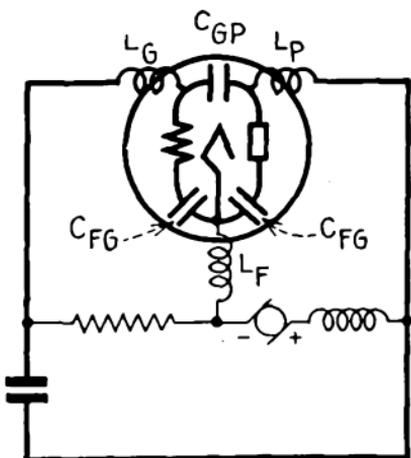
FIG. 418.—Limiting circuit of Colpitts oscillator.
