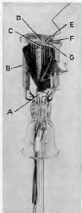
FIG. 93.—Pentagrid converter.
