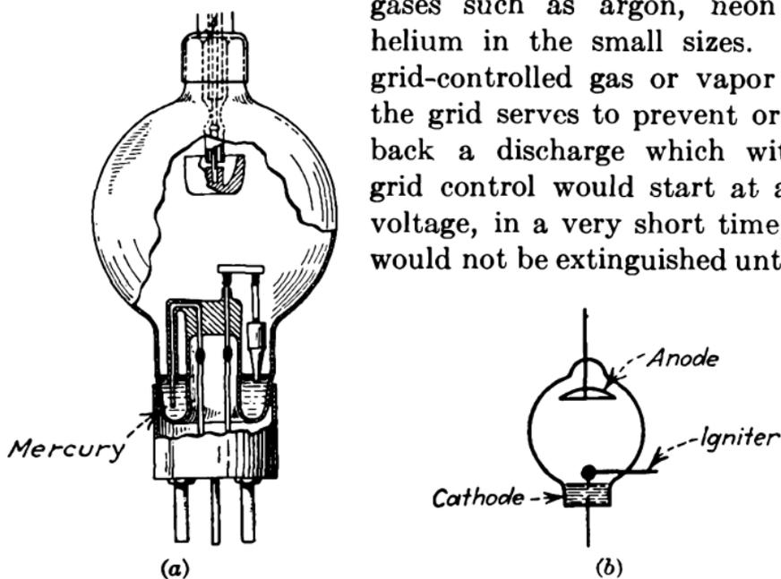
FIG. 155.—Essential parts of ignitron tube.
