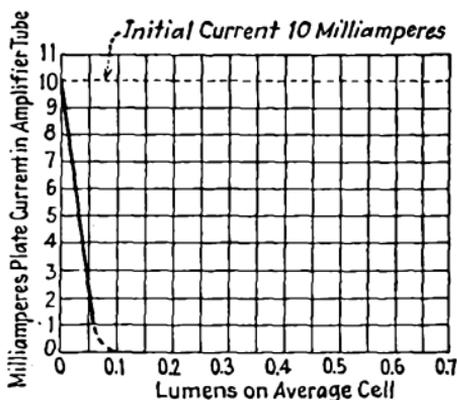
FIG. 382.—Response curve of reverse circuit.
