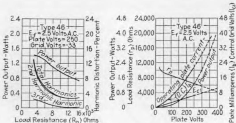
FIG. 69.—Operation characteristics of type 46 tube.
