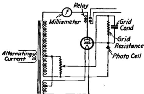
FIG. 385.—Reverse circuit for alternating-current operation
