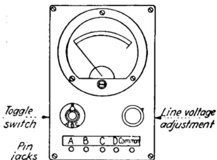
FIG. 205.—Hickok capacity meter.
