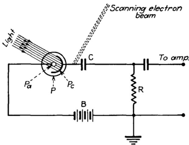
FIG. 429.—Circuit of photoelectric elements in iconoscope.
