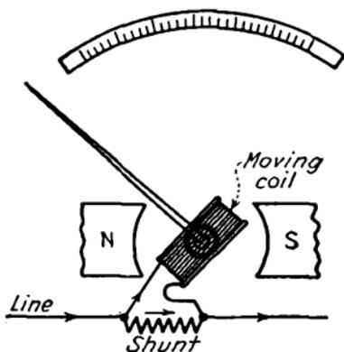
FIG. 194.—Direct-current ammeter with shunt connection.
