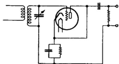
FIG. 266.—Simple diode-detector circuit.
