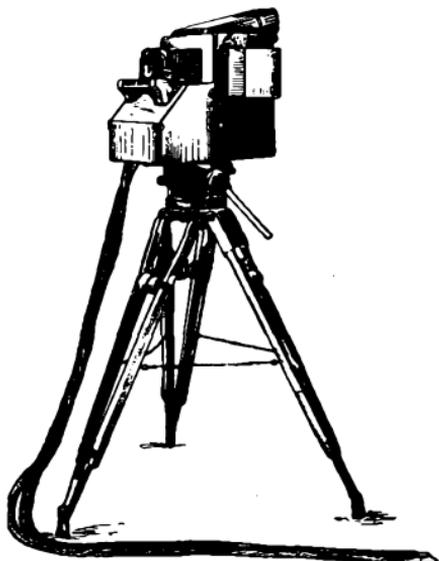
FIG. 437.—Portable iconoscope camera and pick-up equipment.
