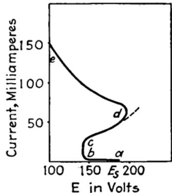
FIG. 158.—Relation of voltage to current in cold-cathode glow lamp.
