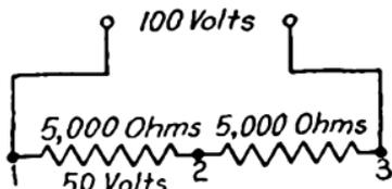
FIG. 191.—Simple electric circuit including two equal resistances.
