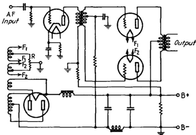
FIG. 250.—Circuit for semi-fixed grid-bias method.
