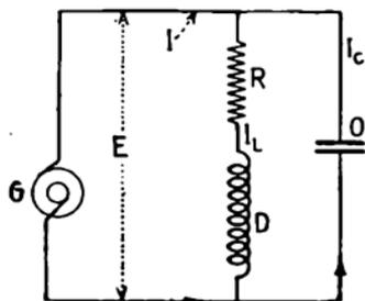
FIG. 36.—Parallel resonance of inductance and condenser.
