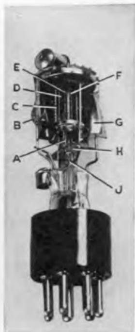
FIG. 99.—Triode-pentode tube.
