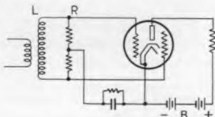
FIG. 71.—Detector circuit for Wunderlich tube.
