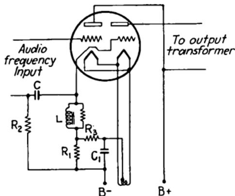
FIG. 80.—Conventional circuit for triple-twin tube.
