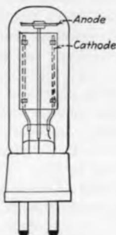
FIG. 172.—Elements of photoelectric tube.
