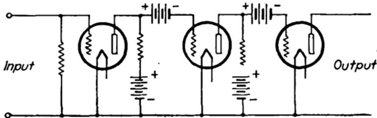
FIG. 370.—Typical direct-coupled amplifier.
