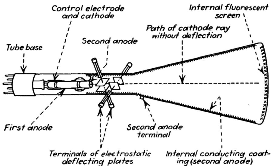
FIG. 183.—Typical cathode-ray tube.
