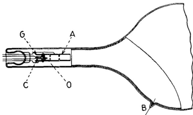
FIG. 434.—Electron gun of iconoscope.
