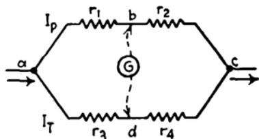
FIG. 204.—Typical Wheatstone-bridge circuit.
