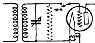
FIG. 363.—Methods of stabilizing circuits by use of grid-bias voltage to prevent oscillation.
