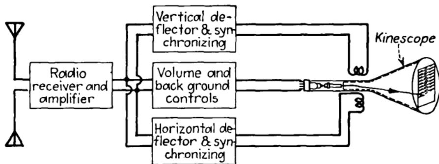
FIG. 439.—Iconoscope receiving equipment.
