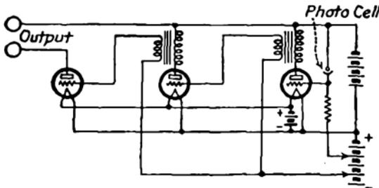
FIG. 390.—Transformer-coupled amplifier including photoelectric tube.
