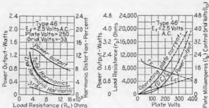
FIG. 69.—Operation characteristics of type 46 tube.
