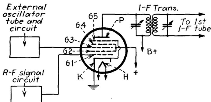
FIG. 108b.—Circuit diagram for type 6L7 tube.
