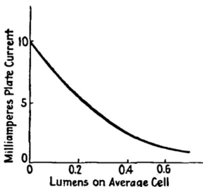
FIG. 386.—Response curve of circuit in Fig. 385.
