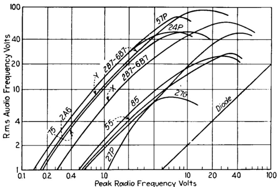
FIG. 275.—Average performance of typical detector tubes.
