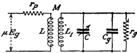
FIG. 362.—Equivalent circuit of tuned radio-frequency stage.
