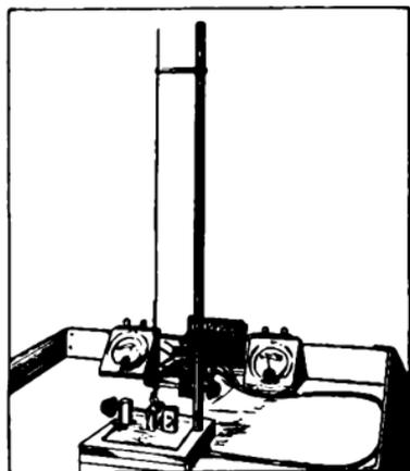
FIG. 121.—Transmitter for 100-centimeter wave lengths.
