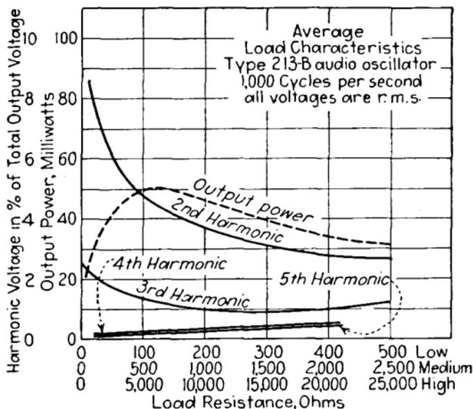
FIG. 210.—Load characteristics of audio-frequency oscillator.
