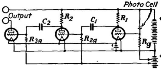
FIG. 389.—Condenser-coupled amplifier including photoelectric tube.
