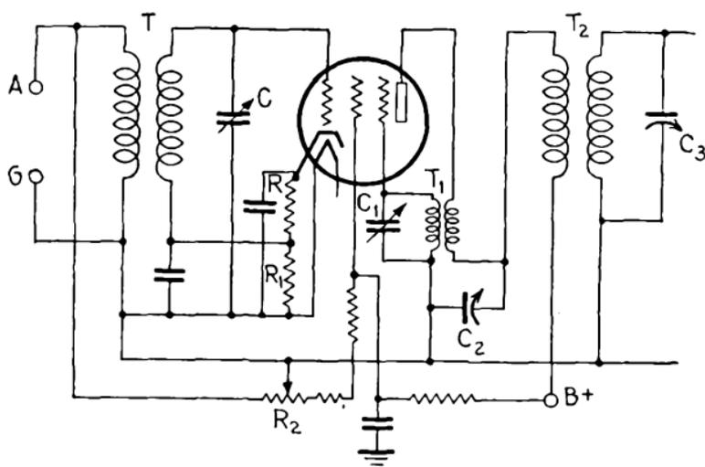
FIG. 409.—Triple-grid tube in oscillator-mixer circuit.
