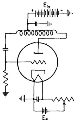
FIG. 119.—Circuit of small triode oscillator.
