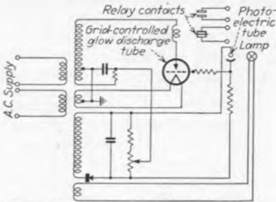
FIG. 448.—Circuit of photoelectric controller.
