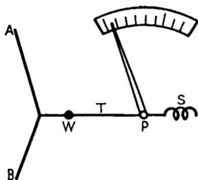
FIG. 197.—Hot-wire ammeter.
