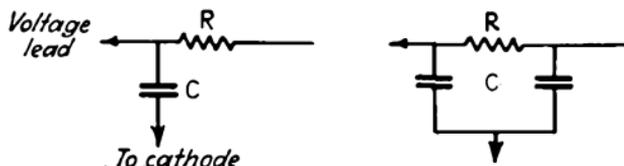
FIG. 254.—Electric filters for voltage-supply wires.
