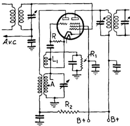
FIG. 408.—Triode-pentode tube in oscillator-mixer circuit.
