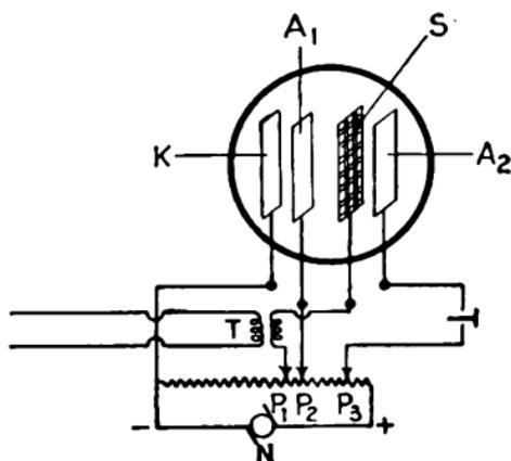
FIG. 167.—Typical circuit for amplification of cold-electrode tube.
