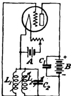
FIG. 397.—Simple oscillator for producing alternating current.
