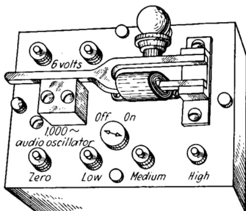
FIG. 208.—Audio-frequency oscillator. (*General Radio.*)
