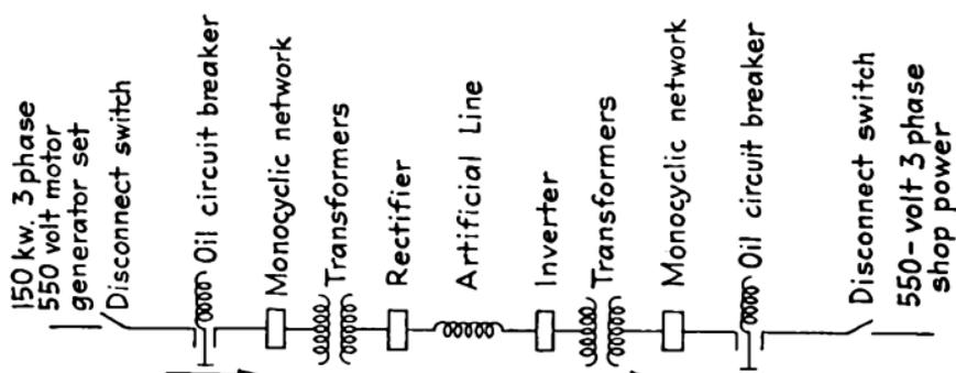
FIG. 471.—Direct-current constant-current transmission system.
