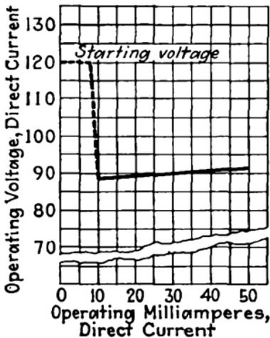
FIG. 163.—Regulation characteristics of UX-874 tube.
