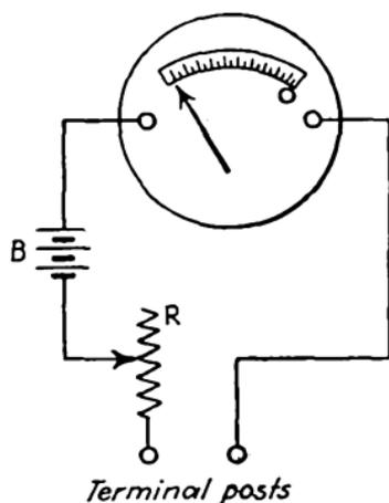
FIG. 199.—Simple ohmmeter.
