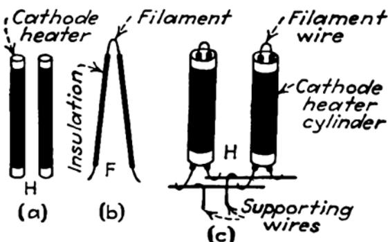
FIG. 10.—Construction of cathode heaters.
