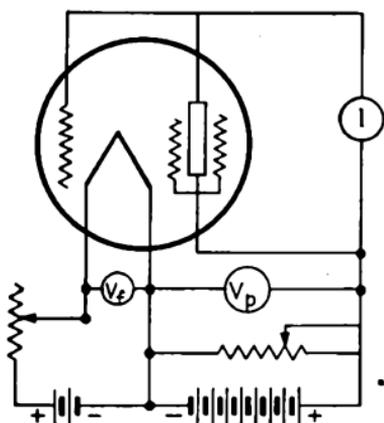
FIG. 215.—Typical circuit for emission testing.
