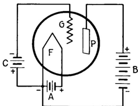
FIG. 44.—Conventional representation of three-element tube.
