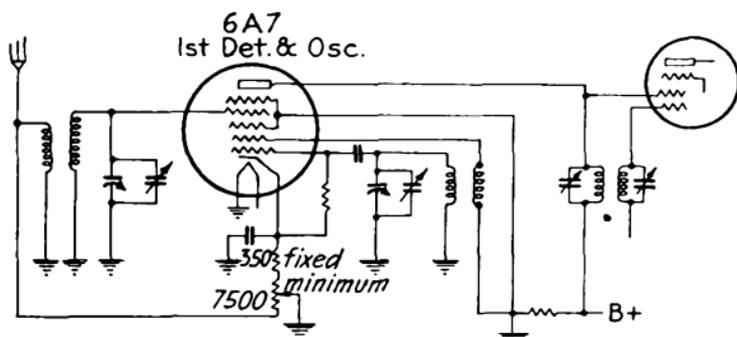
FIG. 350.—Circuit for manual volume control.
