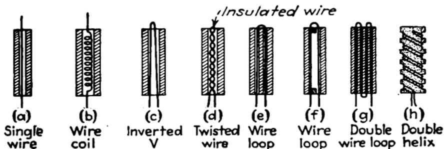
FIG. 5.—Tungsten heating elements.
