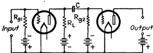
FIG. 374.—Resistance-coupled amplifier.
