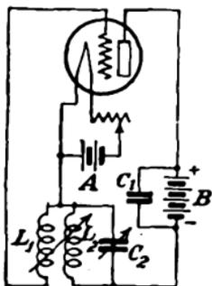
FIG. 397.—Simple oscillator for producing alternating current.
