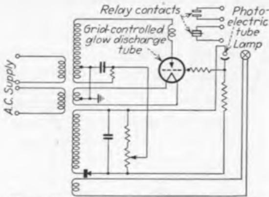
FIG. 448.—Circuit of photoelectric controller.
