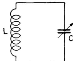
FIG. 411.—Typical radio-frequency circuit in superheterodyne receiver.
