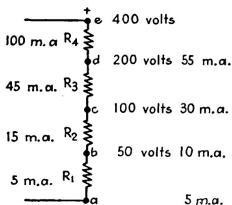
FIG. 312.—Conventional voltage divider.
