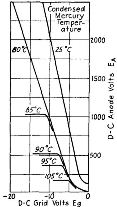
FIG. 138.—Relation of breakdown voltage to grid voltage of gaseous tube (type KU-628).
