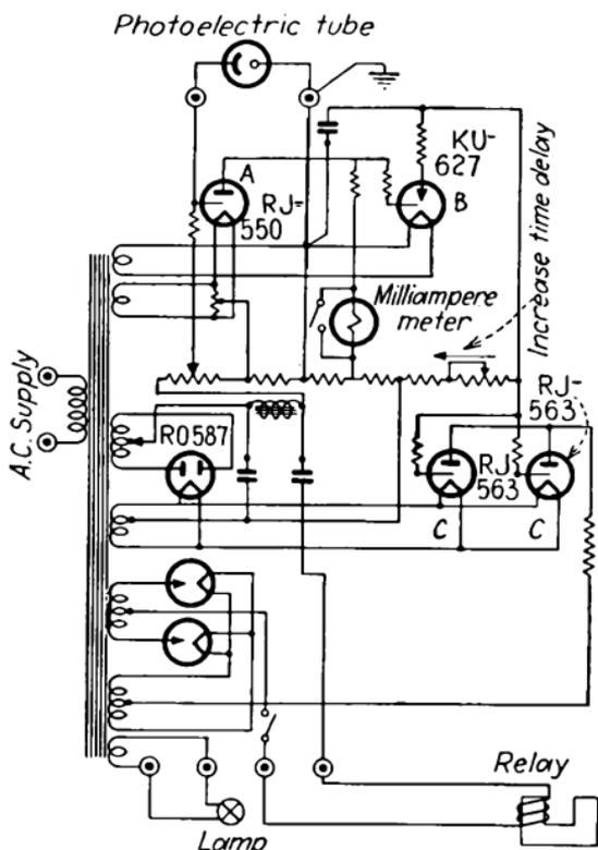
FIG. 451.—Photoelectric controller with time delay.
