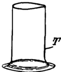
FIG. 6.—Glass support for vacuum tube.
