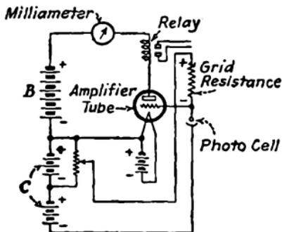
FIG. 381.—Typical direct-current reverse circuit.
