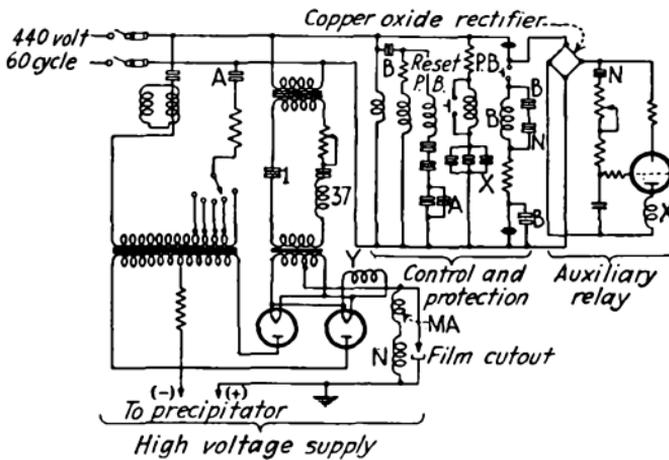
FIG. 458.—Circuit diagram of precipitation apparatus.
