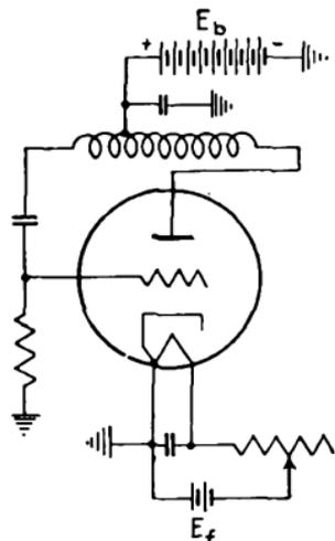
FIG. 119.—Circuit of small triode oscillator.
