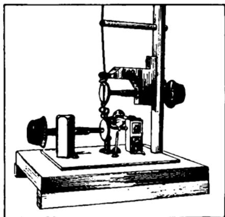
FIG. 120.—Oscillator for 100-centimeter wave lengths.
