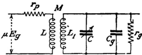
FIG. 362.—Equivalent circuit of tuned radio-frequency stage.
