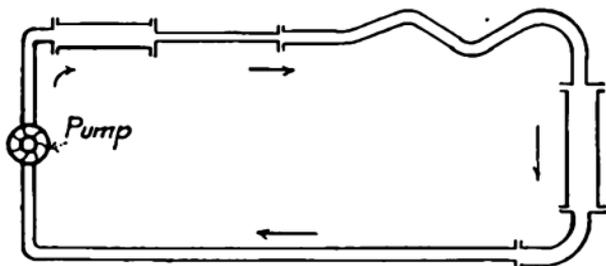
FIG. 18.—Water pipes connected in series.
