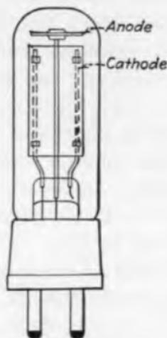
FIG. 172.—Elements of photoelectric tube.
