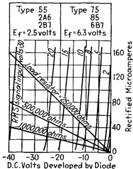
FIG. 84.—Relation of direct-current voltage to rectified current for single diode unit in half-wave rectification.
