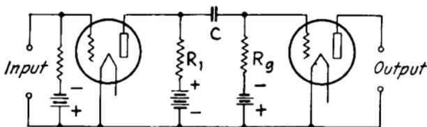
FIG. 343.—Resistance-coupled audio-frequency amplifier.
