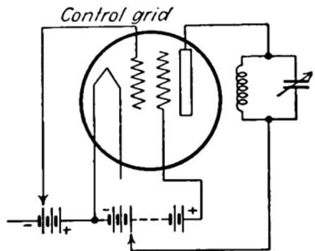
FIG. 187.—Dynatron connection of screen-grid tube to serve as oscillator.
