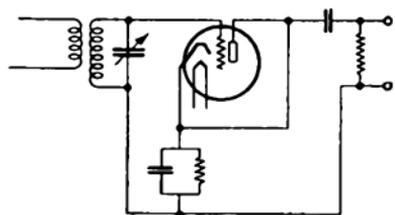
FIG. 266.—Simple diode-detector circuit.
