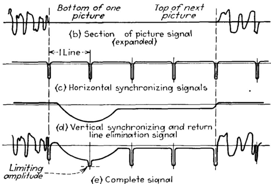
FIG. 445.—Diagram of synchronizing signals in iconoscope.
