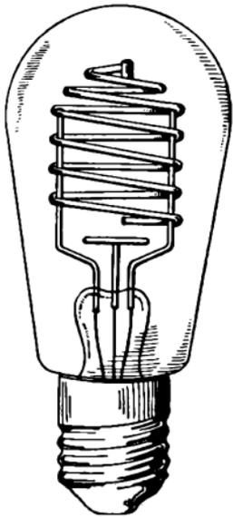
FIG. 156.—Glow lamp with spiral cathode.
