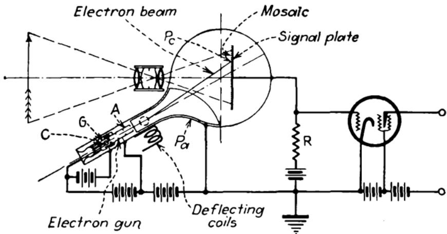
FIG. 428.—Iconoscope circuit.
