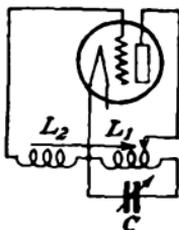
FIG. 401.—Tuned-plate oscillating circuit.
