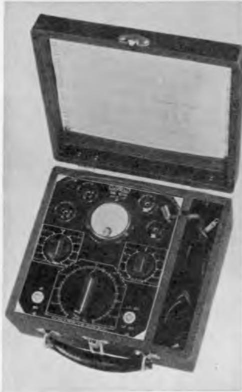
FIG. 241.—Panel of Dayrad Model 14 tube tester.
