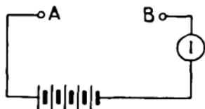
FIG. 211.—Simple circuit for resistance measurements.
