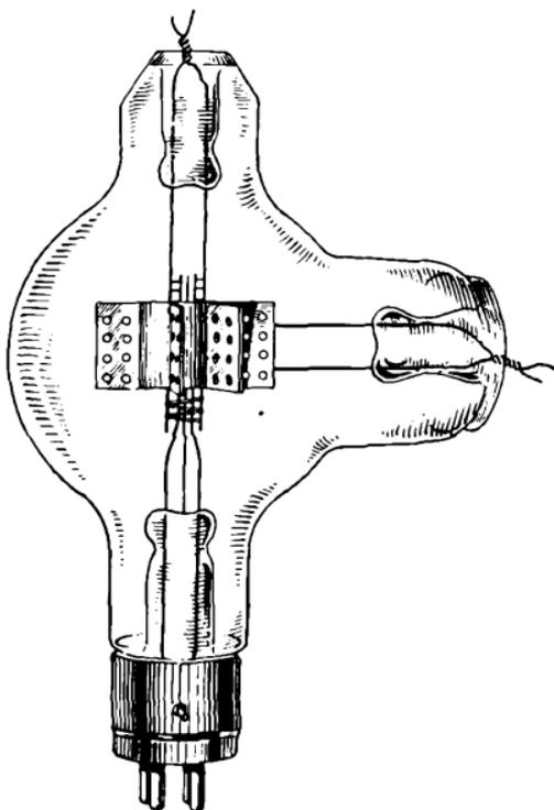
FIG. 419.—Typical air-cooled high-frequency oscillator.
