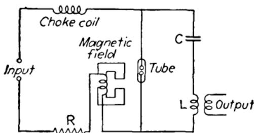
FIG. 477.—General purpose arc-tube circuit.
