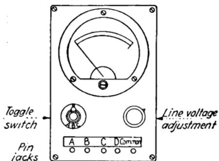
FIG. 205.—Hickok capacity meter.
