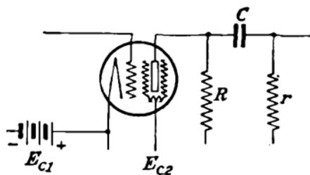
FIG. 284.—Typical circuit using UX-222 tube as detector.
