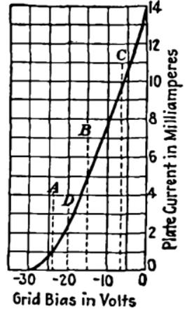
FIG. 379.—Characteristics of typical amplifier tube.
