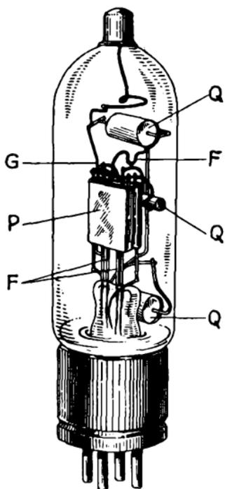
FIG. 109.—Piotron detector tube (FP-54).
