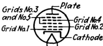
FIG. 94.—Diagram of electrodes in pentagrid converter.
