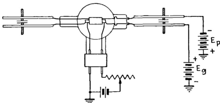
FIG. 424.—Typical positive-grid oscillator circuit.
