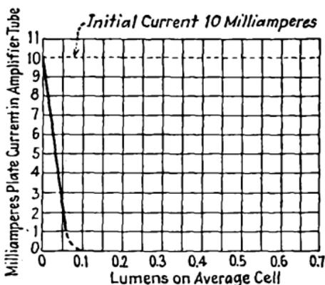
FIG. 382.—Response curve of reverse circuit.
