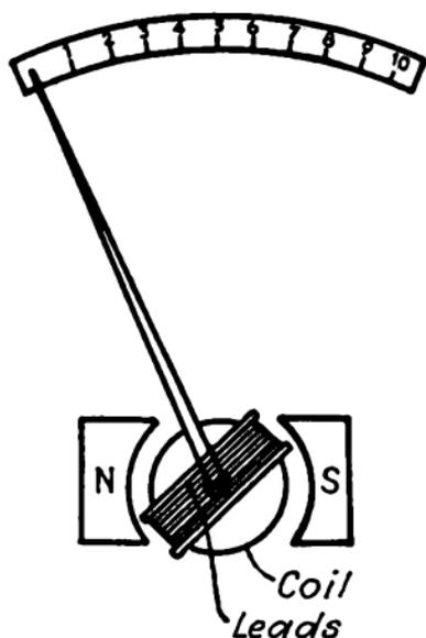
FIG. 190.—Direct-current voltmeter.
