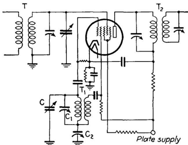
FIG. 410.—Pentagrid-converter tube in oscillator-mixer circuit.
