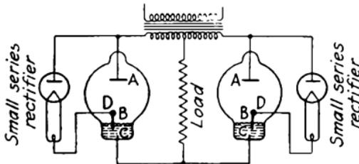
FIG. 315.—Ignitron tube used for full-wave, single-phase rectification.
