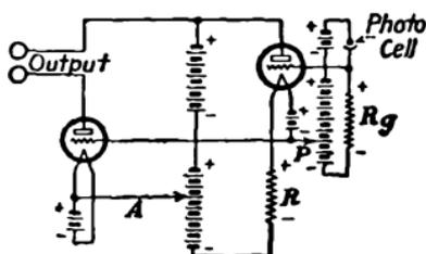
FIG. 388.—Resistance-coupled amplifier including photoelectric tube.
