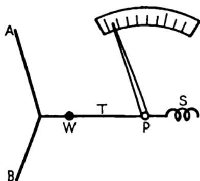
FIG. 197.—Hot-wire ammeter.
