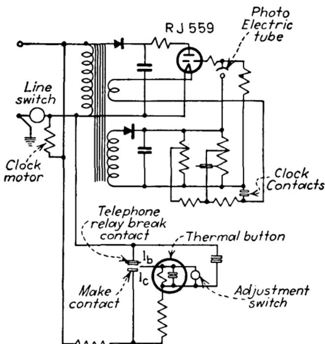
FIG. 452.—Circuit diagram for lighting control.
