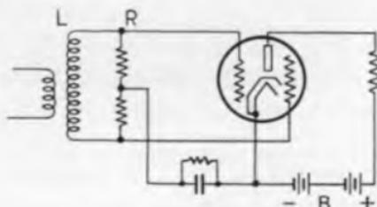
FIG. 71.—Detector circuit for Wunderlich tube.
