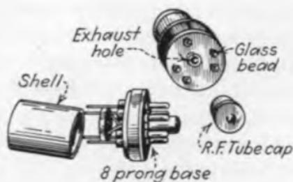
FIG. 106.—Parts of all-metal radio receiving tube.
