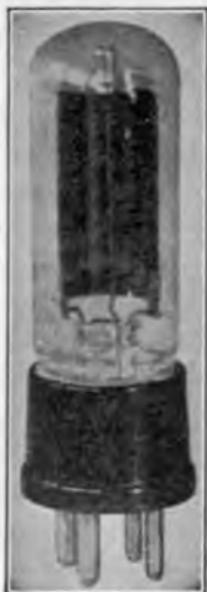
FIG. 171.—Typical photoelectric tube.
