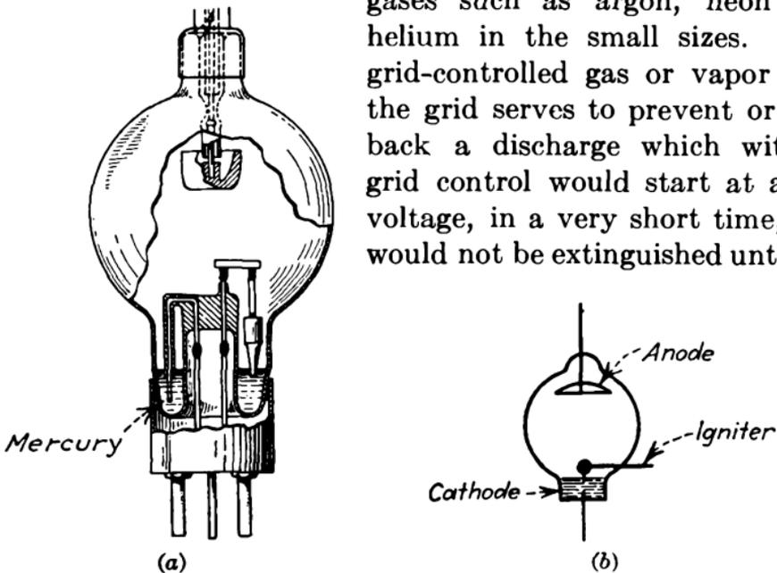
FIG. 155.—Essential parts of ignitron tube.
