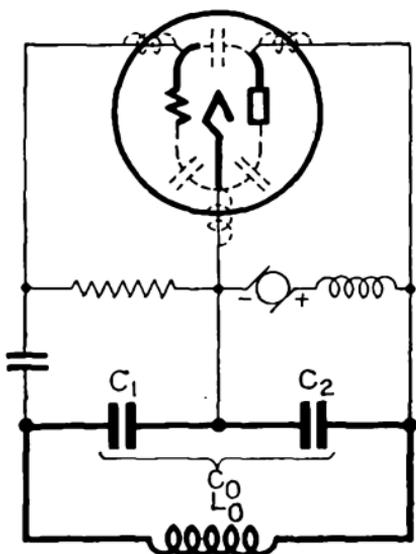
FIG. 417.—Modified Colpitts oscillator circuit.
