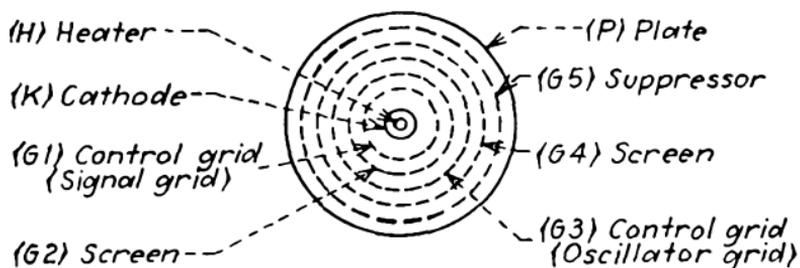
FIG. 108a.—Electrodes in type 6L7 tube.
