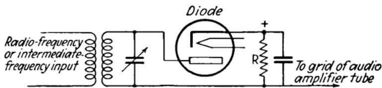
FIG. 259.—Half-wave rectification with diode.
