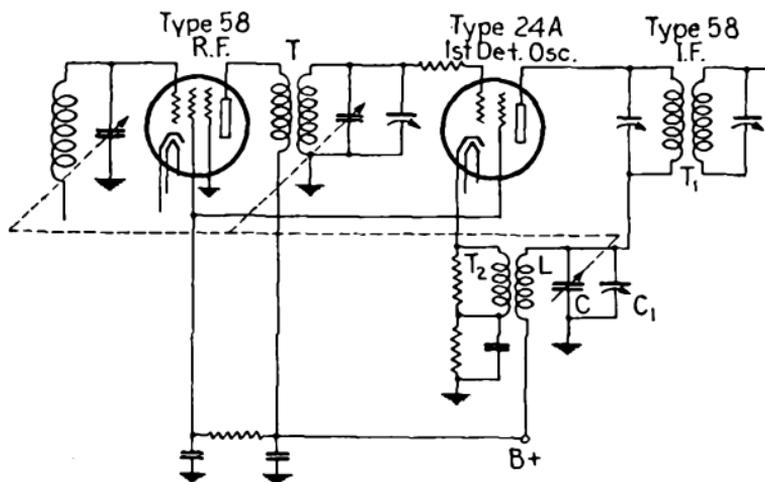
FIG. 406.—Autodyne frequency converter.
