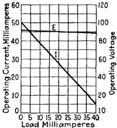
FIG. 164.—Operation characteristics of UX-874 tube.
