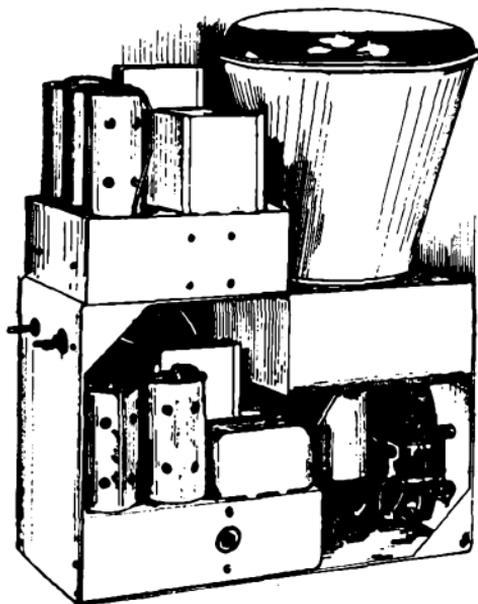
FIG. 446.—Deflecting unit of iconoscope.
