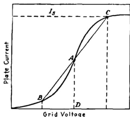
FIG. 404.—Variation of oscillation with grid voltage.
