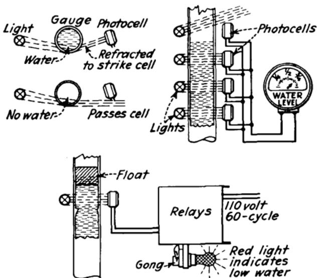
FIG. 469.—Photoelectric water-level indicator.
