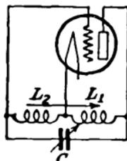
FIG. 399.—Hartley oscillating circuit.
