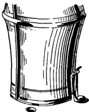
FIG. 486.—Method of grounding metal shield by single-contact spring clip.
