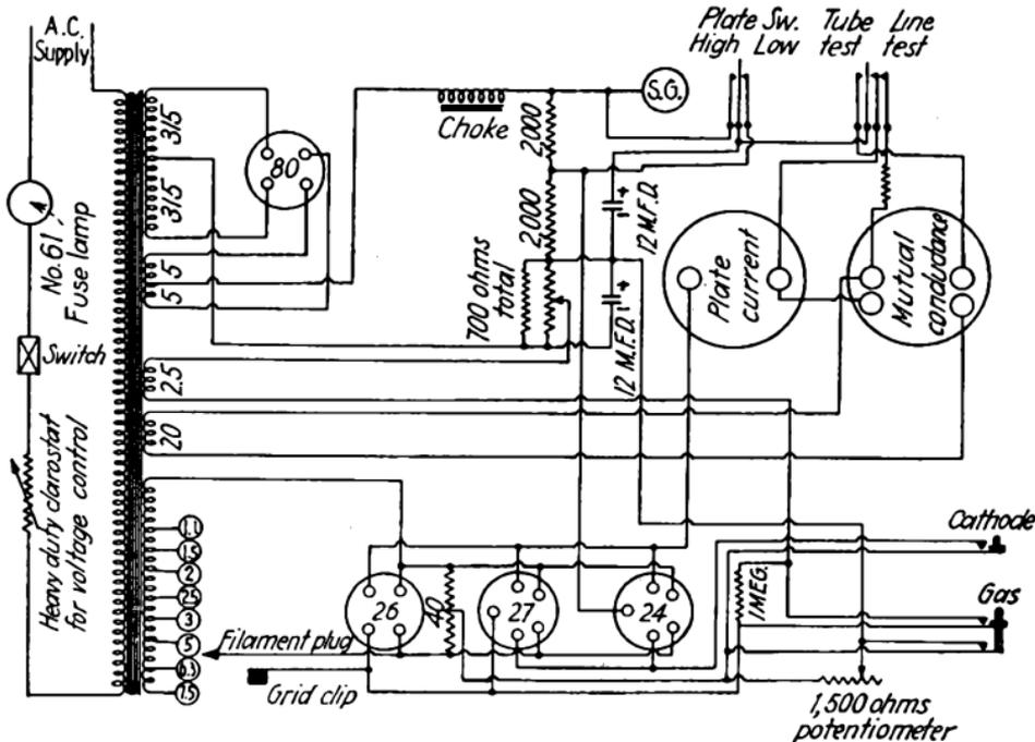
FIG. 235.—Wiring diagram of Hickok Model AC-47 tube tester.
