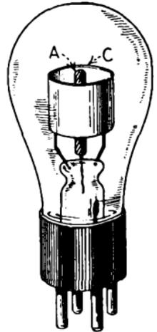
FIG. 162.—Cold-electrode gas-filled, voltage-limiting tube.
