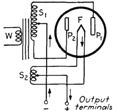
FIG. 289.—Rectifier circuit for full-wave rectification.
