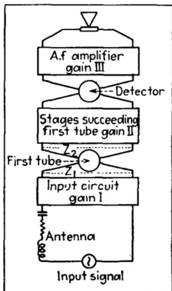
FIG. 394.—Diagrammatic representation of typical radio receiver.
