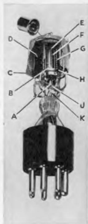
FIG. 87.—Duplex-diode pentode.
