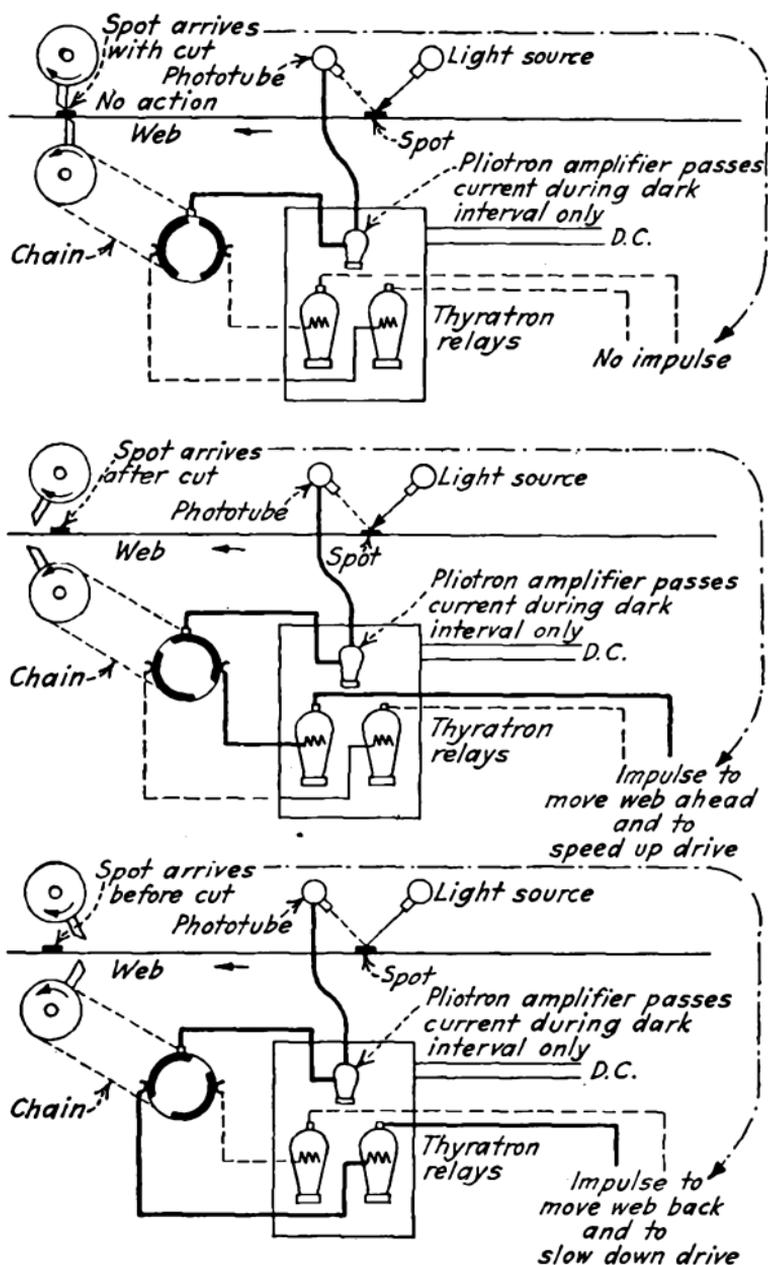
FIG. 463b.—Arrangement of apparatus for register control.
