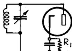
FIG. 276.—Typical two-element tube circuit for detection.
