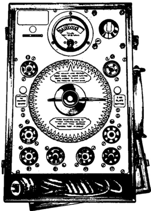
tube, one to a brass plate under the selector rotary switch, and one to a terminal of the push button that is marked "2nd plate button." This push button is located at the right-hand side of the panel, and below the tube socket marked No. 8. It is
