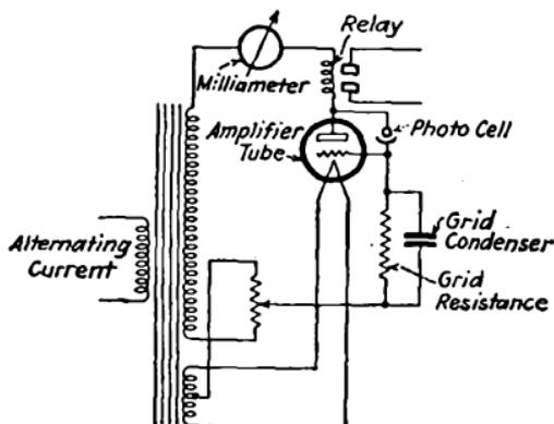
FIG. 383.—Alternating-current circuit of photoelectric tube and amplifier.
