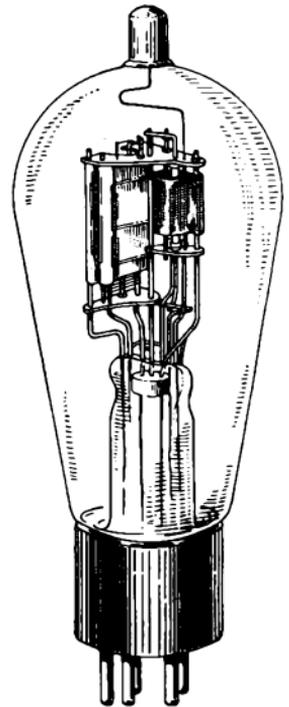
FIG. 79.—Triple-twin tube.
