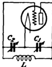
FIG. 402.—Colpitts oscillating circuit.
