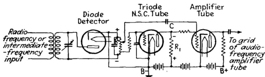
FIG. 353.—Simple circuit for automatic noise suppression.
