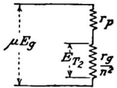
FIG. 348.—Equivalent of plate circuit of tube  $A$  in Fig. 347.
