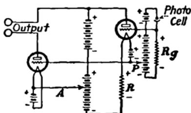
FIG. 388.—Resistance-coupled amplifier including photoelectric tube.
