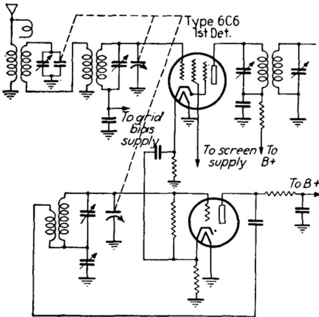
FIG. 407.—Typical all-wave superheterodyne oscillator circuit.
