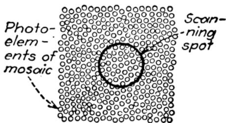
FIG. 432.—Scanning spot on photoelectric elements.
