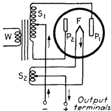
FIG. 289.—Rectifier circuit for full-wave rectification.
