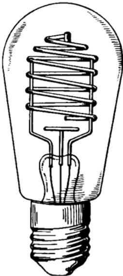
FIG. 156.—Glow lamp with spiral cathode.
