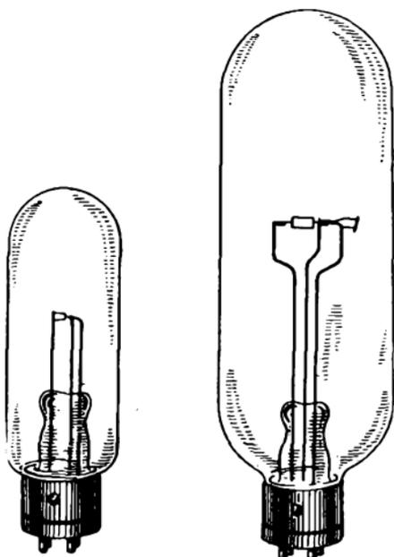
FIG. 476.—Typical arc-oscillator tubes.
