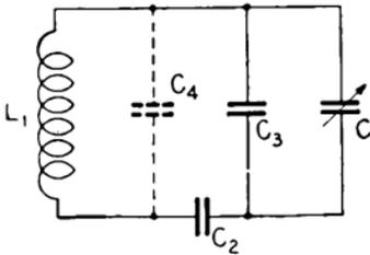
FIG. 412.—Typical oscillator circuit in super-heterodyne receiver.
