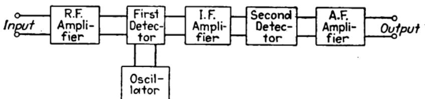
FIG. 368.—Typical superheterodyne receiving set
