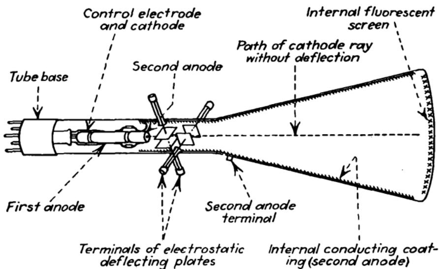
FIG. 183.—Typical cathode-ray tube.
