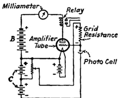
FIG. 381.—Typical direct-current reverse circuit.
