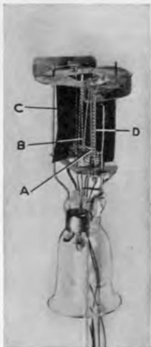
FIG. 66.—Typical dual-grid power amplifier.
