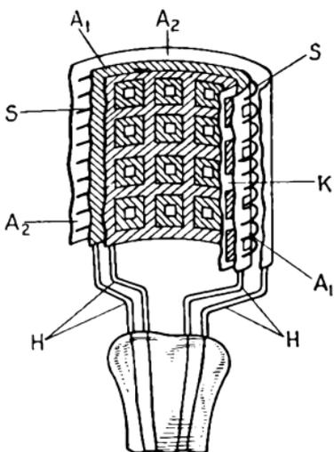
FIG. 166.—Cold-electrode tube with cylindrical electrodes.
