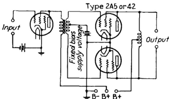
FIG. 247.—Fixed grid-bias arrangement using battery-supply current.
