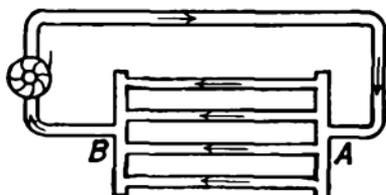
FIG. 19.—Water pipes connected in parallel.
