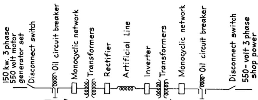
FIG. 471.—Direct-current constant-current transmission system.
