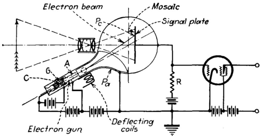
FIG. 428.—Iconoscope circuit.
