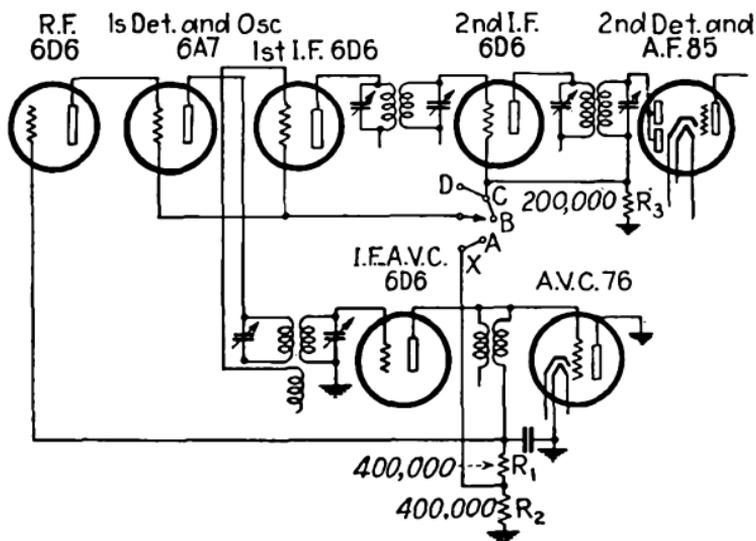
FIG. 356.—Circuit for double-automatic-volume control.
