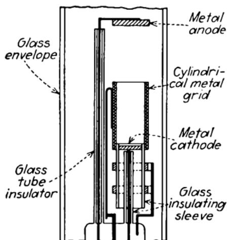
FIG. 169.—Reich and Hesselberth's cold-electrode glow-discharge tube.
