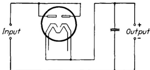
FIG. 304.—Half-wave rectifier using 25Z5 tube.
