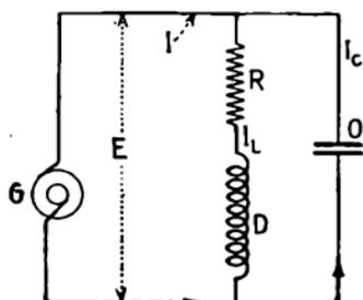
FIG. 36.—Parallel resonance of inductance and condenser.
