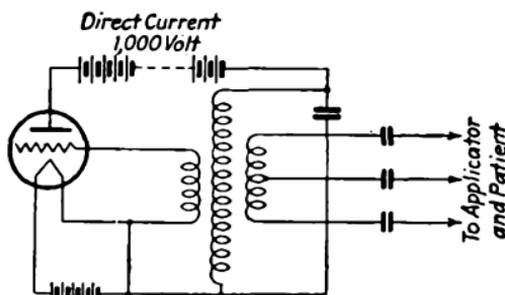
FIG. 479.—Circuit for radio surgical needle.
