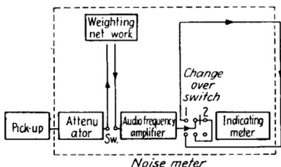
FIG. 482.—Acoustic noise meter.
