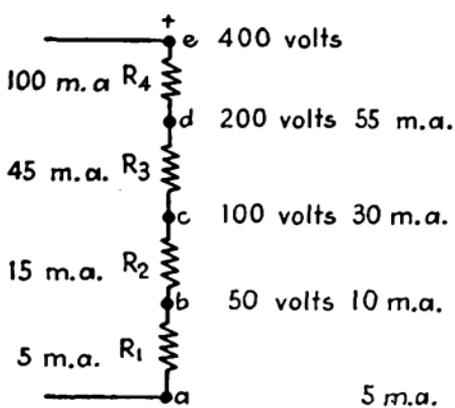
FIG. 312.—Conventional voltage divider.
