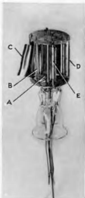
FIG. 90.—Twin triode (complete class B amplifier).
