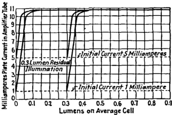
FIG. 380.—Response curve for forward circuit.
