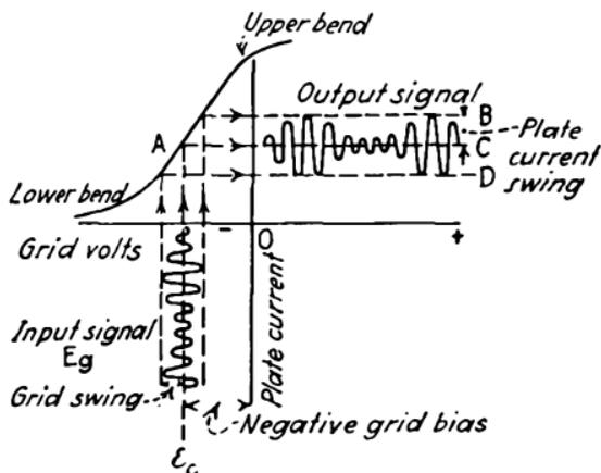
FIG. 325.—Static characteristic curve of simple amplifier.
