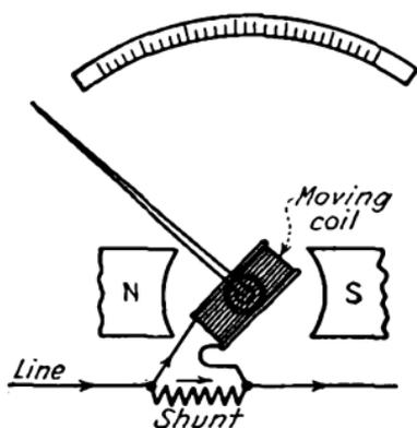
FIG. 194.—Direct-current ammeter with shunt connection.
