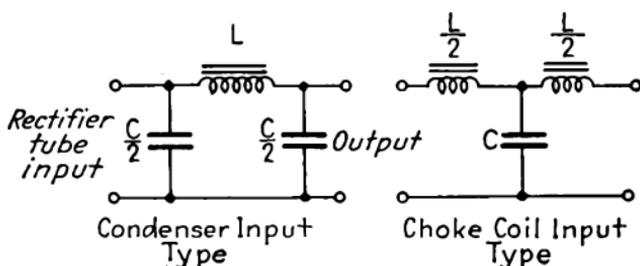
FIG. 294.—Two types of filter sections.
