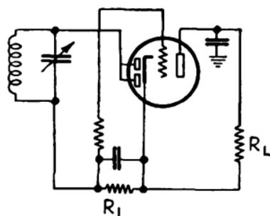
FIG. 278.—Typical detection circuit for duplex-diode-triode tubes.
