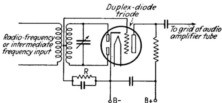
FIG. 260.—Full-wave rectification with duplex-diode triode.
