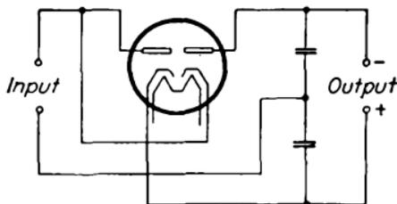
FIG. 305.—Voltage-doubling rectifier using 25Z5 tube.
