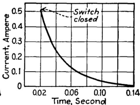
FIG. 29.—Curve of increase of current in inductive circuit when switch is closed.
