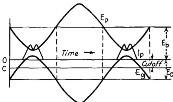
FIG. 331.—Average characteristics of ideal class *C* amplifier.
