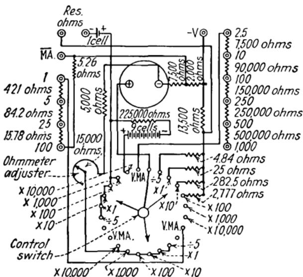
FIG. 201.—Wiring diagram of Weston ohmmeter.
