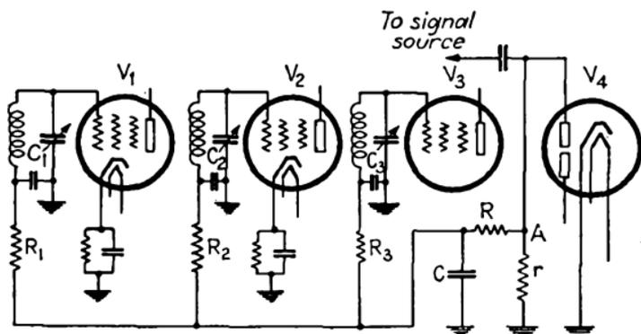
FIG. 355.—Automatic-volume-control circuit with filters.
