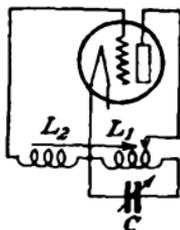
FIG. 401.—Tuned-plate oscillating circuit.
