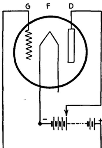
FIG. 185.—Dynatron connection for a three-element tube.
