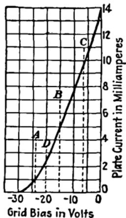
FIG. 379.—Characteristics of typical amplifier tube.
