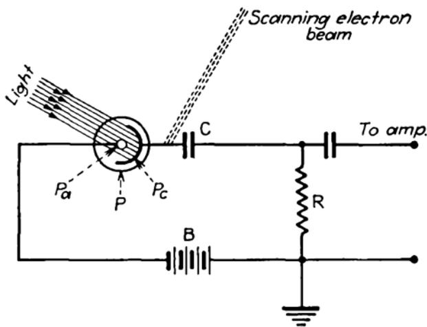
FIG. 429.—Circuit of photoelectric elements in iconoscope.
