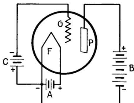
FIG. 44.—Conventional representation of three-element tube.
