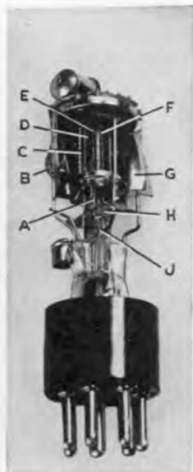
FIG. 99.—Triode-pentode tube.
