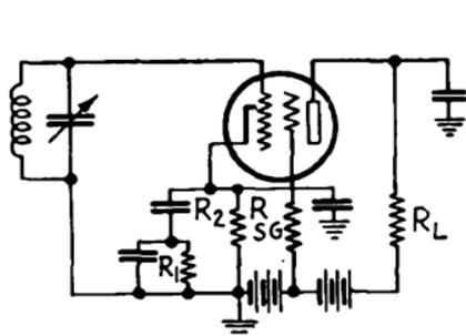
FIG. 277.—Typical detection circuit for four-element tubes.
