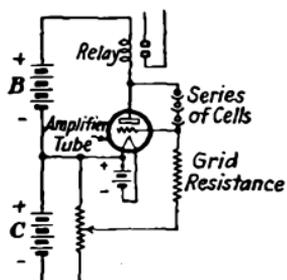
FIG. 387.—Photoelectric tubes in series.
