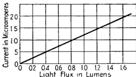
FIG. 174.—High-vacuum photoelectric tube (type SR-50).
