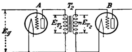
FIG. 347.—Circuit of transformer-coupled amplifier unit.
