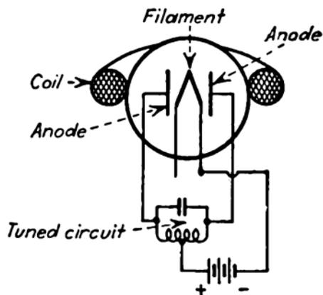
FIG. 189.—Magnetron for generation of high-frequency power.
