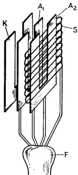
FIG. 168.—Construction details of typical cold-electrode tube.
