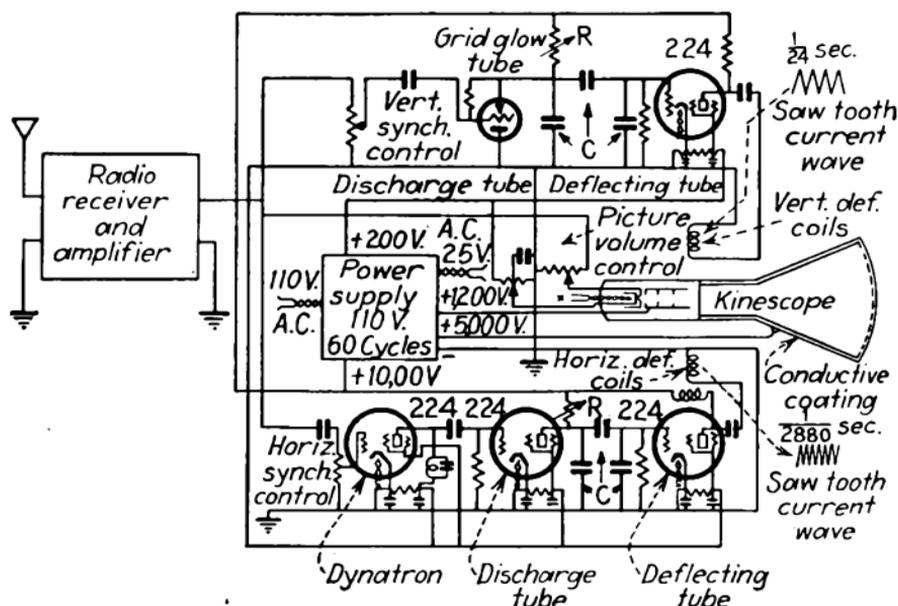
FIG. 444.—Generator for "saw-tooth" deflection current.
