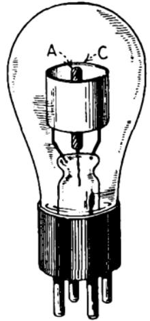
FIG. 162.—Cold-electrode gas-filled, voltage-limiting tube.
