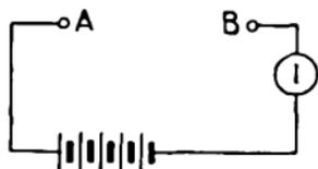
FIG. 211.—Simple circuit for resistance measurements.
