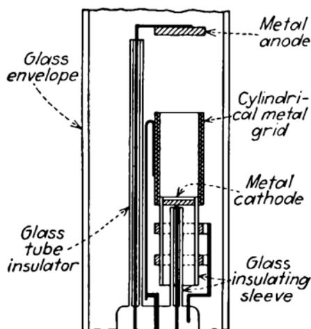
FIG. 169.—Reich and Hesselberth's cold-electrode glow-discharge tube.
