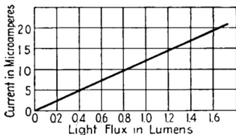
FIG. 174.—High-vacuum photoelectric tube (type SR-50).
