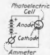
FIG. 173.—Simple photoelectric circuit.
