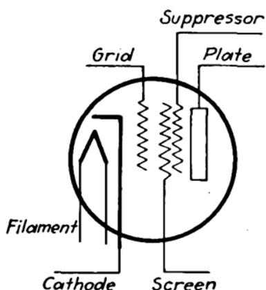
FIG. 63.—Conventional representation of pentode.
