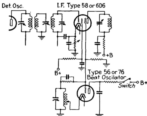
FIG. 413.—Beat-frequency oscillator circuit.
