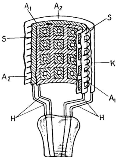
FIG. 166.—Cold-electrode tube with cylindrical electrodes.
