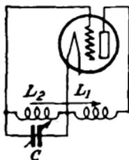
FIG. 400.—Tuned-grid oscillating circuit.
