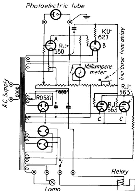
FIG. 451.—Photoelectric controller with time delay.
