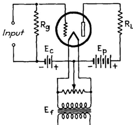
FIG. 372.—Simple amplifier circuit.
