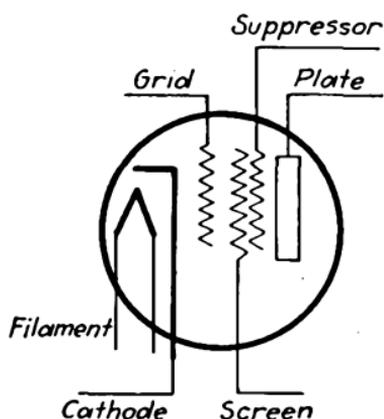
FIG. 63.—Conventional representation of pentode.
