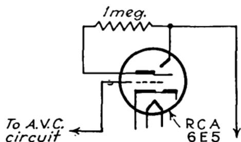
FIG. 367c.—Circuit for tuning indicator.
