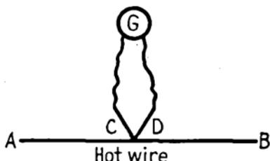
FIG. 98.—Thermocouple ammeter.
