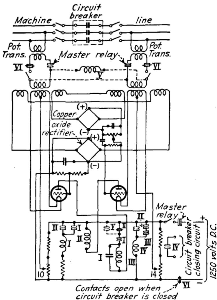
FIG. 456.—Circuit diagram of synchronizing relay.
