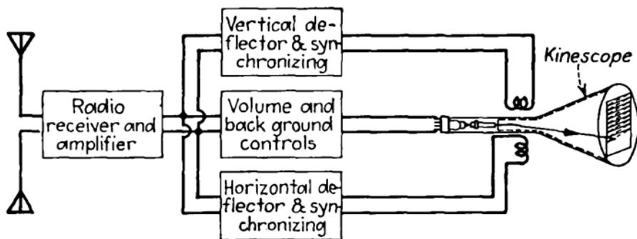
FIG. 439.—Iconoscope receiving equipment.
