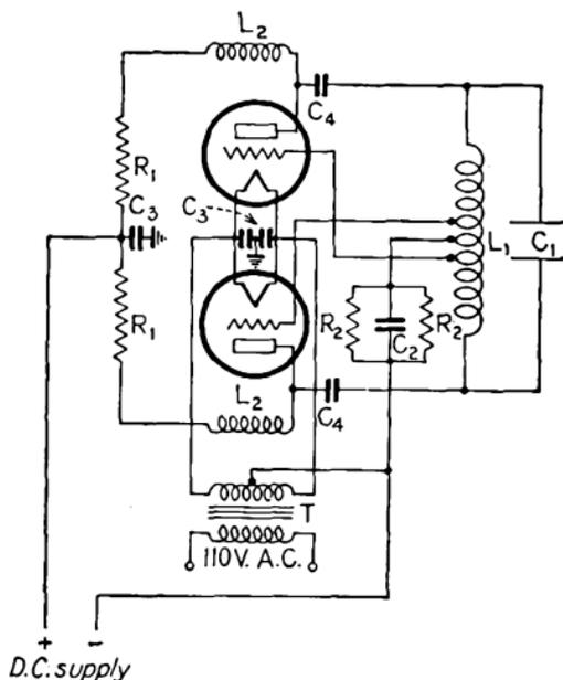
FIG. 415.—Oscillating push-pull circuit for three-electrode tubes.
