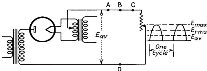
FIG. 292.—Typical rectified power-supply system.
