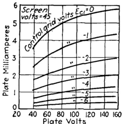
FIG. 118.—Relation of plate current to plate voltage for short-wave tetrode tube.
