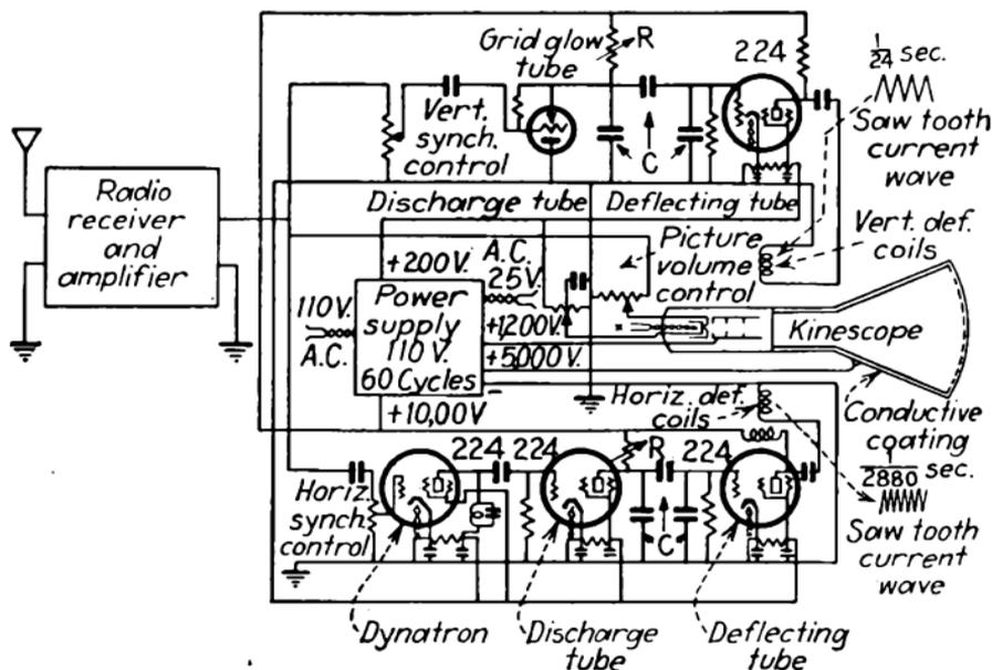
FIG. 444.—Generator for "saw-tooth" deflection current.
