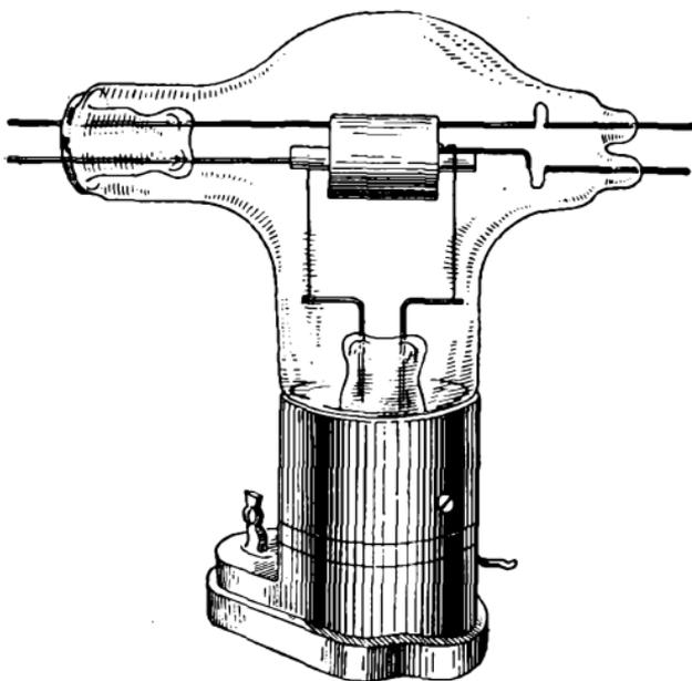
FIG. 423.—Typical positive-grid oscillator tube.
