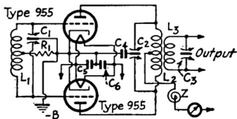
$L_1 C_1, L_2 C_2, L_3 C_3 =$  Depend on frequency range desired
