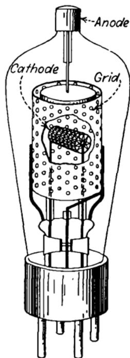
FIG. 134.—Gas-glow grid-controlled tube.
