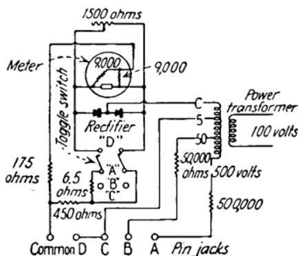
FIG. 206.—Circuit of Hickok capacity meter.
