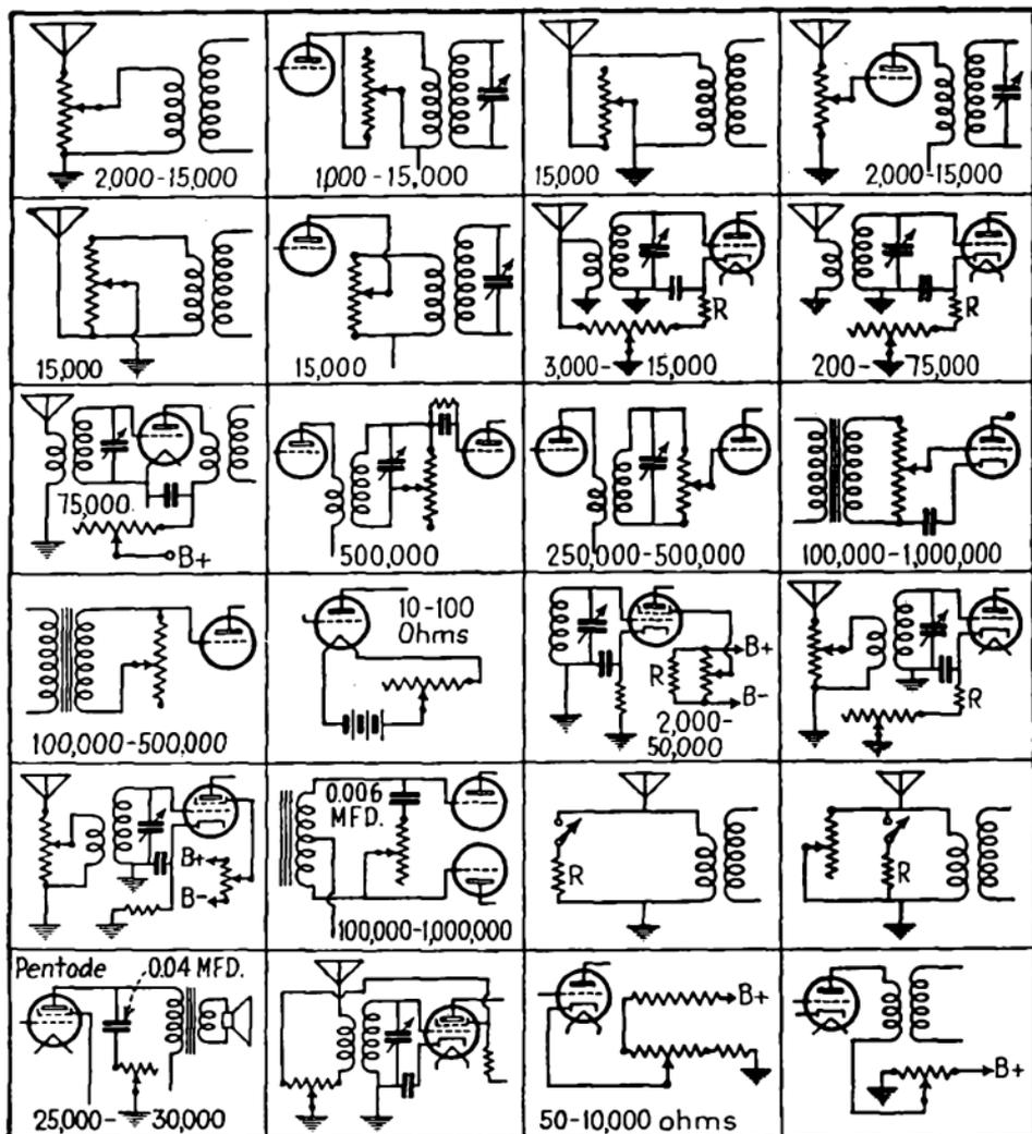
FIG. 349.—Typical volume-control arrangements.
