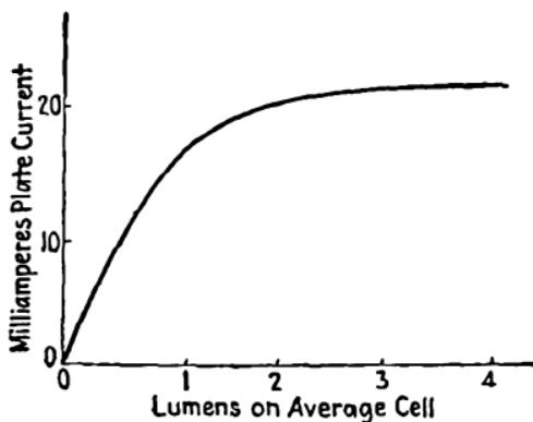
FIG. 384.—Response curve of circuit in Fig. 383.
