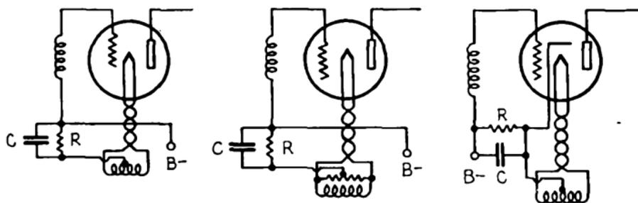
FIG. 244.—Self-biasing method of obtaining grid-bias voltage.
