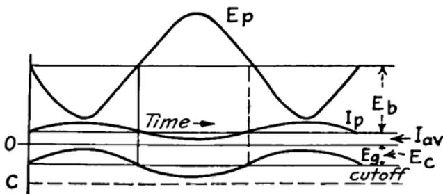
FIG. 329.—Average characteristics of ideal class *A* amplifier.
