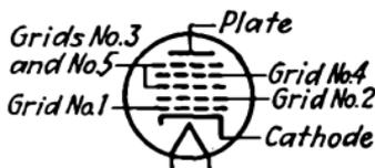
FIG. 94.—Diagram of electrodes in pentagrid converter.
