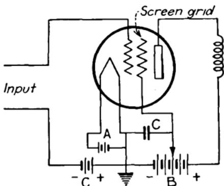
FIG. 54.—Connection of electrodes of screen-grid tube.
