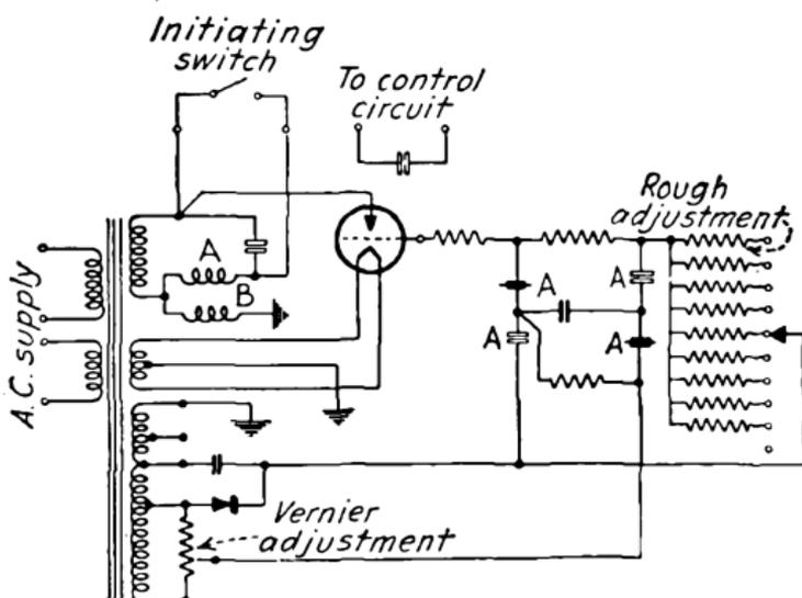
FIG. 457.—Circuit diagram of electronic timer.
