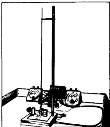
FIG. 121.—Transmitter for 100-centimeter wave lengths.
