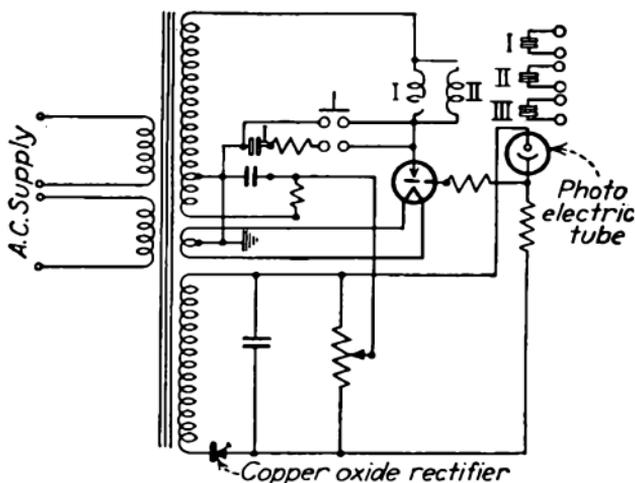
FIG. 454.—Circuit diagram for heater control.
