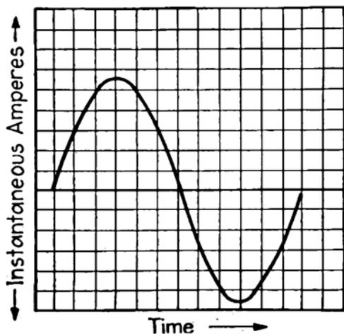
FIG. 22.—Typical sine wave of alternating current.
