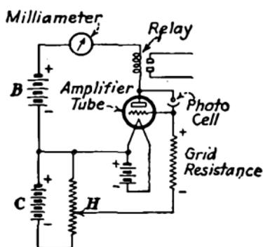
FIG. 378.—Typical direct-current forward circuit.
