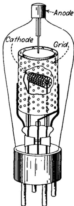
FIG. 134.—Gas-glow grid-controlled tube.
