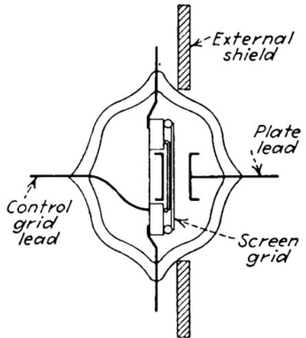
FIG. 114.—Bulb and shield for midget tetrode tube.
