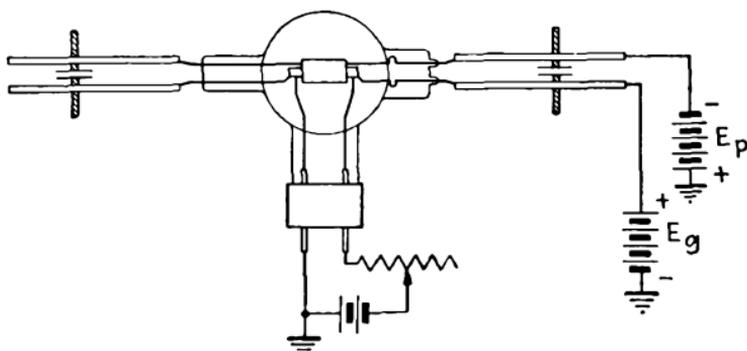
FIG. 424.—Typical positive-grid oscillator circuit.
