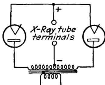
FIG. 322.—Full-wave rectification circuit.
