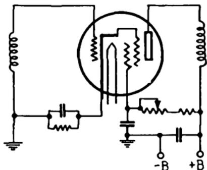
FIG. 252.—Arrangement for obtaining screen-grid voltage.
