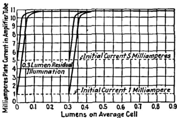
FIG. 380.—Response curve for forward circuit.
