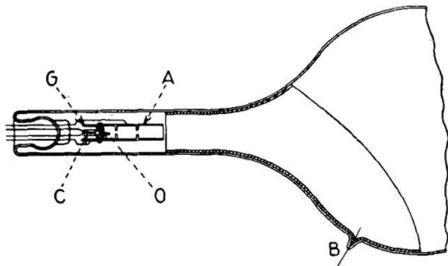
FIG. 434.—Electron gun of iconoscope.
