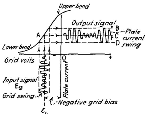
FIG. 325.—Static characteristic curve of simple amplifier.
