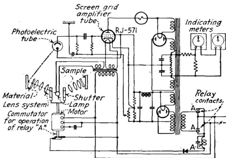
FIG. 455.—Circuit diagram of concentration indicator.
