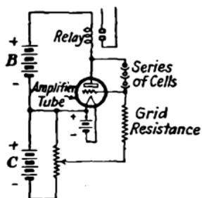
FIG. 387.—Photoelectric tubes in series.
