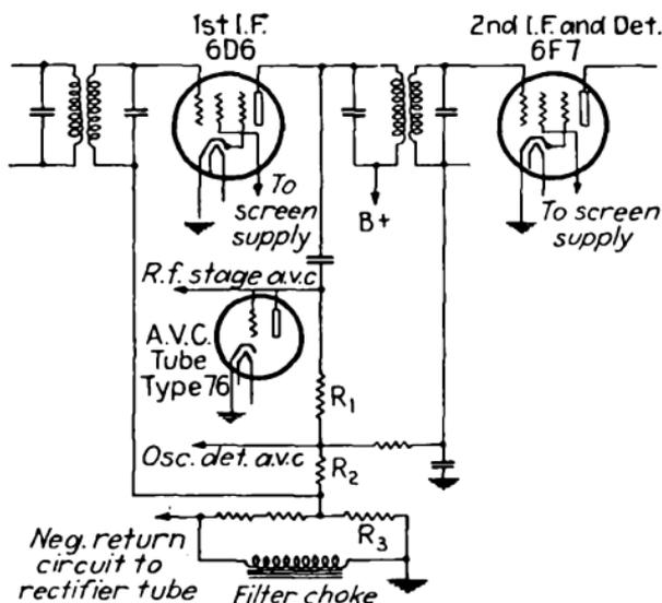
FIG. 358.—Retroactive circuit for automatic volume control.
