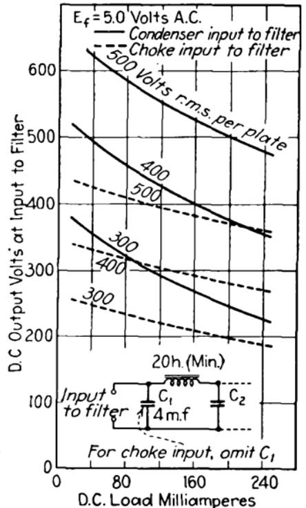
FIG. 302.—Characteristic curves of typical heavy-duty rectifier tube.
