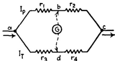
FIG. 204.—Typical Wheatstone-bridge circuit.
