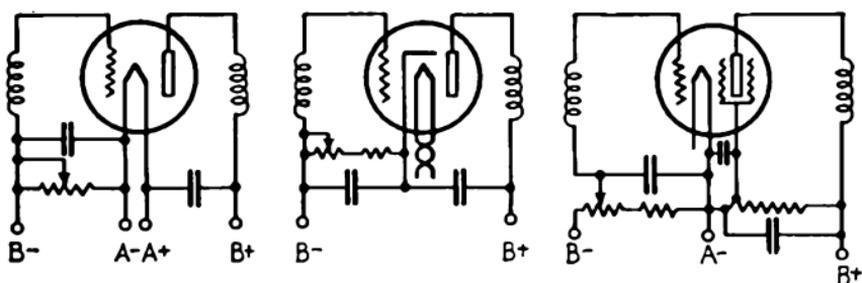
FIG. 251.—Grid-bias voltage variation for volume control.
