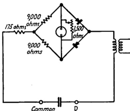
FIG. 207.—Simplified circuit of typical capacity meter.
