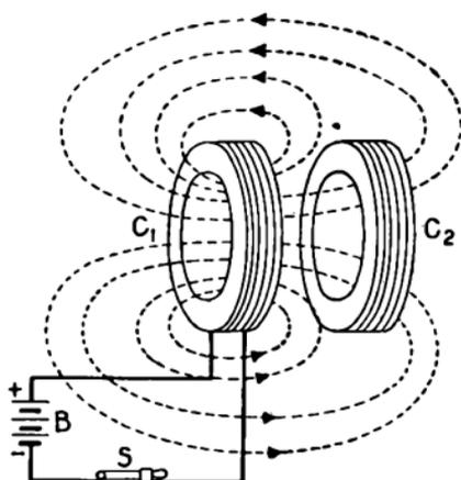
FIG. 31.—Mutual induction between two coupled coils.
