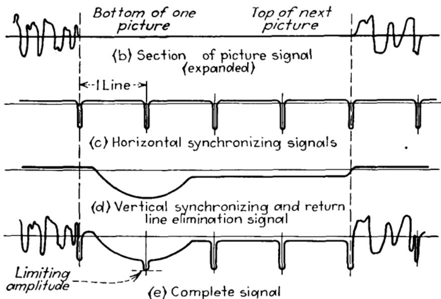
FIG. 445.—Diagram of synchronizing signals in iconoscope.
