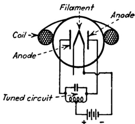
FIG. 189.—Magnetron for generation of high-frequency power.
