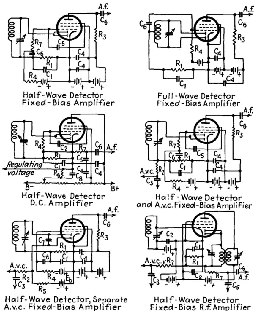
FIG. 89.—Typical circuit diagrams of duplex-diode pentode.
