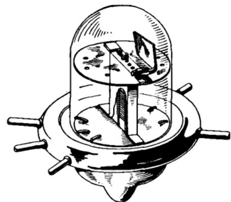
FIG. 123.—Midget triode tube (type 955).
