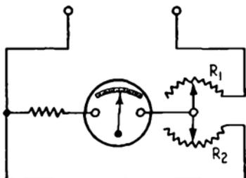
FIG. 203.—Wiring of Weston output meter.
