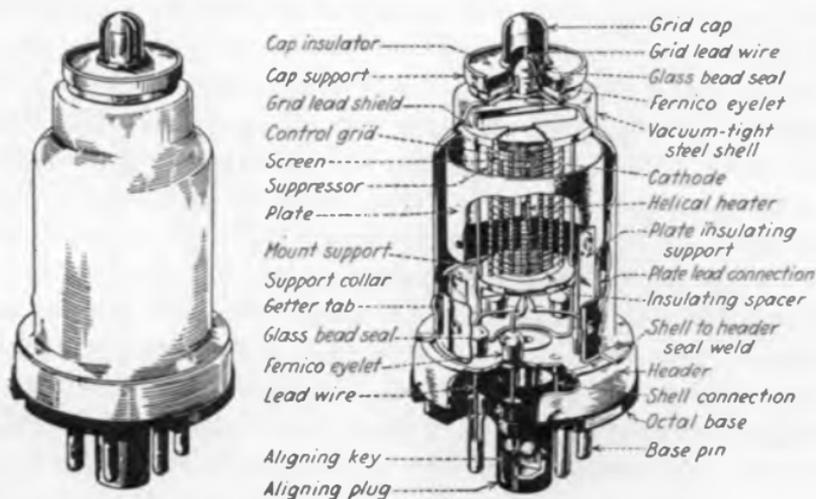
FIG. 105.—Triple-grid super-control device.
