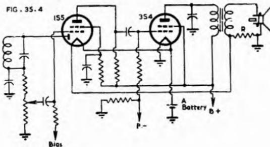
Fig. 35.4 Simple current feedback.
