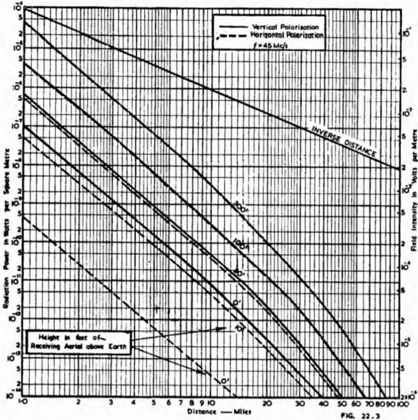
Fig. 22.3. Effect of raising the receiving aerial above the earth (1 KW at 45 Mc/s radiated over earth with conductivity  $\sigma = 10^{-13}$  e.m.u. and transmitting aerial 30 feet above the earth). The same curves also apply when the transmitting and receiving aeriels are transposed.
