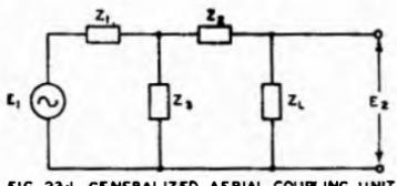
FIG. 23.1 GENERALIZED AERIAL COUPLING UNIT.
