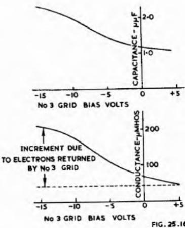
Fig. 25.15. Signal-grid (grid No. 1) current in a typical mixer with a 20-megacycle oscillator voltage applied to grid No. 3.  $E_{c_3} = -10$  volts,  $E_{c_2}$  and  $4 = 100$  volts,  $E_b = 250$  volts.
