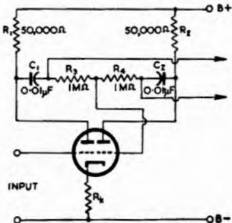
Fig. 12.35. Modified "see-saw" self-balancing phase inverter (Ref. C10).
