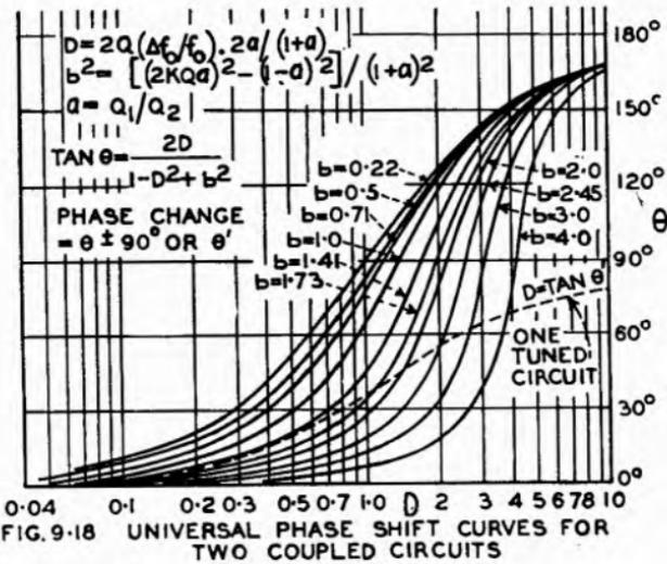
FIG. 9.18 UNIVERSAL PHASE SHIFT CURVES FOR TWO COUPLED CIRCUITS
