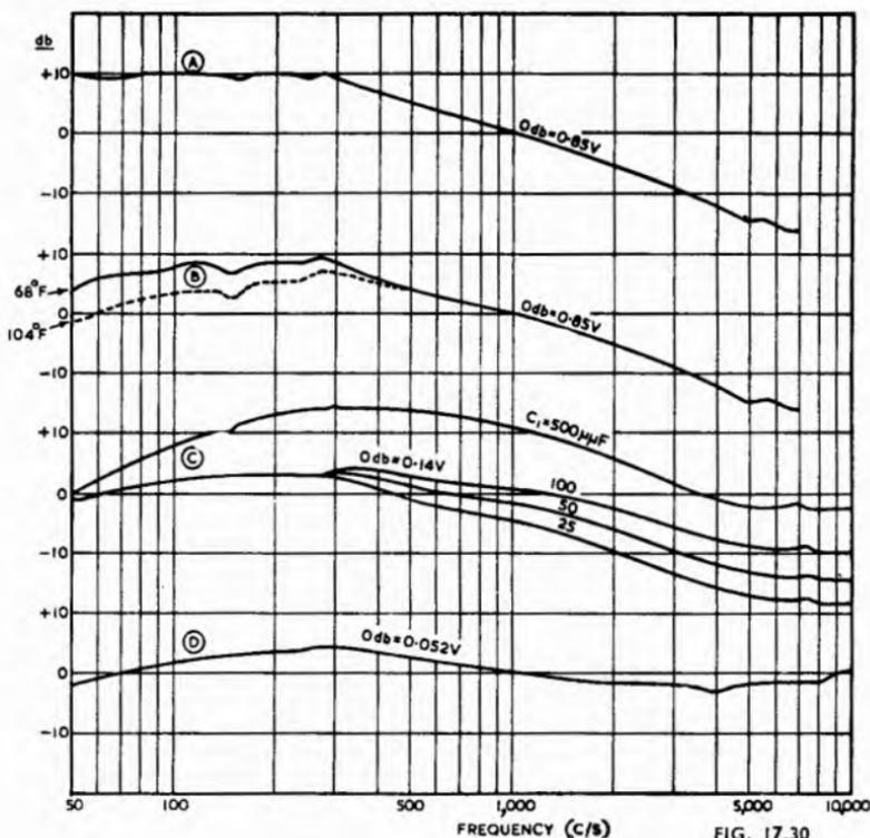
Fig. 17.30. Response curves of typical crystal pickup. (A) load resistance 2 megohms, temperature  $68^\circ F$ ; (B) load resistance 0.5 megohm, temperature  $68^\circ$  and  $104^\circ F$ ; (C) with simple equalizer circuit as Fig. 17.29 having  $R_2 = 0.5$  megohm,  $R_1 = 5$  megohms; (D) with  $R_2 = 0.125$  megohm,  $R_1 = 5$  megohms,  $C_1 = 100 \mu\mu F$ . Test record Audiotone for (A), (B) and (C); Columbia M-10 003 for (D). Curves based on data for Astatic FP-18.
