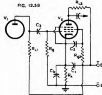
Fig. 12.57. Hum neutralization in a r.c.c. pentode.
