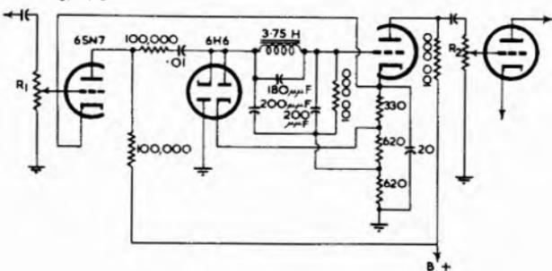
Fig. 16.16. Simple form of speech clipper suitable for an amateur transmitter. The 3.75 H choke must have low d.c. resistance and good a-f characteristics (Ref. 28).
