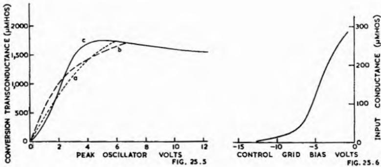
Fig. 25.5. Conversion transconductance of a typical variable- $\mu$ , radio-frequency pentode. Oscillator and signal voltages both applied to grid No. 1. *a*, fixed-bias operation; *b*, cathode resistor used to obtain bias; *c*, bias obtained by means of a high-resistance grid leak. Fig. 25.6. Input conductance of a typical variable- $\mu$ , radio-frequency pentode, at 60 megacycles.
