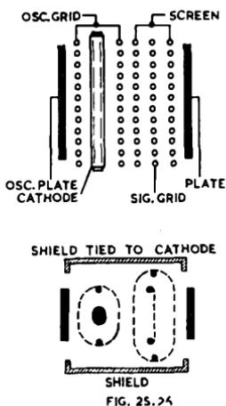
Fig. 25.26. Electrode arrangement of the triode-hexode type 6K8(G).
