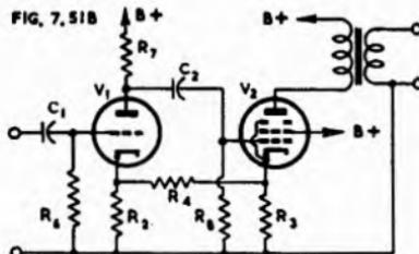
This circuit (Fig. 7.51B) may also be used with any desired degree of feedback. The effective plate resistance of  $V_2$  may be increased or decreased by the positive feedback as shown by the following analysis and Fig. 7.51C. Here  $R_1$  replaces  $R$ , and  $R_8$  in parallel, no input signal is applied but a signal generator  $E$  is inserted in the plate circuit. It is assumed that  $R_4$  is very much greater than  $R_3$ . We thus obtain
