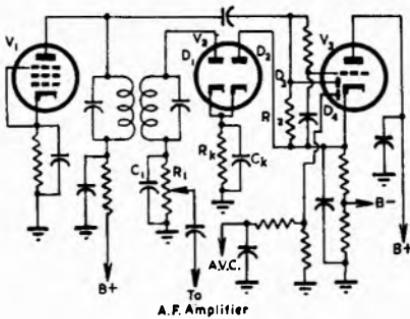
FIG. 27.43 Biased Detector Muting System
