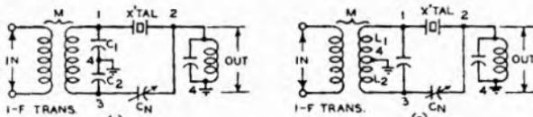
FIG. 26.12 PRACTICAL CIRCUIT ARRANGEMENTS FOR QUARTZ CRYSTAL FILTERS
