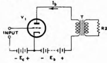
Fig. 13.1. Basic circuit of a Class A<sub>1</sub> triode with transformer-coupled load.
