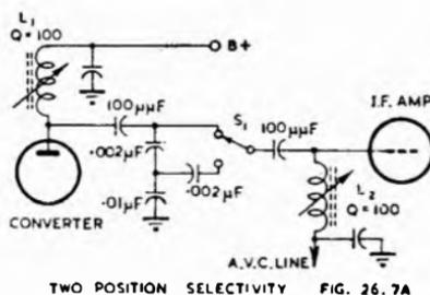
One such bottom coupling method which requires the minimum of switching for two degrees of coupling is shown in Fig. 26.7A (Ref. 42a). The two coils  $L_1$  and  $L_2$  should each be in a separate shield can. With switch  $S_1$  in the position shown, the selectivity is broad; in the lower position the selectivity is normal. Capacitances as shown are only illustrative. The same principle can be used for three values of coupling, using seven capacitors.
