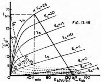
Fig. 13.48. Plate and grid characteristics of a typical small battery-operated Class B triode (1J6-G).
