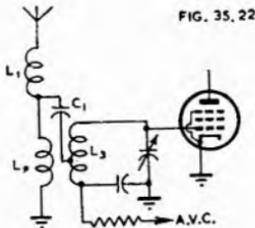
Fig. 35.22. Car-radio aerial input circuit.
