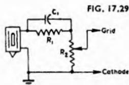
Fig. 17.29. Simple equalizer circuit for a crystal pickup.
