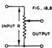
Fig. 18.8. Continuously variable volume control (potentiometer).
