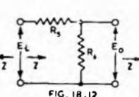
Fig. 18.12. The L type single section attenuator.
