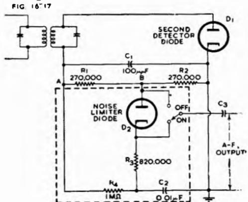
Fig. 16.17. Simple series limiter (Ref. 30).
