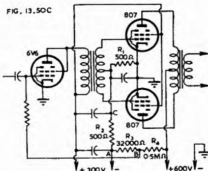
Fig. 13.50C. Class AB<sub>2</sub> amplifier with stabilized bias and screen voltages (Ref. E26).
