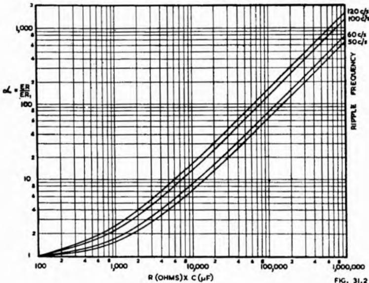
Fig. 31.2. Curve for determining the value of  $\alpha = E_R/E_{R1}$  of a resistance-capacitance type single section filter for frequencies of 50, 60, 100 and 120 c/s. This curve is based on the formula,  $E_R/E_{R1} = \omega CR + 1$ .
