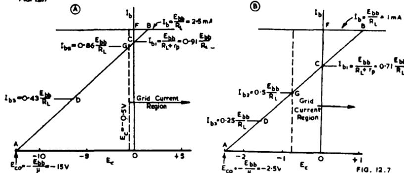
Fig. 12.7. "Ideal" linear dynamic characteristics (A) for general purpose triode with  $\mu = 20$ ,  $r_s = 10000$  ohms,  $R_L = 0.1$  megohm and  $E_{bb} = 250$  volts; (B) for high- $\mu$  triode with  $\mu = 100$ ,  $r_s = 0.1$  megohm,  $R_L = 0.25$  megohm and  $E_{bb} = 250$  volts.
