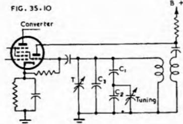
Fig. 35.10. Bandsread circuit to give linear scale.
