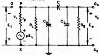
Fig. 12.8. Exact equivalent circuit of r.c.c. triode.
