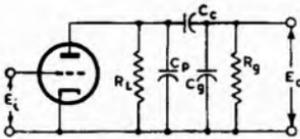
Fig. 7.74. Resistance-capacitance coupled stage.
