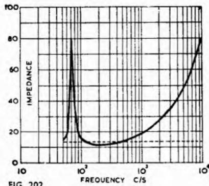
Fig. 20.2. Impedance versus frequency characteristic of a typical popular loudspeaker.
