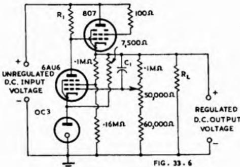
Fig. 33.6. Simplest form of series valve voltage regulator.
