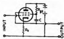
FIG. 7.16. Pentode cathode follower with screen bypassed to cathode.
