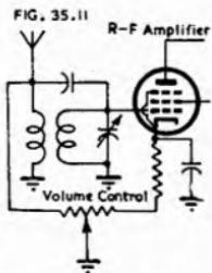
Fig. 35.11. Volume-control circuit used with t-r-f receivers.
