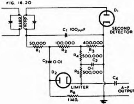
Fig. 16.20. Low-loss series limiter. (Ref. 30).
