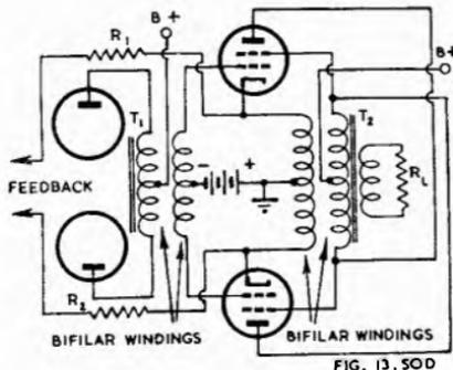
Fig. 13.50D. Basic principles of McIntosh Amplifier (Ref. E28).
