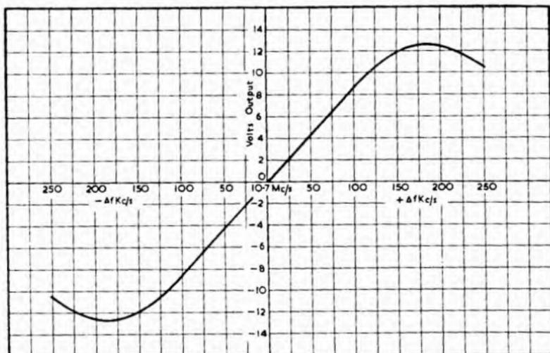
FIG. 27.18(B) Discriminator Characteristic Obtained From Design Example
