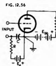
Fig. 12.56. Grid circuit decoupling with fixed bias.
