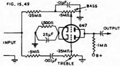
Fig. 15.49. Simple two channel amplifier (Ref. 22).
