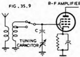
Fig. 35.9. Series-capacitor method of bandspread.
