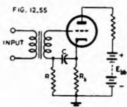
Fig. 12.55. Grid circuit decoupling with transformer input and cathode bias.
