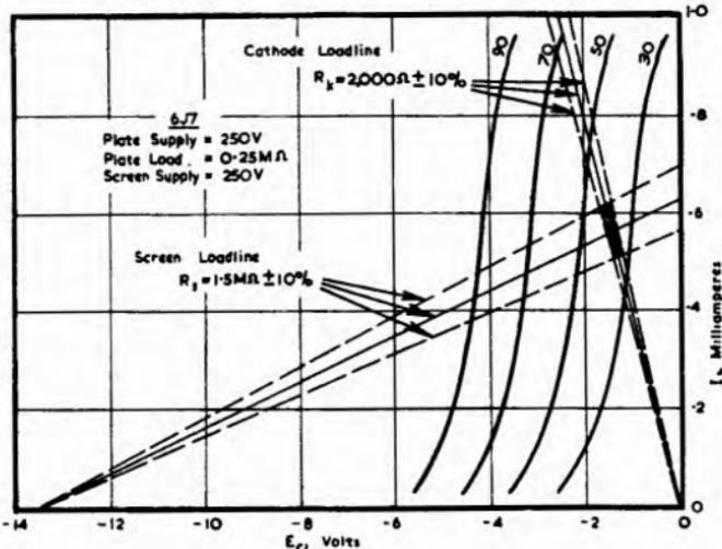
Fig. 12.22. Plate dynamic characteristics of type 6J7 with screen and cathode loadlines, showing the effect of  $\pm 10\%$  tolerances in both  $R_L$  and  $R_k$ .
