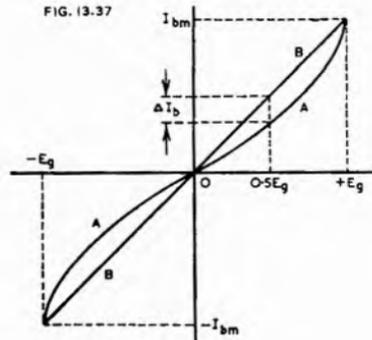
Fig. 13.36. Method of deriving the approximate power output and load resistance of a Class AB<sub>1</sub> amplifier from the characteristics of a single valve. The method may also be used with poorer accuracy for Class A<sub>1</sub>.
