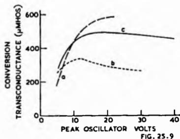
Fig. 25.9. Conversion transconductance of a typical mixer designed for inner-grid injection of oscillator. Signal-grid bias =  $-3$  volts. *a*, fixed-bias operation of oscillator grid; *b*, oscillator-grid bias obtained through high-resistance grid leak; *c*, oscillator-grid bias obtained through a 50,000-ohm grid leak.
