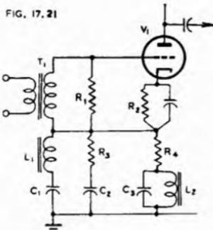
Fig. 17.21. Frequency selective negative feedback used to provide equalizing for English records. (Ref. 199).  $V_1 = 6H4$  ( $\mu = 40, r_p = 11\ 000$  ohms), load resistance = 50 000 ohms.
