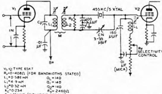
FIG. 28-16 CRYSTAL FILTER CIRCUIT DESIGNED FROM ILLUSTRATIVE EXAMPLE
