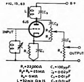
Fig. 15.63. Narrow-band rejection filter for 9 Kc/s (Ref. 74).
