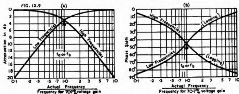
Fig. 12.9(A). Attenuation in decibels for r.c.c. triode at low and high frequencies
