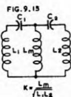
Fig. 9.15. Low impedance inductive coupling.
