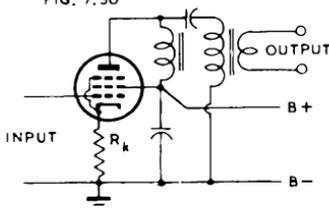
Fig. 7.50. Parallel-fed transformer-coupled output with feedback from an unbypassed cathode resistor.
