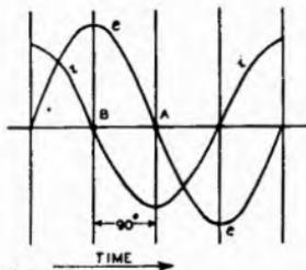
FIG. 4.15. Alternating current through an ideal condenser.
