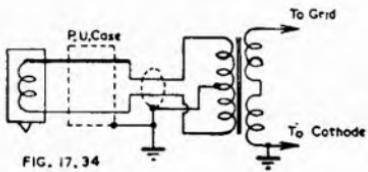
*Fig. 17.34. Low impedance pickup with balanced-to-earth input to step-up transformer.*
