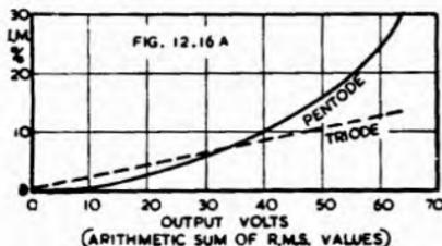
Fig. 12.16A. Intermodulation distortion for type 6SJ7 with  $E_{bb} = 250$  volts,  $R_L = 0.25 \text{ M}\Omega$ ,  $R_o = 1.0 \text{ M}\Omega$ , in both triode and pentode operation.
