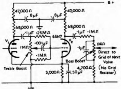
Fig. 15.48. Two-stage bass and treble tone control (Ref. 41).
