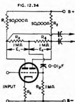
Fig. 12.34. "See-saw" self-balancing phase inverter (Ref. C9).
