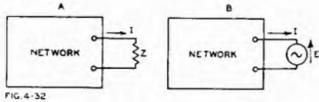
Fig. 4.32. (A) An impedance  $Z$  in a network with current  $I$  and voltage drop  $ZI$  (B) Equivalent circuit having identical results so far as current and voltage drop are concerned, with a generator developing a voltage  $E = ZI$ . This illustrates the Compensation Theorem.
