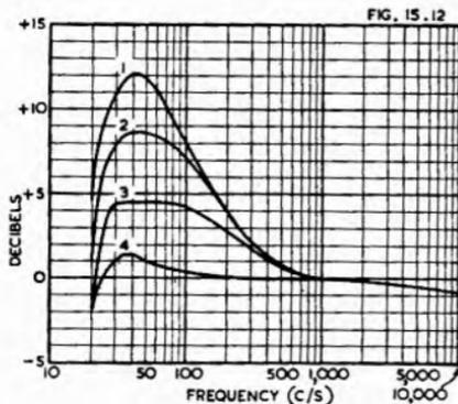
Fig. 15.12. Frequency characteristics of amplifier in Fig. 15.11. Condition (1) tone control max. resistance (2) three quarters max. (3) half max. (4) one quarter max. resistance. The curves have been superimposed to coincide at 1000 c/s.
