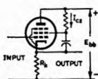
Fig. 7.89. Pentode cathode follower, resistance-loaded, screen by-passed to cathode.
