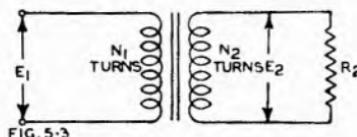
Fig. 5.3. Ideal two-winding transformer with loaded secondary.
