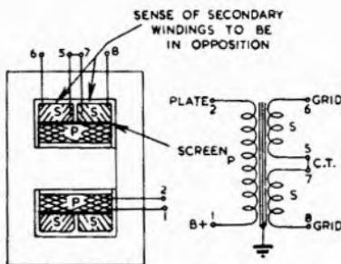
Fig. 5.12. Transformer wound with balanced secondaries.
