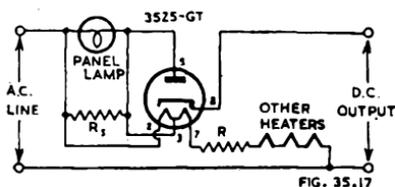
Fig. 35.17. Circuit using 35Z5-GT and dial lamp. The drop across  $R$  and all heaters (with panel lamp) should equal 117 volts at 0.15 ampere.  $R_S$  = shunting resistor required when d.c. output current exceeds 60 mA.
