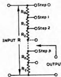
Fig. 18.9. Step-type volume control.
