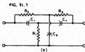
Fig. 31.3. Resistance-capacitance parallel T network and its equivalent  $\Pi$  network.
