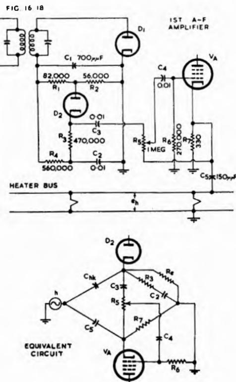
Fig. 16.18. Hum-reduction version of simple series limiter with equivalent circuit to show bridge configuration (Ref. 30).
