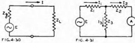
Fig. 4.31. A generator  $E$  supplying voltage to a network, with an ammeter  $A$  to read the current  $I_2$ . The reciprocity theorem states that, when  $A$  and  $E$  are reversed, the transfer impedance  $E/I_2$  will be unchanged.
