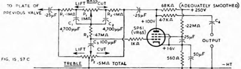
Fig. 15.57C. Tone control circuit. Tolerances  $R_1, R_2, C_1, C_2, R_3, C_3 \pm 5\%$ .  $P_1$  and  $P_2$  are linear potentiometers,  $P_2$  having a fixed tapping at 50% rotation. The source impedance should not be more than 10,000 ohms.  $C_4$  should normally be  $0.05\mu F$  if following stage has  $0.25 M\Omega$  grid leak (Ref. 91). Type 6AU6 could be used as substitute for the type shown, with suitable values of cathode and screen resistors, to give an output of about 2 V r.m.s.
