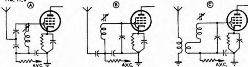
Fig. 11.5. Aerial coupling circuits used with permeability tuning.
