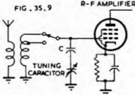
Fig. 35.9. Series-capacitor method of bandspreading.
