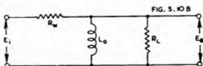
Fig. 5.10B. Low frequency equivalent circuit.
