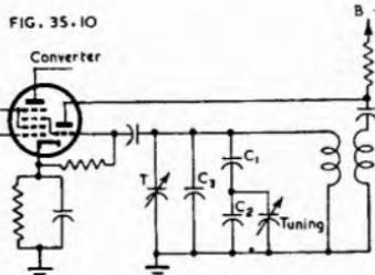
Fig. 35.10. Bandspread circuit to give linear scale.
