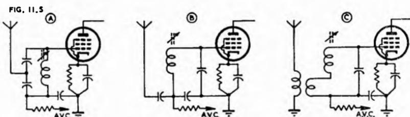
Fig. 11.5. Aerial coupling circuits used with permeability tuning.
