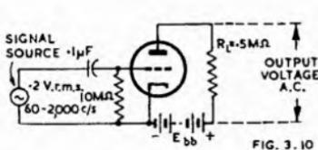
Fig. 3.10. Method of testing for a.c. amplification (after RMA).
