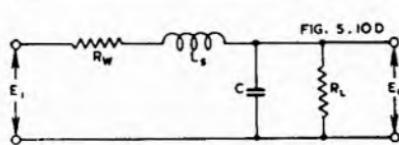
Fig. 5.10D. High frequency equivalent circuit.
