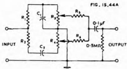
Fig. 15.44A. Simple duo-control circuit giving individual control of bass and treble. Typical values are:  $R_1 = 0.25\text{ M}\Omega$ ;  $R_2 = R_3 = 0.5\text{ M}\Omega$ ;  $R_4 = 0.25\text{ M}\Omega$ ;  $R_5 = R_6 = 0.5\text{ M}\Omega$ ;  $C_1 = 0.01\ \mu\text{F}$ ;  $C_2 = 0.001\ \mu\text{F}$  (Ref. 22).
