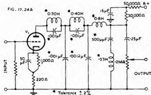
Fig. 17.24A. Amplifier stage incorporating filter with 7000 c/s pass-band and very rapid attenuation at higher frequencies (Ref. 15).  $V_1 = \text{MH4}$ ,  $\mu = 40$ ,  $r_p = 15000 \text{ ohms}$ .
