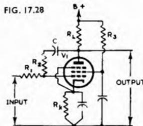
A modification of the circuit of Fig. 17.28 is described in Ref. 280 which gives both bass boosting (with a "very low frequency roll-off") and high frequency de-emphasis. Values of components are:  $R_1 = 0.33\text{ megohm}$ ,  $R_2 = 1.0\text{ megohm}$ ,  $R_L = 0.22\text{ megohm}$ ,  $C = 600\text{ }\mu\text{F}$  approx. (adjustable),  $C_2 = 25\text{ }\mu\text{F}$  approx. (adjustable) shunted across  $R_2$ , and  $V_1 = 6F37$ .
