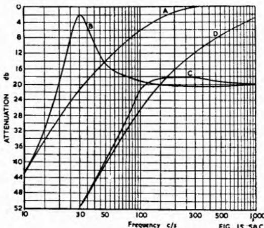
*Fig. 15.58C. Frequency characteristics of circuit of Fig. 15.58B. (A) No feedback, no tone control; (B) feedback without tone control; (C) feedback with tone control; (D) no feedback, with tone control.*
