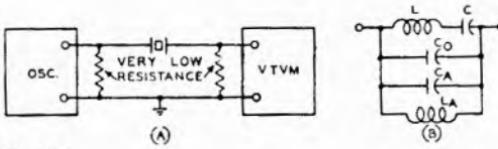
FIG. 26.15 APPROXIMATE METHODS FOR DETERMINING EQUIVALENT ELECTRICAL CONSTANTS OF QUARTZ CRYSTALS
