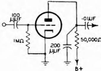
FIG. 27.12. TYPICAL GRID LEAK DETECTOR WITH R-C COUPLING.
