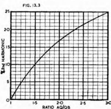
Fig. 13.3. Curve of second harmonic distortion plotted against the ratio AQ/QB for the two portions of the loadline (Fig. 13.2).
