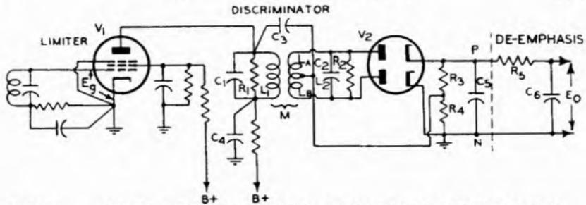
FIG. 27-17 TYPICAL PHASE DISCRIMINATOR ARRANGEMENT FOR F-M DETECTION.
