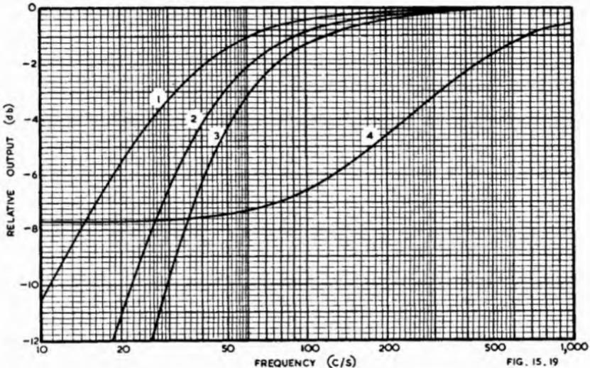
Fig. 15.19. Bass attenuation versus frequency characteristics: (1) Single grid coupling condenser ( $R = 1$  megohm,  $C = 0.005 \mu\text{F}$ ); (2) Two stages each with identical values of time constant  $RC$ ; (3) Three stages each with identical values of time constant; (4) R.c.c. pentode with by-passed cathode resistor (6)7,  $R_L = 0.25 M\Omega$ ,  $R_k = 2000 \Omega$ ,  $C_k = 0.5 \mu\text{F}$  and screen adequately by-passed.
