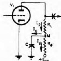
Fig. 12.53. Plate circuit decoupling.
