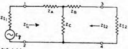
Fig. 4.44 is a single T section network terminated in its image impedances.
