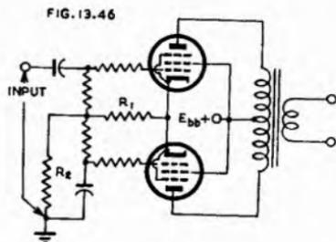
Fig. 13.46. Push-pull circuit with common cathode impedance coupling.
