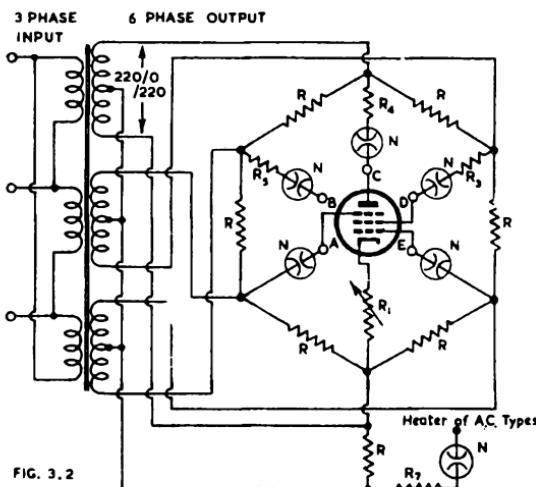
*Fig. 3.2. Hexaphase shorts and continuity tester. Suitable values are  $R = 5000$  ohms,  $R_3 = R_5 = 7500$  ohms,  $R_4 = 1500$  ohms,  $R_2 = 5000$  ohms,  $R_1 = 50\ 000$  ohms for battery valves other than power output, 33 000 ohms for normal a.c. types, or 15 000 ohms for power output valves. Lamps (N) are 110 volt  $\frac{1}{2}$  watt split-anode neon.*
