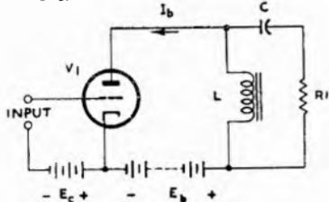
Fig. 13.17. Choke-coupled amplifier.
