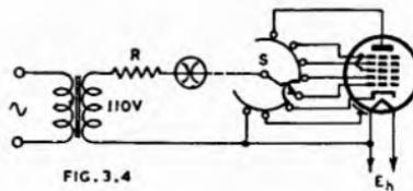
Fig. 3.4. Simpler type of shorts and continuity tester, employing a single lamp.
