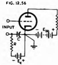
Fig. 12.56. Grid circuit decoupling with fixed bias.
