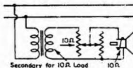
It is important to check for the phasing of the two loudspeakers ; in the vicinity of the cross-over frequency both units should be in phase (aiding one another). This may be checked by the use of a single dry cell connected in series with the secondary of the transformer ; in the case of 2 ohm voice coils there may be a 5 ohm limiting resistor connected in series with the cell.
