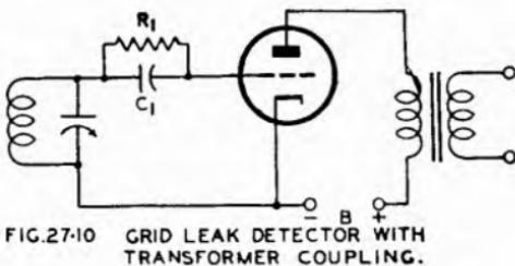
FIG. 27.10 GRID LEAK DETECTOR WITH TRANSFORMER COUPLING.
