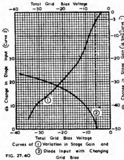
It is now necessary to relate the total bias (a.v.c. + standing bias) to the change in diode input voltage; the change is conveniently expressed in decibels. Any signal voltage applied to the diode may be taken as zero reference level (0 db), and in our case  $E_{rms} = 2$  volts will be convenient. Then the change in diode input voltage is given by,
