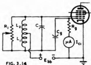
Fig. 3.14. Self-excited oscillator, using the Hartley circuit, for testing oscillator performance.
