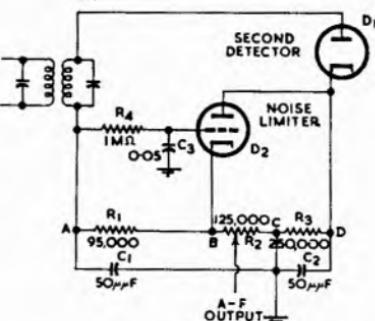
Fig. 16.24. Triode shunt-type noise limiter (Ref. 30).
