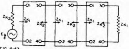
Fig. 4.43 is a combination of three networks in cascade, with iterative impedance relationships.
