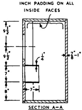
Fig. 20.13. Typical corner cabinet with vented baffle, designed for a Goodmans Axiom 12 inch loudspeaker with a bass resonant frequency of 55 c/s, which can be used with a speaker resonant at 75 c/s by removing the tunnel. Cubic capacity about 8000 cu. ins. = 4.6 cu. ft. (Ref. 182).
