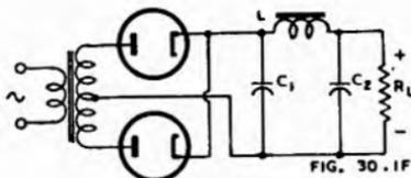
Fig. 30.1G. Basic circuit diagram of full-wave rectifier with choke input filter.
