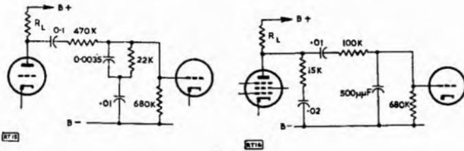
Fig. 17.15E. Equalizing circuit following a triode (RT15).
