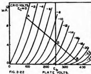
Fig. 2.21. Loadlines of resistance-loaded pentode.
