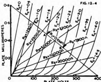
Fig. 12.4. Plate characteristics of high- $\mu$  triode (6SQ7) with  $E_{dd} = 400$  volts and  $R_L = 0.5$  megohm. Cathode bias loadlines for selected values of cathode bias resistance ( $R_k$ ) have been drawn in.
