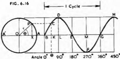
The length  $PX = r \sin \theta$ , so that its projected height CK is proportional to the sine of  $\theta$ . The curve is therefore called a "sine curve" or "sine wave." A cosine curve has exactly the same shape, except that it begins at D (since  $\cos 0^\circ = 1$ ) and the cycle ends at H.
