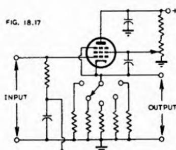
Fig. 18.17. Electronic attenuator using cathode follower (Ref. C15).
