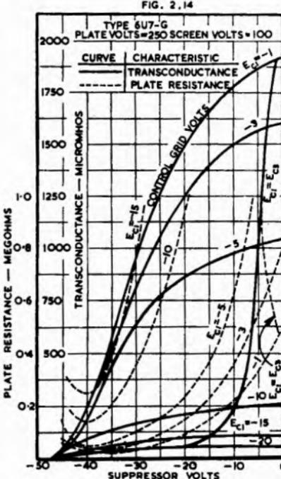
Fig. 2.14. Suppressor characteristics of a remote cut-off pentode (6U7-G) for fixed screen and plate voltages.
