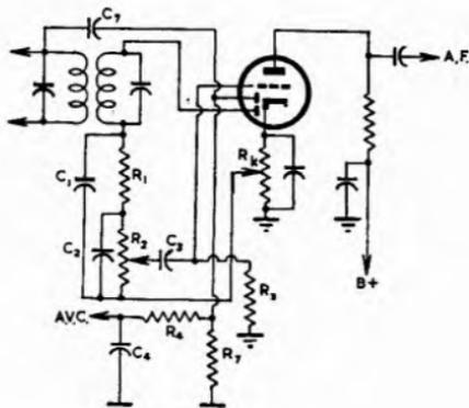
FIG. 27.42 Biased Detector Muting System
