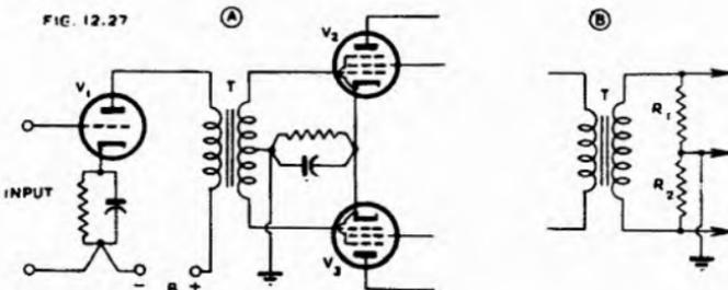
Fig. 12.27. (A) Triode valve ( $V_1$ ) followed by transformer ( $T$ ) having centre-tapped secondary and exciting the grids of the push-pull stage ( $V_2, V_3$ ). (B) Modified form with non-centre-tapped transformer, using two resistors to provide an equivalent centre-tap.
