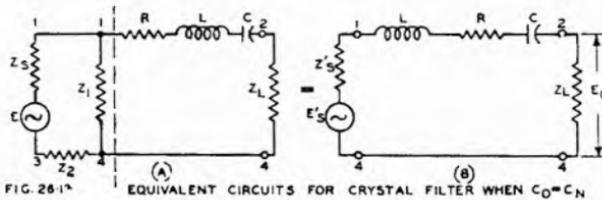
For purposes of analysis it is convenient to rearrange Fig. 26.13(A) as shown in Fig. 26.13(B), and, if we take  $Z_1 = Z_2$ , the value of  $Z'$ , will be a quarter of the total dynamic impedance of the secondary circuit of the i-f input transformer.  $E'$ , will be half the voltage developed across the two series capacitors tuning the i-f transformer secondary.
