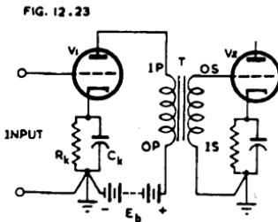
Fig. 12.23. Circuit diagram of transformer-coupled voltage amplifier
