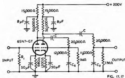
**Fig. 17.17.** Circuit diagram of two stage bass equalizing amplifier with bass boosting in each stage. Pin 4 of the 6SN7-GT should be used for the input circuit. Total boost is 20 db and max. slope 6 db/octave.  $C = 0.25 \mu F$  for good bass response or  $0.1 \mu F$  for some bass attenuation;  $C_2 = 0.1 \mu F$  for cross-over 250 c/s or  $0.05 \mu F$  for 500 c/s. Voltage gain at 1000 c/s = 22 times = 26.8 dbvg.
