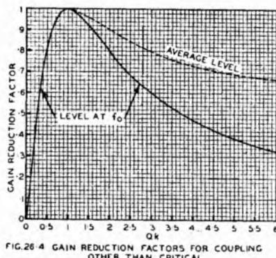
FIG. 26.4 GAIN REDUCTION FACTORS FOR COUPLING OTHER THAN CRITICAL
