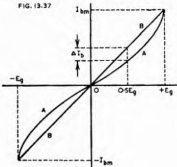
Fig. 13.36. Method of deriving the approximate power output and load resistance of a Class AB<sub>1</sub> amplifier from the characteristics of a single valve. The method may also be used with poorer accuracy for Class A<sub>1</sub>.
