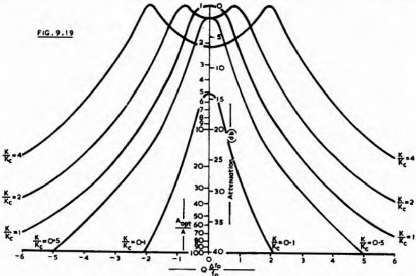
Selectivity Curves for Two Identical Coupled Circuits,
