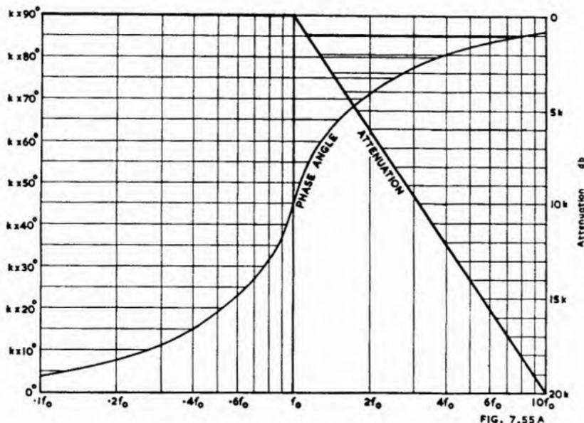
Fig. 7.55A. Phase angle for attenuation characteristic as shown;  $k = 1$  for 6db/octave,  $k = 2$  for 12db/octave etc. (Based on Bode, Refs. H6, H11).
