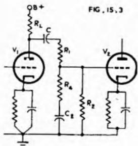
Fig. 15.3. Conventional bass boosting circuit (plate shunt compensation).
