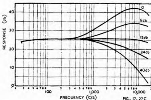
*Fig. 17.27. (A) Circuit of continuously variable equalizing pre-amplifier (B) Variation in attenuation in low frequency control (C) Variation in attenuation in high frequency control (Ref. 246).*
