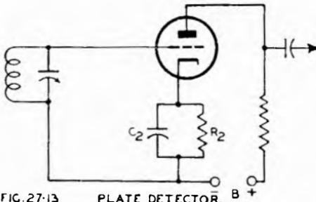
FIG. 27.13 PLATE DETECTOR.
