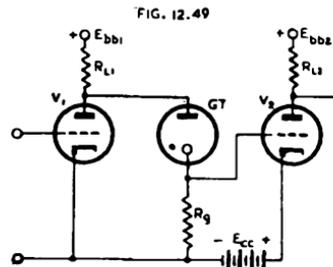
Fig. 12.49. Two stage amplifier with gas tube coupling from the plate of the first stage to the grid of the second stage.
