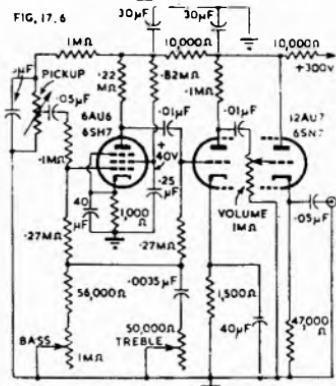
*Fig. 17.6. Pre-amplifier for use with strain-sensitive pickup (Ref. 336)*
