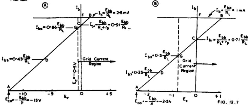
Fig. 12.7. “Ideal” linear dynamic characteristics (A) for general purpose triode with  $\mu = 20$ ,  $r_p = 10\,000$  ohms,  $R_L = 0.1$  megohm and  $E_{bb} = 250$  volts; (B) for high- $\mu$  triode with  $\mu = 100$ ,  $r_p = 0.1$  megohm,  $R_L = 0.25$  megohm and  $E_{bb} = 250$  volts.
