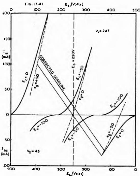
Fig. 13.41. Composite characteristics for two different valves (2A3 and 45) in Class A<sub>1</sub> push-pull.  $E_{bb} = 250$  volts,  $E_c = -50$  volts,  $R_L = 5800$  ohms plate-to-plate.
