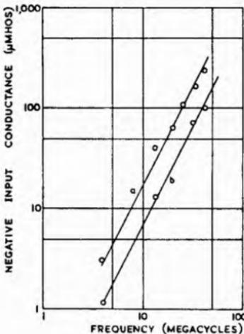
Fig. 25.11. Signal-grid (grid No. 4) conductance of a typical mixer designed for inner-grid injection of oscillator. Lines are drawn with slope of 2. Curve a taken with  $E_c = 0$ ,  $E_4 = -3$  volts. Curve b taken with  $E_{c1} = -6$ ,  $E_4 = -6$  volts.
