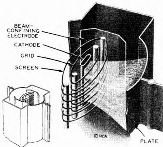
ELECTRON BEAM SHEETS FORMED BY GRID WIRES
