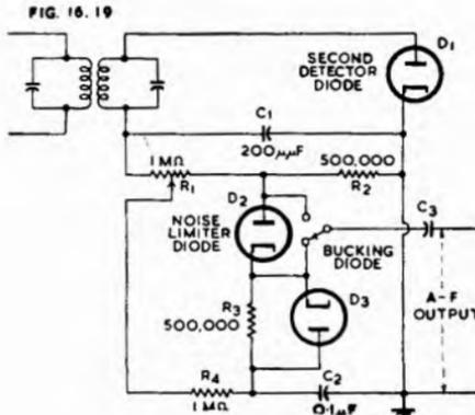
Fig. 16.19. Series-type noise limiter with threshold adjustment (Ref. 30).
