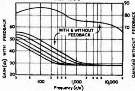
Fig. 17.19B. Frequency characteristics of circuit of Fig. 17.19A with high frequency control in "flat" position (Ref. 239).
