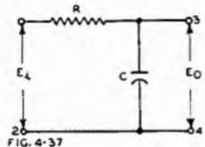
Fig. 4.37. Is a low pass resistance-capacitance filter
