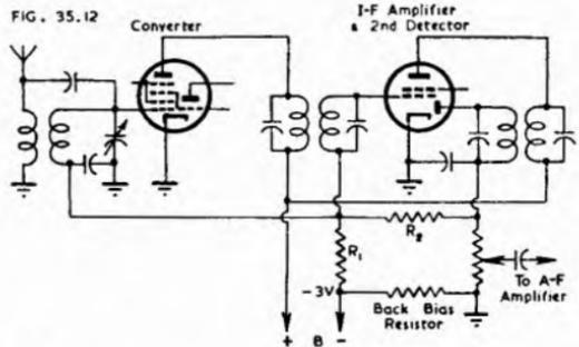
Fig. 35.12. A.V.C. circuit suitable for 3/4 valve receiver.
