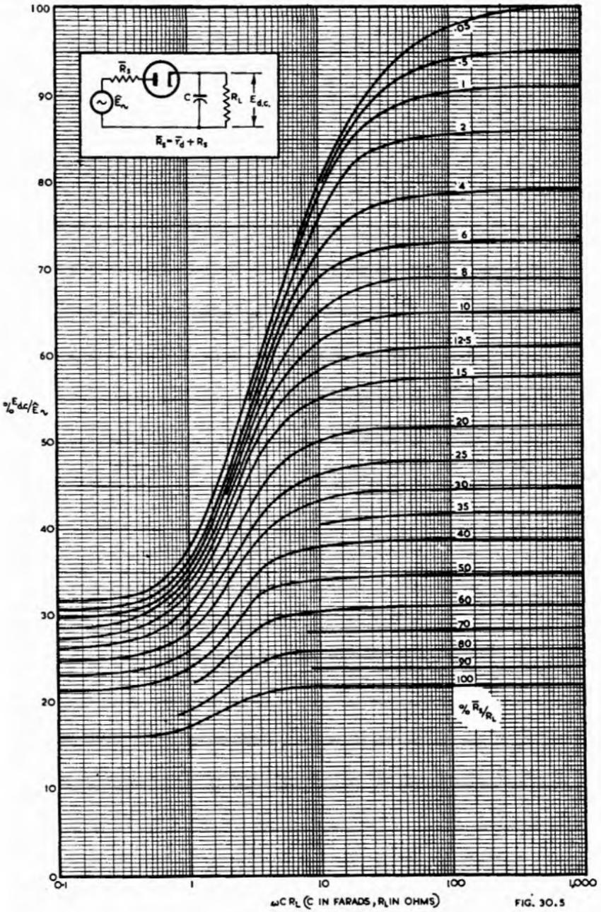
Fig. 30.5. Ratio of rectified (direct) output voltage to peak a.c. rectifier input voltage expressed as a percentage, as a function of  $\omega CR_L$  for a half-wave rectifier with a condenser input filter (Ref. 6).
