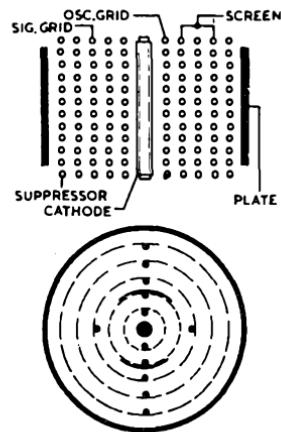
Fig. 25.27. Electrode arrangement of the pentagrid type 6SA7(GT).
