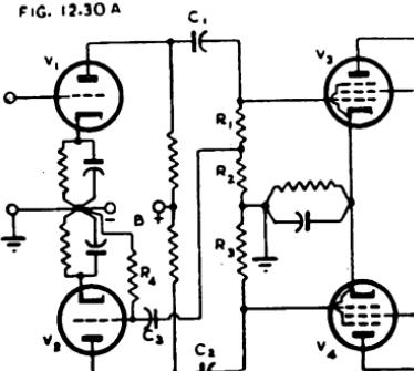
Fig. 12.30A. Conventional form of phase inverter in which  $V_1$  excites  $V_3$ , and  $V_2$  excites  $V_4$ , the grid of  $V_4$  being connected to a tapping on the grid resistor of  $V_3$ .
