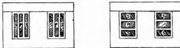
Fig. 5.13A. Typical coil arrangements in audio transformers.
