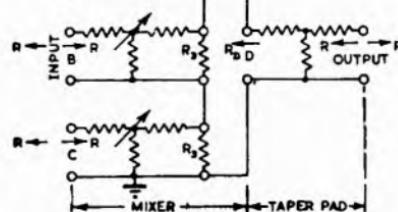
If this mixer is followed by a transformer there is no further loss, but if it is followed by a taper pad as in Fig. 18.28 there must be added the loss in the taper pad, the value of which is given by
