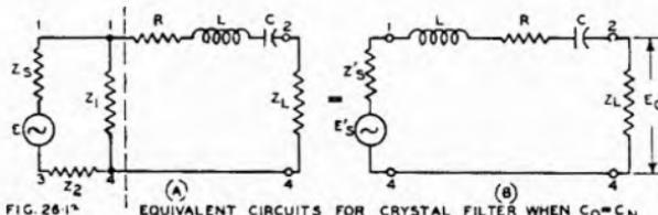
FIG. 26.13 (A) EQUIVALENT CIRCUITS FOR CRYSTAL FILTER WHEN  $C_0 = C_N$
