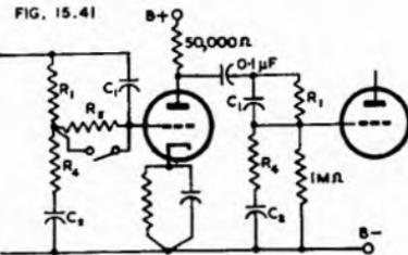
Fig. 15.41. Circuit giving fixed bass and treble boosting (Ref. 7).
