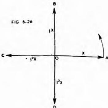
If the operator *j²* is applied twice in succession, the result should be equivalent to multiplication by  $-1$  twice in succession, i.e.  $(-1) \times (-1) = +1$ . This is so, because the operator *j⁴* brings the vector back to its original direction.
