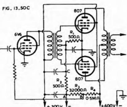
Fig. 13.50C. Class AB<sub>2</sub> amplifier with stabilized bias and screen voltages (Ref. E26).
