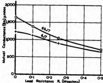
Fig. 12.14B. Mutual conductance of resistance-capacitance coupled pentodes types 6J7 and 6S7 plotted against load resistance. In each case the value of  $K$  is taken as being adjusted to give maximum mutual conductance.
