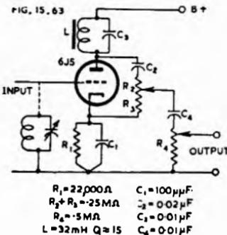
Fig. 15.63. Narrow-band rejection filter for 9 Kc/s (Ref. 74).
