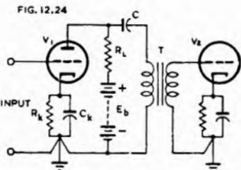
Fig. 12.24. Circuit diagram of parallel-fed transformer-coupled voltage amplifier.
