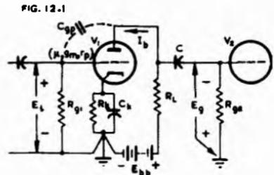
Fig. 12.1. Triode valve ( $V_1$ ) resistance-capacitance coupled to  $V_2$ .
