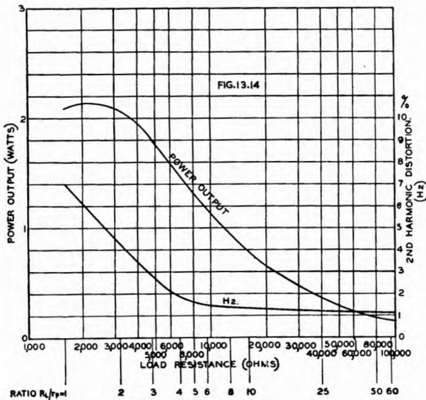
Fig. 13.14. Power output and distortion of type 45 triode plotted against load resistance. The curves were derived graphically, with allowance for shifting loadline. The operating conditions are:  $E_b = 250$  volts,  $F_c = -50$  volts, peak grid signal voltage 50 volts,  $I_b = 34$  mA (zero signal),  $r_p = 1610$  ohms.
