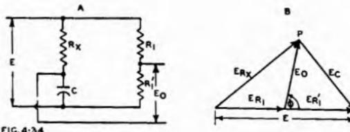
Fig. 4.34 (A) A phase-shift network providing full range phase shifting from 0 to  $180^\circ$  with 6 db attenuation for all degrees of phase shift (B) vector diagram of voltage relationships.
