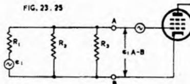
Fig. 23.25. Circuit for reflecting various voltages to the grid (Ref. B33). To find the effective voltage of the antenna, the tuned circuit, and the induced grid noise at the grid of the tube let  $R_1$  equal one of the above noise resistances and  $e_1$  its generated voltage. If  $R_2$  and  $R_3$  equal the other two noise resistances the effective voltage at the grid is
