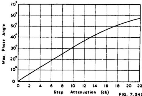
Fig. 7.54C. Maximum phase shift as a function of attenuation in the circuit of Fig. 7.59A (Ref. H18).
