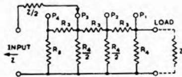
Fig. 18.14. Modified form of ladder attenuator.
