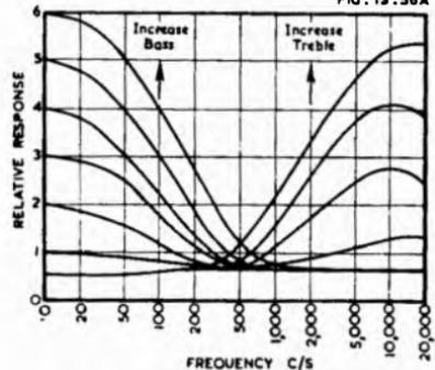
Fig. 15.56A. Response characteristics of Patchett tone control circuit with S<sub>1</sub> open and S<sub>2</sub> closed, and other control at minimum (Ref. 9).
