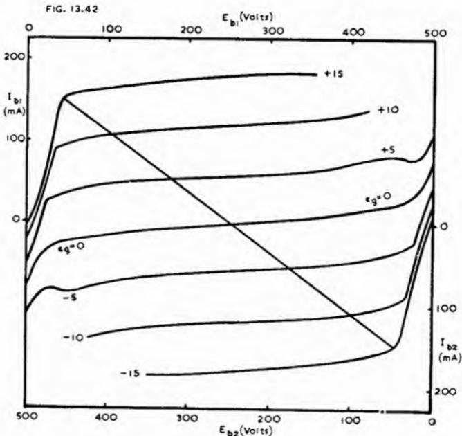
Fig. 13.42. Composite characteristics for push-pull Class A<sub>1</sub> beam power amplifiers type 6L6,  $E_{b0} = 250$  volts,  $E_{c2} = 250$  volts,  $E_{c1} = -15$  volts.
