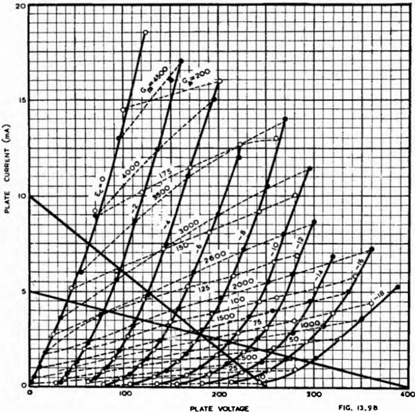
Fig. 13.9B. Plate characteristics type 6J5 with  $g_m$  and  $g_b$  curves and loadlines (Ref. B5).
