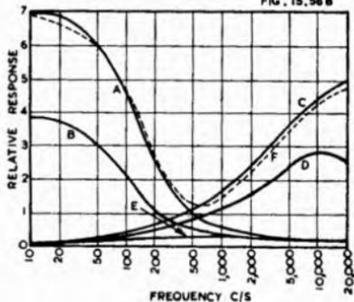
Fig. 15.56B. Response characteristics of Patchett tone control circuit with S<sub>1</sub> closed and S<sub>2</sub> open (Ref. 9).
