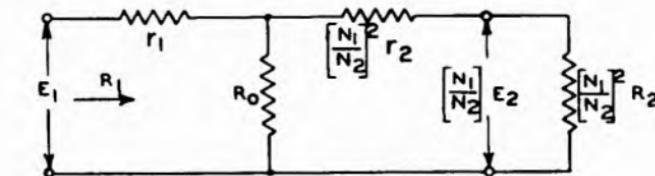
Fig. 5.11. Simplified equivalent circuit referred to the primary.
