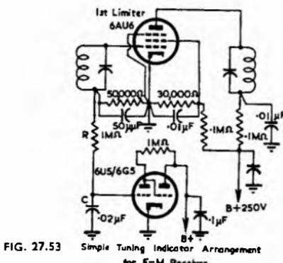
FIG. 27.53 Simple Tuning Indicator Arrangement for F-M Receiver
