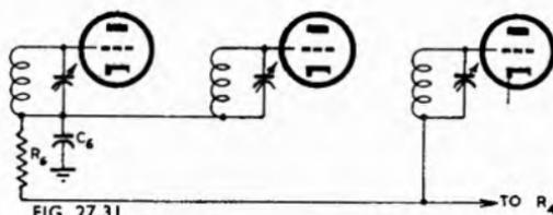
With the r.f. stages an alternative arrangement is to insulate the rotor of the ganged capacitors, and to by-pass it to earth by a single capacitor ( $C_6$ , Fig. 27.31). This enables the a.v.c. voltage to be applied without using any blocking capacitors in the r-f tuned circuits, and has the further advantage that the time constant of the a.v.c. circuit may be made small. The arrangement also has obvious disadvantages and is little used.
