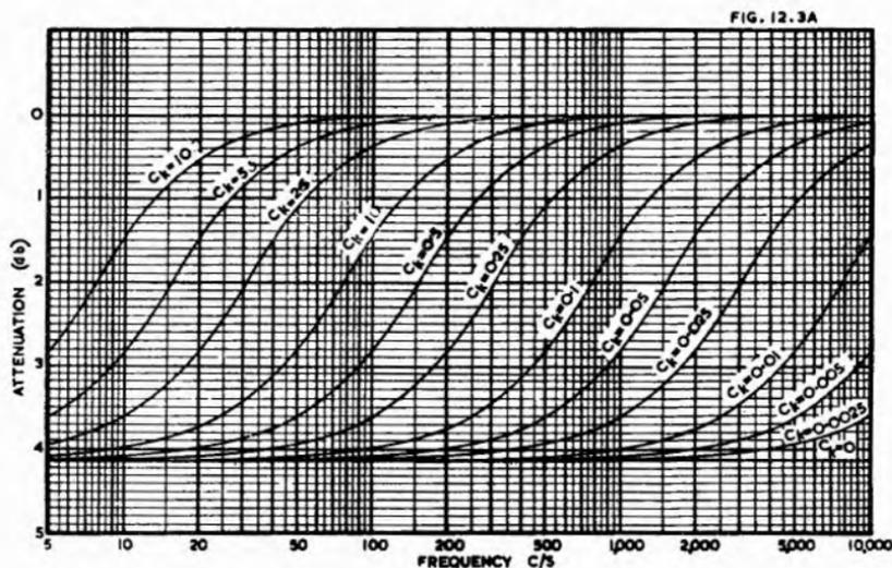
Fig. 12.3A. Frequency characteristics due to cathode by-pass condenser with general purpose triode having  $\mu = 20$ ,  $r_p = 10,000$  ohms,  $R_L = 0.1$  megohm,  $R_{g2} = 0.5$  megohm,  $R_k = 2700$  ohms.
