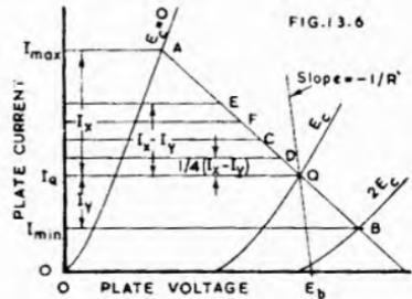
Fig. 13.6. Plate characteristics of triode exaggerated to show rectification effects.
