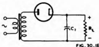
Fig. 30.1F. Basic circuit diagram of full-wave rectifier with condenser input filter.
