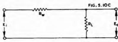
Fig. 5.10C. Medium frequency equivalent circuit.
