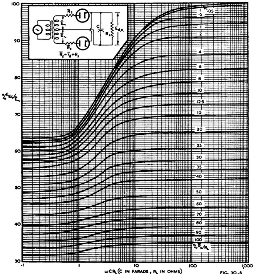
Fig. 30.6. Ratio of rectified (direct) output voltage to peak a.c. rectifier input voltage, expressed as a percentage, as a function of  $\omega CR_L$  for a full-wave rectifier with a condenser input filter (Ref. 6).
