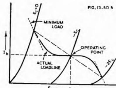
Fig. 13.50B. Loadline on a typical triode driver.
