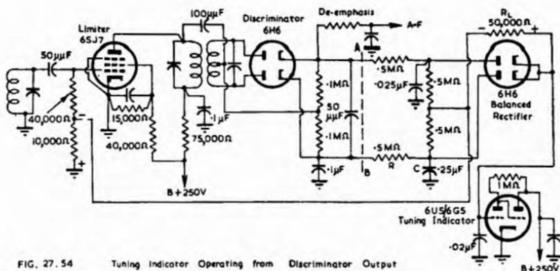
FIG. 27.54 Tuning Indicator Operating from Discriminator Output
