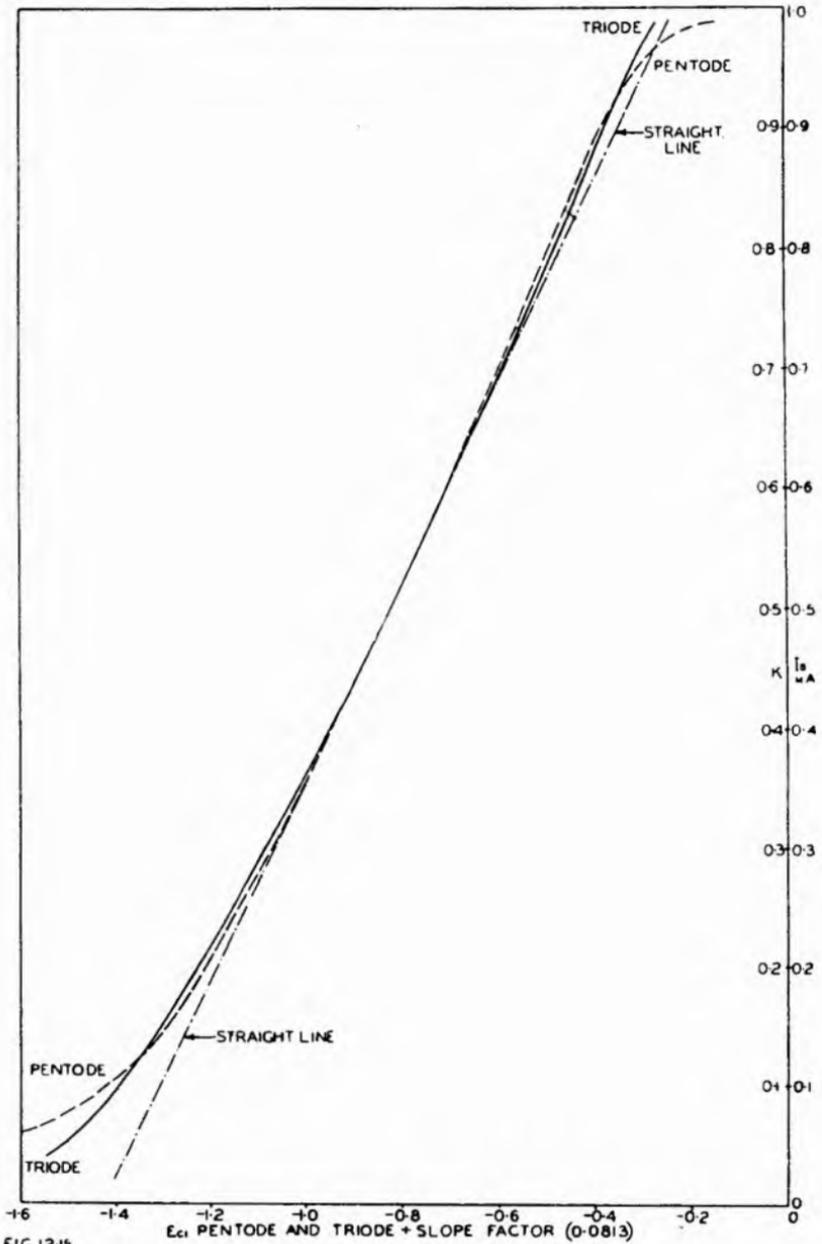
Fig. 12.15. Comparison between pentode and triode dynamic characteristics of the same valve (6SJ7 with  $E_{b} = 250$  volts,  $R_L = 0.25$  megohm,  $E_{c2} = 22.5$  volts for pentode,  $E_{c2}$  connected to plate for triode characteristics; triode characteristics divided by slope factor 0.0813 and superimposed so that points for  $I_b = 0.5$  mA coincide).
