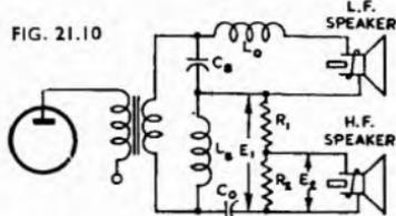
Fig. 21.10. Complete circuit from valve plate to loudspeakers, incorporating the filter of Fig. 21.8 with an attenuator on the h.f. speaker.
