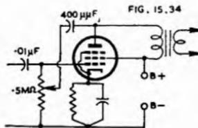
Fig. 15.34. Power amplifier valve with variable negative feedback at high audio frequencies (treble attenuation).
