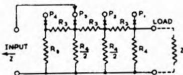
Fig. 18.13. Ladder attenuator ( $\Pi$  section).
