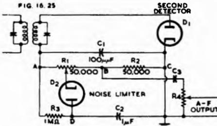
Fig. 16.25. Diode shunt-type noise limiter (Ref. 30).
