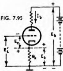
Fig. 7.95. Basic circuit of cathode degenerative triode.
