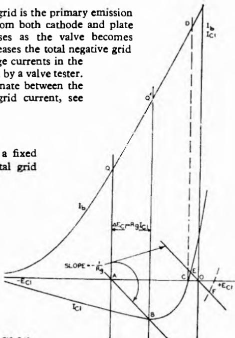
Fig. 2.10. Grid current characteristics with grid loadlines.
