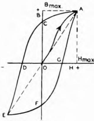
Fig. 5.16. Hysteresis loop of a typical magnetic material.
