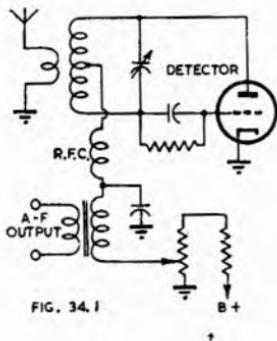
Fig. 34.1. Self quenched superregenerative receiver incorporating linear reflex detector.
