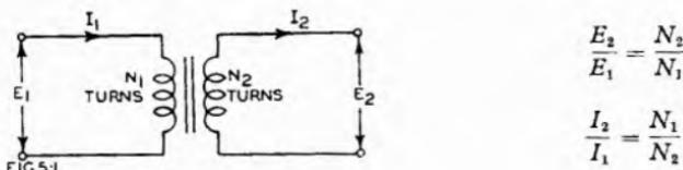
*Fig. 5.1. Ideal two-winding transformer.  $E_1$  and  $E_2$  are alternating voltages (r.m.s.).  $I_1$  and  $I_2$  are alternating currents (r.m.s.) but the indicated directions of current flow are at a chosen instant and correspond to the direction of voltage at that instant. Similar remarks apply to Fig. 5.2.*
