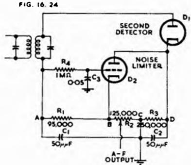
Fig. 16.23. Balancing-type noise limiter (Ref. 30).
