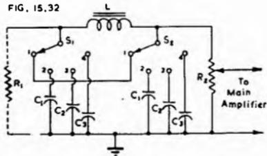
Fig. 15.32. Approximate constant  $k$  low-pass  $\Pi$  section filter.  $R_1 =$  source impedance. When  $R_1 = R_2 = 0.1 M\Omega$ ,  $L = 5 H$ ,  $C_1 = 0.0001$ ,  $C_2 = 0.0002$  and  $C_3 = 0.0004 \mu F$ , the cut-off frequencies will be (1) none (2) 10 000 c/s (3) 7000 c/s (4) 5000 c/s.
