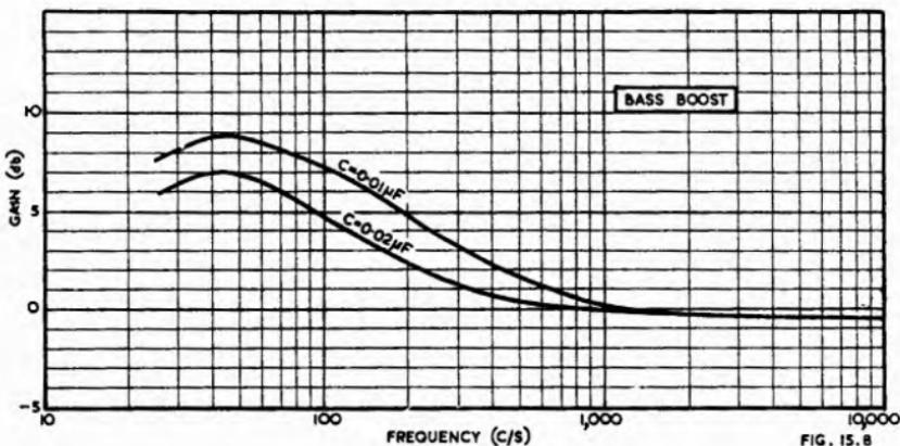
Fig. 15.8. Frequency characteristics with the circuit of Fig. 15.7,  $V_1 = 6J7$ ,  $R_L = 0.05 M\Omega$ ,  $R_1 = 0.2 M\Omega$ ,  $R_t = 2000 \Omega$ ,  $C_k = 25 \mu F$ ,  $R_s = 1.5 M\Omega$ ,  $C_s = 0.1 \mu F$ ,  $C = 0.02 \mu F$ ,  $R_g = 1 M\Omega$ .
