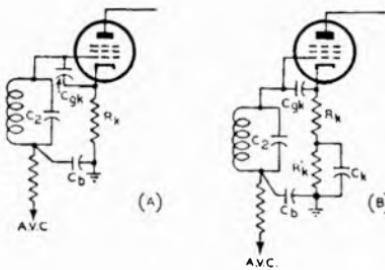
FIG. 26.18 METHOD FOR REDUCING VARIATIONS OF INPUT ADMITTANCE
