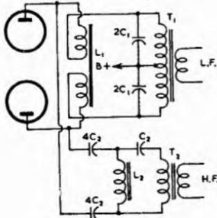
Fig. 21.9. Alternative form of divider network using two stepdown transformers (Ref. 9).
