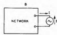
Fig. 4.32. (A) An impedance  $Z$  in a network with current  $I$  and voltage drop  $ZI$  (B) Equivalent circuit having identical results so far as current and voltage drop are concerned, with a generator developing a voltage  $E = ZI$ . This illustrates the Compensation Theorem.
