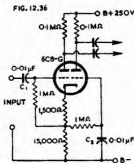
Fig. 12.36. Practical "Schmitt" common cathode impedance self-balancing inverter using type 6C8-G twin triode ( $\mu = 36$ ).  $C_1$  and  $C_2$  should have high insulation resistance.
