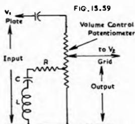
Fig. 15.59. Tone-compensated volume control with tapped potentiometer.
