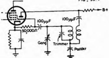
Fig. 35.7. Oscillator circuit with padder feedback.
