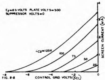
Fig. 2.8. Screen current mutual characteristics of a pentode (same as for Fig. 2.7).
