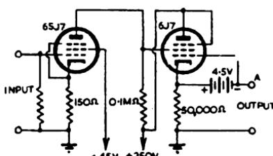
Fig. 12.48. Two stage amplifier with the plate of the first stage directly-coupled to the screen of the second stage (Ref. D14).
