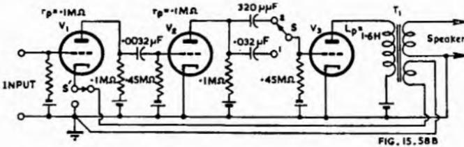
Fig. 15.58B. Use of feedback to provide special attenuation characteristics at low frequencies. The total effective resistance across  $T_1$  primary is taken as 1000 ohms. Switch  $S_1$  normal;  $S_2$  tone control (low frequency attenuation). Switch  $S'$  controls feedback.
