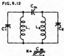
Fig. 9.12. High impedance capacitive coupling.
