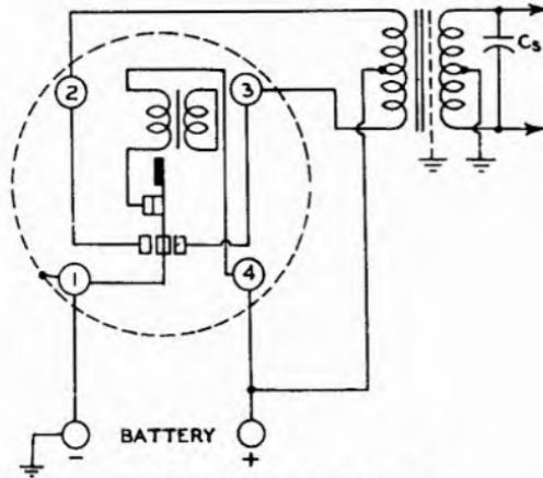
FIG. 32.1 INTERRUPTER TYPE VIBRATOR.
