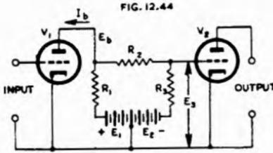
Fig. 12.44. "Bridge" circuit, direct-coupled amplifier.
