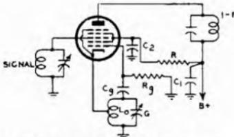
FIG. 24-6 PENTAGRID CONVERTER USING ELECTRON-COUPLED HARTLEY OSCILLATOR
