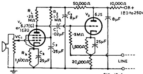
This circuit has the disadvantage that the cathode follower stage may give rise to audible hum. It should therefore be restricted to use with a sensitive type of crystal microphone or to applications where a low hum level is not essential.
