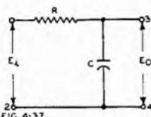
FIG. 4.37. Is a low pass resistance-capacitance filter
