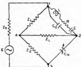
FIG. 26-11 CIRCUIT ARRANGEMENT FOR VARYING  $C' (= C_0 - C_N)$
