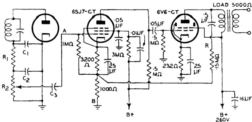
FIG. 27-3 AUDIO AMPLIFIER GIVING LOW A.C. SHUNTING ACROSS DIODE LOAD.
