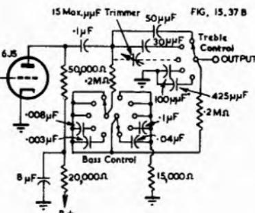
Fig. 15.37B. Step-type tone control not using inductors (Ref. 70).
