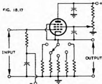
Fig. 18.17. Electronic attenuator using cathode follower (Ref. C15).
