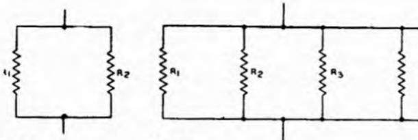
Fig. 4.8. Two resistances in parallel. Fig. 4.9. Several resistors in parallel.
