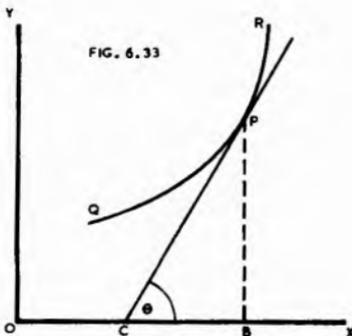
When a line is curved, its slope varies from point to point. The slope at any point is given by the slope of the tangent at that point. In Fig. 6.33 the curve is QPR, and the slope at P is given by  $BP/CB$  or  $\tan \theta$ .
