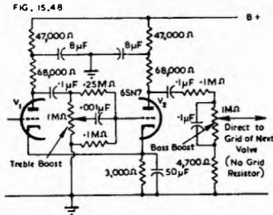
Fig. 15.48. Two-stage bass and treble tone control (Ref. 41).
