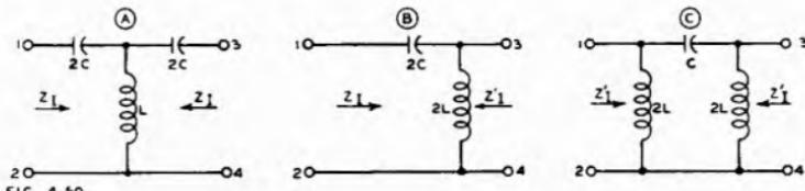
Fig. 4.50. Three varieties of high-pass constant  $k$  filters (A) T section (B) Half section (C) II section.
