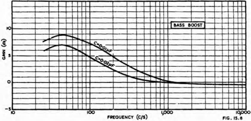
Fig. 15.8. Frequency characteristics with the circuit of Fig. 15.7,  $V_1 = 6J7$ ,  $R_L = 0.05 M\Omega$ ,  $R_1 = 0.2 M\Omega$ ,  $R_k = 2000 \Omega$ ,  $C_k = 25 \mu F$ ,  $R_2 = 1.5 M\Omega$ ,  $C_1 = 0.1 \mu F$ ,  $C = 0.02 \mu F$ ,  $R_o = 1 M\Omega$ .
