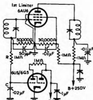
FIG. 27.53 Simple Tuning Indicator Arrangement for F-M Receiver
