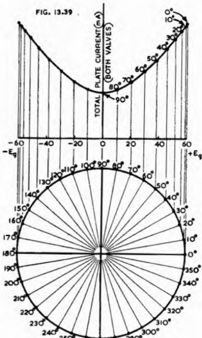
Fig. 13.39. Plate current (both valves) with 10° angular increments.
