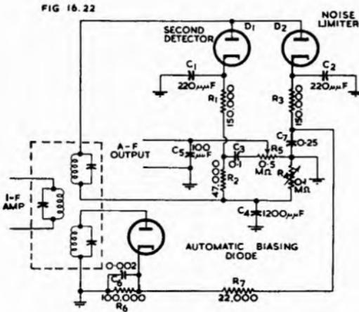
Fig. 16.22. Automatic balanced-detector noise limiter. (Ref. 30).
