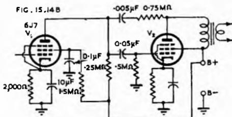
Fig. 15.14B. Amplifier with  $0.005 \mu\text{F}$  condenser in feedback network to provide bass boosting.  $V_2$  is a power amplifier valve (Ref. 68).
