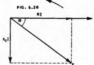
A similar procedure applies with a capacitance instead of an inductance (Fig. 6.28) except that the capacitive reactance is  $X_C$  instead of  $X_L$  and the vector of peak voltage drop across  $C$  ( $X_C I$ ) is drawn vertically downwards, since it must be opposite to  $X_L I$ . The current ( $I$ ) here leads the voltage ( $E$ ) by the angle  $\theta$ .
