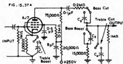
Fig. 15.37A. Simple universal tone control not using inductors.
