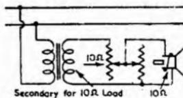
It is important to check for the phasing of the two loudspeakers ; in the vicinity of the cross-over frequency both units should be in phase (aiding one another). This may be checked by the use of a single dry cell connected in series with the secondary of the transformer ; in the case of 2 ohm voice coils there may be a 5 ohm limiting resistor connected in series with the cell.
