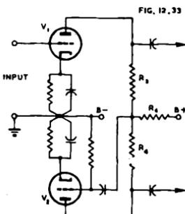
Fig. 12.33. Common plate impedance self-balancing phase inverter.
