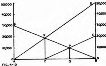
Fig. 4.10. Graphical method for the determination of the effective resistance of two or more resistors in parallel (after *Wireless World*).
