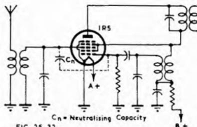
Fig. 25.32. Circuit for short-wave operation of 1R5 converter.
