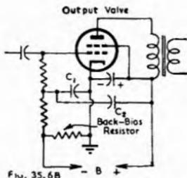
Fig. 35.6B. Reduction of "flutter" by negative feedback.
