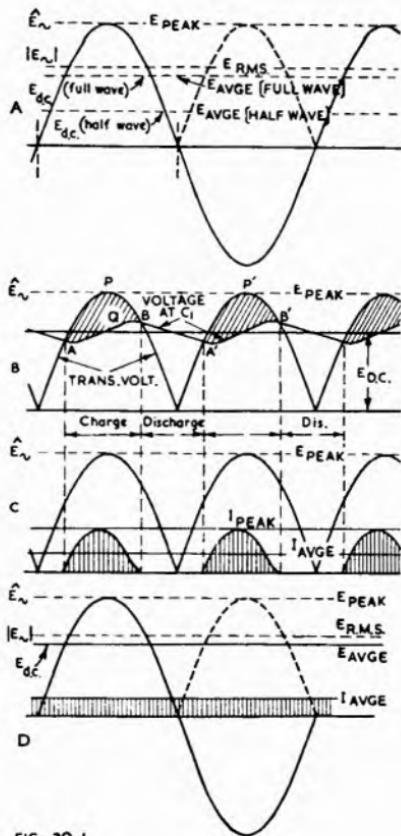
Fig. 30.1. (A, B, C & D). Voltage and current waveforms of condenser input and choke input rectifier systems. The symbols on the left are those used in Section 2.
