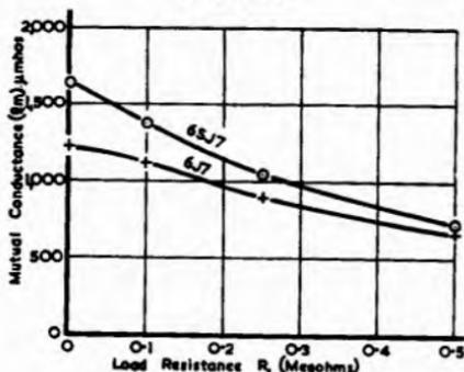
Fig. 12.14B. Mutual conductance of resistance-capacitance coupled pentodes types 6J7 and 6SJ7 plotted against load resistance. In each case the value of  $K$  is taken as being adjusted to give maximum mutual conductance.
