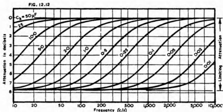
Fig. 12.12. Attenuation characteristics for selected values of cathode by-pass condenser with valve type 6J7 and  $E_{bb} = 250$  volts,  $R_L = 0.25$ ,  $R_g = 0.5$ ,  $R_s = 1.5$  megohms,  $R_k = 2000$  ohms: screen adequately by-passed.
