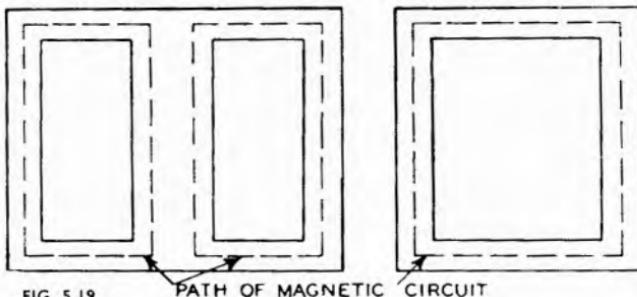
FIG. 5.19 PATH OF MAGNETIC CIRCUIT
