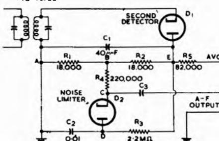
Fig. 16.26. Modified shunt noise limiter (Ref. 30).
