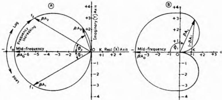
Fig. 7.53. (A) Locus of  $\beta A$  vectors ("Nyquist diagram") for a single stage resistance capacitance coupled triode amplifier with fixed bias (B) Similar locus for a 2 stage amplifier.
