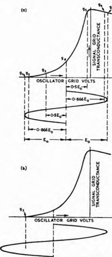
Fig. 25.2a. Points used for 30-degree analysis of conversion transconductance.
