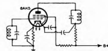
FIG. 23-8 R-F AMPLIFIER WITH TWO CATHODE CONNECTIONS.
