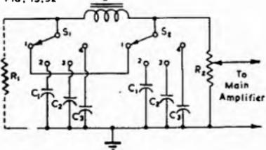
Fig. 15.32. Approximate constant  $k$  low-pass  $\Pi$  section filter.  $R_1 = \text{source impedance}$ . When  $R_1 = R_2 = 0.1 M\Omega$ ,  $L = 5 H$ ,  $C_1 = 0.0001$ ,  $C_2 = 0.0002$  and  $C_3 = 0.0004 \mu F$ , the cut-off frequencies will be (1) none (2) 10 000 c/s (3) 7000 c/s (4) 5000 c/s.
