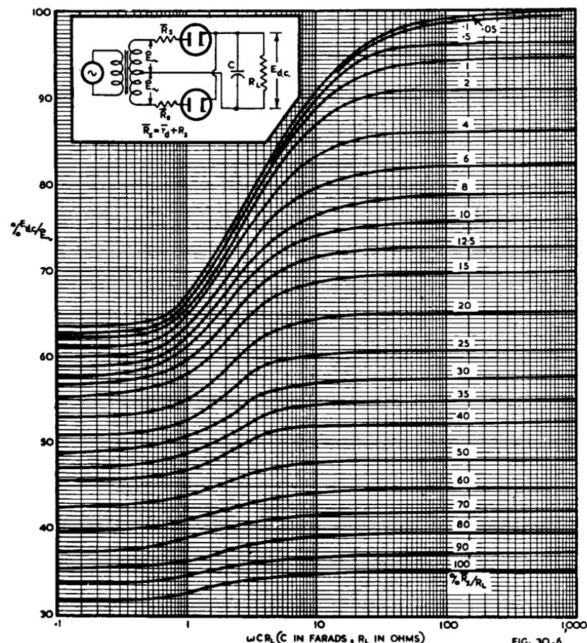
Fig. 30.6. Ratio of rectified (direct) output voltage to peak a.c. rectifier input voltage, expressed as a percentage, as a function of  $\omega CR_L$  for a full-wave rectifier with a condenser input filter (Ref. 6).
