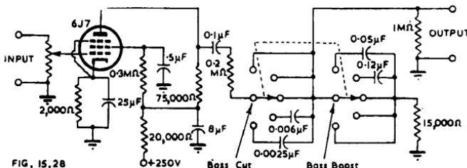
Fig. 15.28. Step-control giving bass boosting and bass attenuation.
