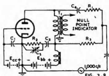
Fig. 3.9. Method of testing for plate resistance.
