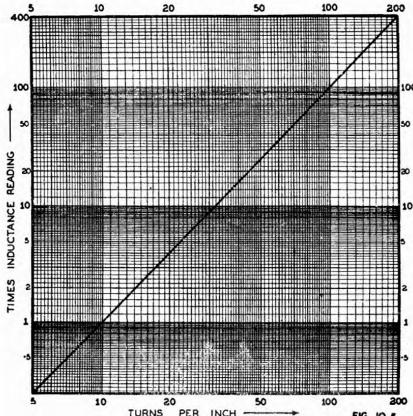
Fig. 10.5. Winding pitch correction for Fig. 10.4.
