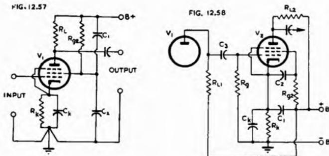
Fig. 12.57. Hum neutralization in a r.c.c. pentode.
