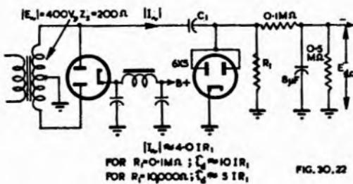
Fig. 30.22. Shunt diode bias supply with r.c. filtering.
