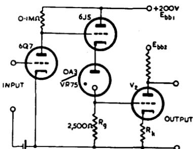
Fig. 12.50. Improved two stage amplifier with gas tube coupling, in which a cathode follower is introduced for better performance.
