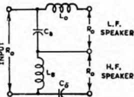
Fig. 21.8. Filter type frequency dividing network, series connection.
