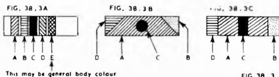
Fig. 38.3A. British Standard coloured band marking (preferred).
