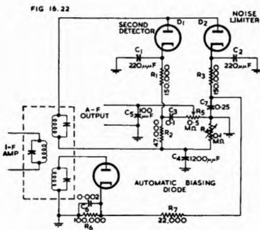
Fig. 16.22. Automatic balanced-detector noise limiter. (Ref. 30).
