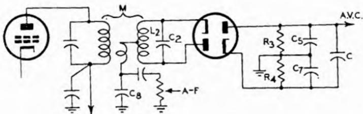
FIG. 27.22 BALANCED TYPE OF RATIO DETECTOR CIRCUIT.
