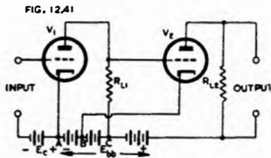
Fig. 12.41. Direct-coupled amplifiers without "hot" grid bias battery.
