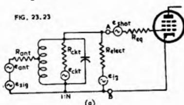
$R_{ant}$  = Antenna Radiation Resistance
