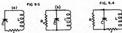
Fig. 9.3(a). Parallel resonance with series loss resistance.
