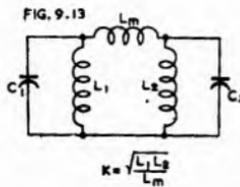
Fig. 9.13. High impedance inductive coupling.
