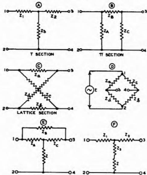
FIG. 4.33 Four Terminal Networks (A) T Section (B)  $\Pi$  Section (C) Lattice Section (D) Lattice Section redrawn in the form of a bridge (E) Bridged T Section (F) T Section equivalent to Bridged T.
