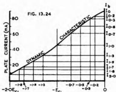
Fig. 13.24. Calculation of pentode power output and distortion using the eleven selected ordinate method.
