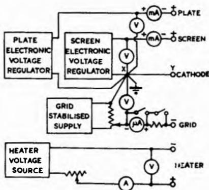
Fig. 3.1. Basic circuit for testing electrode currents.
