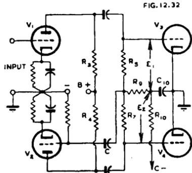
Fig. 12.31. The Floating Paraphase self-balancing phase inverter with cathode bias.
