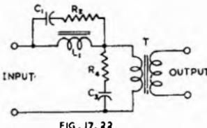
Fig. 17.22. Bass equalizer incorporating  $L$ ,  $C$  and  $R$  (Ref. 188).
