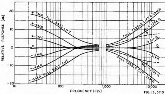
*Fig. 15.57D. Measured frequency response curves of circuit of Fig. 15.57C. Labels on curves are resistance values between potentiometer slider and centre of element. Dotted curves are with  $P_2$  centre-tap disconnected from earth and with one  $0.33 M\Omega$  resistor connected from each end of  $P_2$  to earth (Ref. 91).*
