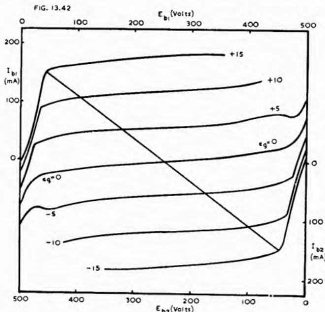
Fig. 13.42. Composite characteristics for push-pull Class A<sub>1</sub> beam power amplifiers type 6L6,  $E_{bb} = 250$  volts,  $E_{cg} = 250$  volts,  $E_{cl} = -15$  volts.
