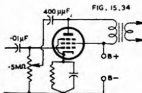
Fig. 15.34. Power amplifier valve with variable negative feedback at high audio frequencies (treble attenuation).
