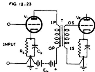
Fig. 12.23. Circuit diagram of transformer-coupled voltage amplifier
