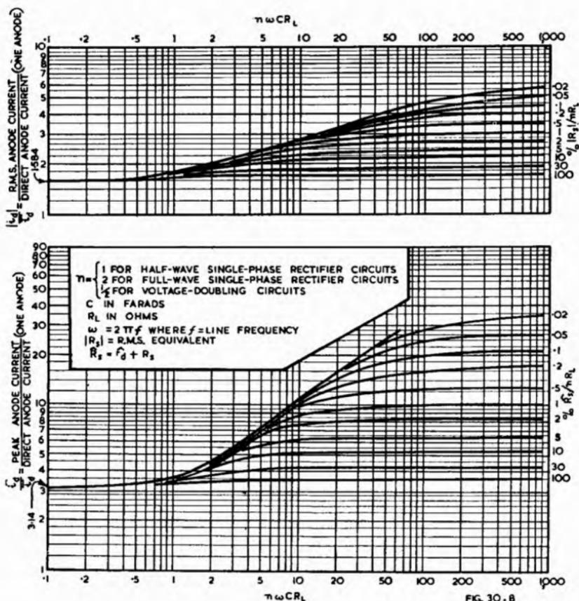
Fig. 30.8 (above). Ratio of r.m.s. diode current to average diode current for one anode, expressed as a function of  $\omega CR_L$ ; (below) Ratio of peak diode current to average diode current for one anode, expressed as a function of  $\omega CR_L$  (Ref. 6).
