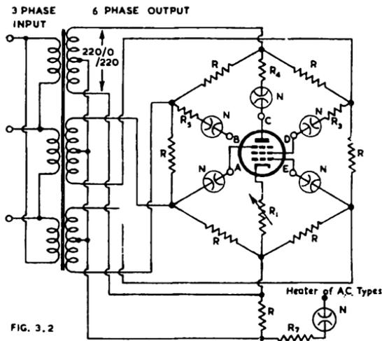
Fig. 3.2. Hexaphase shorts and continuity tester. Suitable values are  $R=5000$  ohms,  $R_3=R_5=7500$  ohms,  $R_4=1500$  ohms,  $R_7=5000$  ohms,  $R_1=50\,000$  ohms for battery valves other than power output, 33 000 ohms for normal a.c. types, or 15 000 ohms for power output valves. Lamps (N) are 110 volt  $\frac{1}{2}$  watt split-anode neon.
