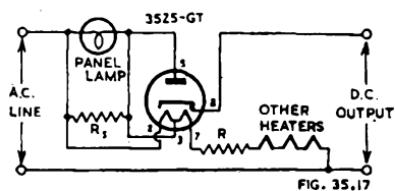
Fig. 35.17. Circuit using 35Z5-GT and dial lamp. The drop across  $R_s$  and all heaters (with panel lamp) should equal 117 volts at 0.15 ampere.  $R_s$  = shunting resistor required when d.c. output current exceeds 60 mA.
