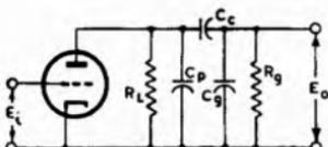
Fig. 7.74. Resistance-capacitance coupled stage.
