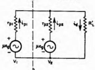
Fig. 13.35. Equivalent circuit which may be used for deriving certain impedance and current relationships.
