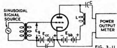
Fig. 3.11. Method for testing for power output.
