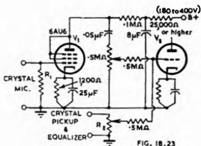
Fig. 18.23. Complete pre-amplifier incorporating parallel network mixer, for use with high level crystal microphone and crystal pickup.  $R_1 = 1$  to  $5M\Omega$ ;  $R_2 = 0.5M\Omega$  or higher. Gain in  $V_1$  is 30 dbvg.
