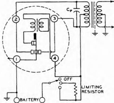
FIG. 32.13 STARTING ARRANGEMENTS FOR 24 AND 32 VOLT VIBRATORS.
