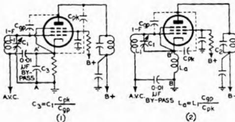
FIG. 26.20 METHODS FOR STABILISING R-F AND I-F AMPLIFIERS
