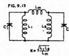
Fig. 9.13. High impedance inductive coupling.
