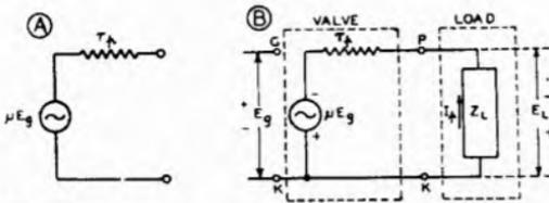
Fig. 2.37. (A) *Equivalent circuit of valve using constant voltage generator* (B) *Equivalent circuit of valve and load.*
