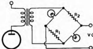
Fig. 16.6. Bridge type of volume expander using lamps.
