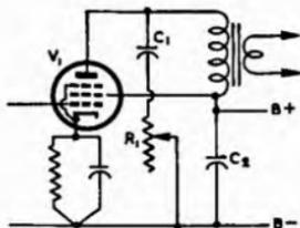
Fig. 15.31. Typical "tone control" used in radio receivers. In a typical case  $C_1 = 0.05 \mu F$ ,  $R_1 = 50\,000 \Omega$  (max.),  $V_1 =$  power pentode with load resistance about 5000 ohms.
