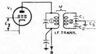
FIG. 26-14 CIRCUIT FOR DETERMINING  $E'_s$
