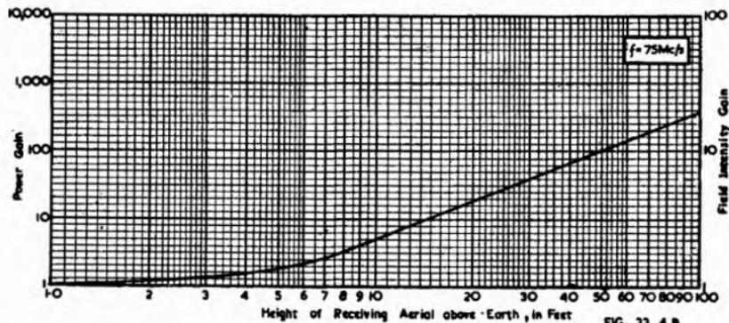
Fig. 22.4 (A) Attenuation at 75 Mc/s of the radiation from a transmitter (1 KW radiated over earth with  $\sigma = 10^{-13}$  e.m.u.,  $\epsilon = 5$ , with receiving aerial at zero height); (B) Multiplying factor for height of receiving aerial above earth.
