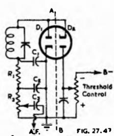
\*Shunt Diode Noise Limiter FIG. 27.47
