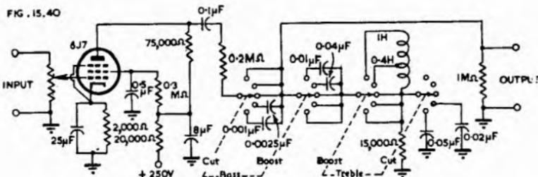
Fig. 15.40. Universal step-type tone control using inductors.
