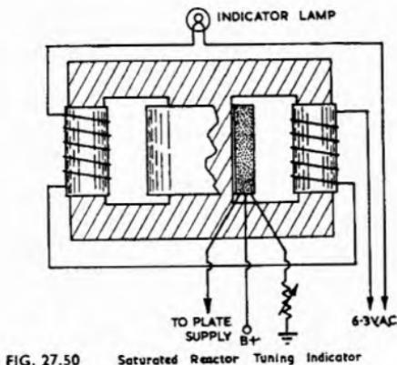
FIG. 27.50 Saturated Reactor Tuning Indicator
