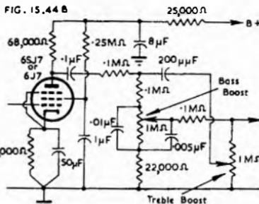
Fig. 15.44A. Simple duo-control circuit giving individual control of bass and treble. Typical values are :  $R_1 = 0.25 \text{ M}\Omega$ ;  $R_2 = R_3 = 0.5 \text{ M}\Omega$ ;  $R_4 = 0.25 \text{ M}\Omega$ ;  $R_5 = R_6 = 0.5 \text{ M}\Omega$ ;  $C_1 = 0.01 \mu\text{F}$ ;  $C_2 = 0.001 \mu\text{F}$  (Ref. 22).
