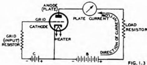
Fig. 1.3. Fundamental circuit including indirectly-heated triode, B and C batteries, and load resistor in plate circuit.
