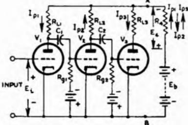
Fig. 12.52. Three stage amplifier demonstrating the effects of impedance ( $R_4$ ) in the power supply.
