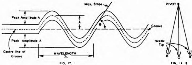
Fig. 17.1. Unmodulated (left) and modulated (right) groove of lateral recording
