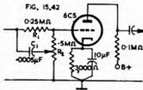
Fig. 15.42. Single control continuously variable tone control (Ref. 22).
