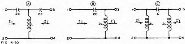
Fig. 4.50. Three varieties of high-pass constant  $k$  filters (A) T section (B) Half section (C)  $\Pi$  section.
