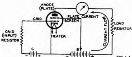
Fig. 1.4. Fundamental circuit including indirectly-heated tetrode, B and C batteries, and load resistor in plate circuit.
