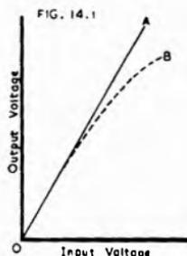
*Fig. 14.1. Linearity characteristic (or transfer characteristic)
