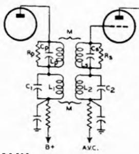
FIG 26.3 ARRANGEMENT FOR F-M AND A-M I-F STAGE
