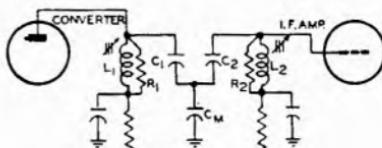
FIG. 26.2 SHUNT CAPACITANCE COUPLED I.F. CIRCUIT
