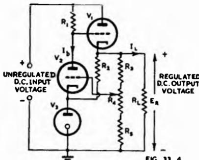
Referring again to Fig. 33.4. If constant output voltage is to be maintained across the load, the valve  $V_1$  must be capable of adjusting its voltage drop to compensate for voltage input changes. A similar condition exists if the input voltage is constant and variable output voltage is required. The valve has therefore to satisfy conditions at four points as set out in Table 2.
