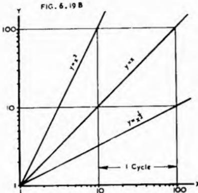
Occasionally it is desirable to use log. log. ruled paper; this is ruled logarithmically on both X and Y axes. An important feature of this form of representation is that a curve of the type
