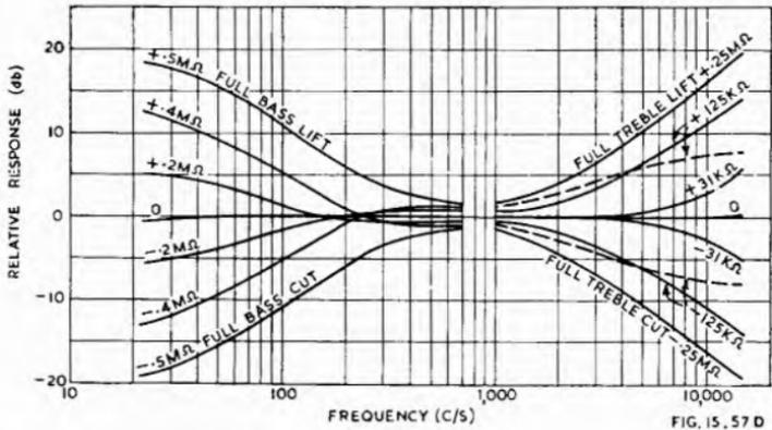
Fig. 15.57D. Measured frequency response curves of circuit of Fig. 15.57C. Labels on curves are resistance values between potentiometer slider and centre of element. Dotted curves are with  $P_2$  centre-tap disconnected from earth and with one  $0.33 M\Omega$  resistor connected from each end of  $P_2$  to earth (Ref. 91).
