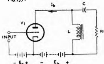
Fig. 13.17. Choke-coupled amplifier.
