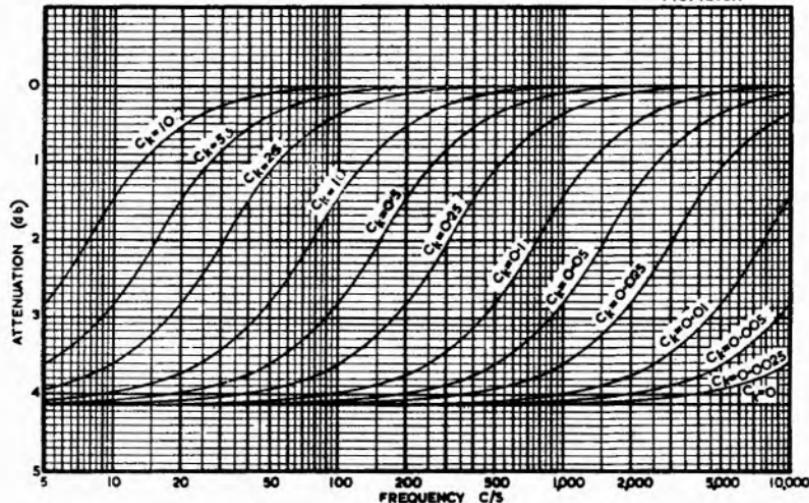
Fig. 12.3A. Frequency characteristics due to cathode by-pass condenser with general purpose triode having  $\mu = 20$ ,  $r_p = 10,000$  ohms,  $R_L = 0.1$  megohm,  $R_{o2} = 0.5$  megohm,  $R_k = 2700$  ohms.
