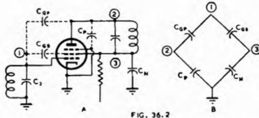
Fig. 36.2. Circuit for i-f amplifier neutralization (A) Actual circuit (B) Capacitance rearranged to show bridge (Ref. 5).
