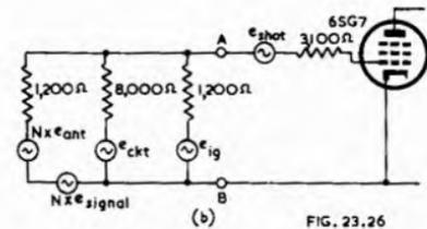
Fig. 23.26. Typical F-M receiver input circuit (Ref. B33).
