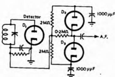
FIG. 27.49 Automatic Noise Limiting Circuit
