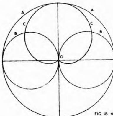
Fig. 18.4. Polar diagrams showing directional characteristics of microphones
