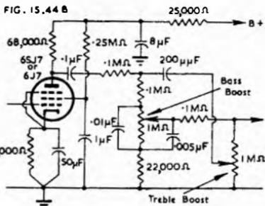
**(B) Duo-control circuit incorporating L and C (Fig. 15.45, Ref. 26)**
