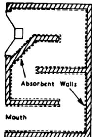
Fig. 20.18. Sectional view of acoustical labyrinth loudspeaker.
