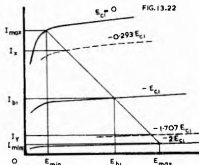
Fig. 13.22. Calculation of pentode power output and distortion using the five selected ordinate method.
