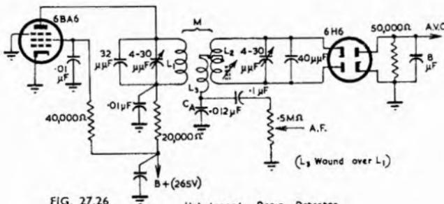
FIG. 27.26 Unbalanced Ratio Detector
