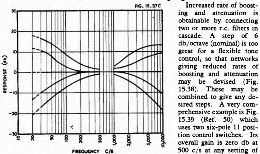
Fig. 15.37C. Frequency response characteristics of the circuit of Fig. 15.37B (Ref. 70).
