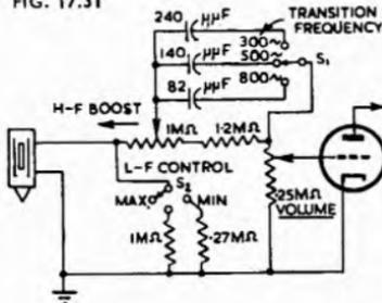
Fig. 17.31. Flexible equalizer for high-fidelity crystal pickups (Ref. 127).
