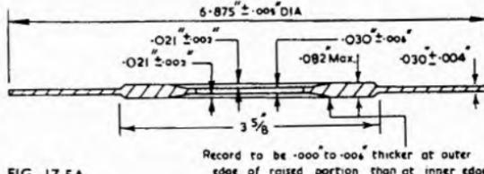
The cross-sectional view of a record is shown in Fig. 17.5A. The outermost music groove is  $6\frac{1}{8}$  inch diameter, while the innermost music groove is 4.875 inches minimum diameter—the latter gives 10% intermodulation distortion and a groove velocity of 11.5 inches per second.
