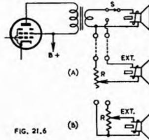
may be neglected provided that  $R$  is not less than five times the voice-coil impedance. At low levels this arrangement has a high impedance but here again the effect will not be serious.
