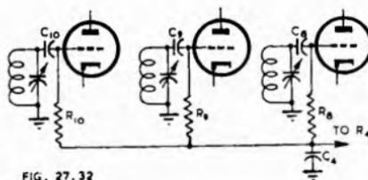
"Parallel feed" for the r-f stages is sometimes more convenient than "series feed," and appears to be satisfactory in most respects, although it has been found that grid blocking is more likely to occur with "parallel feed" than with "series feed."
