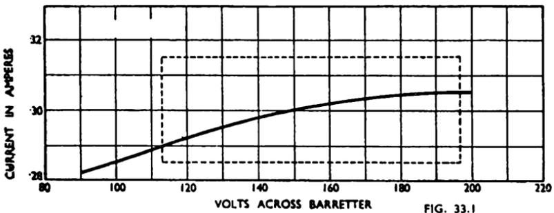
*Fig. 33.1. The characteristic of a typical barretter.*
