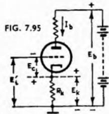
FIG. 7.95. Basic circuit of cathode degenerative triode.
