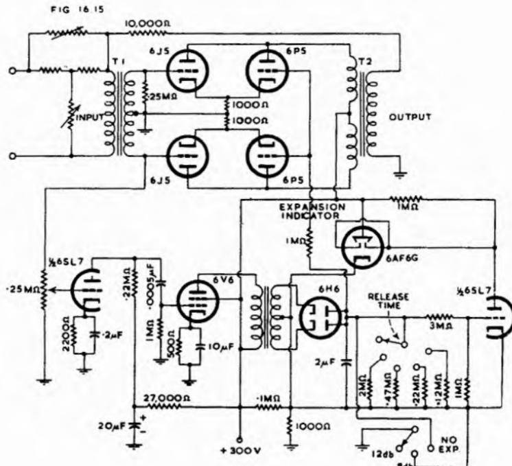
Fig. 16.15. Volume expander incorporating plate resistance control (Ref. 43).
