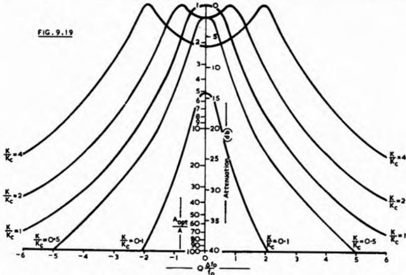
Selectivity Curves for Two Identical Coupled Circuits,
