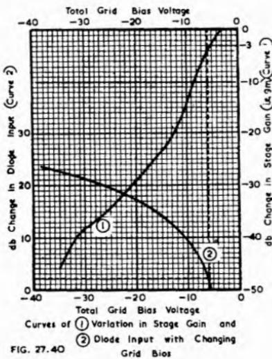
It is now necessary to relate the total bias (a.v.c. + standing bias) to the change in diode input voltage; the change is conveniently expressed in decibels. Any signal voltage applied to the diode may be taken as zero reference level (0 db), and in our case  $E_{r.m.s.} = 2$  volts will be convenient. Then the change in diode input voltage is given by,
