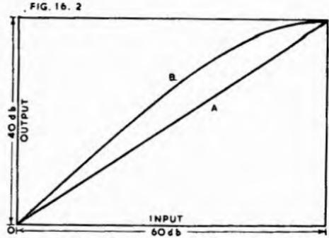
Fig. 16.2. Compression characteristics of volume compressors.
