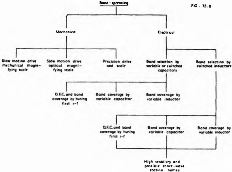
Fig. 35.8. Possible types of bandspreading (from Ref. 14).
