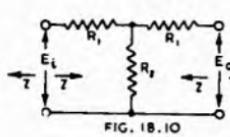
Fig. 18.10. Constant impedance T section attenuator.
