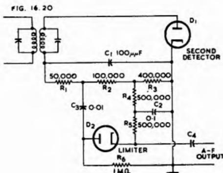
Fig. 16.20. Low-loss series limiter. (Ref. 30).
