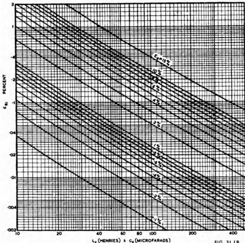
Fig. 31.1B. Approximate relationships between  $ER$ ,  $ER_1$  and  $L_2C_2$  for 50 c/s full-wave rectification (i.e. 100 c/s ripple frequency) and single section filter. For other ripple frequencies, the value of the LC scale should be multiplied by the appropriate factor as follows.
