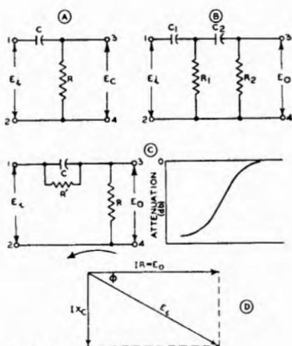
Fig. 4.35. (A) is a resistance capacitance high-pass filter; (B) is a two section filter; (C) is a modified form of A, providing attenuation within top and bottom limits; (D) is the vector diagram of A.
