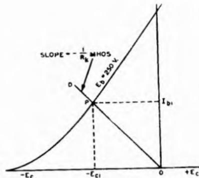
Fig. 2.27. Triode mutual characteristics with cathode bias loadline OD.
