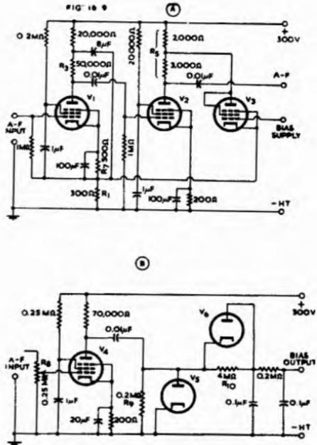
Fig. 16.9. Volume expander using negative feedback ; (A) amplifier (B) circuit for supplying control bias to the amplifier (Refs. 22, 24).  $V_1 = V_2 = V_3 = V_4 = SP41$  ;  $V_5$  and  $V_6$  together = 6H6.
