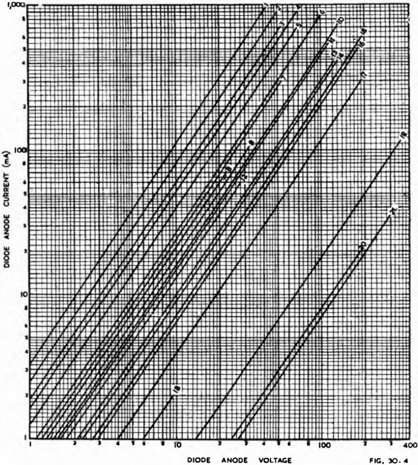
Fig. 30.4. Average anode characteristics of some rectifier valves (based on Ref. 6, with additions). The value of  $r_a$  for any rectifier at any diode current may be determined by dividing the diode anode voltage by the diode current.
