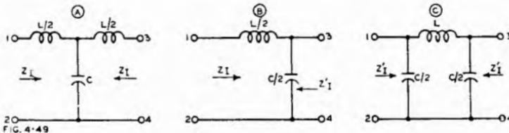
Fig. 4.49. Three varieties of low-pass constant  $k$  filters: (A) T section (B) Half section (C) II section.
