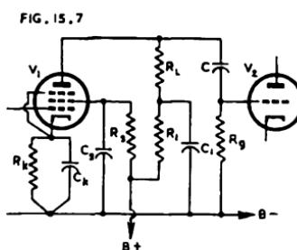
Fig. 15.7. Bass boosting—plate series compensation.
