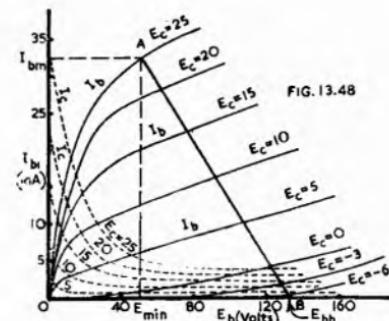
dissipation is the only limiting factor, six times more output may be obtained from the same valves in Class B than in Class A.
