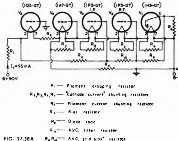
FIG. 27.38A      R<sub>1</sub> — Filament dropping resistor
