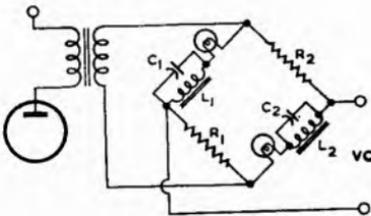
Fig. 16.7. Bridge type of volume expander using lamps which provides bass boosting at low levels.
