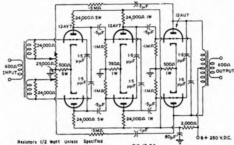
*Fig. 18.7B. Three-stage balanced cross-neutralized pre-amplifier using two 12AY7 valves and 12AU7 (Ref. B17).*
