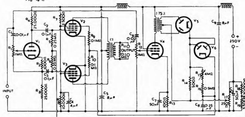
Fig. 16.11. Volume expander incorporating push-pull suppressor-controlled pentodes (Ref. 7).  $V_1 = MH_4$ ,  $V_2 = V_3 = AC/SP1$ ,  $V_4 = KT41$ ,  $V_5 = V_6 = AZ3$ .
