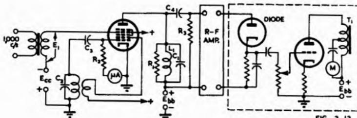
FIG. 3.13. Side-band method of measuring conversion transconductance.
