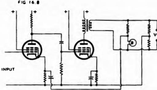
Fig. 16.8. Lamp-operated negative feedback volume expander (Ref. 22).
