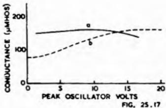
Fig. 25.17. Signal-grid (grid No. 1) conductance of typical mixer designed for outer-grid injection of oscillator. Frequency, 31.5 megacycles, signal-grid bias,  $E_{c_1} = -3$  volts. Curve *a* corresponds to fixed No. 3 grid bias,  $E_{c_3} = -8$  volts. Curve *b* corresponds to bias through a 50 000-ohm grid leak.
