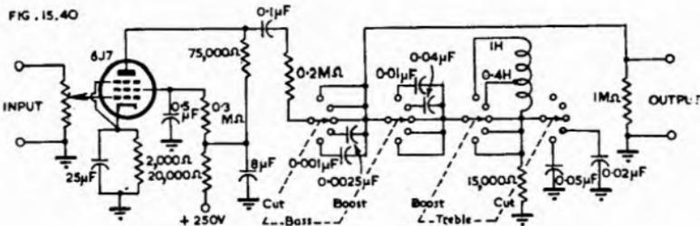
Fig. 15.40. Universal step-type tone control using inductors.
