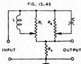
Fig. 15.45. Duo-control circuit incorporating  $L$  and  $C$  (Ref. 26).
