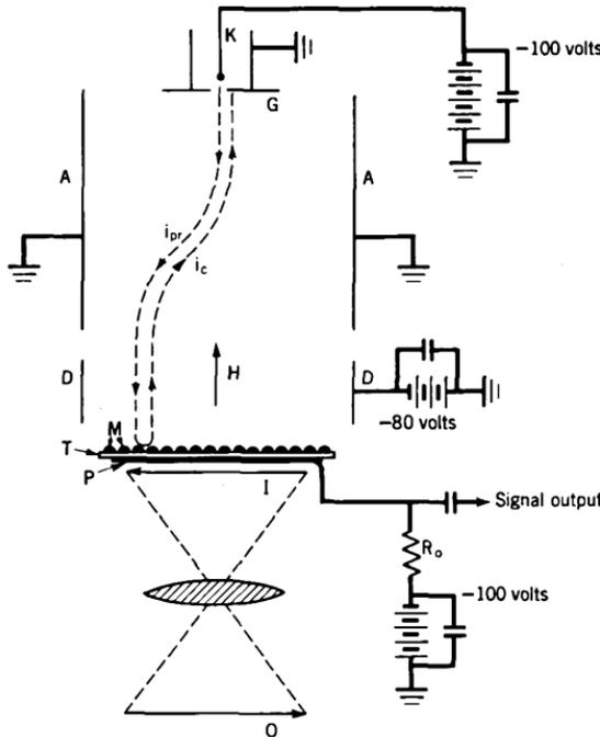
Fig. 29. Television-camera storage tube (Orthicon).
