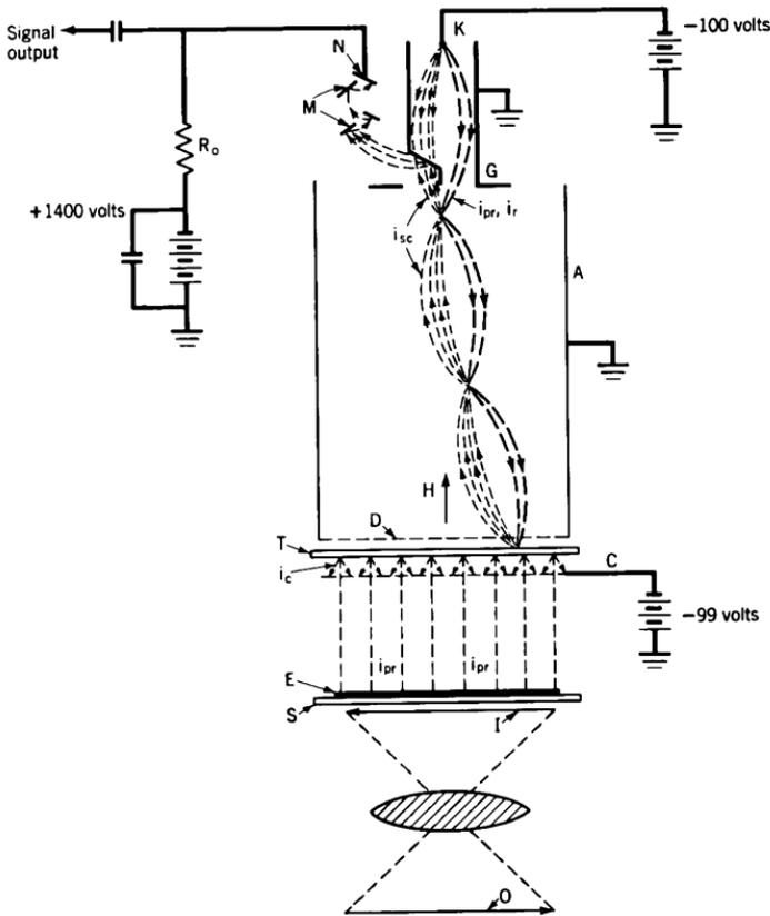
Fig. 33. Television-camera storage tube (Image Isocon).
