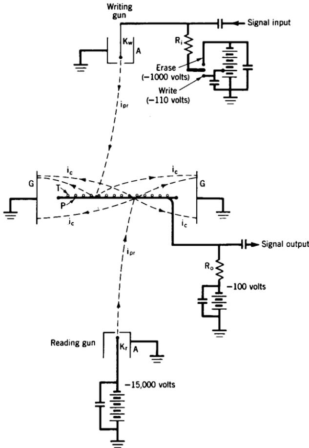
Fig. 17. Signal-converter storage tube (Knoll and Randmer).
