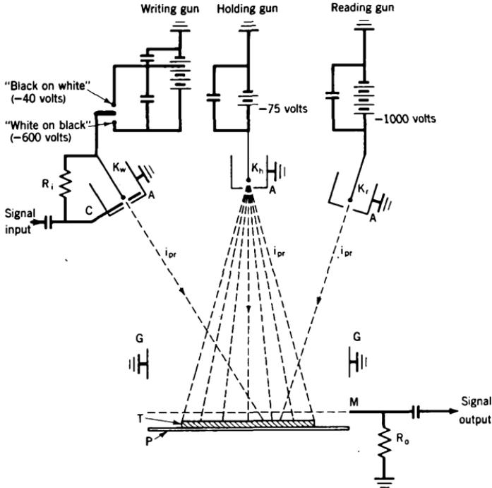
Fig. 16. Signal-converter storage tube (Memory Tube).
