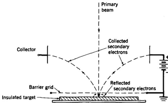
Fig. 8b. Barrier grid for reducing electron redistribution.
