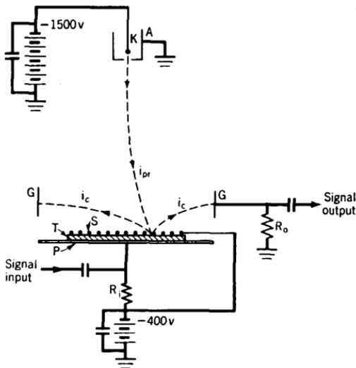
Fig. 18. Signal-converter storage tube (Radechon).
