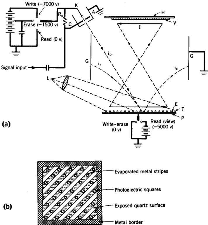
**Fig. 19.** Photoelectric viewing storage tube (Krawinkel). (a), tube with metallic viewing-cathode support and mosaic storage elements on it. (b), homogeneous insulating plate for the viewing-cathode support.
