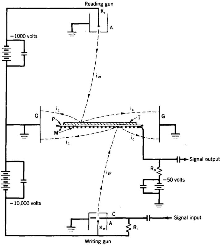
Fig. 15. Signal-converter storage tube (Graphechon).
