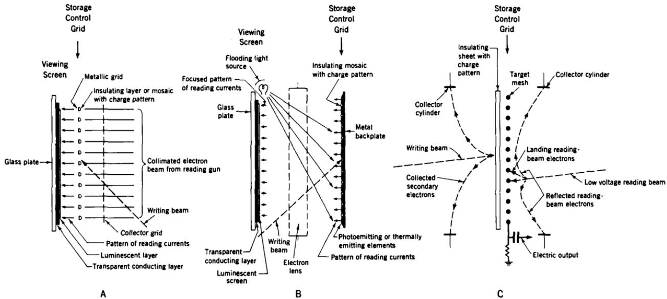
Fig. 12. Grid-control reading systems.
