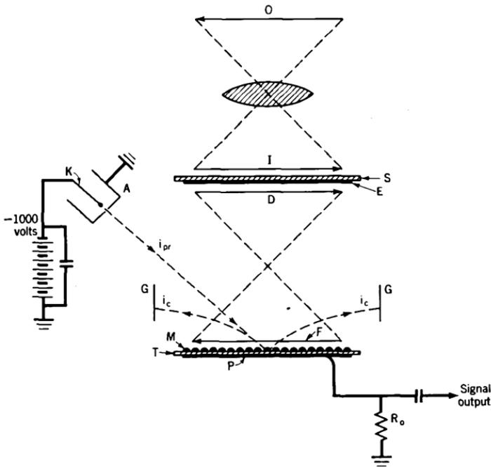
Fig. 31. Television-camera storage tube (Image Iconoscope).
