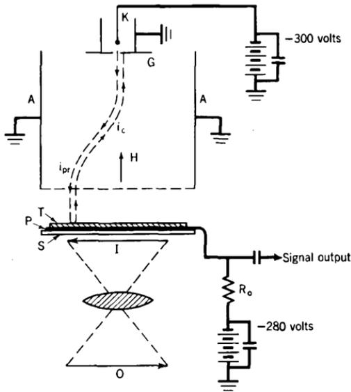
Fig. 30. Television-camera storage tube (Vidicon).
