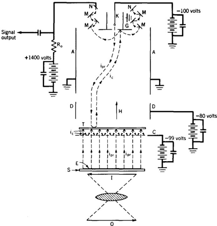
Fig. 32. Television-camera storage tube (Image Orthicon).
