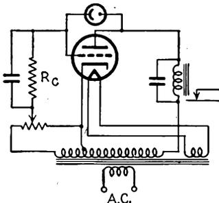
FIG. 13-14.—A-c-operated forward phototube circuit.
