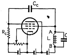
FIG. 10-42.—Transitron oscillator.
