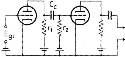
Fig. 6-9.—Two-stage resistance-capacitance-coupled amplifier.
