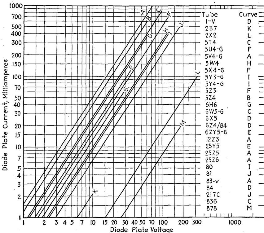
FIG. 14-8.—Average static plate characteristics of high-vacuum power rectifier tubes.
