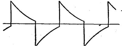
FIG. 10-22.—Typical wave form of grid-to-grid voltage in a symmetrical multivibrator.
