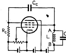
FIG. 10-42.—Transitron oscillator.
