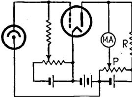
FIG. 13-17.—Phototube circuit for the measurement of illumination.
