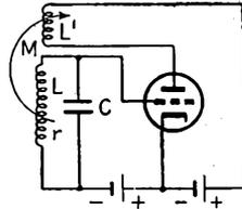
FIG. 10-49.—Tuned-grid oscillator.
