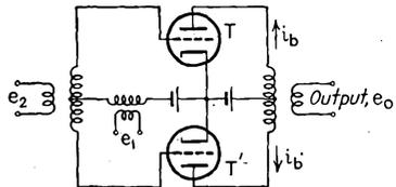
FIG. 9-5.—Balanced modulator.
