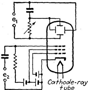
FIG. 15-64.—Circuit for the oscillographic comparison of frequency.
