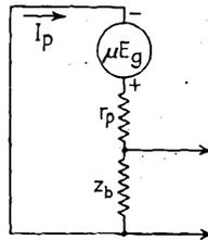
FIG. 6-19b.—Equivalent plate circuit of the cathode-follower amplifier.
