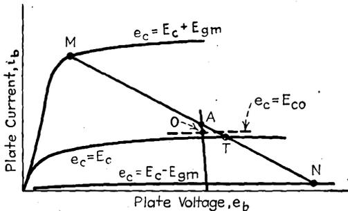
FIG. 4-19.—Plate diagram for self-biased circuit.  $r_b > R_b$ .
