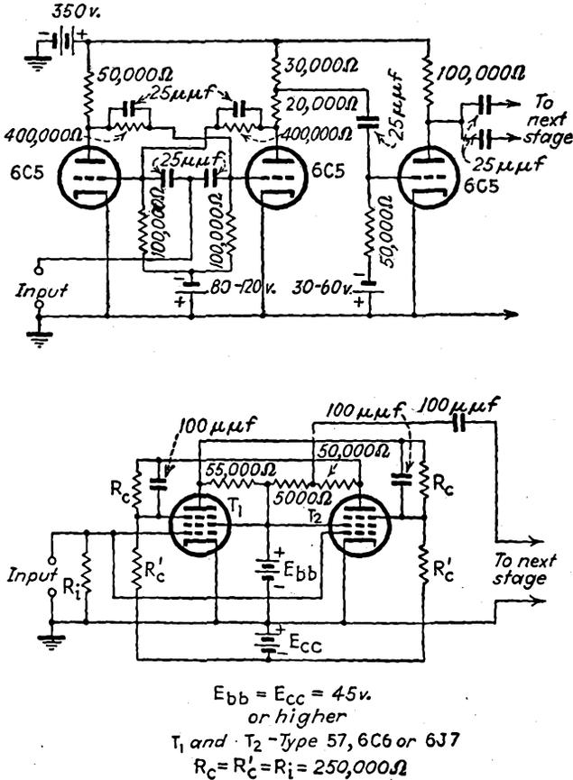
Fig. 15-38.—Counting circuits based upon high-vacuum-tube trigger circuits.
