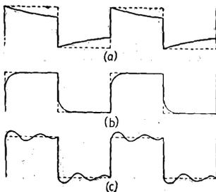
FIG. 15-95.—Distortion of rectangular wave caused by: (a) poor low-frequency response; (b) poor high-frequency response; (c) transient oscillations in coupling transformers.
