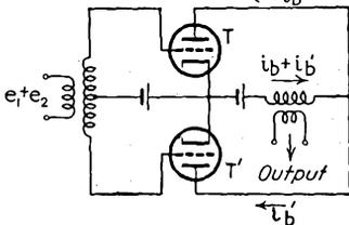
FIG. 9-6.—Balanced modulator.
