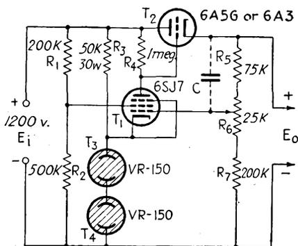
FIG. 14-22.—Two-stage degenerative voltage stabilizer.
