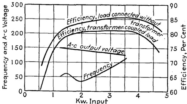
FIG. 12-62.—Performance curves for a parallel inverter.
