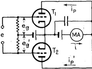
FIG. 15-2.—Basic circuit of balanced plate-detection vacuum-tube voltmeter.
