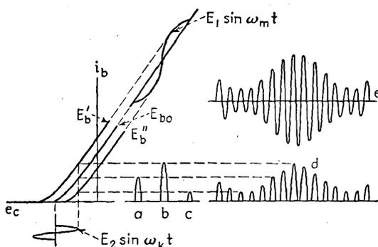
Fig. 9-14.—Graphical explanation of linear plate modulation.
