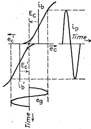
FIG. 5-20.—Push-pull Class B2 operation.
