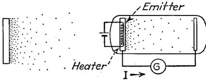
FIG. 2-2.—Distribution of electrons near an emitting surface.
