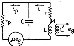
FIG. 10-50.—Equivalent plate circuit for the tuned-plate oscillator.
