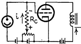
FIG. 13-11.—Forward d-c phototube circuit.
