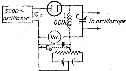
FIG. 9-51.—Circuit for determining the modulation characteristic of a diode modulator.
