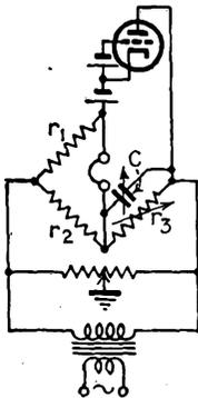
FIG. 15-75.—Bridge for the measurement of plate resistance.
