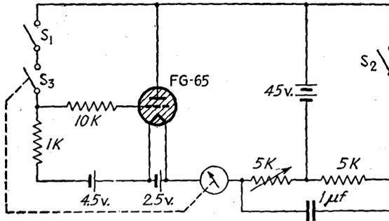
FIG. 15-36.—Circuit for the measurement of time intervals.
