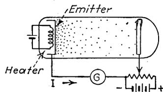
FIG. 2-2.—Distribution of electrons near an emitting surface.
