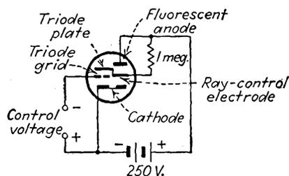
FIG. 15-71.—Electron-ray-tube circuit.
