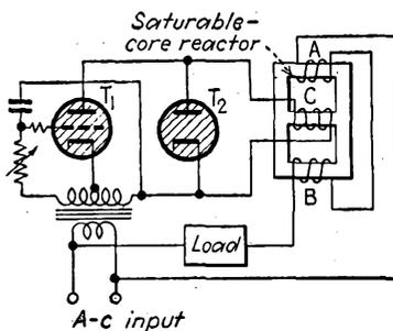
FIG. 12-86.—Phase-control circuit incorporating a saturable reactor.
