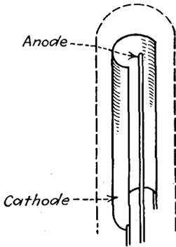
FIG. 13-3.—Electrode structure of one type of phototube.
