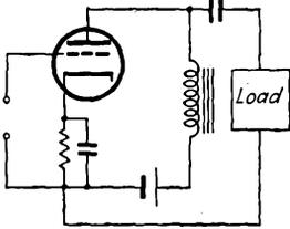
FIG. 5-17.—Choke-condenser-coupled load.
