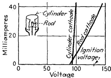
FIG. 11-3.—Current-voltage characteristics for the type 874 glow tube.
