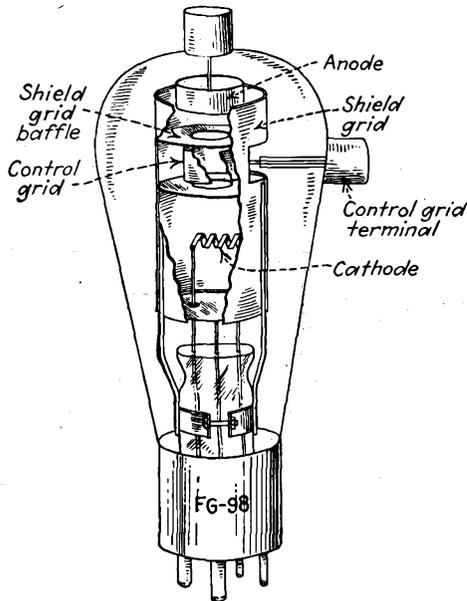
FIG. 12-30.—Electrode structure of the type FG-98 shield-grid thyratron.
