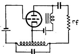
FIG. 10-71.—Resistance-stabilized Hartley oscillator.
