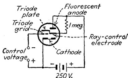
FIG. 15-71.—Electron-ray-tube circuit.
