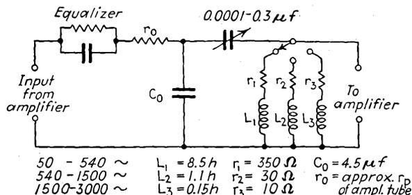
FIG. 15-89.—Amplifier-coupling filter for tuned-filter harmonic analyzer.
