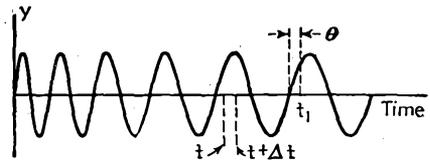
FIG. 9-39.—Frequency-modulated wave.
