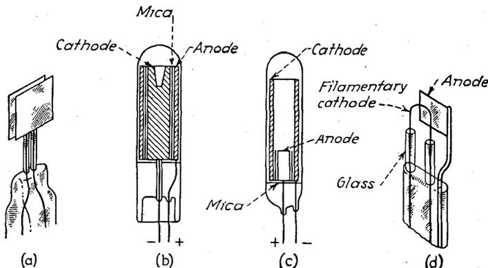
FIG. 12-2.—Tubes for the production of modulated light.
