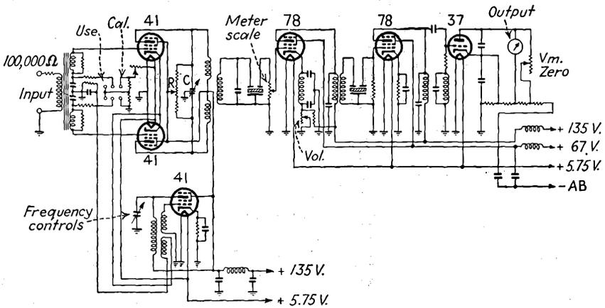
FIG. 15-91.—Heterodyne wave analyzer using a quartz-crystal filter. (Courtesy of General Radio Co.)
