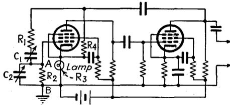
FIG. 10-63.—Practical form of the oscillator of Fig. 10-62.
