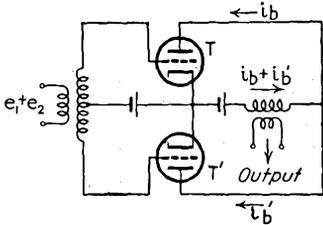
FIG. 9-6.—Balanced modulator.
