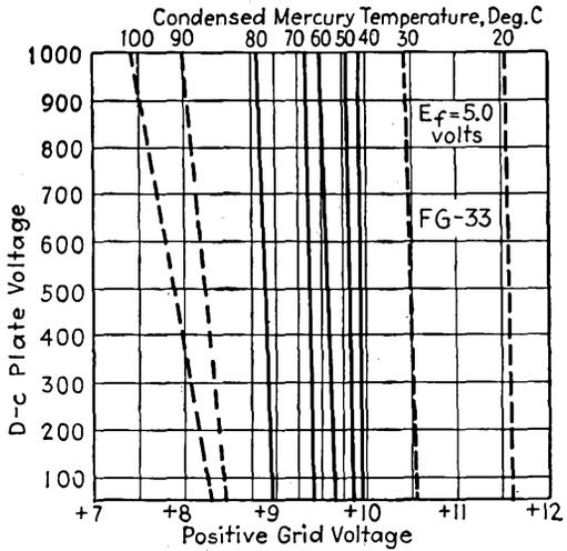
FIG. 12-29.—Grid-control characteristics of the type FG-33 thyatron.
