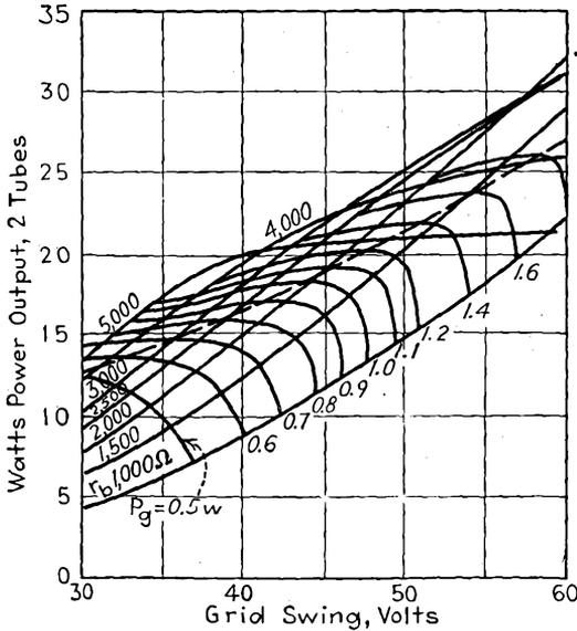
FIG. 8-18.—Power output as a function of grid swing for various values of load resistance  $r_L$  and for various values of peak grid power  $P_g$ .
