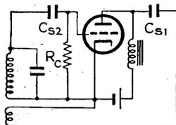
FIG. 10-75.—Practical form of doubly stabilized tuned-grid oscillator.
