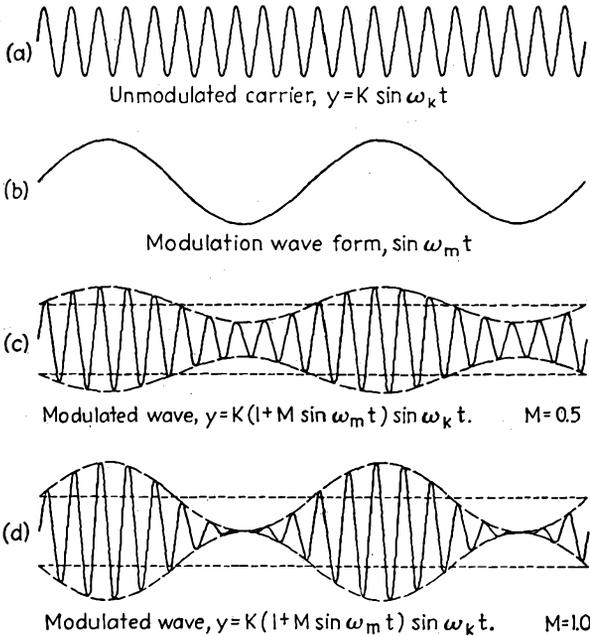
FIG. 9-1.—Amplitude modulation.
