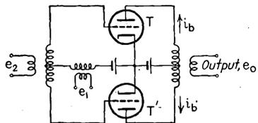
FIG. 9-5.—Balanced modulator.
