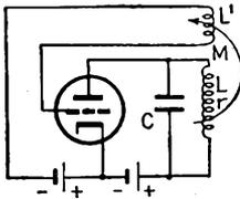
FIG. 10-48.—Tuned-plate oscillator.
