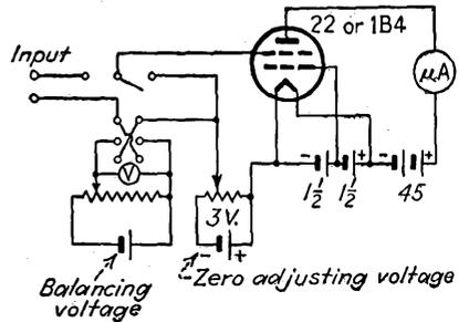
FIG. 15-20.—Slide-back voltmeter using tetrode with space-charge connection.
