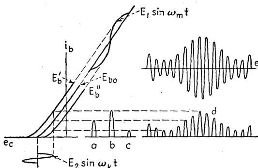
Fig. 9-14.—Graphical explanation of linear plate modulation.
