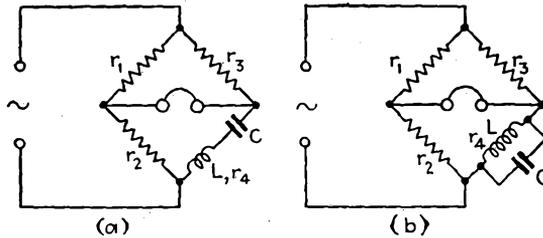
FIG. 15-41.—Belzils resonance bridges: (a) series; (b) parallel.
