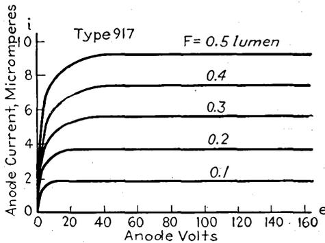
FIG. 13-4.—Current-voltage characteristics for the type 917 vacuum phototube.
