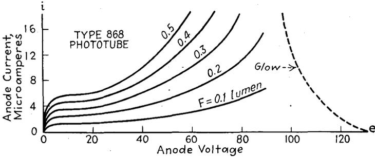
FIG. 13-7.—Current-voltage characteristics for the type 868 gas phototube.
