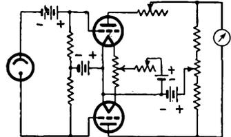
FIG. 13-18.—Balanced circuit for the measurement of illumination.
