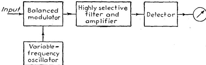
FIG. 15-90.—Block diagram of a heterodyne harmonic analyzer.
