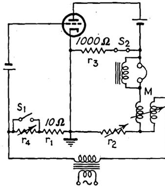
FIG. 15-76.—Bridge for the measurement of plate resistance.
