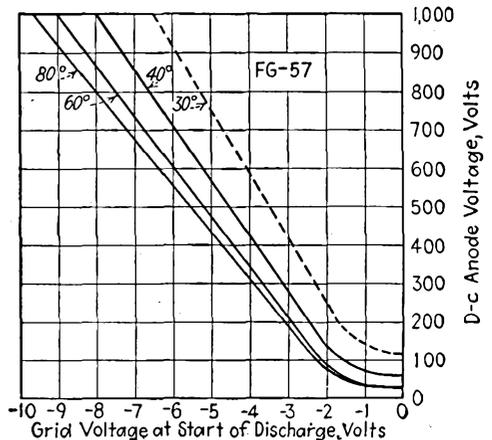
FIG. 12-27.—Grid-control characteristics of the type FG-57 thyatron.
