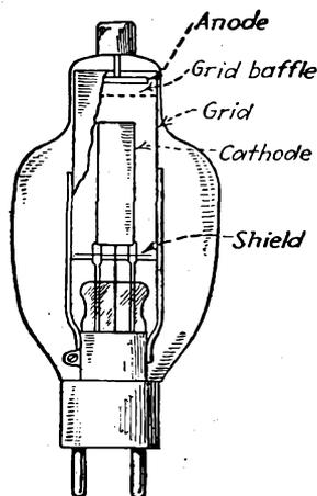
FIG. 12-24.—Electrode structure of the type FG-67 thyatron.
