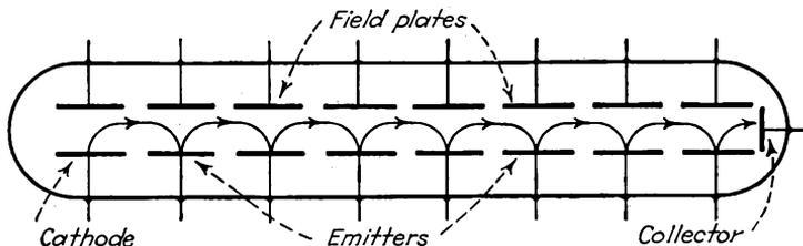
FIG. 13-25.—Arrangement of electrodes in secondary-emission current multiplier using crossed magnetic and electric fields.
