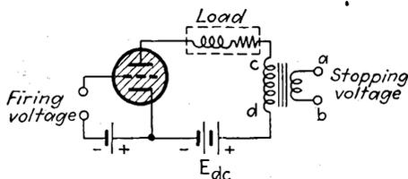
FIG. 12-45.—Practical form of the counter-e.m.f. control circuit.
