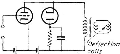
FIG. 15-55.—Amplifier for producing linear electromagnetic sweep.
