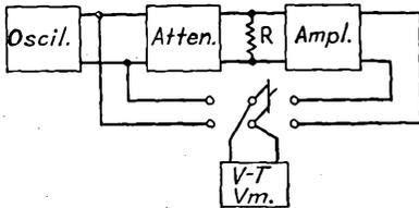
FIG. 15-93.—Circuit for the measurement of voltage amplification.
