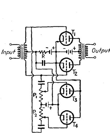
FIG. 8-22.—Circuit for preventing distortion resulting from C-supply impedance.
