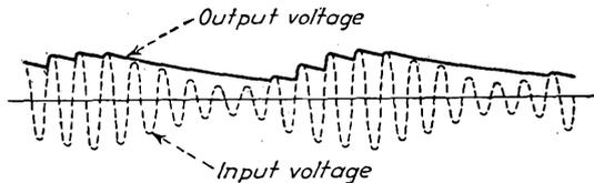
FIG. 9-29.—Nonlinear distortion in a diode detector resulting from improper choice of circuit values.
