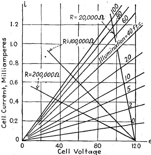
FIG. 13-29.—Typical current-voltage diagram for a selenium cell.
