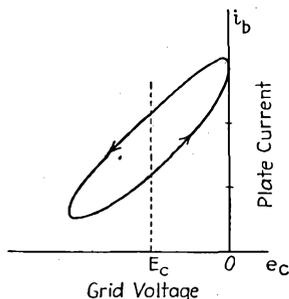
FIG. 3-25.—Typical dynamic transfer characteristic for inductive load.
