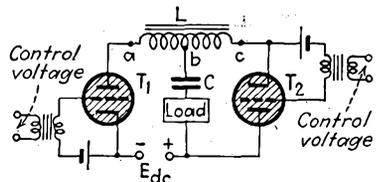
Fig. 12-37.—Series control circuit with center-tapped commutating inductance.
