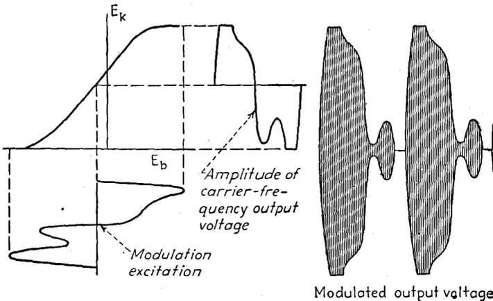
FIG. 9-13.—Modulation distortion resulting from excessive modulation excitation voltage. by detection. Figure 9-12 shows the manner in which incorrect choice of biasing voltage  $E_{b0}$  results in distortion of the modulated wave, and Fig. 9-13 shows how the modulated wave is distorted by excessive amplitude of modulation excitation voltage.
