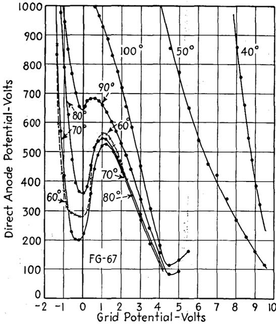
FIG. 12-25.—Grid-control characteristics of the type FG-67 thyatron.
