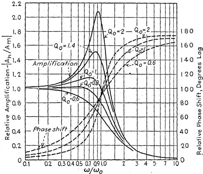
FIG. 6-31.—Generic curves of relative amplification and relative phase shift for transformer-coupled audio-frequency amplifiers at high frequency.  $\omega_0 = \frac{1}{\sqrt{L_e C_e}}$ ;  $Q_0 = \frac{\omega_0 L_e}{r_e}$ .
