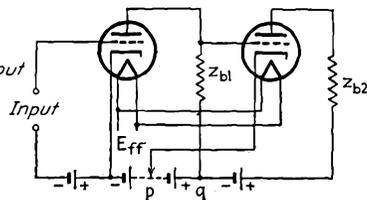
FIG. 5-4.—Direct-coupled amplifier.
