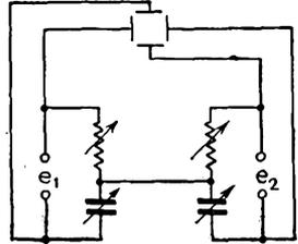
FIG. 15-65.—Circuit for the oscillographic comparison of frequency.
