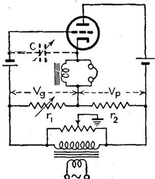
FIG. 15-73.—Bridge for the measurement of amplification factor.
