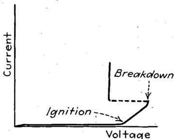
FIG. 11-5.—Current-voltage curve for discharge between needle points.
