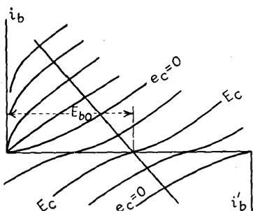
FIG. 8-2.—Composite plate diagram for triodes biased to cutoff.
