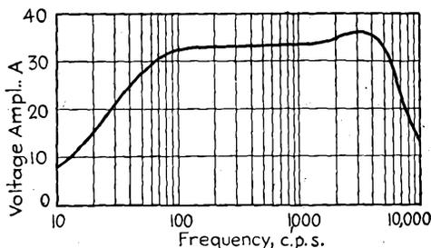
FIG. 6-27.—Frequency-response curve of a transformer-coupled audio-frequency amplifier.
