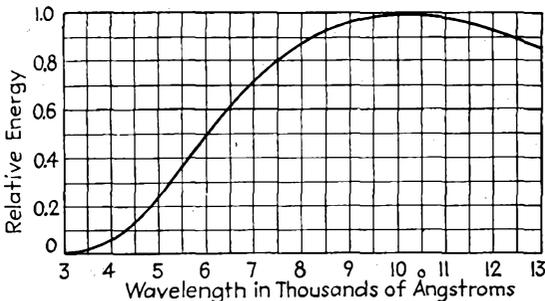
FIG. 13-6.—Relative energy distribution for radiation from a tungsten filament at a color temperature of 2870°K. (From data by W. E. Forsythe and E. Q. Adams, *Denison University Bulletin, J. of the Scientific Laboratories*, **32**, 70 (1937).)
