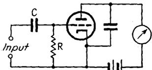
FIG. 15-15.—Grid-detection voltmeter.
