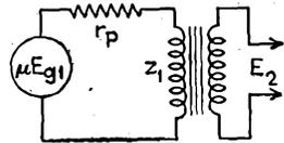
FIG. 6-25.—Simplified equivalent plate circuit of a transformer-coupled audio-frequency stage at low and mid-band frequencies.
