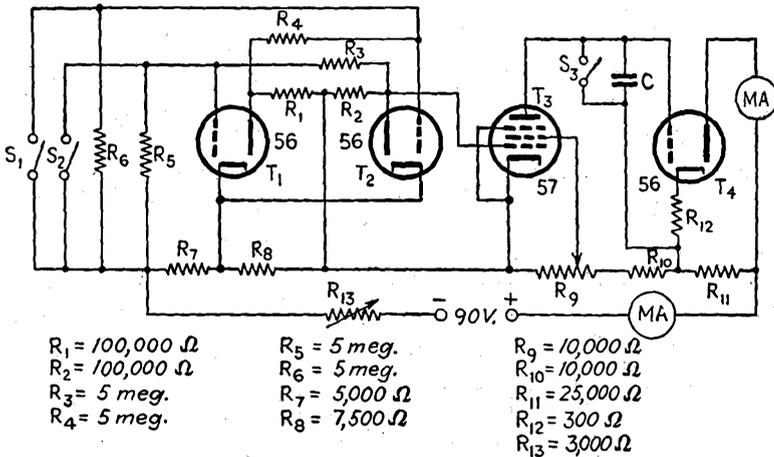
FIG. 15-35.—Circuit for the measurement of time intervals.
