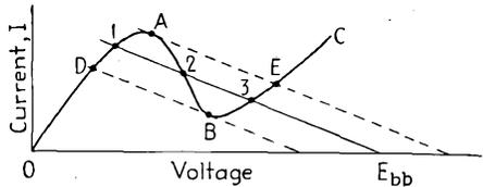
FIG. 10-2.—Current-voltage diagram for the circuit of Fig. 10-1.
