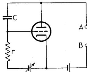
FIG. 6-48.—Reactance-tube circuit.
