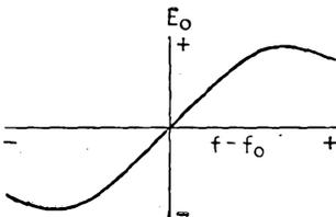
FIG. 9-49.—Detection characteristic for the discriminator of Fig. 9-45.
