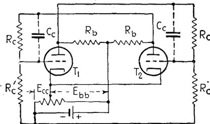
FIG. 10-7.—Practical form of the Eccles-Jordan trigger circuit.
