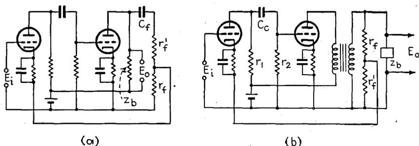
FIG. 6-41.—Two-stage single-sided inverse-feedback amplifiers.
