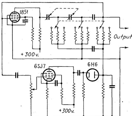
FIG. 10-66.—Practical form of the oscillator of Fig. 10-65.
