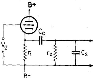
FIG. 6-21.—Resistance-capacitance coupled cathode-follower amplifier stage.
