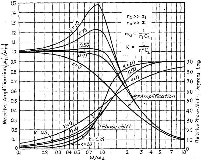
FIG. 6-18.—Generic curves of high-frequency relative amplification and relative phase shift at five values of  $K = \frac{L}{r_1^2 C_2}$  for an inductance-compensated resistance-capacitance-coupled amplifier.
