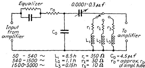
FIG. 15-89.—Amplifier-coupling filter for tuned-filter harmonic analyzer.
