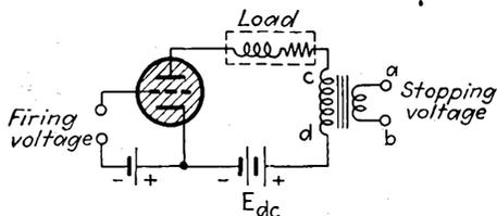
FIG. 12-45.—Practical form of the counter-e.m.f. control circuit.
