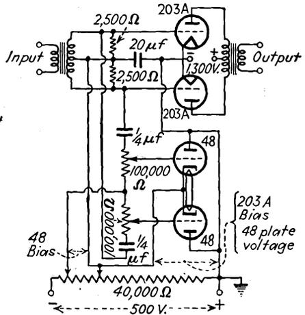
FIG. 8-23.—Practical form of the circuit of Fig. 8-22.
