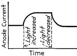
FIG. 13-9.—Lag in response of a gas phototube.
