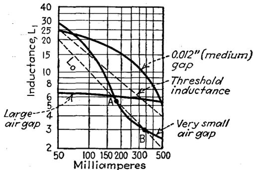
FIG. 14-18.—Variation of choke inductance with direct current.
