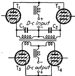
FIG. 12-68.—D-c transformer based upon the parallel inverter.
