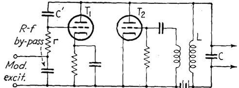
FIG. 9-43.—Frequency modulator.
