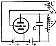
FIG. 10-48.—Tuned-plate oscillator.
