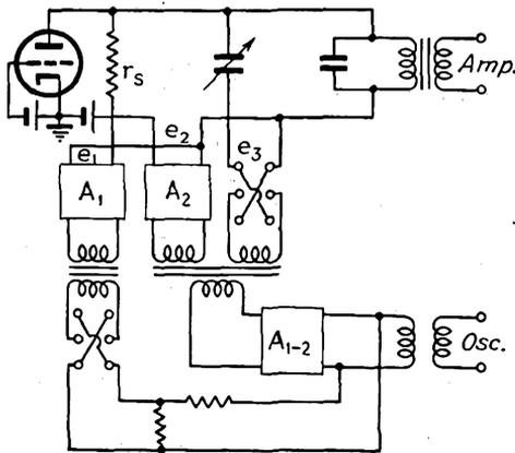
FIG. 15-85.—Bridge for the measurement of electrode resistance.
