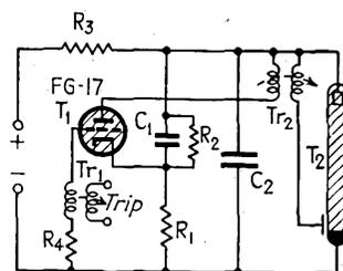
Figure 12-101 shows a typical circuit in which a thyatron controls the tripping impulse applied to the external grid of a mercury pool arc tube.<sup>1</sup> The large condenser  $C_2$  is charged through the resistance  $R_3$ ,
