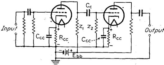
FIG. 5-7.—Impedance-capacitance-coupled amplifier with self-biasing resistors  $R_{cc}$ .
