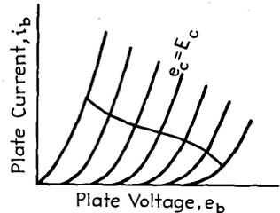
FIG. 8-24.—Curvature of path of operation of driver resulting from variation of effective load.
