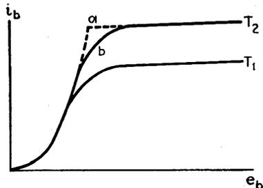
FIG. 2-11.—Curves of anode current  $i_b$  *vs.* anode voltage  $e_b$  at two values of emitter temperature.
