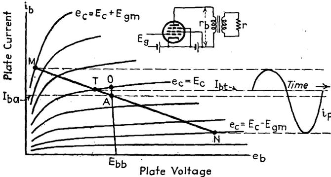
FIG. 4-18.—Plate diagram for a pentode with nonreactive load.  $r_b > R_b$ . Conditions of operation such that average plate current decreases with excitation.
