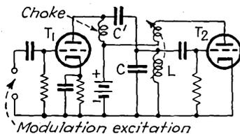
FIG. 9-42.—Frequency modulator.
