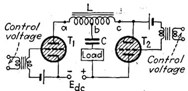
Fig. 12-37.—Series control circuit with center-tapped commutating inductance.
