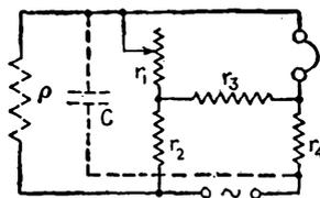
FIG. 15-82.—Bridge for the measurement of negative resistance.
