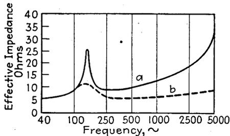
FIG. 7-11.—Variation of effective impedance of a loud-speaker, (*a*) without shunting network, and (*b*) with resistance-capacitance shunt.
