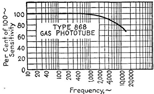
FIG. 13-10.—Dynamic response curve for type 868 gas phototube.
