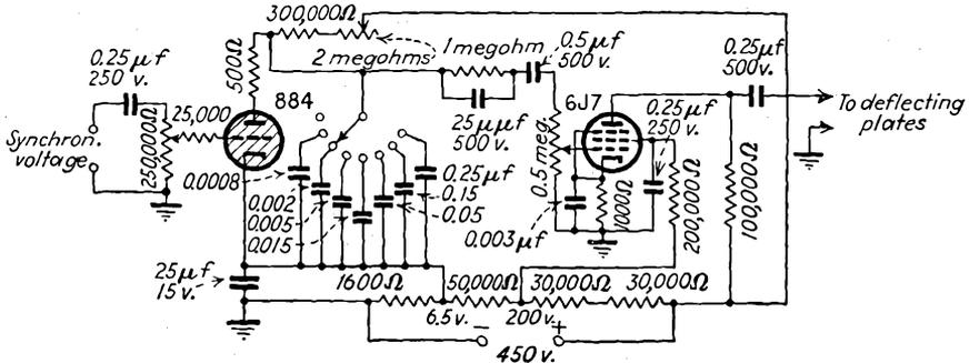
FIG. 15-50.—Sweep oscillator and amplifier.
