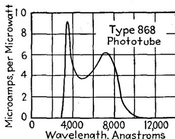
FIG. 13-2.—Current-wave-length characteristic for the type 868 phototube.
