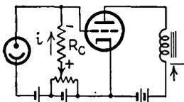
FIG. 13-11.—Forward d-c phototube circuit.
