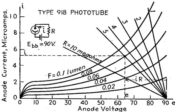
FIG. 13-22.—Anode diagram for the type 918 gas phototube.
