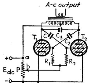
FIG. 12-54.—Self-excited parallel inverter.      FIG. 12-55.—Self-excited parallel inverter.
