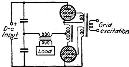
FIG. 12-59.—Separately excited series inverter using two condensers.
