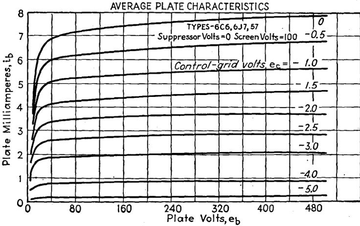
FIG. 3-13.—Plate characteristics of a typical voltage pentode.
