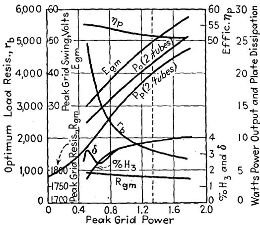
Fig. 8-20.—Optimum power output, optimum load resistance, peak grid swing, plate dissipation, percentage  $H_3$ , distortion factor, and peak grid resistance as a function of peak grid power. Type 46 tube in zero-bias Class B operation.
