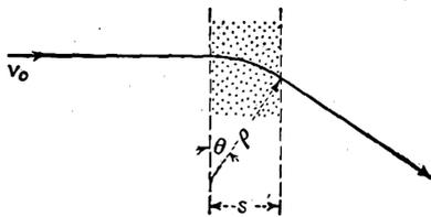
FIG. 1-3.—Deflection of electron beam by magnetic field.
