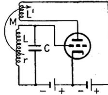
FIG. 10-49.—Tuned-grid oscillator.
