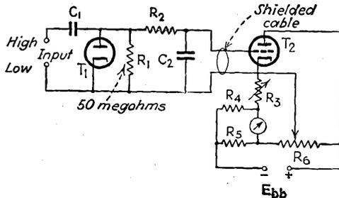
FIG. 15-14.—General Radio diode voltmeter.
