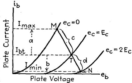
FIG. 7-2.—Triode plate diagram for Class A1 operation.
