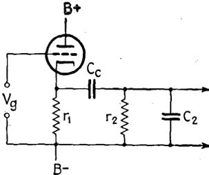
FIG. 6-21.—Resistance-capacitance coupled cathode-follower amplifier stage.
