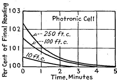
FIG. 13-35.—Curves showing fatigue in the Photronic cell.
