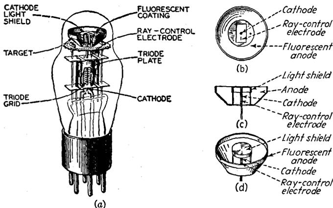
FIG. 15-70.—Structure of the type 6AB5 electron-ray tube.
