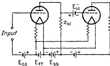
FIG. 5-3.—Direct-coupled amplifier.
