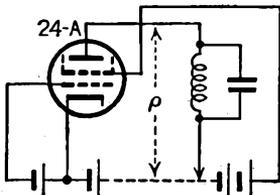
FIG. 10-40.—Dynatron-oscillator circuit.
