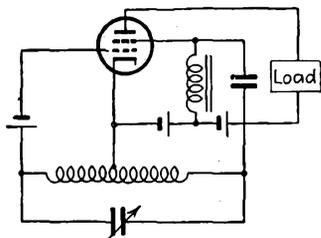
FIG. 10-69.—Hartley oscillator with electron-coupled load.
