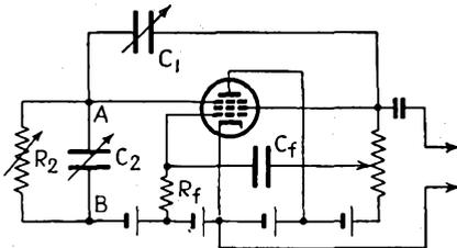
FIG. 10-64.—Single-tube version of the circuit of Fig. 10-62.
