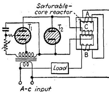
FIG. 12-86.—Phase-control circuit incorporating a saturable reactor.
