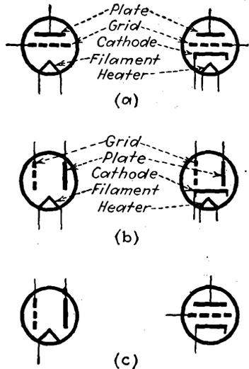
FIG. 3-2.—Symbols for filamentary and heater-type high-vacuum triodes.
