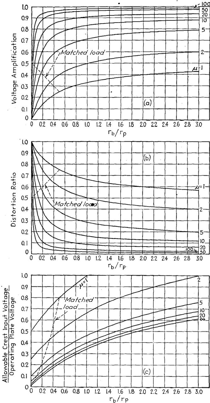
FIG. 6-20.—(a) Voltage amplification of a cathode-follower amplifier as a function of  $r_b/r_p$ . (b) Ratio of nonlinear distortion in a cathode-follower amplifier to that in a conventional amplifier using the same tube and load. (c) Ratio of allowable crest input voltage to operating plate voltage of a cathode-follower amplifier.
