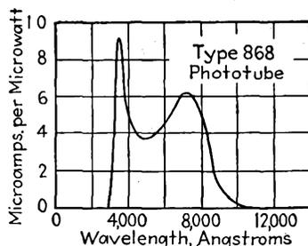
FIG. 13-2.—Current-wave-length characteristic for the type 868 phototube.
