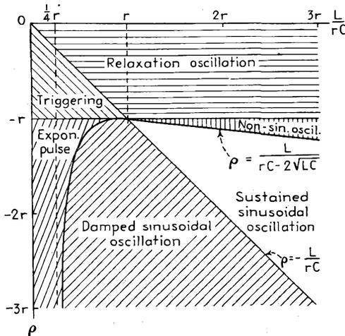
FIG. 10-37.—Theoretical diagram showing the relative ranges of circuit parameters of a negative-resistance oscillator throughout which the various types of operation should occur.
