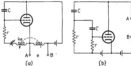
FIG. 6-49.—Variants of the reactance-tube circuit of Fig. 6-48.
