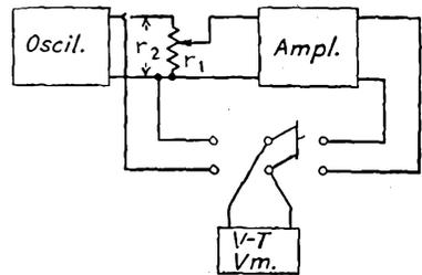
FIG. 15-94.—Circuit for the measurement of voltage amplification.
