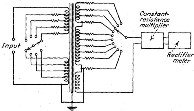
FIG. 15-96.—Circuit diagram of General Radio power-output meter.
