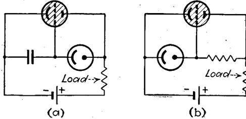
FIG. 12-19.—Two grid-glow tube circuits that incorporate phototubes.
