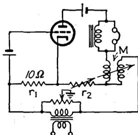
FIG. 15-74.—Bridge for the measurement of amplification factor.
