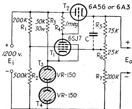
FIG. 14-22.—Two-stage degenerative voltage stabilizer.
