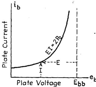
FIG. 8-14.—Class B power-output hyperbola.
