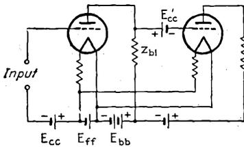
FIG. 5-3.—Direct-coupled amplifier.
