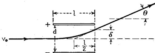
FIG. 1-2.—Deflection of electron beam by electric field.
