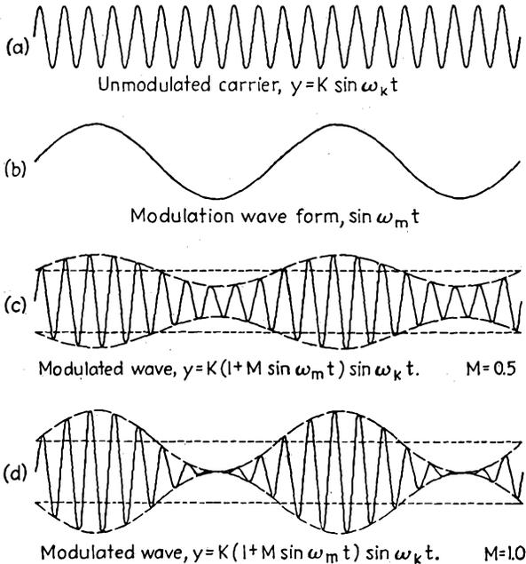
FIG. 9-1.—Amplitude modulation.
