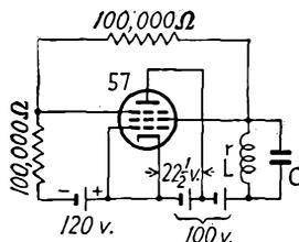
FIG. 10-82.—Negative resistance oscillator circuit for problem 10-3.
