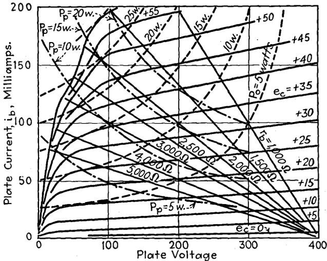
FIG. 8-16.—The use of hyperbolas in the approximate graphical determination of Class B power output and plate dissipation.
