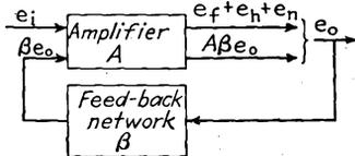
FIG. 6-38.—Schematic diagram of feedback amplifier.
