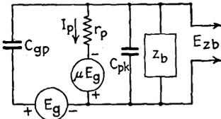
FIG. 6-2.—Equivalent circuit for the amplifier of Fig. 6-1.
