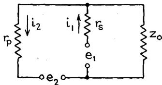
FIG. 15-86.—Equivalent circuit for the bridge of Fig. 15-85.
