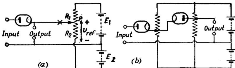
FIG. 189. AMPLITUDE SELECTION WITH SERIES DIODES
