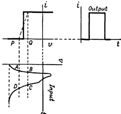
FIG. 186. PRINCIPLE OF SHAPING
