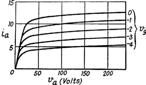
FIG. 18. CHARACTERISTICS OF PENTODE
