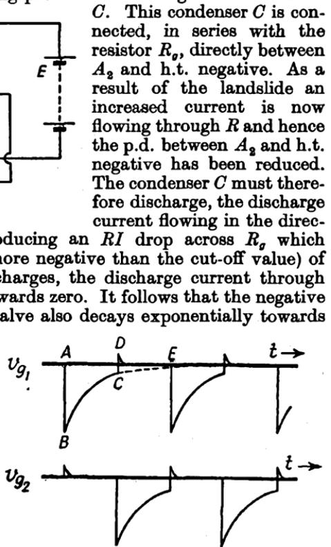
FIG. 114. MULTIVIBRATOR WAVEFORMS
