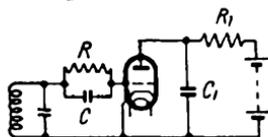
FIG. 134. CUMULATIVE-GRID DETECTOR
