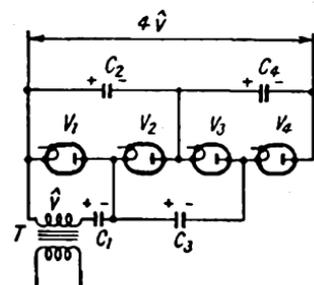
FIG. 146. VOLTAGE-QUADRUPLING RECTIFIER
