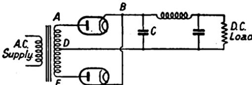
FIG. 141. FULL-WAVE RECTIFIER
