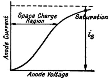
FIG. 7. CHARACTERISTICS OF DIODE
