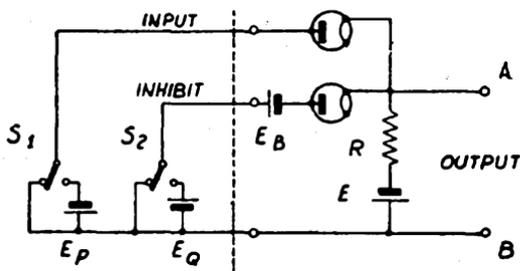
FIG. 229. INHIBITION GATE
