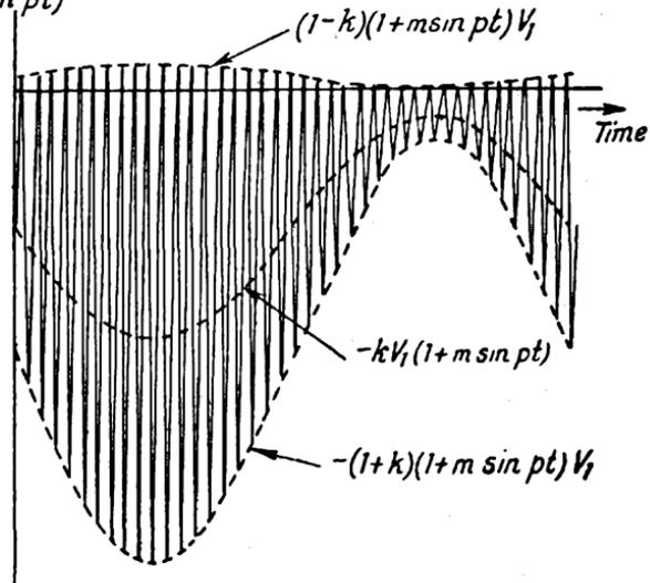
FIG. 135. RESULTANT GRID-VOLTAGE OF CUMULATIVE-GRID DETECTOR WITH MODULATED INPUT
