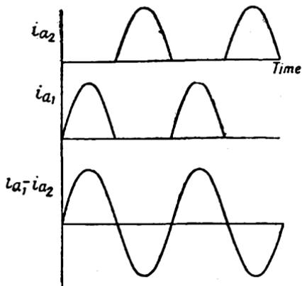
FIG. 86. CLASS B OPERATION—RELATION BETWEEN THE ANODE-CURRENTS OF THE TWO VALVES
