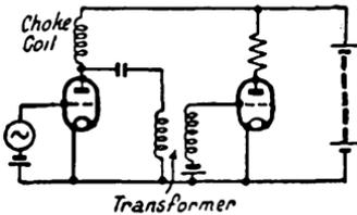
FIG. 36. PARALLEL-FED TRANSFORMER COUPLING
