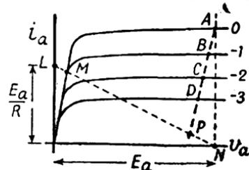
FIG. 220. LOAD-LINE DIAGRAM FOR MILLER SWEEP GENERATOR
