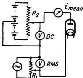
FIG. 130. CIRCUIT FOR MEASURING DYNAMIC-CHARACTERISTICS
