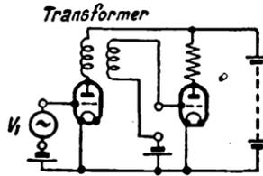
FIG. 34. INTERSTAGE TRANSFORMER COUPLING
