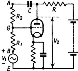
FIG. 76. SINGLE STAGE WITH SHUNT-CONNECTED NEGATIVE FEEDBACK
