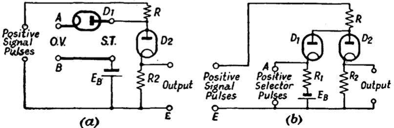
FIG. 199. TWO-DIODE TIME-SELECTION CIRCUIT
