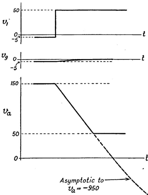
FIG. 217. WAVEFORMS OCCURRING IN FIG. 216
