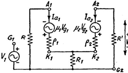
FIG. 51. CATHODE COUPLING
