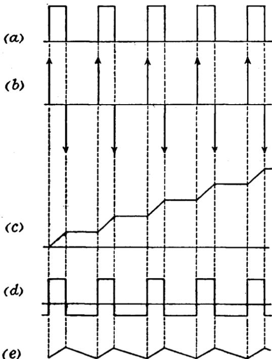
FIG. 174. DIFFERENTIATION AND INTEGRATION OF WAVEFORMS
