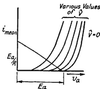
FIG. 136. RECTIFICATION CHARACTERISTICS OF ANODE-BEND DETECTOR
