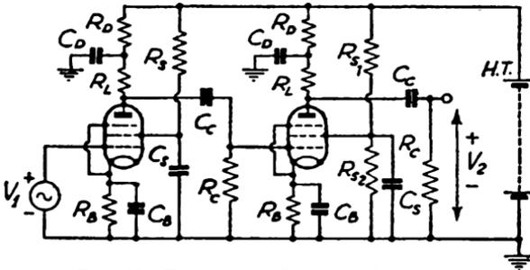
FIG. 48. TWO-STAGE PENTODE AMPLIFIER
