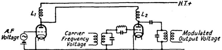
FIG. 162. CHOKE-COUPLED MODULATOR
