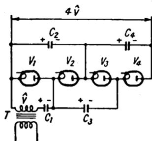
FIG. 146. VOLTAGE-QUADRUPLING RECTIFIER
