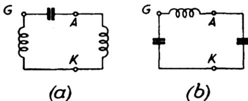
FIG. 98. CLOSED-CIRCUIT OSCILLATORS: THE TWO BASIC POSSIBILITIES
