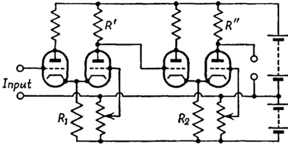
FIG. 52. LONG-TAILED PAIRS IN A D.C. AMPLIFIER
