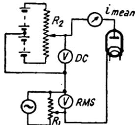
FIG. 130. CIRCUIT FOR MEASURING DYNAMIC-CHARACTERISTICS
