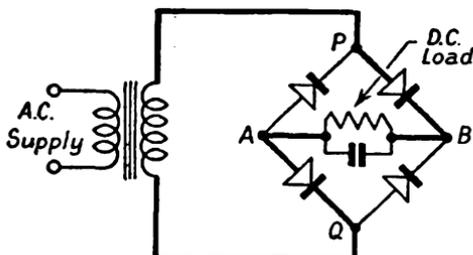
FIG. 144. BRIDGE RECTIFIER
