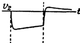
FIG. 207. COMBINED EFFECT OF ANODE-CATHODE CAPACITANCE AND  $R-C$  COUPLING
