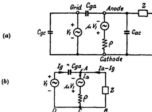
FIG. 59. EQUIVALENT CIRCUIT OF AMPLIFIER SHOWING INTER-ELECTRODE CAPACITANCES
