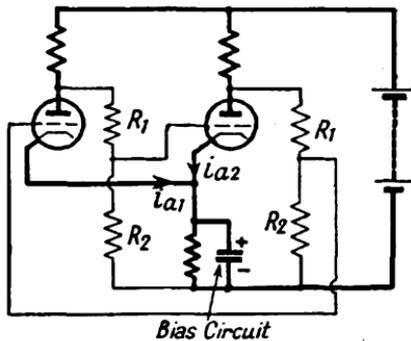
FIG. 117. RESISTANCE-COUPLED KIPP RELAY
