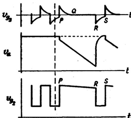
FIG. 225. WAVEFORMS IN SCREEN-COUPLED PHANTATRON OF FIG. 224 (b)
