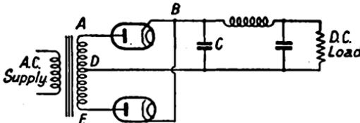
FIG. 141. FULL-WAVE RECTIFIER
