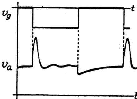
FIG. 185. WAVEFORMS IN RINGING CIRCUIT
