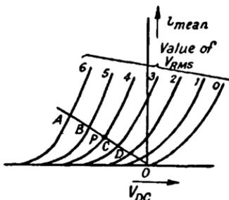
FIG. 129. DYNAMIC-CHARACTERISTICS OF DIODE
