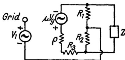
FIG. 74. EQUIVALENT CIRCUIT OF THE BRIDGE FEED-BACK
