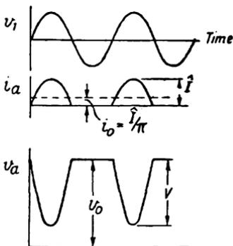
FIG. 87. CLASS B OPERATION—VOLTAGE AND CURRENT RELATIONS IN ONE OF THE VALVES
