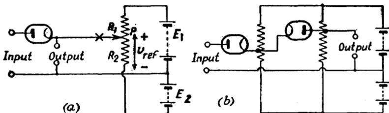
FIG. 189. AMPLITUDE SELECTION WITH SERIES DIODES
