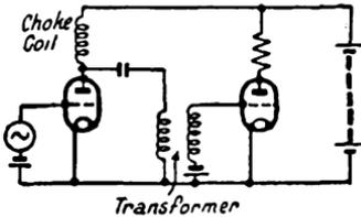
FIG. 36. PARALLEL-FED TRANSFORMER COUPLING
