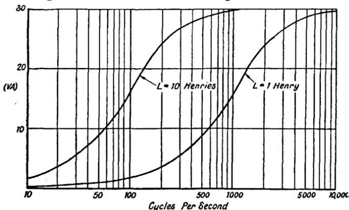
FIG. 32. FREQUENCY DISTORTION IN AMPLIFIER STAGE WITH CHOKE LOAD
