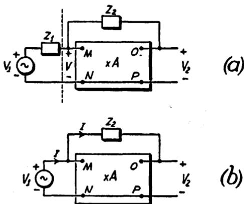
FIG. 75. SHUNT-CONNECTED FEEDBACK
