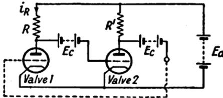
FIG. 116. SIMPLE BI-STABLE MULTIVIBRATOR
