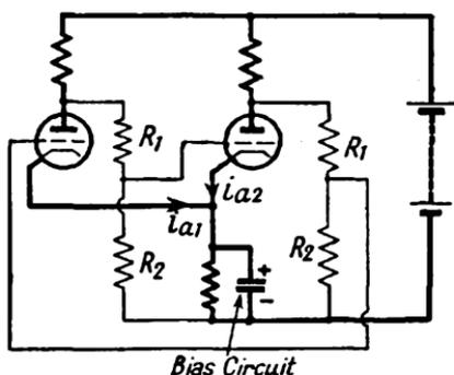
FIG. 117. RESISTANCE-COUPLED KIPP RELAY
