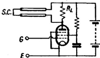
FIG. 182. CIRCUIT OF A DELAY-LINE PULSE GENERATOR
