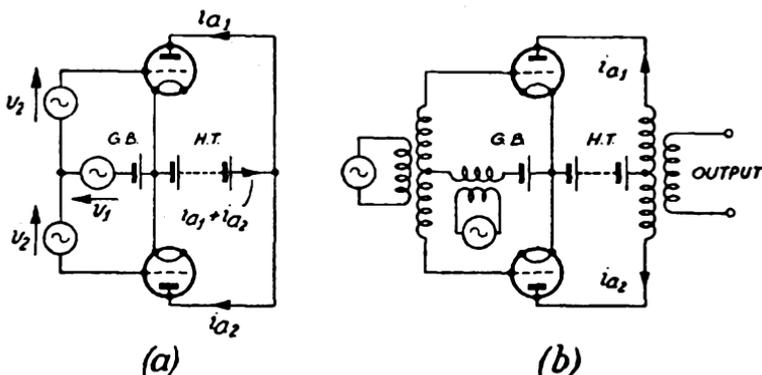
FIG. 154. BALANCED MODULATOR
