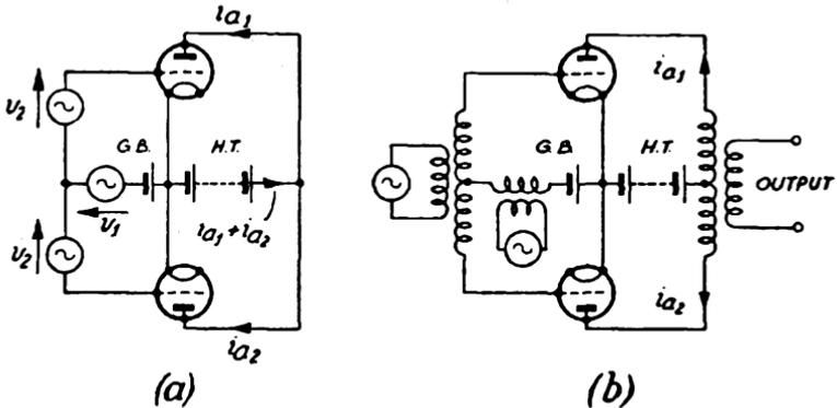
FIG. 154. BALANCED MODULATOR
