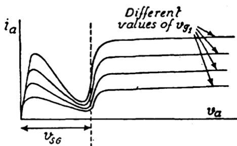
FIG. 17. CHARACTERISTICS OF SCREEN-GRID TETRODE
