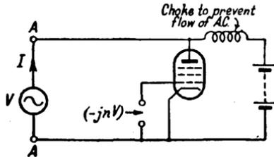
FIG. 163. PRINCIPLE OF REACTANCE VALVE
