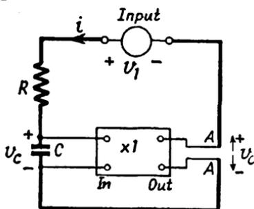
FIG. 221. PRINCIPLE OF THE BOOTSTRAP INTEGRATING CIRCUIT
