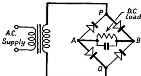
FIG. 144. BRIDGE RECTIFIER
