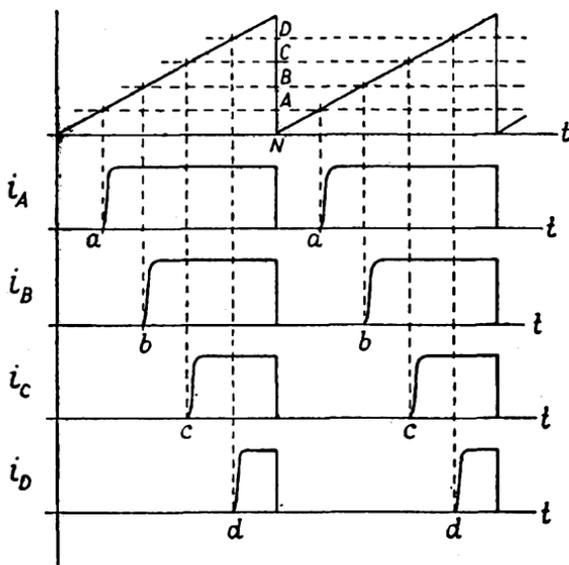
FIG. 172. AMPLITUDE COMPARISON
