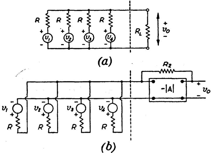
FIG. 79. ANALOGUE ADDING CIRCUIT
