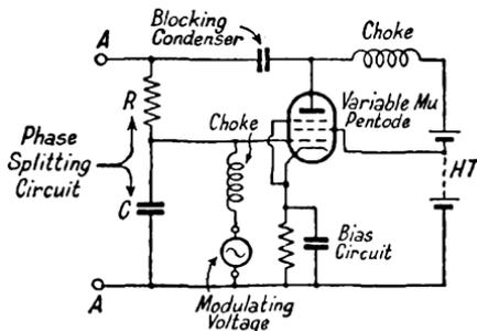
FIG. 165. REACTANCE-VALVE CIRCUIT
