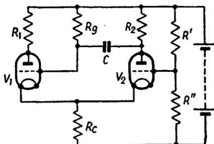
FIG. 119. CATHODE-COUPLED FLIP-FLOP
