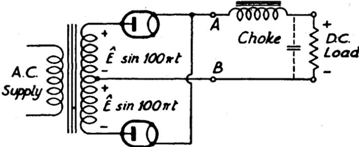
FIG. 142. SERIES-CHOKE FULL-WAVE RECTIFIER
