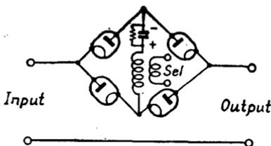
FIG. 201. BRIDGE-TYPE SWITCH CIRCUIT
