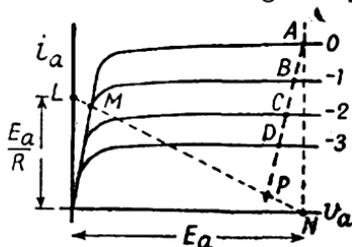
FIG. 220. LOAD-LINE DIAGRAM FOR MILLER SWEEP GENERATOR
