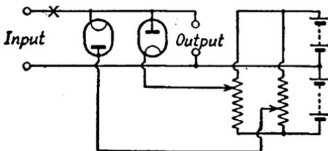
FIG. 190. AMPLITUDE SELECTION WITH SHUNT DIODES
