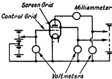
FIG. 16. CIRCUIT FOR MEASURING CHARACTERISTICS OF SCREEN-GRID VALVE
