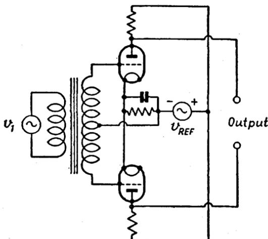
FIG. 149. PHASE-SENSITIVE DETECTOR
