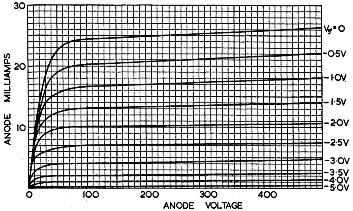
FIG. P-3. PENTODE CHARACTERISTICS, DRAWN FOR A SCREEN-GRID VOLTAGE OF 250 V
