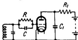
FIG. 134. CUMULATIVE-GRID DETECTOR
