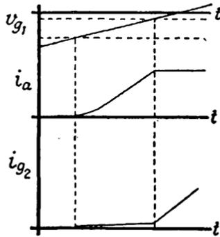
FIG. 193. VARIATION OF ANODE-CURRENT AND SCREEN CURRENT DURING BOTTOMING
