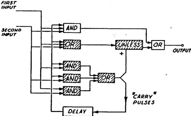
FIG. 230. BINARY ADDING CIRCUIT
