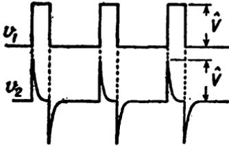
FIG. 176. QUASI-DIFFERENTIATION WITH THE CIRCUIT OF FIG. 175 (a)
