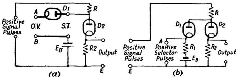
FIG. 199. TWO-DIODE TIME-SELECTION CIRCUIT
