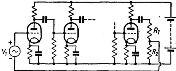
FIG. 64. NEGATIVE FEED-BACK AMPLIFIER WITH AN ODD NUMBER OF STAGES
