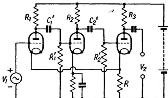
FIG. 68 NEGATIVE FEED-BACK AMPLIFIER WITH AN ODD NUMBER OF STAGES (Permitting earthing of one input terminal)
