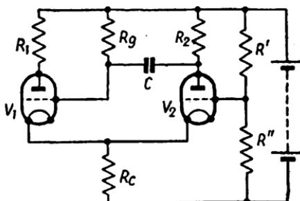
FIG. 119. CATHODE-COUPLED FLIP-FLOP
