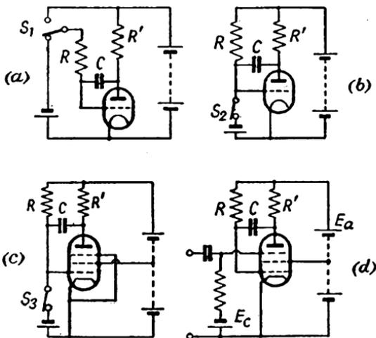
FIG. 218. INITIATING THE RUN-DOWN IN A MILLER SWEEP GENERATOR
