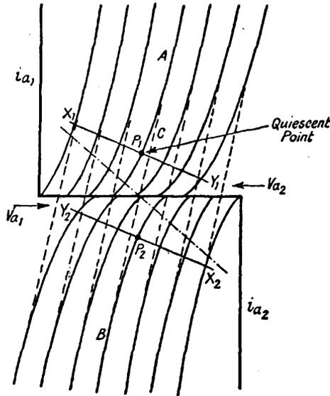
FIG. 43. COMPOSITE CHARACTERISTICS FOR PUSH-PULL CIRCUIT
