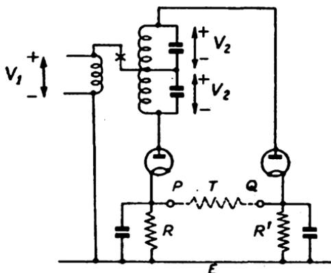
FIG. 151. PRINCIPLE OF THE FOSTER-SEELEY DISCRIMINATOR
