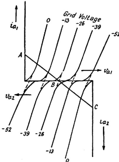
FIG. 90. COMPOSITE CHARACTERISTICS FOR CLASS B STAGE (Correct Bias Voltage)
