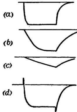
FIG. 204. PULSE-WAVEFORM DISTORTION CAUSED BY INTER-ELECTRODE CAPACITANCE
