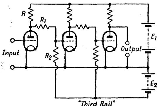
FIG. 39. RESISTANCE-COUPLED D.C. AMPLIFIER WITH "THIRD RAIL" H.T. SUPPLY
