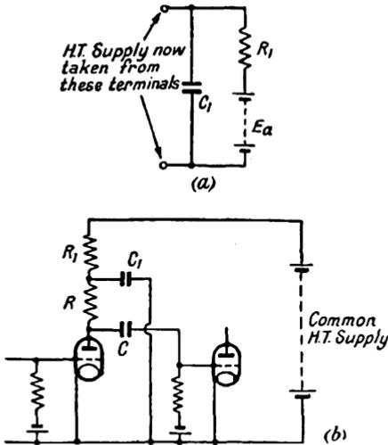
FIG. 44. ANODE-CIRCUIT DECOUPLING
