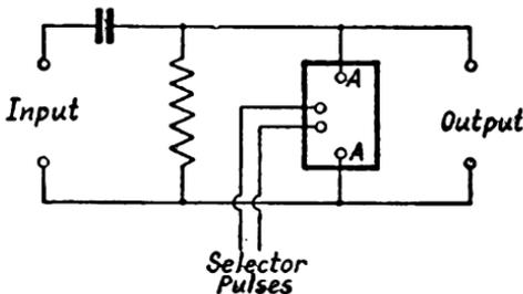
FIG. 209. LEVEL-SETTING CIRCUIT
