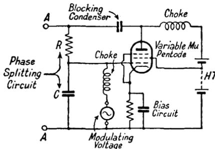
FIG. 165. REACTANCE-VALVE CIRCUIT
