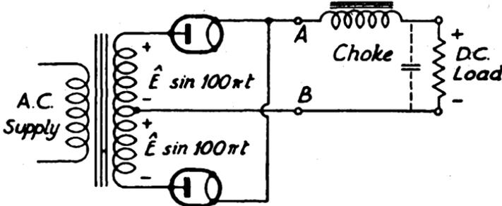
FIG. 142. SERIES-CHOKE FULL-WAVE RECTIFIER
