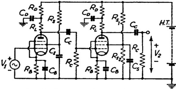
FIG. 48. TWO-STAGE PENTODE AMPLIFIER
