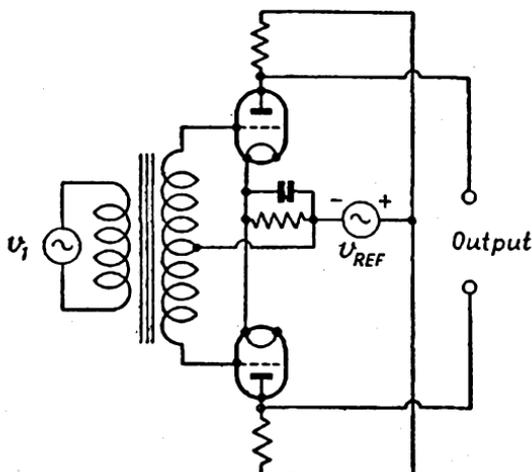
FIG. 149. PHASE-SENSITIVE DETECTOR
