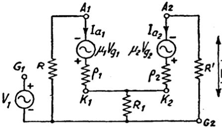
FIG. 51. CATHODE COUPLING
