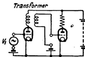
FIG. 34. INTERSTAGE TRANSFORMER COUPLING
