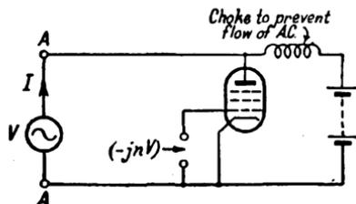
FIG. 163. PRINCIPLE OF REACTANCE VALVE
