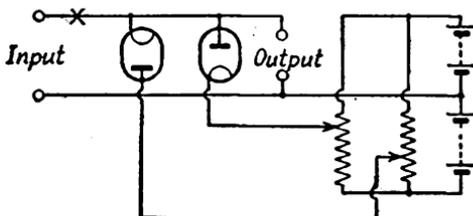
FIG. 190. AMPLITUDE SELECTION WITH SHUNT DIODES
