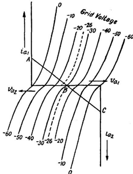
FIG. 88. COMPOSITE CHARACTERISTICS FOR CLASS B STAGE
