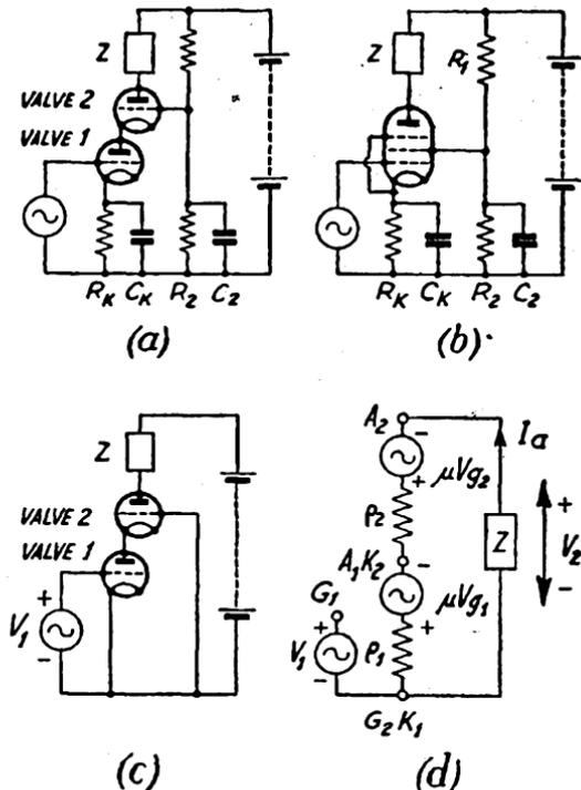
FIG. 61. THE CASCODE CIRCUIT
