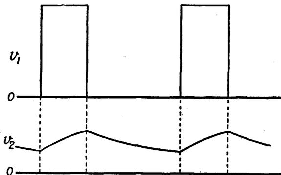
FIG. 177 QUASI-INTEGRATION WITH THE CIRCUIT OF FIG. 175 (b)
