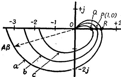
FIG. 72. POLAR PLOT OF THE LOOP GAIN
