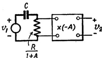
FIG. 214. EQUIVALENT CIRCUIT OF FIG. 212 (a)
