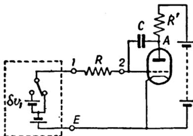
FIG. 216. SIMPLE MILLER INTEGRATOR CIRCUIT WITH STEP-FUNCTION INPUT
