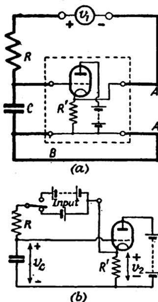
FIG. 222. BOOTSTRAP INTEGRATING CIRCUIT
