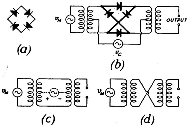
FIG. 158. THE RING MODULATOR
