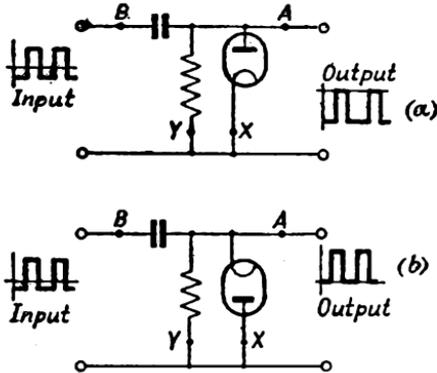
FIG. 208. D.C. RESTORATION CIRCUITS
