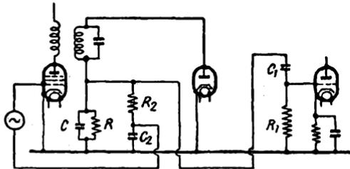
FIG. 137. AUTOMATIC GAIN CONTROL. SINGLE DIODE FOR DETECTION AND A.G.C.
