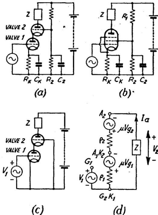
FIG. 61. THE CASCODE CIRCUIT
