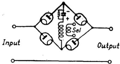
FIG. 201. BRIDGE-TYPE SWITCH CIRCUIT
