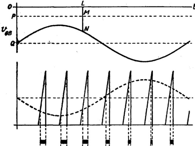
FIG. 173. PULSE-WIDTH MODULATION. ADDITION AND AMPLITUDE SELECTION
