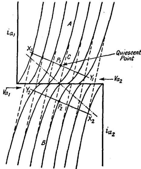
FIG. 43. COMPOSITE CHARACTERISTICS FOR PUSH-PULL CIRCUIT
