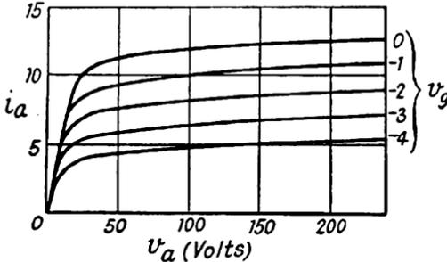
FIG. 18. CHARACTERISTICS OF PENTODE
