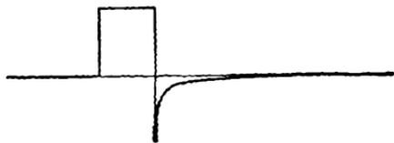
FIG. 3-25.—Spike often produced by shunt capacity.
