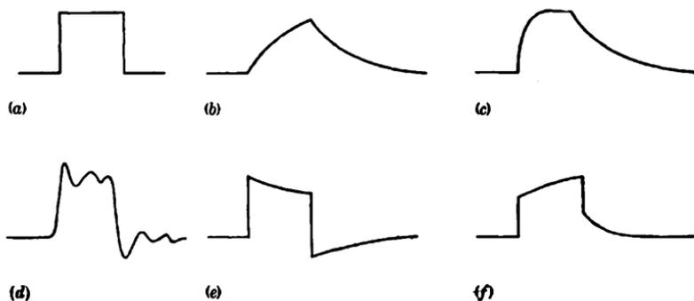
FIG. 8-14.—Effects of amplifier characteristics on output-pulse shape.
