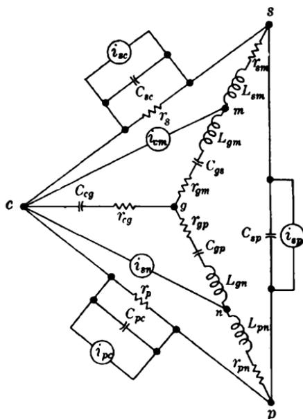
FIG. 12-15.—Noise representation of a pentode at moderately high frequencies.
