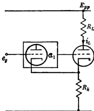
FIG. 11-54.—Cathode and screen feedback.
