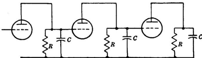
FIG. A-5.—Cascade of  $n$  identical  $RC$ -coupled pulse-amplifier stages.
