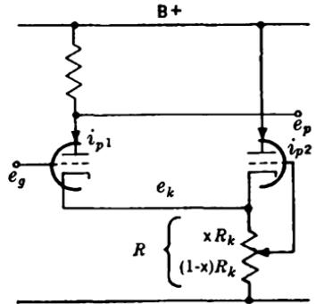
FIG. 11-45.—Balancing  $E_f$  variation with a self-biased cathode follower.
