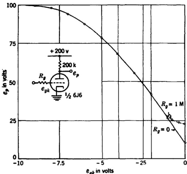
FIG. 11-11.—Typical triode amplifier characteristics.
