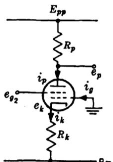
FIG. 11-48.—First grid as diode plate.
