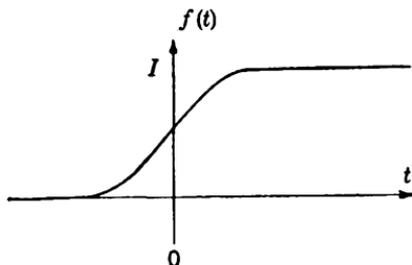
FIG. A-2.—Step-function response of Gaussian-error-curve filter.
