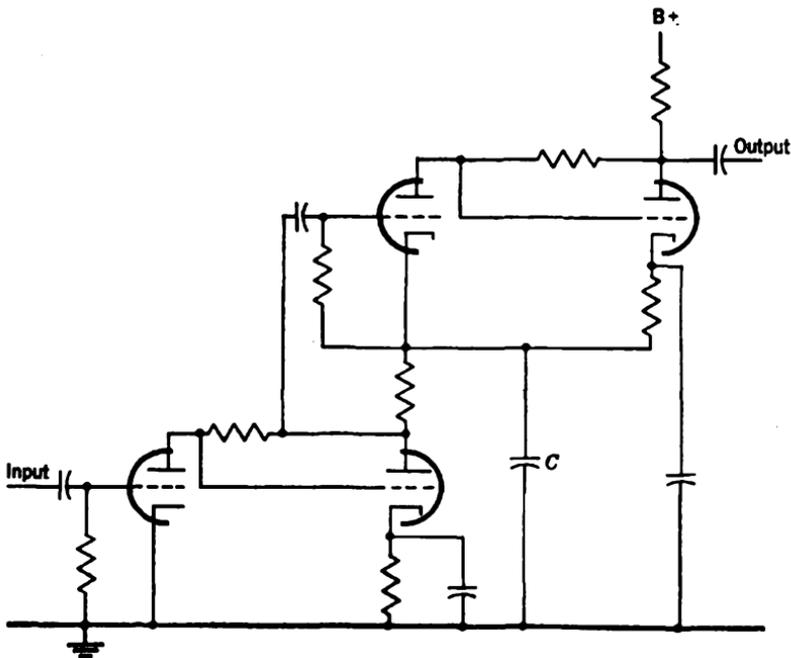
FIG. 3-34.—Series-fed direct-coupled inverse-feedback pairs.
