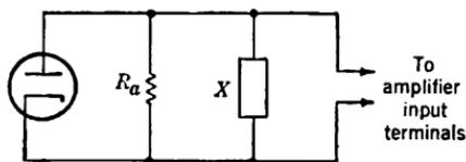
FIG. 14.4.—High-impedance diode noise generator.
