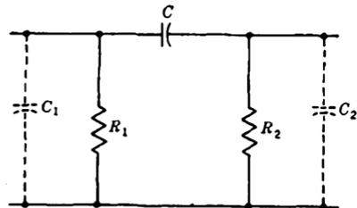
FIG. 3-24.—Coupling circuit including shunt capacity.
