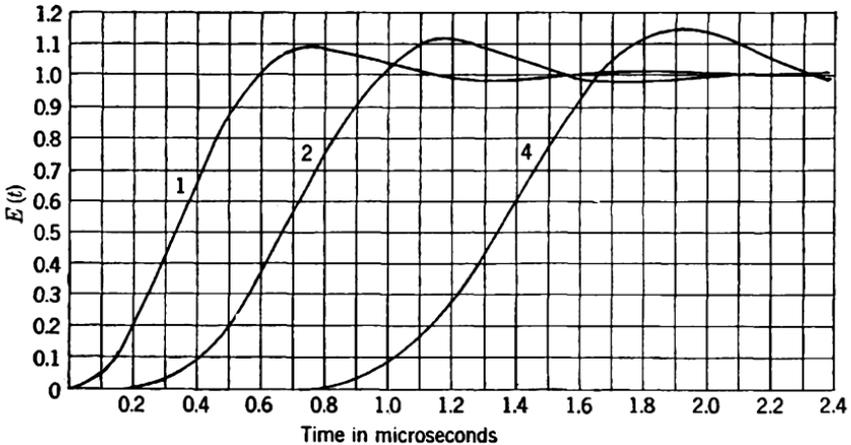
FIG. 7-6.—Step-function response of a cascade of  $n$  flat staggered triples,  $n = 1, 2, 4$ , each triple of bandwidth 2 Mc/sec between 3-db points. These curves also apply to transitionally coupled triple-tuned circuits, flat inverse-feedback triples, flat combinations of an overcoupled double-tuned circuit and a single-tuned circuit, and in general to all minimum-phase circuits having absolute value vs. frequency curves of the form  $1/\sqrt{1+x^2}$ .
