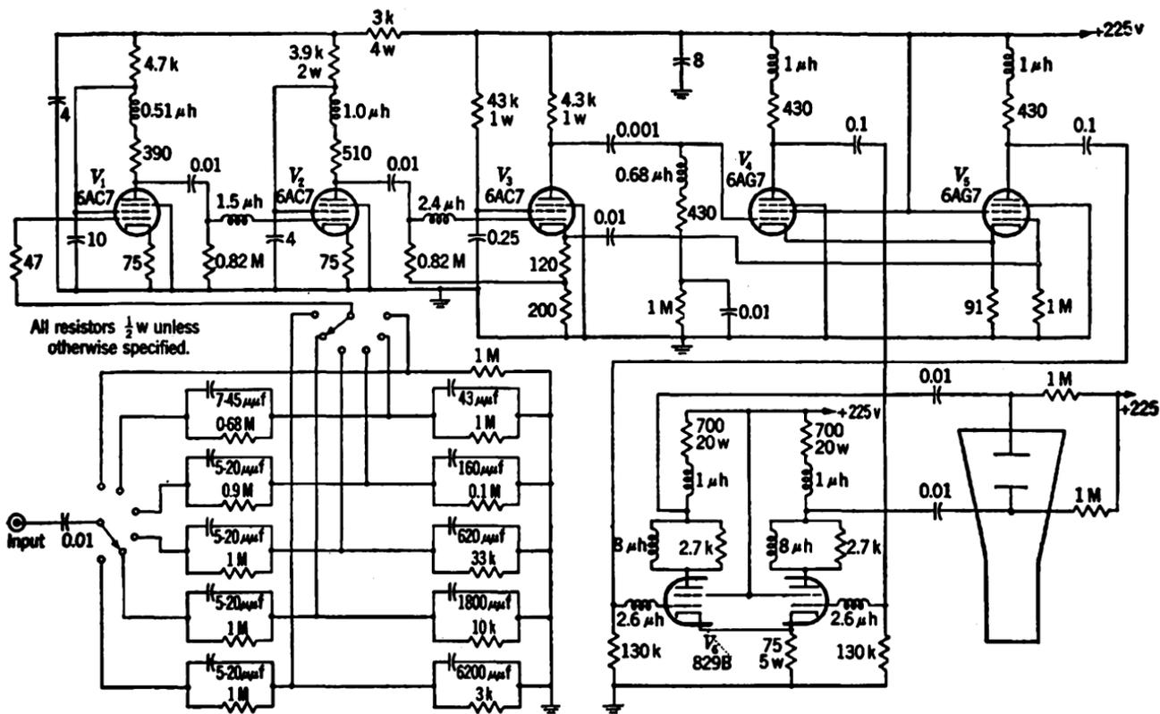
FIG. 2-38.—Pulse amplifier for deflection-modulated cathode-ray tube.
