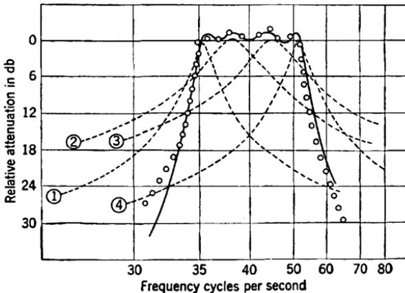
FIG. 10-16.—Pass band, four-section stagger-tuned filter. Calculated values, solid line; experimental values, dotted line. (a)  $f_1 = 40.6$  cps,  $Q_1 = 15$ ; (b)  $f_2 = 46.0$  cps,  $Q_2 = 6$ ; (c)  $f_3 = 54.9$  cps,  $Q_3 = 6$ ; (e)  $f_4 = 61.9$  cps,  $Q_4 = 15$ .
