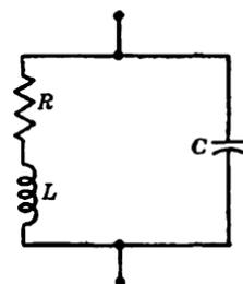
FIG. 2-4.—Shunt-peaked circuit.
