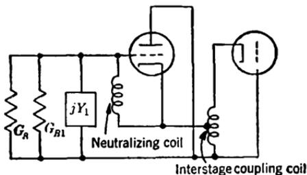
FIG. 13-17.—Grounded-plate-triode-grounded-grid-triode input configuration.
