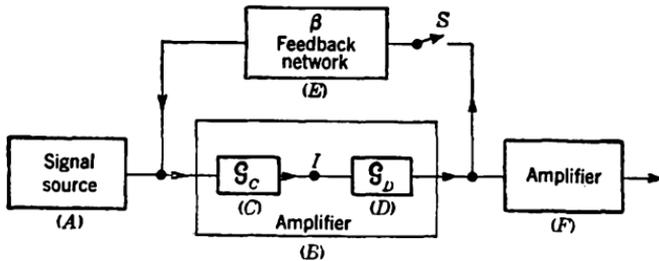
FIG. 13-18.—Block diagram of amplifier with feedback.
