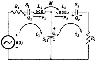
FIG. 1·7.—Two-mesh network.
