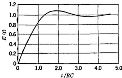
FIG. 2-13.—Response to step-function current of two-terminal flat-gain network of maximum gain-bandwidth product. The overshoot is 9.4 per cent, and the gain/rise time advantage over a parallel  $RC$ -circuit is 2.2.
