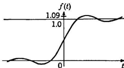
FIG. A·4.—Step-function response of idealized low-pass filter.
