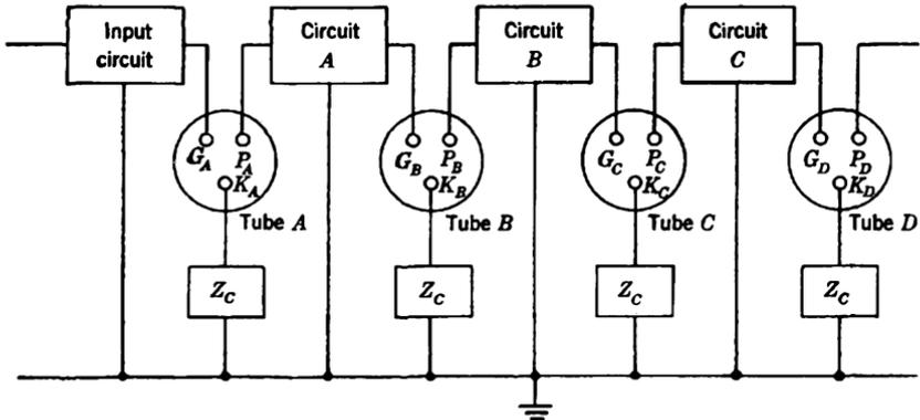
FIG. 8-13.—Tube and circuit line-up in an amplifier. The cathode-circuit impedance  $Z_c$  is a short circuit at the intermediate frequency and is equal to the bias resistance (50 to 200 ohms) at pulse and lower frequencies.
