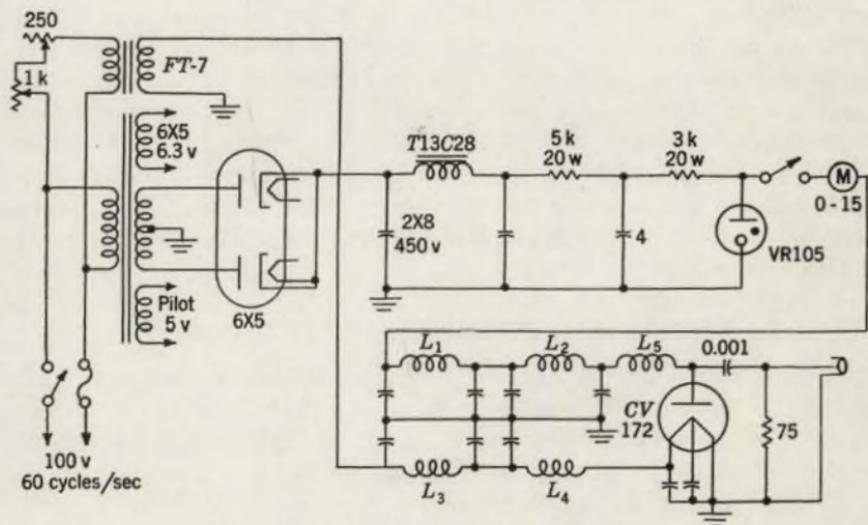
FIG. 14-9.—Circuit of noise generator.
