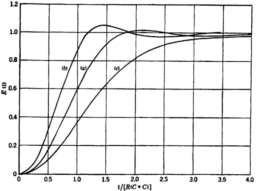
FIG. 2·9.—Response to current step function of network shown in Fig. 2·8. (a)  $C_2 = C$ ; (b)  $C_2 = C/2$ ; (c)  $C_2 = 2C$ .
