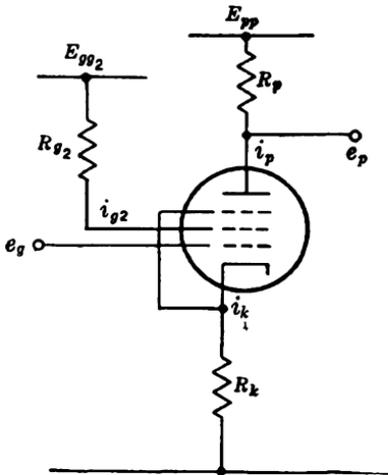
FIG. 11-19.—Pentode amplifier with cathode and screen resistors.
