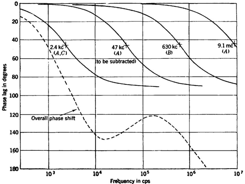
FIG. 9-37.—Over-all phase characteristic of amplifier at high frequencies (calculated).
