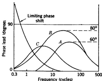
FIG. 9-30.—First approximation of synthesis of phase networks.
