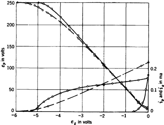
FIG. 11-20a.—Output characteristics of a triode amplifier with and without a “constant-current” diode as plate load (6SL7 triode,  $E_{pp} = 250$  volts). Solid curves: plate load is a 6H6 diode,  $E_f = 2.4$  volts; dashed curves: plate load is a 1.1-megohm resistor.
