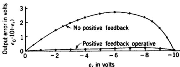
FIG. 11-61.—Deviation from linearity of output voltage, with and without positive feedback for each curve; negative feedback was adjusted so  $e_o = 0$  at  $e_i = 0$  and  $e_o = 100$  at  $e_i = -10$ .
