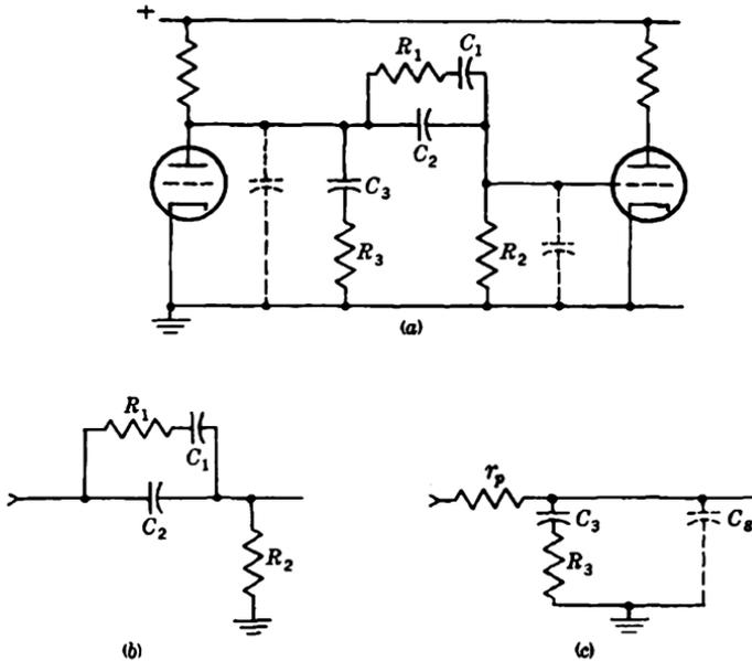
FIG. 9-4.—Typical coupling network. (a) Coupling network; (b) low-frequency equivalent circuit; (c) high-frequency equivalent circuit.
