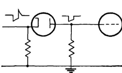
FIG. 3-14a.—Series diode.
