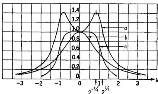
FIG. 5-8.—Stagger-damped pair (a)  $1/\sqrt{1 - y^2 \sqrt{2} + y^4}$ ; (b)  $1/\sqrt{1 + y^2 \sqrt{2} + y^4}$ ; (c)  $1/\sqrt{1 + y^8}$ . (a) and (b) are the component selectivity curves of a stagger-damped pair; (c) is the over-all result.
