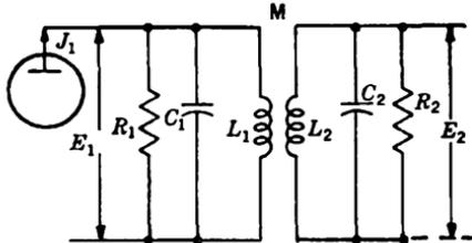
FIG. 5-1a.—Inductance-coupled double-tuned circuit.
