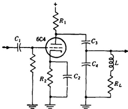
FIG. 9-13.—Output stage of driver.
