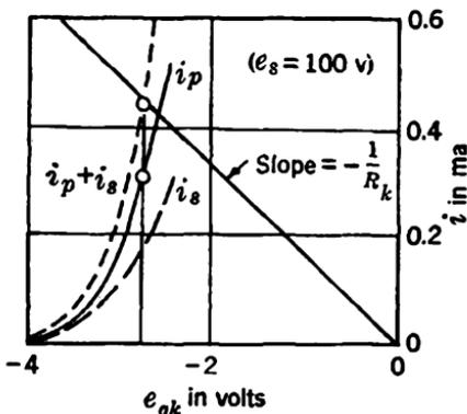
FIG. 11-74.—Determination of constant-current pentode current.
