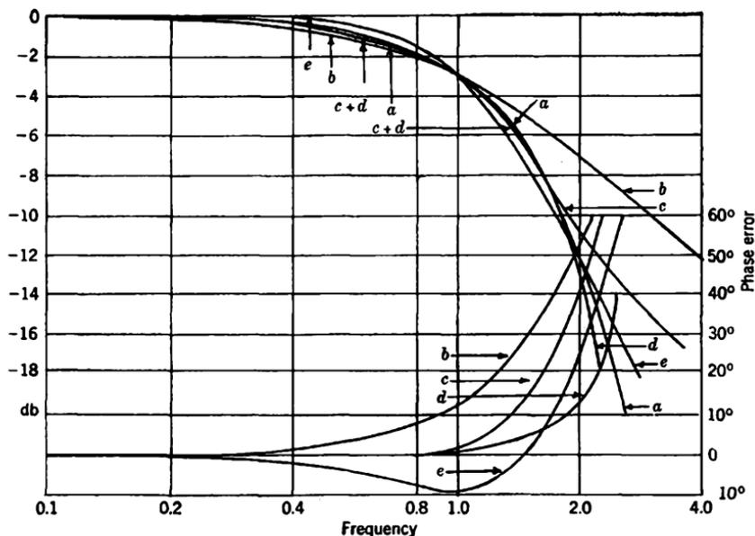
FIG. 2-12.—Normalized absolute value and phase error curves. (a) Gaussian error curve, overshoot = 0 per cent (phase assumed linear); (b) RC-circuit, overshoot = 0 per cent; (c) two-terminal linear-phase network, overshoot = 1 per cent; (d) four-terminal linear-phase network, overshoot = 1 per cent; (e) low-pass equivalent of transitionally coupled double-tuned circuit, overshoot = 4.3 per cent.
