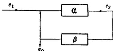
FIG. 10-7.—Block diagram of rejection amplifier.
