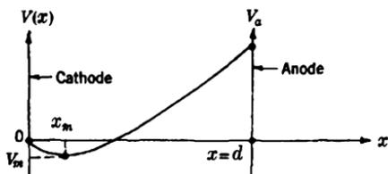
FIG. 12-11.—Potential distribution in a plane parallel diode under space charge conditions.
