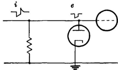
FIG. 3-14b.—Shunt diode.
