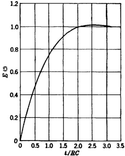
FIG. 2-7.—Response of two-terminal linear-phase network to a step function of current. Gain/rise time advantage over the RC-circuit is 1.77; overshoot is 1 per cent.
