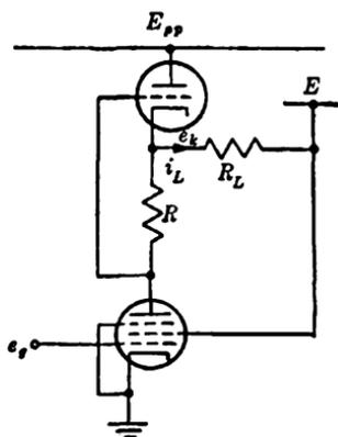
FIG. 11-39.—Series amplifier using pentode.
