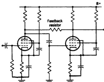
FIG. 2-21.—Feedback from plate to preceding plate.
