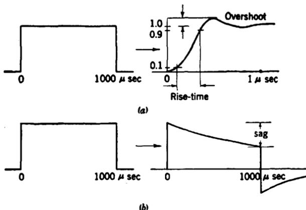
FIG. 2-1.—Reproduction of a rectangular pulse. (a) Reproduction of the leading edge of a rectangular pulse. Note the rise time and the overshoot. If the amplifier is linear and the pulse duration is large compared with the rise time, the reproduction of the trailing edge is the negative of the leading edge. (b) Reproduction of the flat top of a rectangular pulse. Note the sag. If the amplifier is linear, the amplitude of the undershoot following the pulse is equal to the sag.
