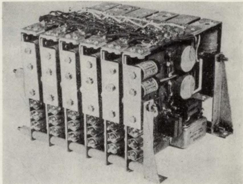
FIG. 10-13.—Photograph showing lightweight selective amplifiers and detectors constructed of subminiature tubes.
