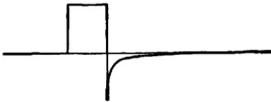
FIG. 3-25.—Spike often produced by shunt capacity.
