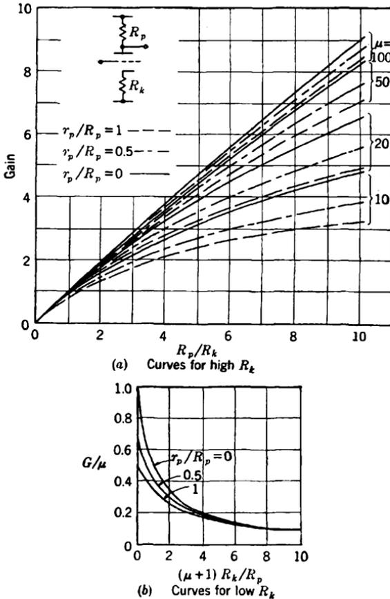
FIG. 11-15.—Gain of triode amplifier with cathode resistor.
