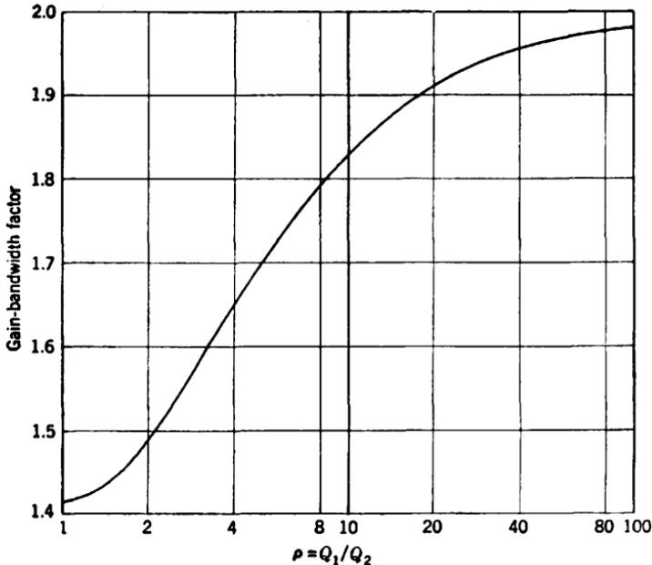
FIG. 5-2.—Gain-bandwidth factor of transitionally coupled double-tuned circuit as function of Q-ratio.
