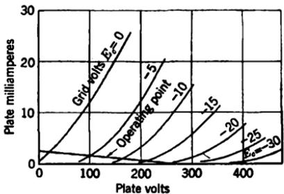
FIG. 9-28.—D-c operation of third amplifier stage.
