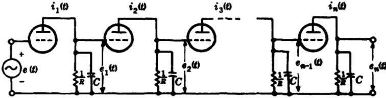
FIG. 1-23.—The  $n$ -stage RC-coupled pulse amplifier.
