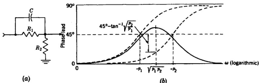
FIG. 9-6.—“Phase-advance” network. (a) Network; (b) phase response as a function of frequency,  $\frac{p_2}{p_1} = 10$ ;  $-p_1 = \frac{1}{CR_1}$ ;  $-p_2 = \frac{(R_1 + R_2)}{R_1 R_2 C}$ ;  $\sqrt{p_1 p_2} = \frac{1}{CR_1} \sqrt{1 + \left(\frac{R_1}{R_2}\right)}$ .
