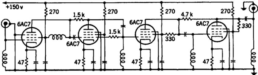
FIG. 6-18.—Flat quadruple feedback amplifier.
