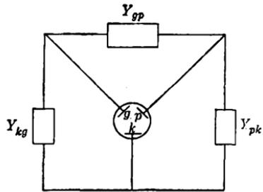
FIG. 13-6.—The general externally loaded three-node network.
