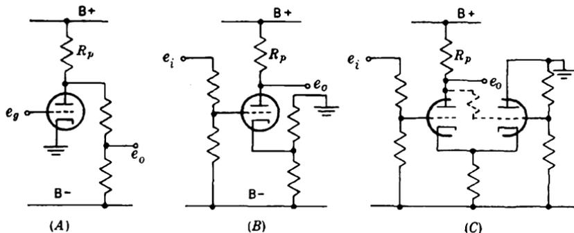
FIG. 11-33.—Voltage output embracing ground potential.
