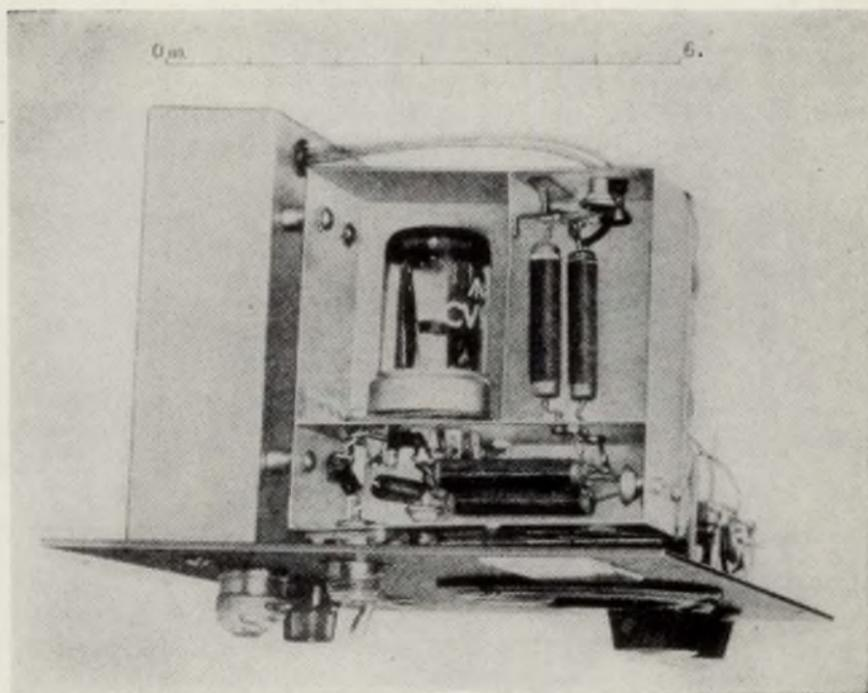
FIG. 14-8.—Interior view of CV172 noise source.
