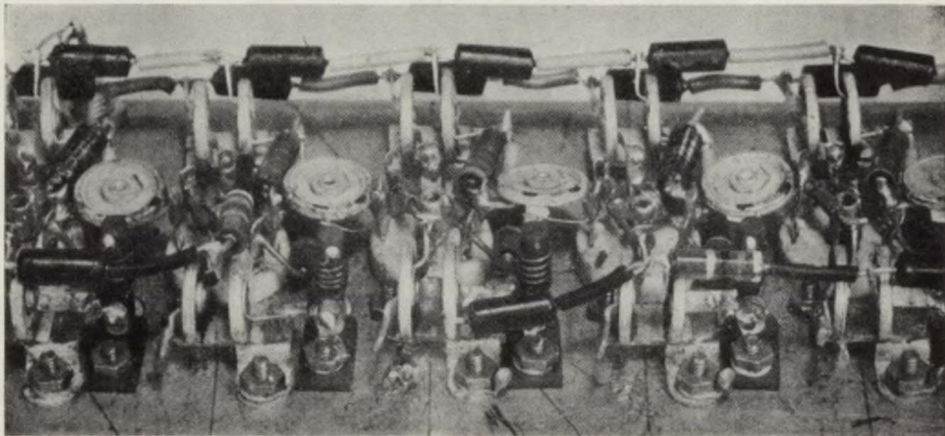
FIG. 4-16.—Bottom view of a few stages of a 12-stage 100-db 6AK5 amplifier made up of four flat-staggered triples, 20 Mc/sec wide at 200 Mc/sec.
