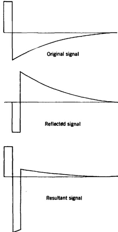
FIG. 3-18.—Effect of delay line upon signal with overshoot (delay time equal to pulse width).
