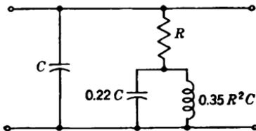
FIG. 2-6.—Two-terminal linear-phase network.
