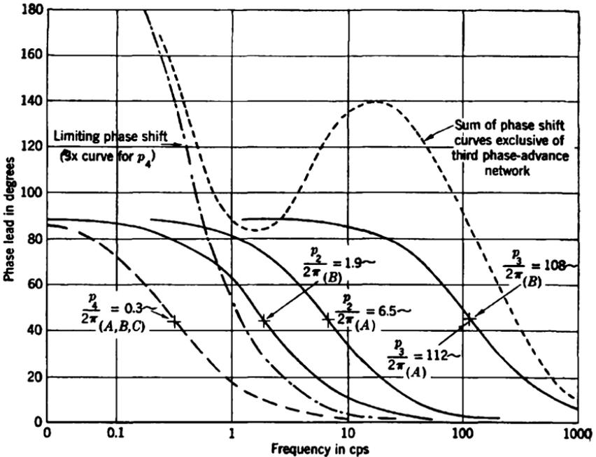
FIG. 9-31.—Phase characteristics for two stabilization networks.
