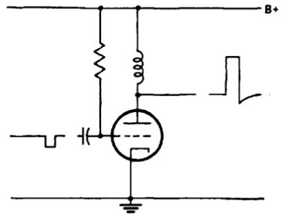
FIG. 3-29.—High-output voltage circuit.
