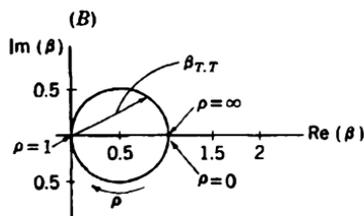
FIG. 10-2.—Phase-amplitude diagram of twin-T network.
