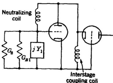
FIG. 13-12.—Grounded-cathode-triode-grounded-grid-triode input configuration.
