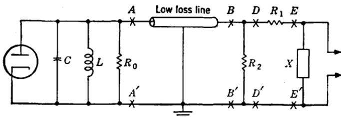
FIG. 14-5.—Matched-line diode noise generator.
