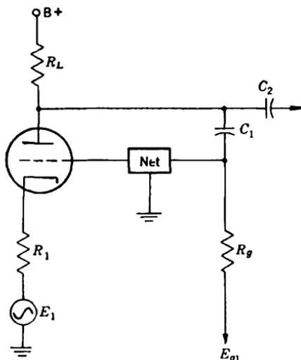
FIG. 10-8.—Single-stage frequency-selective amplifier.
