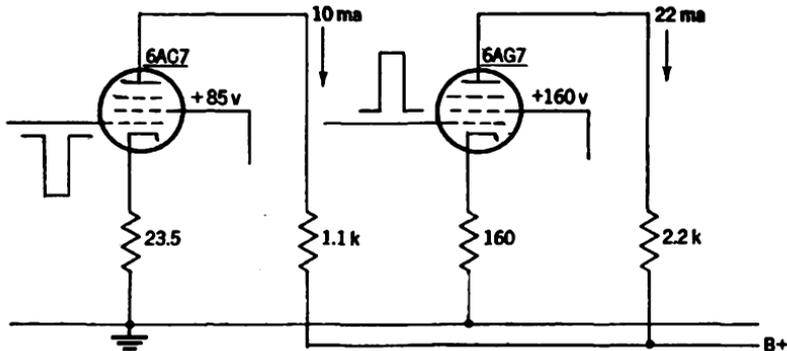
Fig. 3-35.—Typical pair of stages for amplifier No. 1.
