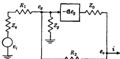
FIG. 9-2.—Schematic circuit for resistive-mixing feedback.
