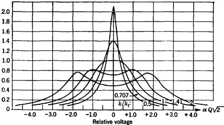
FIG. 5.4.—High- $Q$  double-tuned circuit, loaded one side only,  $Q$  fixed,  $k$  variable.
