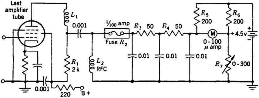
FIG. 14-16.—Unbalanced-bridge bolometer.
