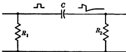
FIG. 3-1.—Coupling circuit.
