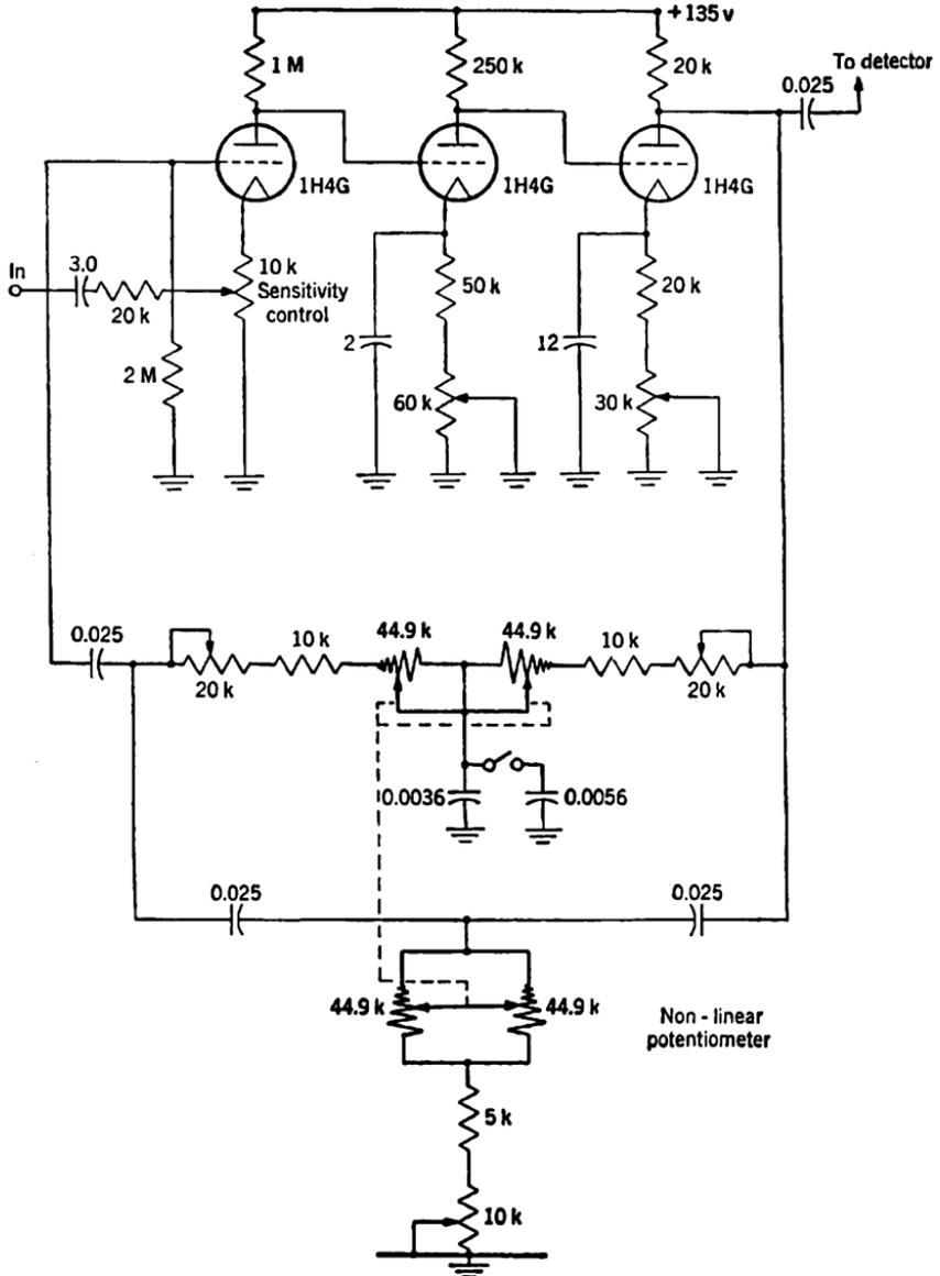
FIG. 10-15.—Three-stage direct-coupled amplifier. (Courtesy of General Radio.)
