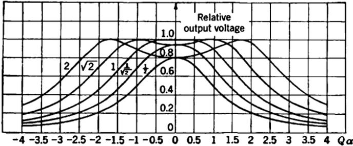
FIG. 5-3.—Absolute value vs. frequency curves of high-Q equal-Q double-tuned circuits as function of coefficient of coupling. The parameters associated with the various curves are the values of  $kQ$ .
