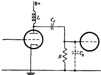
FIG. 3-10.—Choke-coupling circuit.
