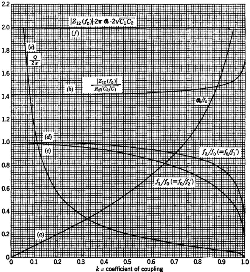
FIG. 5-7.—Design data for low- $Q$  transitionally coupled double-tuned circuit  $Q_1 = \infty$ ,  $Q_2 = Q$ . (a) Fractional bandwidth  $\mathcal{B}/f_0$ ; (b) normalized midband gain; (c) primary resonant frequency; (d) secondary resonant frequency; (e)  $Q/2\pi = f_0 R_2 C_2$ ; (f) gain-bandwidth factor  $|Z_{12}(f_0)| 2\pi \mathcal{B} \sqrt{C_1 C_2}$ .
