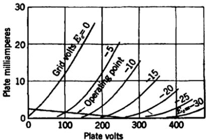
FIG. 9-28.—D-c operation of third amplifier stage.
