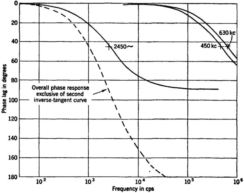
FIG. 9-35.—Calculated phase characteristics of high-frequency network.
