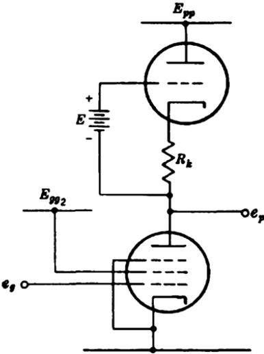
FIG. 11-18.—Constant-current device as a pentode load resistor.
