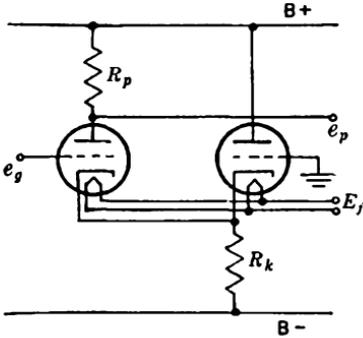
FIG. 11-44.—Balancing  $E_p$  variation with a cathode follower.
