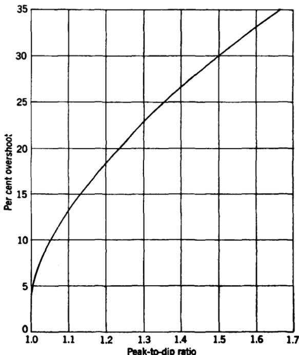
FIG. 7-4.—Overshoot of overstaggered pair, as function of ratio of maximum response to response at midband. The curve also applies to double-tuned circuits of arbitrary  $Q$ -ratio, and inverse-feedback pairs.
