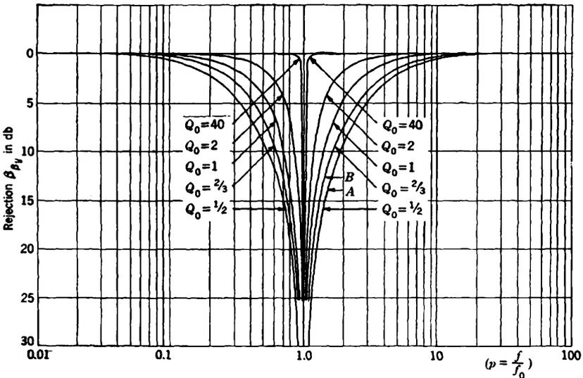
FIG. 10-3.—Characteristics of rejection networks. The values of  $Q_0$  pertain to the bridged-T network; curve A pertains to a twin-T network for which  $n = 1$ ; curve B pertains to a Wien-bridge network. (a) Phase characteristics; (b) amplitude characteristics.
