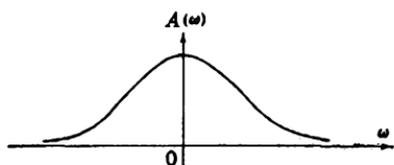
FIG. A-1.—Gaussian-error-curve filter,
