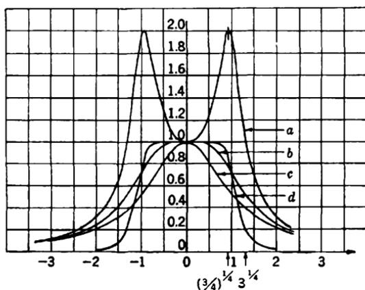
FIG. 5-9.—Stagger-damped triple. (a)  $1/\sqrt{1 - y^2 \sqrt{3} + y^4}$ ; (b)  $1/\sqrt{1 + y^4}$ ; (c)  $1/\sqrt{1 + y^2 \sqrt{3} + y^4}$ ; (d)  $1/\sqrt{1 + y^{12}}$ . (a), (b), and (c) are the component selectivity curves of a stagger-damped triple; (d) is the over-all result.
