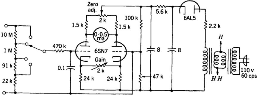
FIG. 11-62.—Simple vacuum-tube voltmeter.
