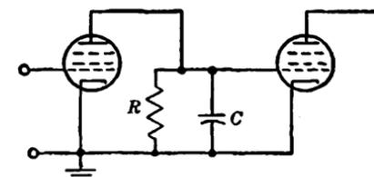
FIG. 2-3.—Simplified circuit of pulse-amplifier stage employing  $RC$ -coupling.
