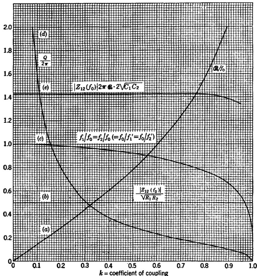
FIG. 5-6.—Design data for low- $Q$  transitionally coupled double-tuned circuit,
