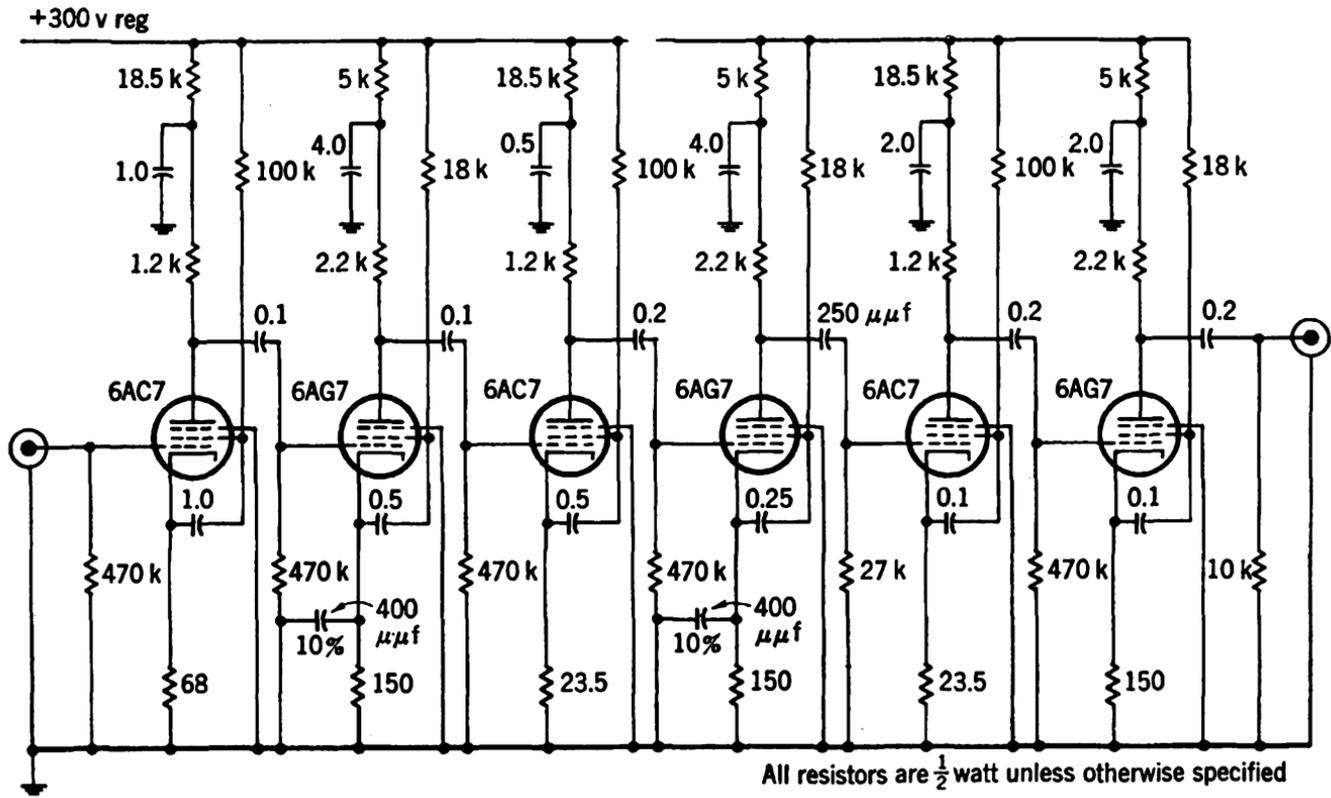
FIG. 3-36.—Complete circuit diagram for amplifier No. 1.
