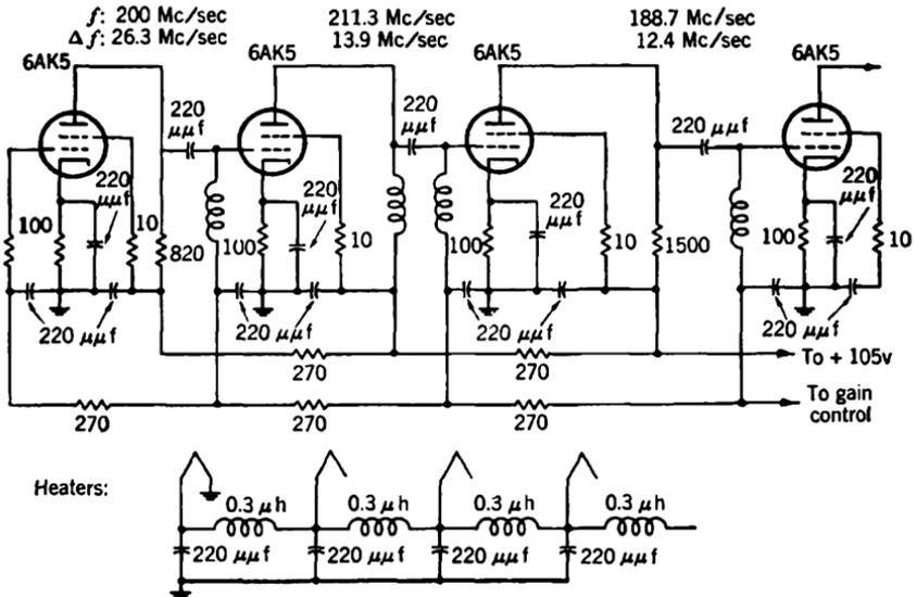
FIG. 4-15.—Circuit diagram of one triple of 12-stage 100-db 6AK5 amplifier made up of four flat-staggered triples, 20 Mc/sec wide at 200 Mc/sec.
