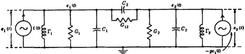
FIG. 1-14.—Equivalent two-node active network.
