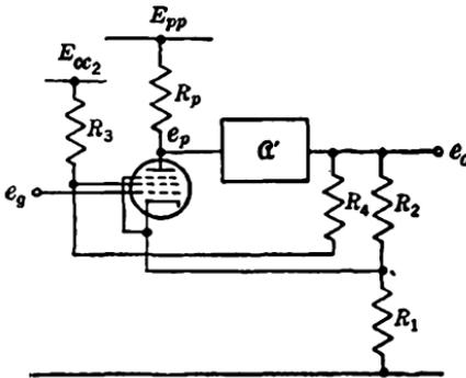
FIG. 11-55.—Example of current feedback.
