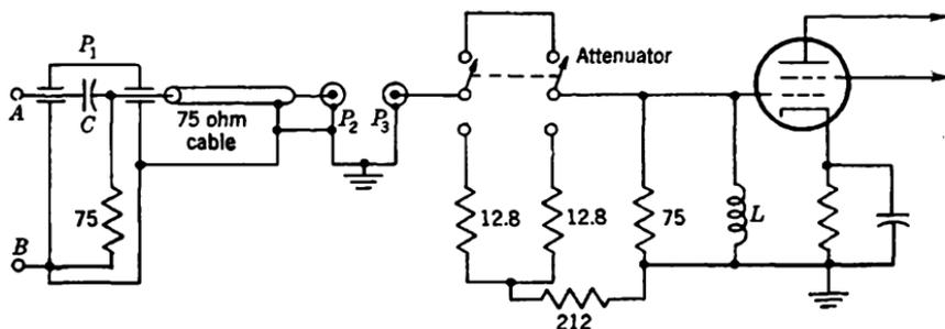
FIG. 14-12.—Details of attenuator and its immediate circuit.
