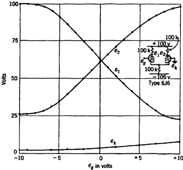
FIG. 11-29.—Example of differential amplifier and characteristic
