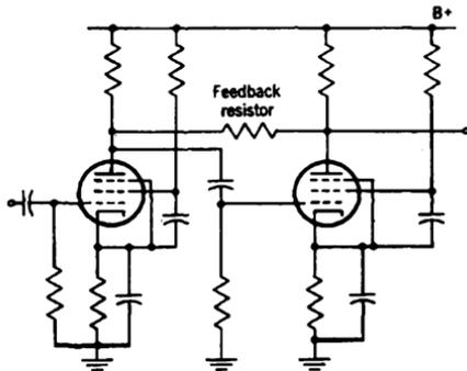
FIG. 2-21.—Feedback from plate to preceding plate.
