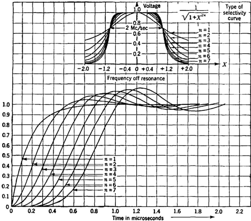
FIG. 7.7.—Step-function response of the (minimum phase shift) networks having the absolute value curves shown above.
