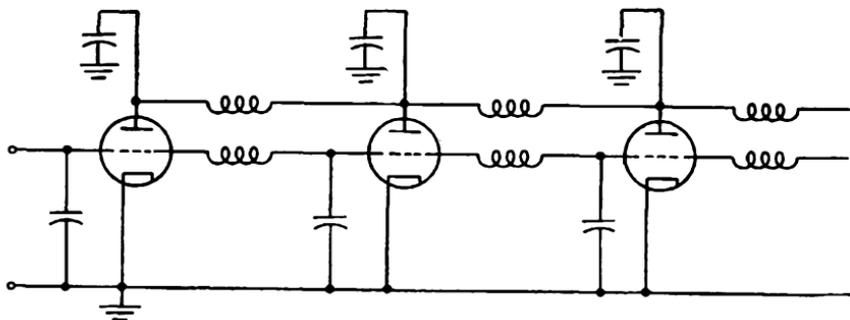
FIG. 2-16.—"Transmission-line" amplifier.
