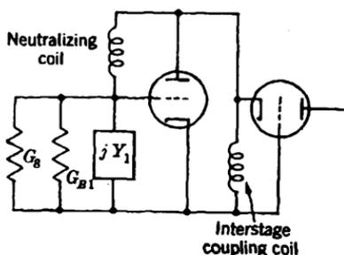
FIG. 13-12.—Grounded-cathode-triode-grounded-grid-triode input configuration.
