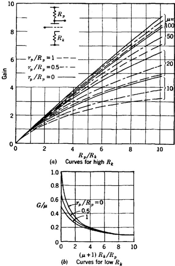
FIG. 11-15.—Gain of triode amplifier with cathode resistor.
