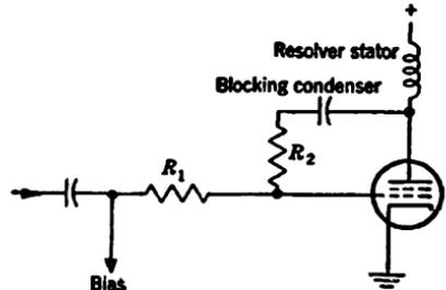
FIG. 9-11.—Single-stage driver with plate-to-grid feedback.
