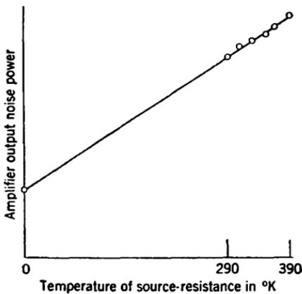
FIG. 14-17.—Radiometer determination of amplifier noise figure.
