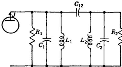
FIG. 5-1b.—Capacity-coupled double-tuned circuit.
