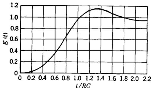
FIG. 2-14.—Response to step-function current of the  $n = 3$  approximation to the four-terminal flat-gain network of maximum gain-bandwidth product. The overshoot is 15.2 per cent, and the gain/rise time advantage over a parallel  $RC$ -circuit is 3.75.
