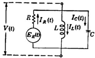
FIG. 12-3.—Thermal noise variables in  $RLC$  circuit.
