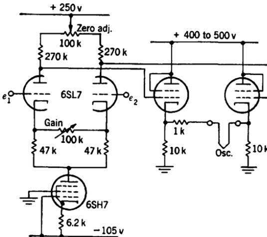
FIG. 11-64.—Two-stage oscillograph driver.
