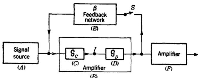
FIG. 13-18.—Block diagram of amplifier with feedback.
