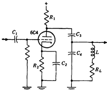
FIG. 9-13.—Output stage of driver.
