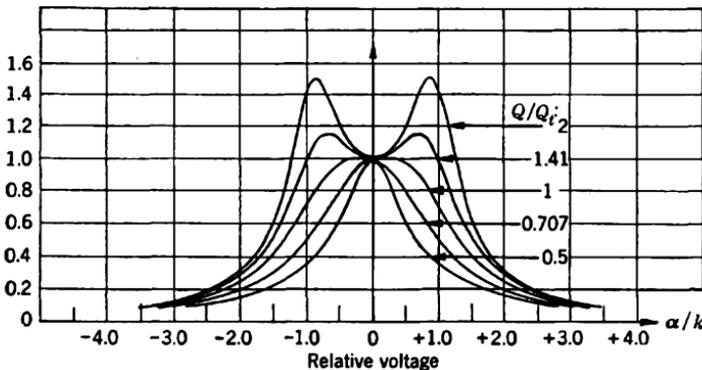
FIG. 5-5.—High- $Q$  double-tuned circuit, loaded one side only,  $k$  fixed,  $Q$  variable.
