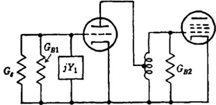
FIG. 13-11.—High-stability interstage coupling with grounded-cathode-triode input stage.
