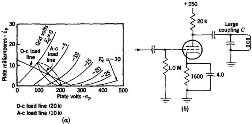
FIG. 9-15.—Operation of 6C4 output stage.
