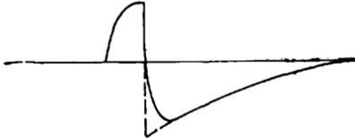
FIG. 3-11.—Overshoot produced by choke-coupling circuit.
