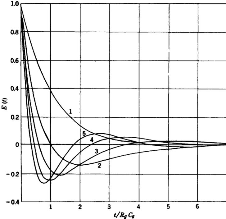
FIG. 2-17.—Step-function response of  $n$  capacitance-coupled stages each of time constant  $R_oC_o$ .
