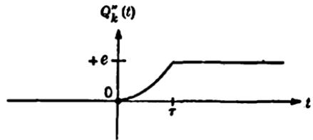
FIG. 12-10.—Induced charge due to the passage of a single electron  $k$  from cathode to anode.
