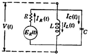
FIG. 12-3.—Thermal noise variables in  $RLC$  circuit.
