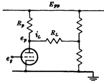
FIG. 11-32.—Plate as output terminal.
