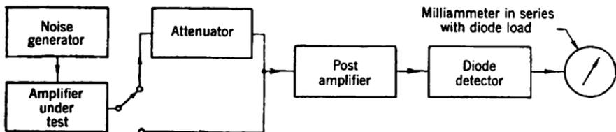
FIG. 14-11.—Attenuator and postamplifier method of measuring noise.
