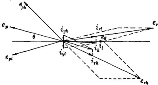
FIG. 6-12.—Vector diagram off resonance showing transit-time effect.
