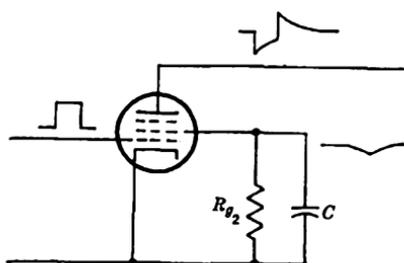
FIG. 3-4.—Screen bypass circuit.
