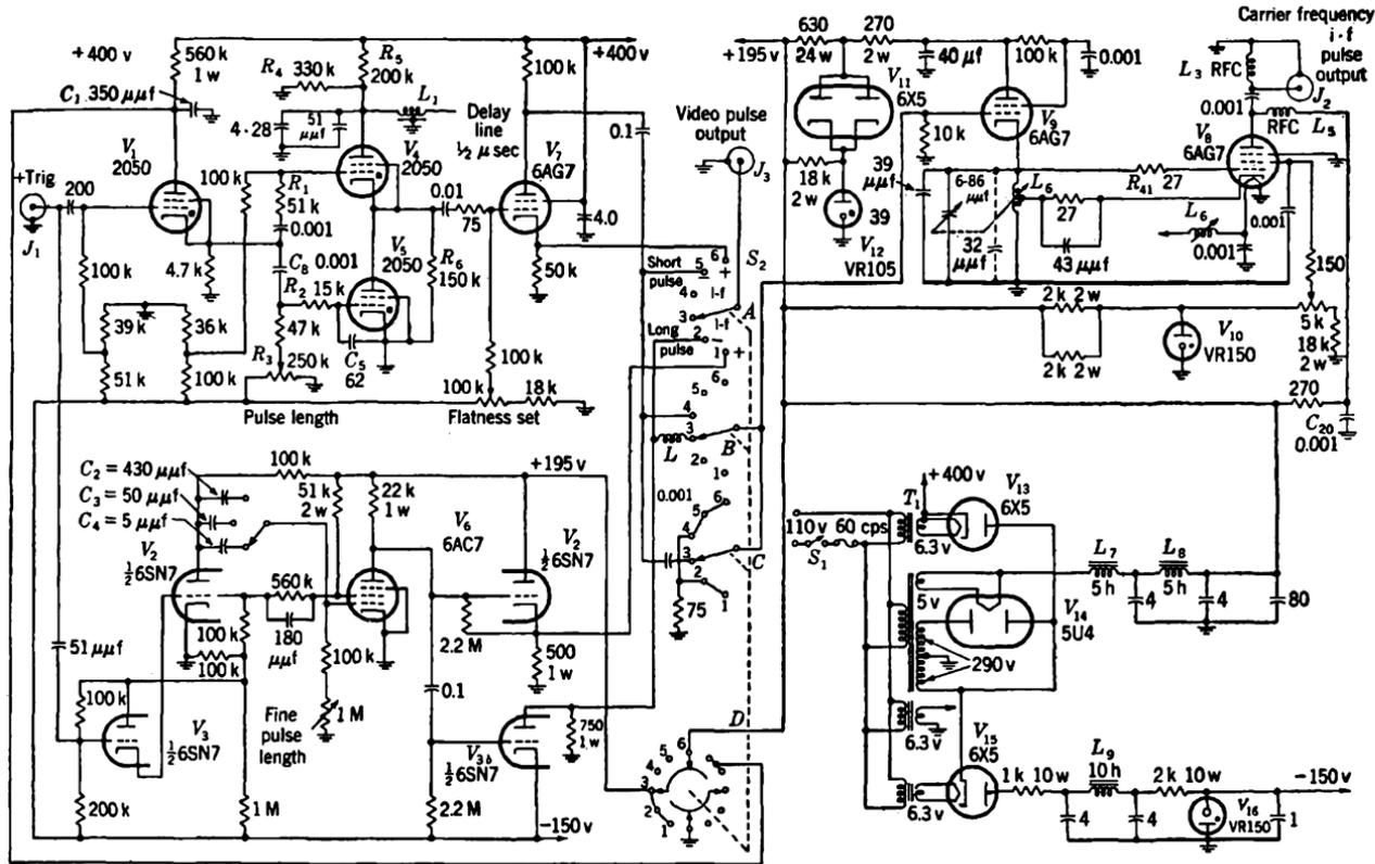
FIG. 8-5.—Circuit diagram of pulse generator.  $S_2 - A, B,$  and  $C$  are nominally 1-gang 11-position switch decks.  $S_2 - D$  is nominally a 2-gang 5-position deck, but a sixth position is used as an OFF position.  $S_2$  is shown in position 3.  $S_2$  positions: (a) — long; (b) + long; (c) carrier-frequency long; (d) carrier-frequency short; (e) — short; (f) + short.
