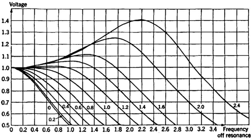
FIG. 7-8.—Overstaggered pairs. The parameter is the ratio  $a$  of separation of the resonant frequencies of the staggered circuits to their bandwidth. The value  $a = 1$  corresponds to a flat-staggered pair.
