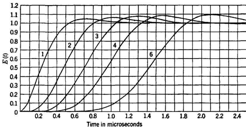
FIG. 7-5.—Step-function response of cascade of  $n$  flat-staggered pairs,  $n = 1, 2, 3, 4, 5, 6$ , each pair of bandwidth 2 Mc/sec between 3-db points. These curves also apply to transitionally coupled double-tuned circuits, flat inverse-feedback pairs, and in general to all minimum-phase circuits having absolute value vs. frequency curves of the form  $1/\sqrt{1+x^4}$ .
