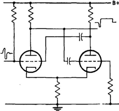
FIG. 3-28.—Multivibrator output circuit.
