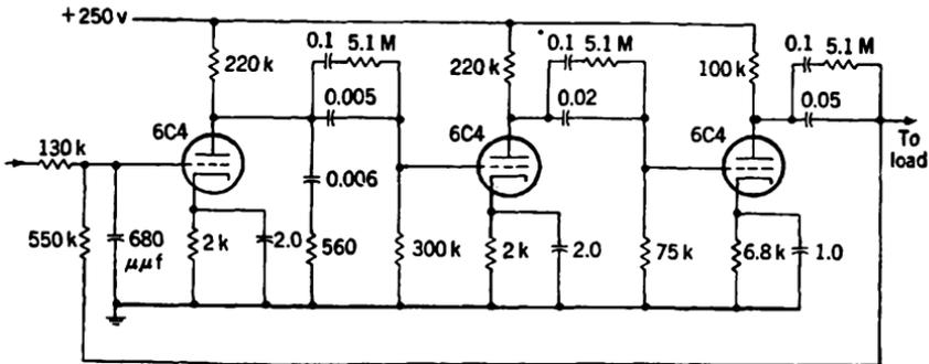
FIG. 9-39.—Design of three-stage feedback amplifier with stabilization networks.
