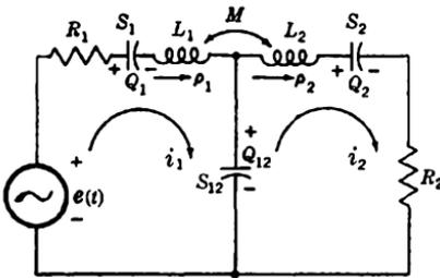
FIG. 1·7.—Two-mesh network.
