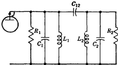
FIG. 5-1b.—Capacity-coupled double-tuned circuit.
