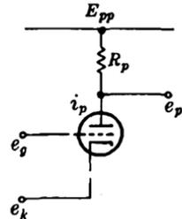
FIG. 11-24.—Triode with two input terminals.
