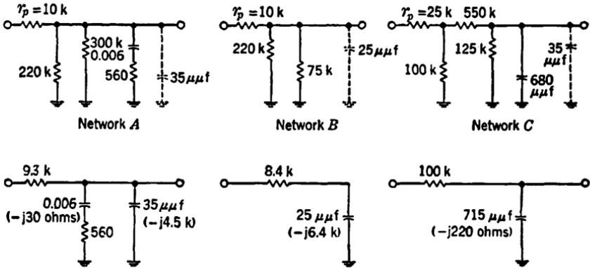
FIG. 9-38.—High-frequency stabilization networks with reactances at 1.0 Mc/sec.
