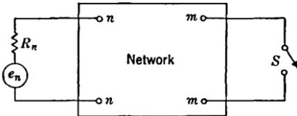
FIG. 12-7.—Arbitrary linear passive network showing one component resistance  $R_n$  at temperature  $T_n$ , regarded as input with terminals  $(n,n)$ ; and any two points of the network  $(m,m)$  regarded as output terminals.  $S$  is a short-circuiting switch.
