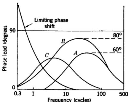
FIG. 9-30.—First approximation of synthesis of phase networks.
