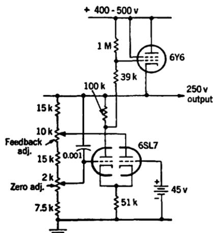
FIG. 11-58.—Voltage regulator employing positive feedback.
