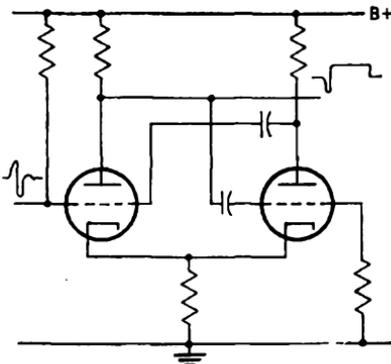
FIG. 3-28.—Multivibrator output circuit.
