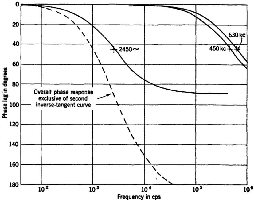
FIG. 9-35.—Calculated phase characteristics of high-frequency network.
