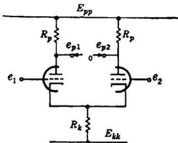
FIG. 11·28.—Symmetrical differential amplifier.
