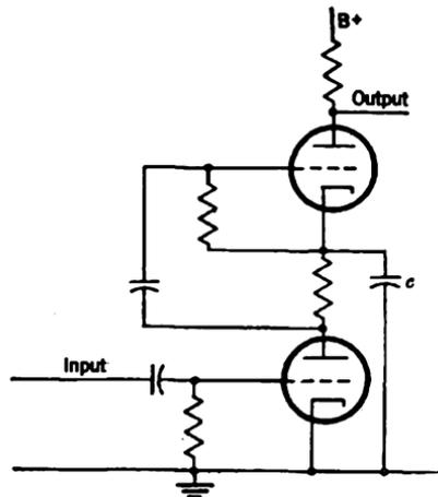
FIG. 3-33.—Series-fed circuit.
