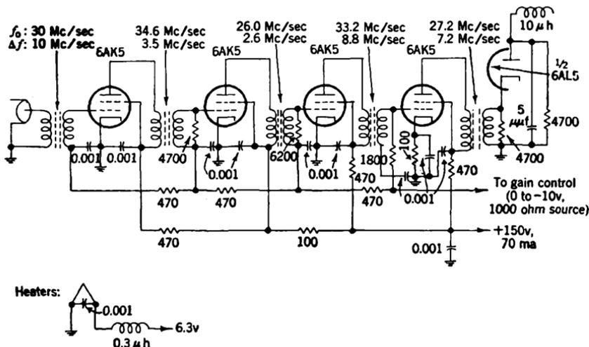
FIG. 4-13.—Circuit diagram of four-stage 80-db 6AK5 flat-staggered quintuple, 10 Mc/sec wide at 30 Mc/sec. The coils are unity-coupled. The chassis shown in Fig. 4-14 contains a pulse amplifier stage also.
