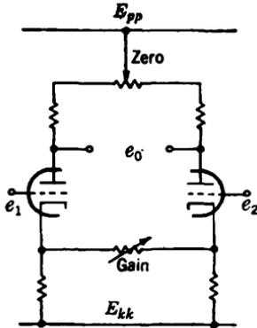
FIG. 11-30.—Differential amplifier with gain and zero adjustments.
