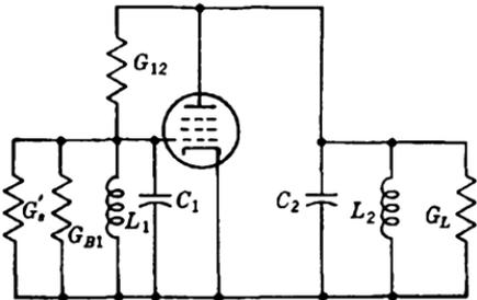
FIG. 13-20.—Pentode with plate-grid resistance feedback.
