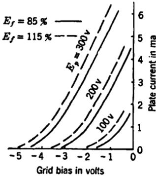
FIG. 11-7.—Effect of heater voltage on 6SL7 characteristics.
