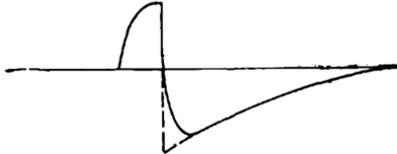
FIG. 3-11.—Overshoot produced by choke-coupling circuit.
