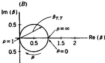
FIG. 10-2.—Phase-amplitude diagram of twin-T network.
