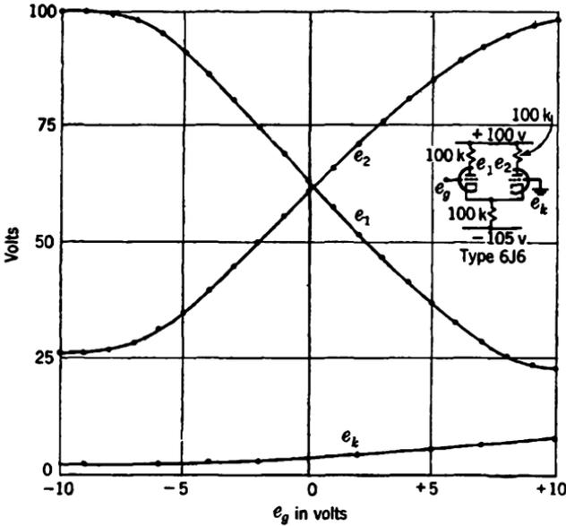
FIG. 11-29.—Example of differential amplifier and characteristic
