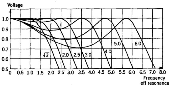
Fig. 7-9.—Overstaggered triples. The parameter is the ratio  $a$  of separation of the resonant frequencies of the staggered circuits to their bandwidth. The value  $a = \sqrt{3}$  corresponds to a flat triple.
