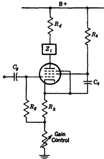
Fig. 2-25.—Variation of gain by feedback (cathode degeneration).
