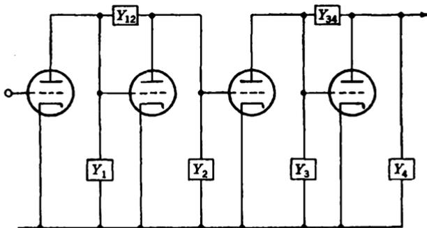
FIG. 6-4.—Feedback pairs.
