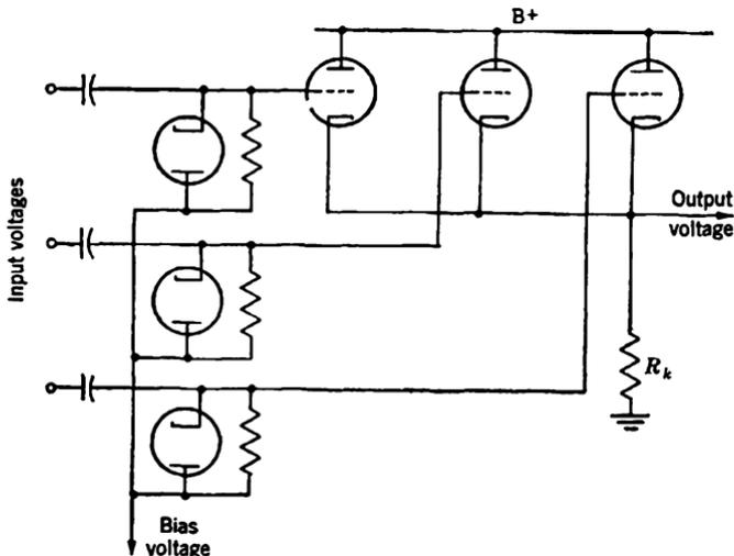
FIG. 2-32.—Nonadditive mixer for positive-polarity signals. Any number of input channels can be used, with one tube for each input channel.
