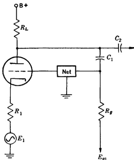
FIG. 10-8.—Single-stage frequency-selective amplifier.
