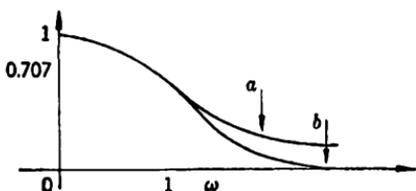
FIG. A-6.—Absolute value vs. frequency curves of (a) cascade of  $n$  identical  $RC$ -coupled stages, (b) gaussian-error curve; both curves adjusted to have their 3-db points at  $\omega = 1$ .
