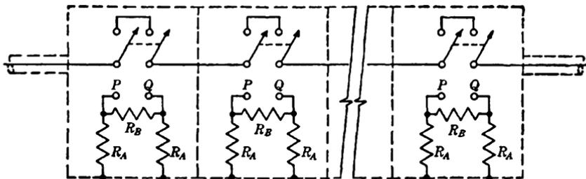
FIG. 8-9.—A 75-ohm attenuator. The accuracy of any section may be determined with a bridge by measuring the resistances from  $P$  to  $Q$  and from  $P$  and  $Q$  to ground with the switch in the out position. The values that should be obtained are shown in Table 8-1 together with the values of the individual resistors. For any other iterative impedance, multiply these values by the ratio of the new impedance to 75 ohms.
