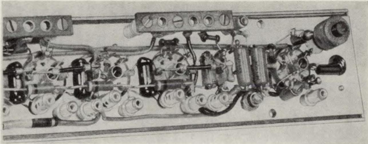
FIG. 6-20.—High-frequency inverse-feedback amplifier.
