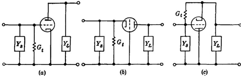
FIG. 13-5.—Alternative connections of first tube.
