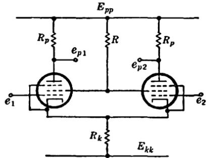
FIG. 11-31.—Pentode differential amplifier.
