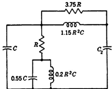
FIG. 2-8.—Four-terminal network designed for 1/1 capacity ratio.
