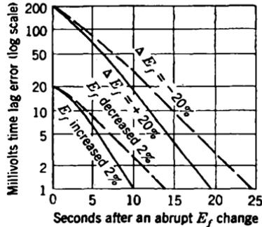
FIG. 11-8.—Heater-cathode time lag of a 6SL7.
