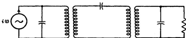
FIG. 1-6.—Network with three separable parts.
