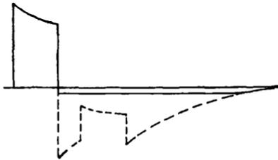
FIG. 3-13.—Loss of weak signal when clipping overshoot.
