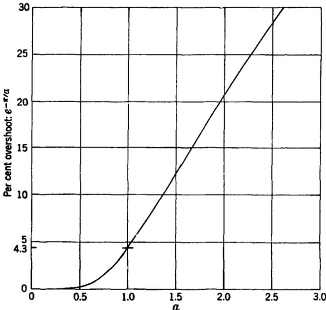
Fig. 7-3.—Overshoot of staggered pair as function of ratio  $a$  of separation of the resonant frequencies of the staggered circuits to their bandwidth. The value  $a = 1$  corresponds to a flat staggered pair. The curve also applies to double-tuned circuits if  $a$  is suitably interpreted:
