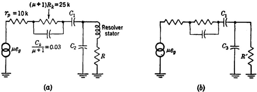
FIG. B-2.—Equivalent circuits of output stage.  $R'$  = apparent resistance of parallel-resonant circuit.  $C_3$  = excess of  $C_3$  over value required for resonant tuning. (a) Equivalent circuit of output stage; (b) simplified equivalent circuit if stator is tuned capacitatively.
