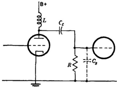
FIG. 3-10.—Choke-coupling circuit.
