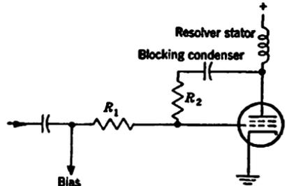
FIG. 9-11.—Single-stage driver with plate-to-grid feedback.
