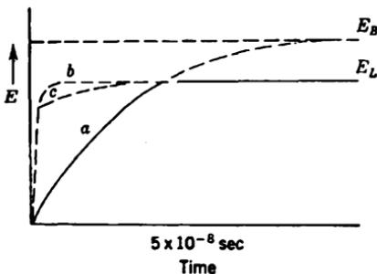
FIG. 8-7.—Shape of voltage rise at the  $V_4, V_5$  junction. (a) Without compensating condensers  $C_{10}$  and  $C_{11}$ ; (b) compensating condensers set correctly; (c) compensating condensers too small.  $E_L$  is the voltage at which the grid of  $V_7$  starts to draw current.
