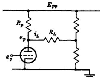
FIG. 11-32.—Plate as output terminal.
