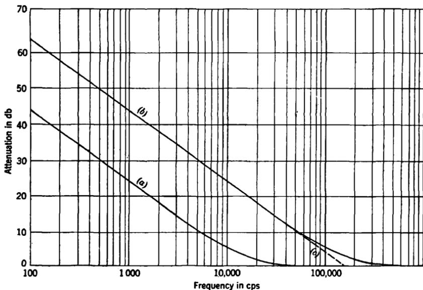
FIG. 3-30.—Attenuation vs. frequency for microphonic rejection circuits. (a)  $RC$ -circuit,  $T = 10 \mu\text{sec}$ ; (b)  $RC$ -circuit,  $T = 1 \mu\text{sec}$ ; (c) delay line,  $t_d = 1 \mu\text{sec}$ .
