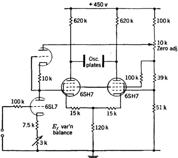
FIG. 11-67.—Two-stage voltage amplifier for oscilloscope deflection.
