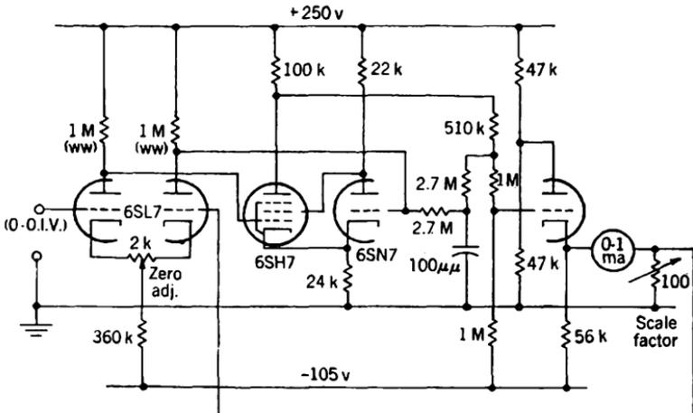
FIG. 11-63.—Voltmeter using high-gain amplifier.
