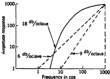
FIG. 9-3.—Low-frequency asymptotic characteristics. Solid line represents possible asymptotic characteristic for a three-stage amplifier.
