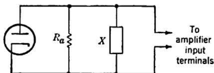
FIG. 14.4.—High-impedance diode noise generator.
