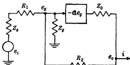
FIG. 9-2.—Schematic circuit for resistive-mixing feedback.
