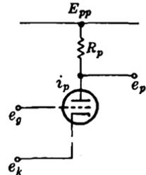
FIG. 11-24.—Triode with two input terminals.
