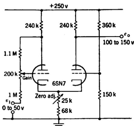
FIG. 11-70.—Differential amplifier arranged as a level shifter.
