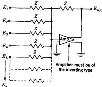
FIG. 2-29.—Feedback-amplifier mixer.
