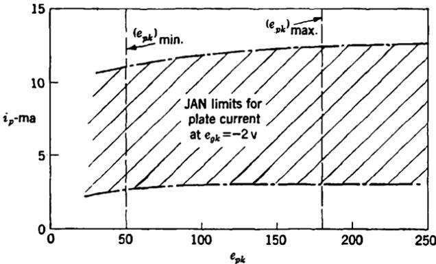
FIG. 9-16.—Type 6AK5 characteristic with tolerances.
