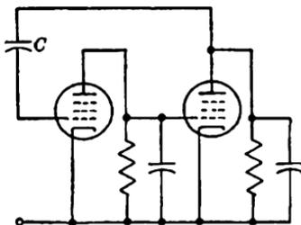
FIG. 2-15.—Negative-capacity circuit.
