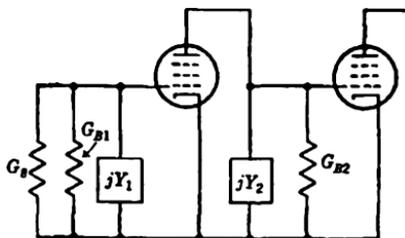
FIG. 13-9.—Grounded-cathode-pentode input circuit.
