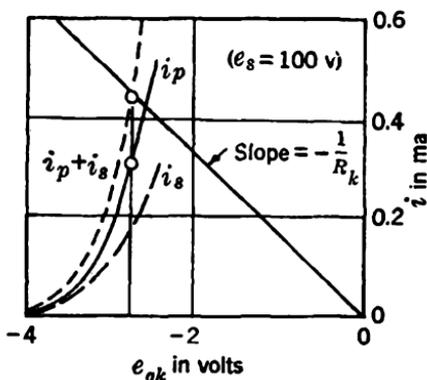
FIG. 11-74.—Determination of constant-current pentode current.
