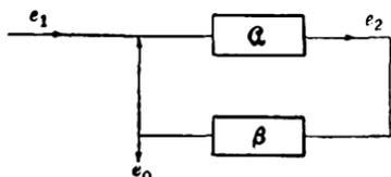
FIG. 10-7.—Block diagram of rejection amplifier.
