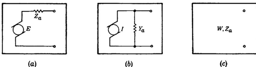
FIG. 14·1.—Three representations of a generator.
