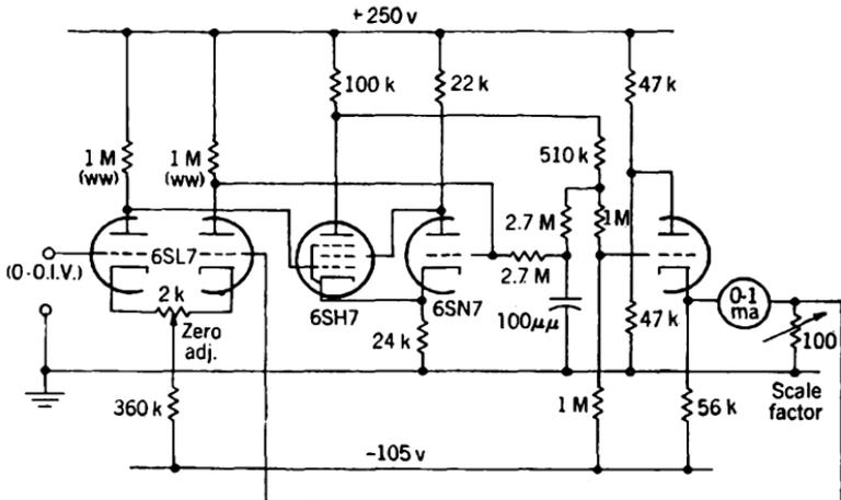
FIG. 11-63.—Voltmeter using high-gain amplifier.
