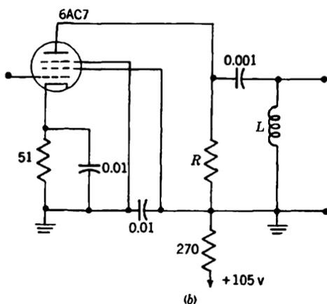
FIG. 4-12.—(a) Block diagram of nine-stage 80-db 6AC7 flat-staggered triple amplifier covering the band 8.25 to 24.75 Mc/sec. (b) Typical stage. Apart from the values of  $R$  and  $L$  the various amplifier stages have the same constants.
