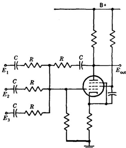
FIG. 2-31.—Typical three-channel feedback-amplifier mixer.
