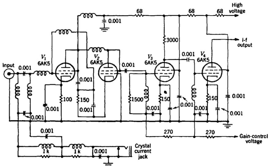
FIG. 13-13. Circuit diagram of practical grounded-cathode-triode-grounded-grid-triode input amplifier.
