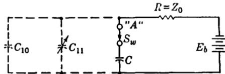
FIG. 8-6.—Equivalent circuit of delay line after firing of  $V_4$ . Before the firing of  $V_4$ , represented by the switch  $Sw$ , the voltage across  $C$  is zero and the voltage across  $C_{10}$  and  $C_{11}$  is the supply voltage  $E_b$ . When  $Sw$  is closed, the charge on  $C_{10}$  and  $C_{11}$  is rapidly redistributed and shared by  $C$ .
