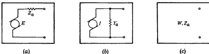
FIG. 14·1.—Three representations of a generator.
