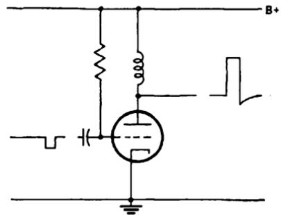
FIG. 3-29.—High-output voltage circuit.
