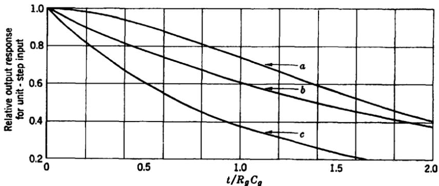
FIG. 2-19.—Flat-top compensation for  $R_o C_o$  with  $R_d C_d$ . Curves (a) and (b) for the case  $R_d = R_i$ . (a)  $R_i C_d = R_o C_o$ ; (b)  $[R_i R_d / (R_i + R_d)] C_d = R_o C_o$ ; (c)  $R_d = 0$ .
