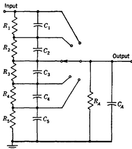
$$R_1 C_1 = R_2 C_2 = R_3 C_3 = R_4 C_4 = R_5 C_5 = R_A C_A$$
