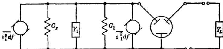
FIG. 13-2.—Equivalent circuit for input network.
