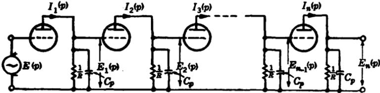
FIG. 1-24.—The  $n$ -stage RC-coupled pulse amplifier transform.
