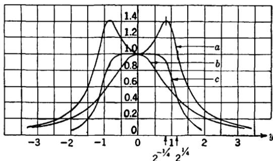
FIG. 5-8.—Stagger-damped pair (a)  $1/\sqrt{1 - y^2 \sqrt{2} + y^4}$ ; (b)  $1/\sqrt{1 + y^2 \sqrt{2} + y^4}$ ; (c)  $1/\sqrt{1 + y^8}$ . (a) and (b) are the component selectivity curves of a stagger-damped pair; (c) is the over-all result.
