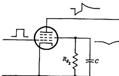
FIG. 3-4.—Screen bypass circuit.
