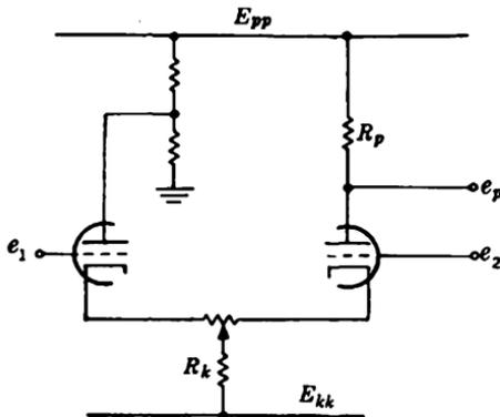
FIG. 11·27.—Method of zero adjustment.
