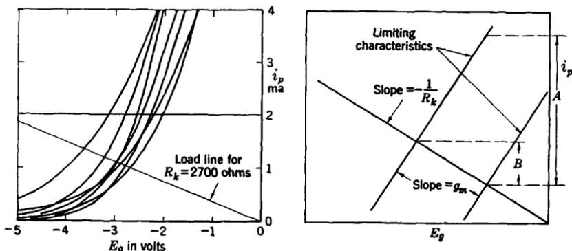
FIG. 9-18.—Stabilization of plate current by cathode resistor. (a) Mutual characteristics of several type 6AK5's,  $E_p = E_s = 90'$ ,  $E_f = 6.3'$ , four different manufacturers; (b) idealized characteristics, A = spread of  $i_p$ , with fixed bias, B = spread of  $i_p$ , with cathode bias.
