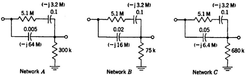
FIG. 9-33.—Low-frequency stabilization networks with reactances at 0.5 cps.
