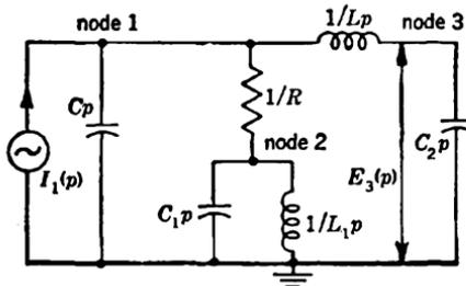
FIG. 1-27.—Transform of the network of Fig. 1-26.
