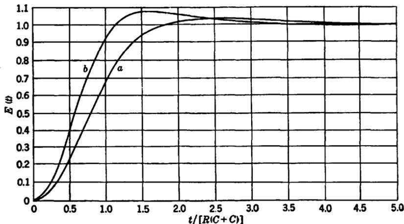
FIG. 2-11.—Response to current step function of series shunt-peaked circuit shown in Fig. 2-10. (a)  $C_1 = C$ ; (b)  $C_1 = C/2$ .
