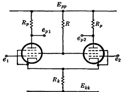
FIG. 11-31.—Pentode differential amplifier.
