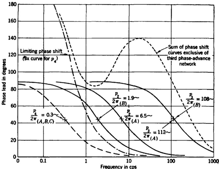
FIG. 9-31.—Phase characteristics for two stabilization networks.
