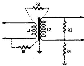
Fig. 606. Possible leakage paths in a transformer.
