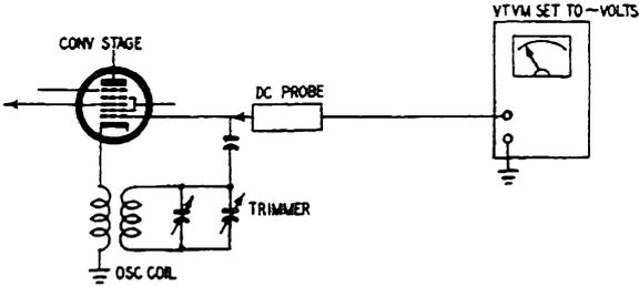
Fig. 705. Test setup for checking the local oscillator.
