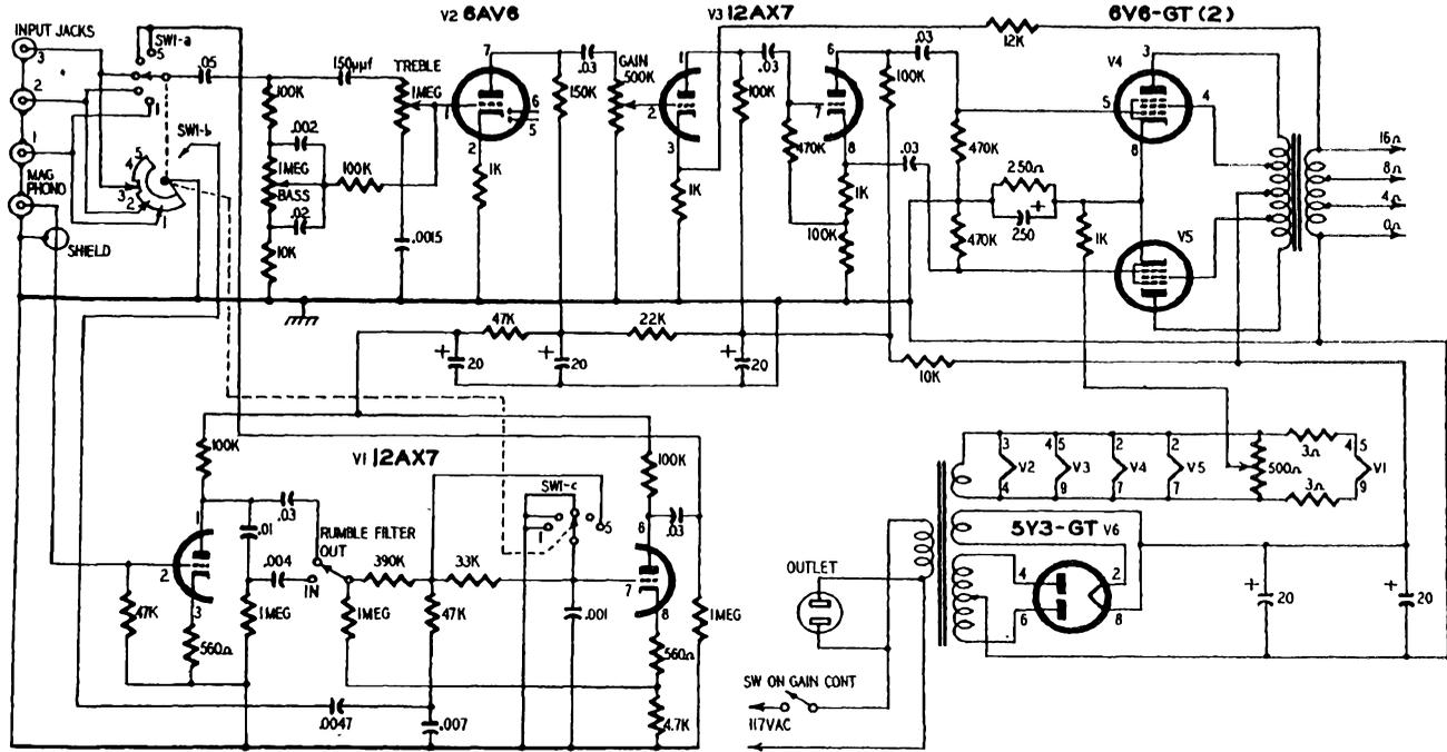
Fig. 801. Representative circuit diagram of a high-fidelity amplifier. The v.t.u.m. can be used to service the amplifier (in the event of component failure) or can be used to get optimum performance. For servicing and maintenance of such units the v.t.u.m. is practically indispensable. Checking techniques are described in the text.
