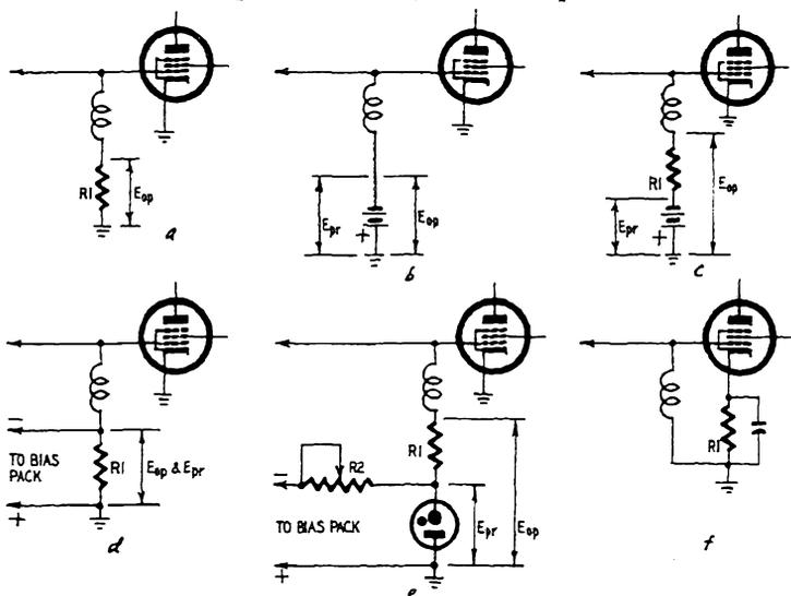
Fig. 903-a to f. Bias arrangements for transmitter tubes. Circuit a uses grid-leak bias while in circuit b could represent a bias (power supply) pack. Circuit c uses a combination of the types shown in a and b. In circuit d,  $R_1$  is the bleeder across the bias pack. Circuit e has the advantage of using a gas-tube regulator across the bias pack output. Bias is developed across the cathode resistor,  $R_1$ , in circuit f.
