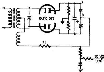
Fig. 713. Ratio-detector circuit.
