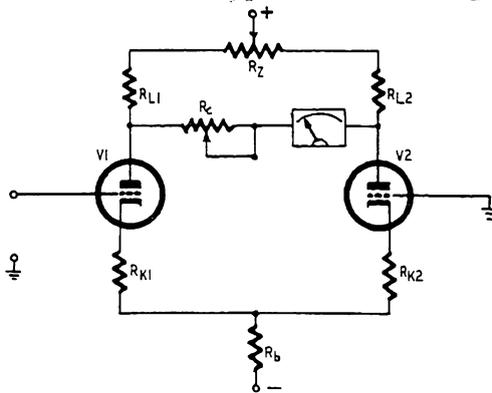
*Fig. 202. Bridge circuit used in a modern v.t.v.m. Although separate tubes are shown here, twin triodes (with independent cathodes) are generally used.*
