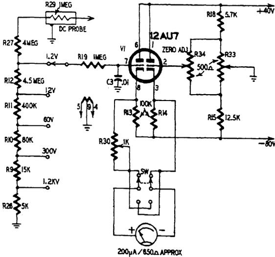
Fig. 1106. D.c. voltage measuring section of the v.t.v.m.
