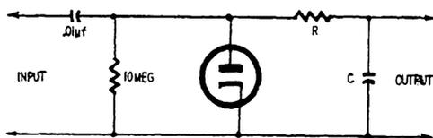
Fig. 406. Circuit of a vacuum-tube rectifying probe.
