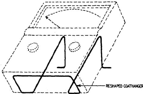
Fig. 1025. *Convenient mounting stand for the v.t.v.m.*
