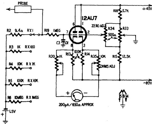
Fig. 1108. Resistance measuring circuit of the v.t.v.m.
