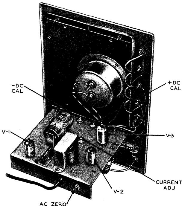
Fig. 1111. View of the interior of a v.t.u.m. Voltage and current calibration adjustments are easily available, can easily be made with a screwdriver. The battery (used for ohms measurements) is clamped into place, but a new unit can be readily substituted.
