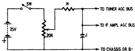
Fig. 608. Circuit of an external bias supply.
