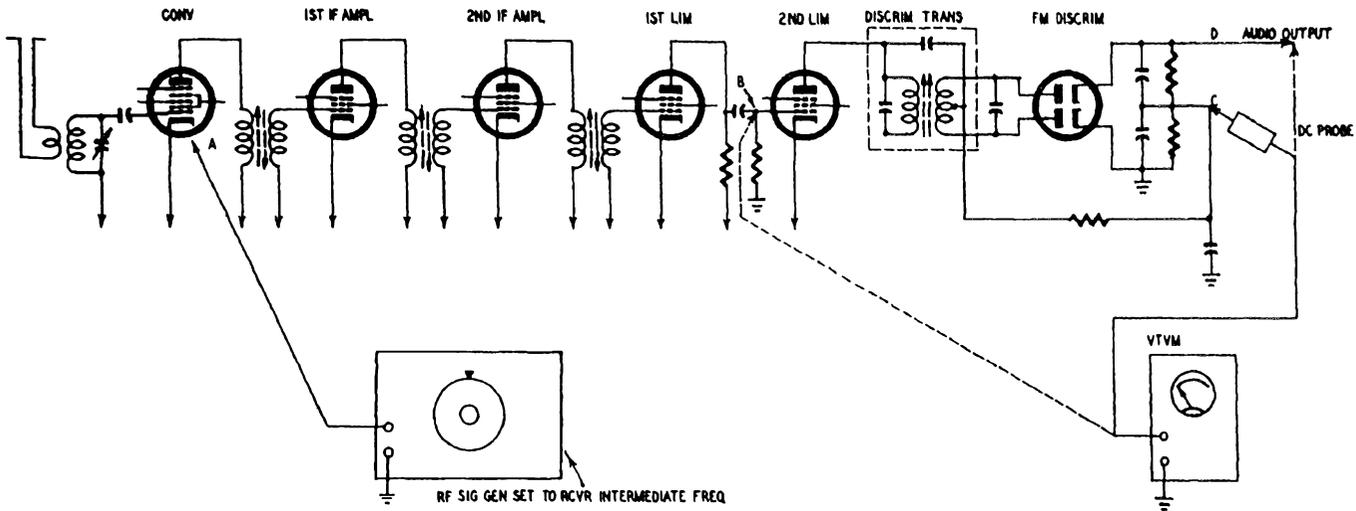
Fig. 712. Simplified circuit diagram of FM receiver using two limiter stages and discriminator-type detector. This arrangement is gradually being replaced by FM sets using ratio detectors. Such receivers do not ordinarily have limiter circuits. Various test points are shown in the FM circuit above. The audio stages have been eliminated since these are checked in the same manner for all receivers.
