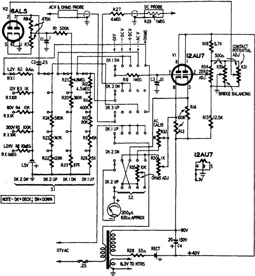
Fig. 1105. Complete diagram of a vacuum-tube voltmeter. The circuit is analyzed in the text and in the illustrations which follow.
