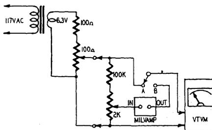
Fig. 1022. Calibration of the v.t.v.m. using the preamplifier.
