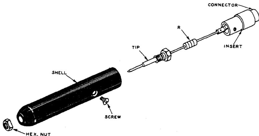
Fig. 403. Exploded view of a d.c. (or isolating) probe. The resistor,  $R$ , most often has a value of one megohm. The probe, held together by a single screw and hex nut, can easily be taken apart when repairs are needed.
