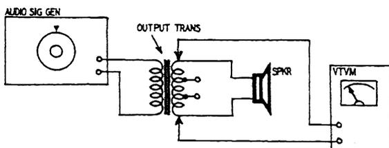
*Fig. 1005. Audio-output transformers are often supplied with multiple taps on the secondary. The v.t.v.m. can be used for finding the best impedance match between the voice coil of the speaker and the secondary winding. A listening test is not as conclusive as the method shown here.*
