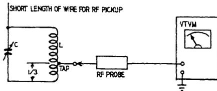
Fig. 906. The v.t.v.m. can be used as a field-strength meter.
