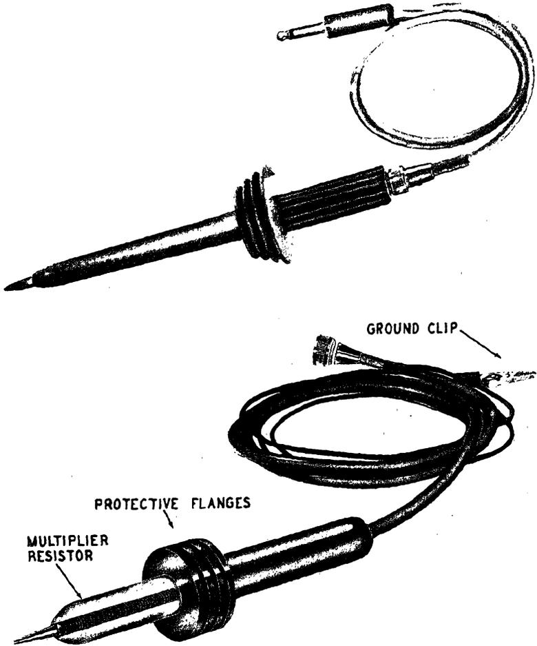
Fig. 412. Two types of high-voltage probes. These are used to extend the d.c. range of the v.t.v.m., should not be used for the measurement of a.c. voltages.
