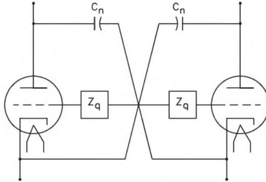
**Figure 3.49** Circuit of grounded-grid amplifier having grid impedance and neutralized for reactive currents.
