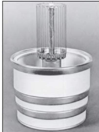
**Figure 3.26** Bar-type tungsten filament.
