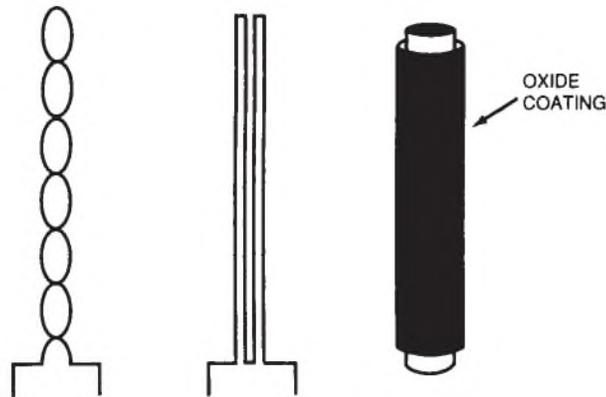
**Figure 3.2** Common types of heater and cathode structures. (From [2]. Used with permission.)
