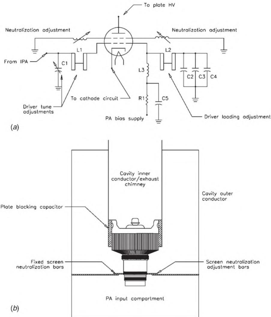
**Figure 3.48** A grounded-screen PA stage neutralized through the use of stray inductance between the screen connector and the cavity deck: (a) schematic diagram, (b) mechanical layout of cavity.
