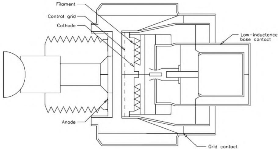
**Figure 3.10** Internal configuration of a planar triode.
