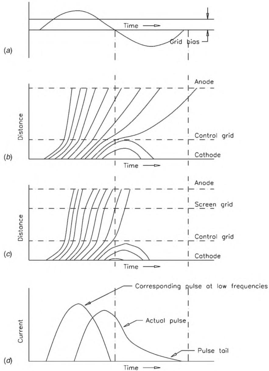
**Figure 3.18** Transit-time effects in a class C amplifier: (a) control grid voltage, (b) electron position as a function of time (triode case), (c) electron position as a function of time (tetrode case), (d) plate current (triode case).
