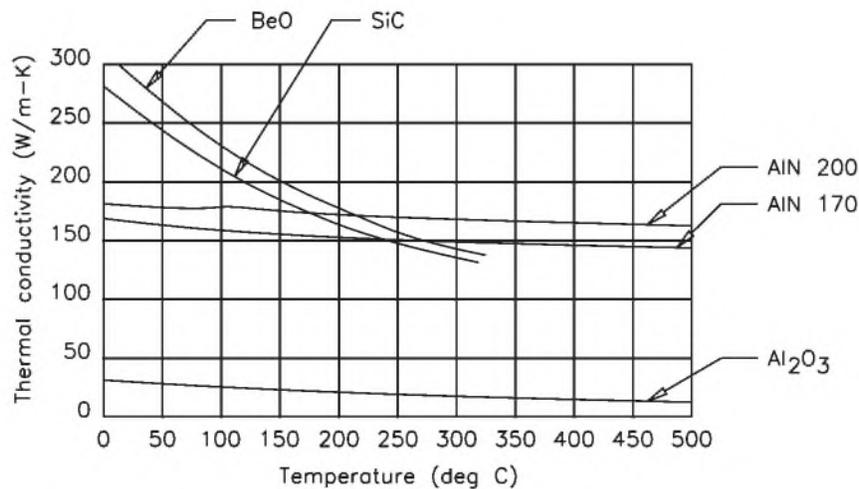
**Figure 3.37** Thermal conductivity of common ceramics.
