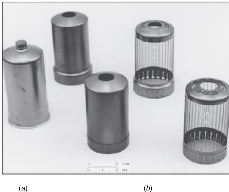
**Figure 3.29** Pyrolytic graphite grid: (a) before laser processing, (b) completed assembly. (Courtesy of Varian.)
