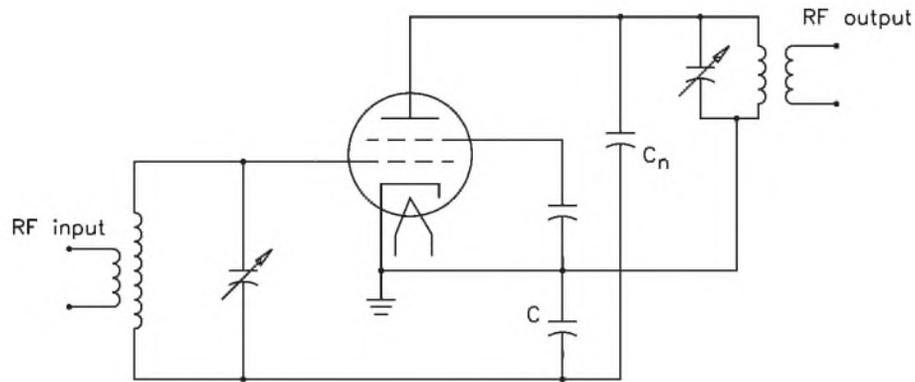
**Figure 3.44** Single-ended grid neutralization for a tetrode.
