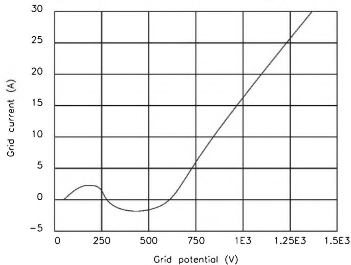
**Figure 3.34** Typical curve of grid current as a function of control grid voltage for a high-power thoriaed-tungsten filament tetrode.
