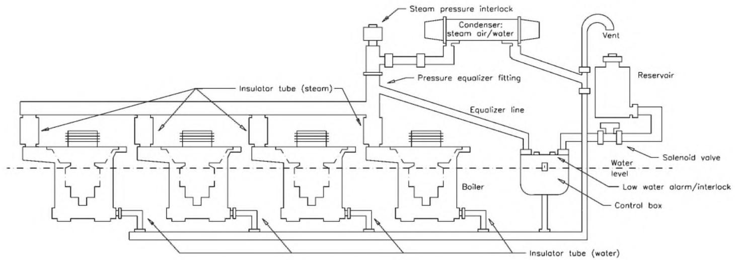
**Figure 3.23** Vapor-phase cooling system for a 4-tube transmitter using a common water supply.
