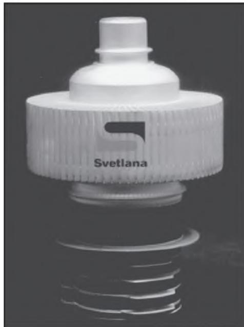
**Figure 3.14** 5CX1500B power pentode device.
