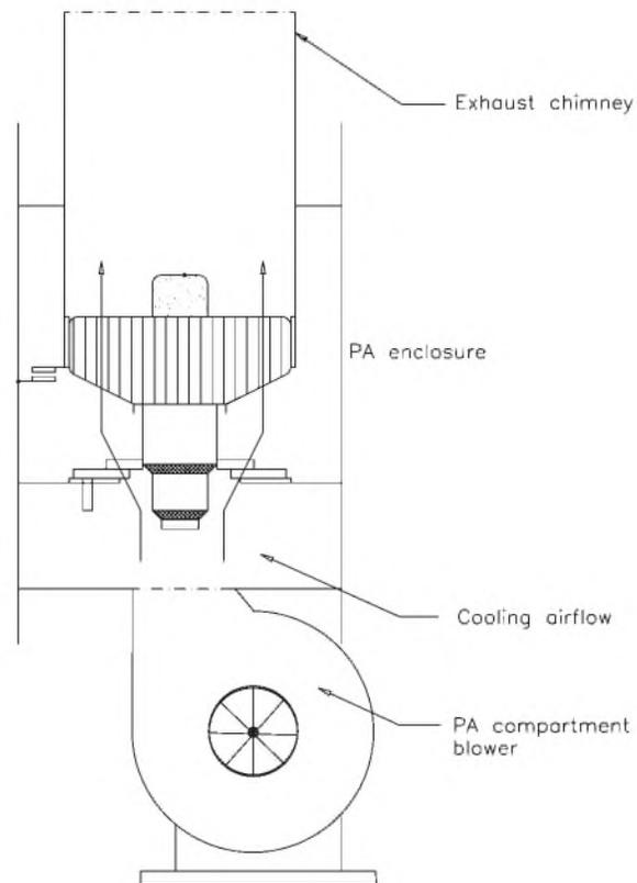
**Figure 3.20** A typical transmitter PA stage cooling system.
