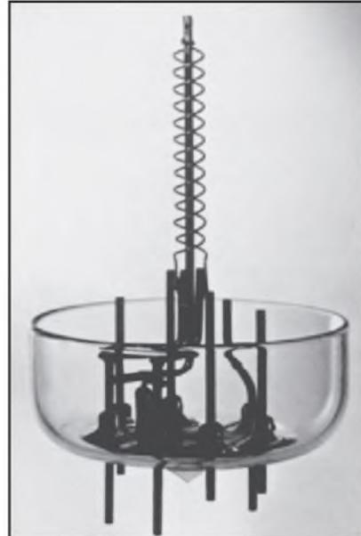
**Figure 3.25** Spiral-type tungsten filament.
