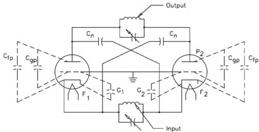
**Figure 3.42** Symmetrical stage neutralization for a grounded-grid circuit.
