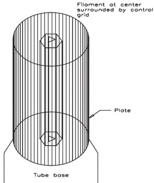
**Figure 3.6** Mechanical configuration of a power triode.
