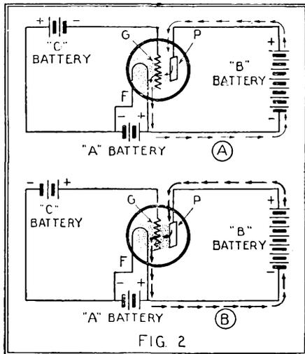
Illustrating the effects of a positive and a negative "C" battery voltages on the grid of a vacuum tube. When the voltage is negative, as shown at A, the "B" current flow is low, as the flow of electrons to the plate is greatly reduced. When the grid voltage is positive, however, as shown at B, the electron stream is increased and consequently the flow of "B" current is greater. This explains why the use of a "C" battery lengthens the life of "B" batteries.
