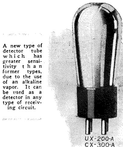
A new type of detector tube which has greater sensitivity than former types, due to the use of an alkaline vapor. It can be used as a detector in any type of receiving circuit.
