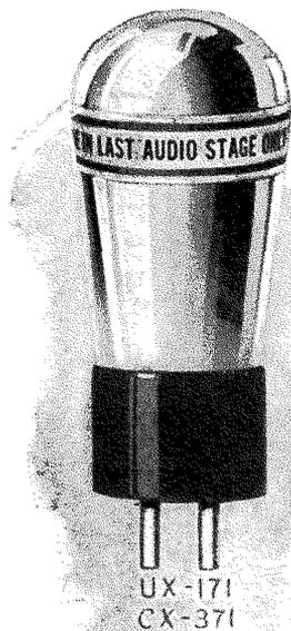
A new storage-battery type power amplifier tube, for use in the last stage audio amplifier only. This tube takes the same filament voltage and filament current as the No. 112 tube shown above, but employs a "B" voltage of 180 and a 40½-volt "C" battery. Special means should be provided for handling its heavy output. Two arrangements are shown in Fig. 6.
