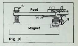
its position owing to the pull of the permanent magnet. The Disc adjustment may not be sufficient to overcome this, and a slight turn of the adjusting screw towards "Open" will be necessary, but is should be realised, of course, that a fresh adjustment of the Disc may be needed.
