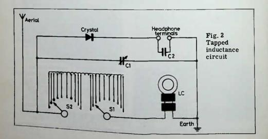
by the rotating arms S1, S2. The loading coil LC was used when receiving long wave and was a plug-in type No. 150 or 200. The loading coil was sometimes short circuited, by the means of a switch, when receiving the ordinary broadcast band. Condenser C2.002 $\mu$ F. across the headphones, was a by-pass for any high frequency pulsations of current.
