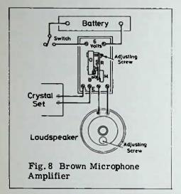
poles could be worked to the reed without actually touching, the greater the magnification obtained from the instrument.
