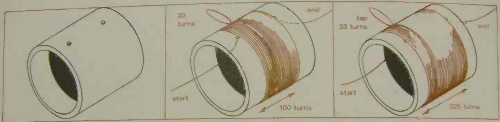
1. Find a card postal tube as near as you can to 25 mm (1") diameter and cut off a 2" length. Pierce two small holes in line, as shown, about 25 mm (1") apart.
