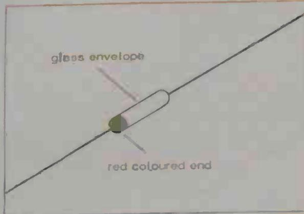
4. A DIODE is a tiny cylindrical-shaped component with a glass body, usually with rounded ends. A thin wire emerges from each end (the connecting leads). One end of the diode is marked + or coloured red.
