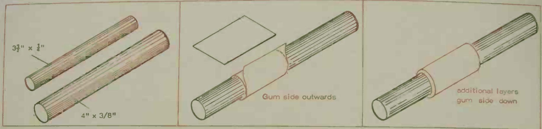
1. Two standard diameter sizes of Ferrite rod are shown. You can use either for making a *ferrite rod aerial*. Cut to length with a hacksaw, or mark with a sharp file and break off.
