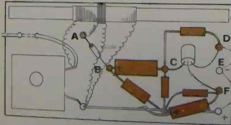
This circuit is the same as that on page 18, with *capacity coupling* between terminals B and C and the addition of several more components in the *transistor amplifier* stage; intended to 'fix' and stabilise the working point of the transistor. This should give more consistent results.
