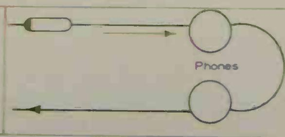
5. If this electrical signal from the diode is passed through high impedance earphones it can be heard—provided the aerial circuit has done its job and produced enough magnification of the signal.
