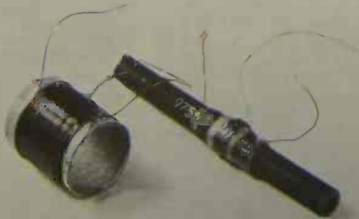
Air-cored coils are not as efficient as ferrite rod aeriels, but they are cheaper to make. You can wind these coils on card tube formers—or even a length of hardwood or balsa dowel. Coil diameter should be 25 mm (1")—not smaller. You can use a larger coil former (in which case reduce the number of turns), but this produces a more cumbersome coil. The size shown in the illustrations matches a 500 pF tuning capacitor.
