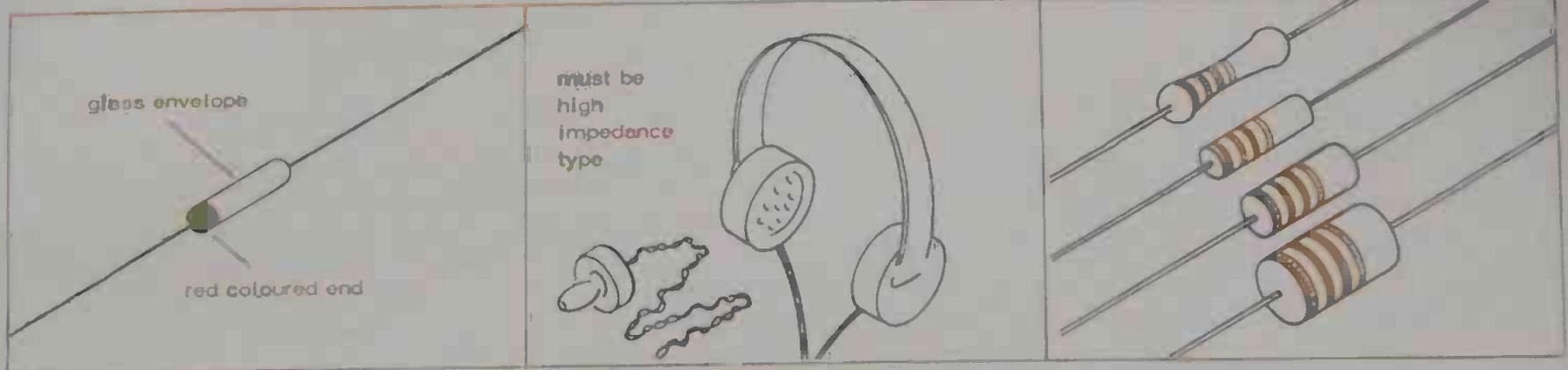
4. A DIODE is a tiny cylindrical-shaped component with a glass body, usually with rounded ends. A thin wire emerges from each end (the connecting leads). One end of the diode is marked + or coloured red.
