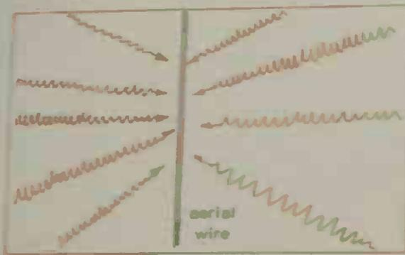
1. The air is full of radio signals transmitted from broadcast stations all over the world. These signals vary a lot in strength, as well as wavelength (or frequency). But each signal received will induce a very, very tiny signal in a length of wire, or aerial.
