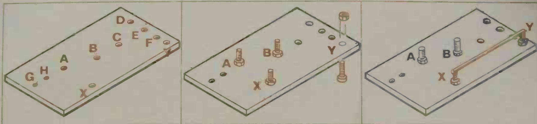
4. Use a 3 mm drill to drill holes A, B, C, D, E and F. Use the same drill to drill holes X and Y. Then change to a  $\frac{1}{16}$ " drill to drill holes G and H.
