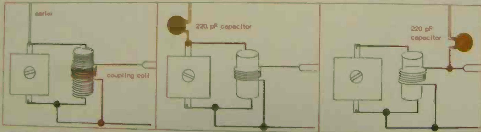
This type of aerial coil, with an overwound coupling coil, will often work better than a single coil with a tapping point. Adjust coupling coil position up or down for best results.
