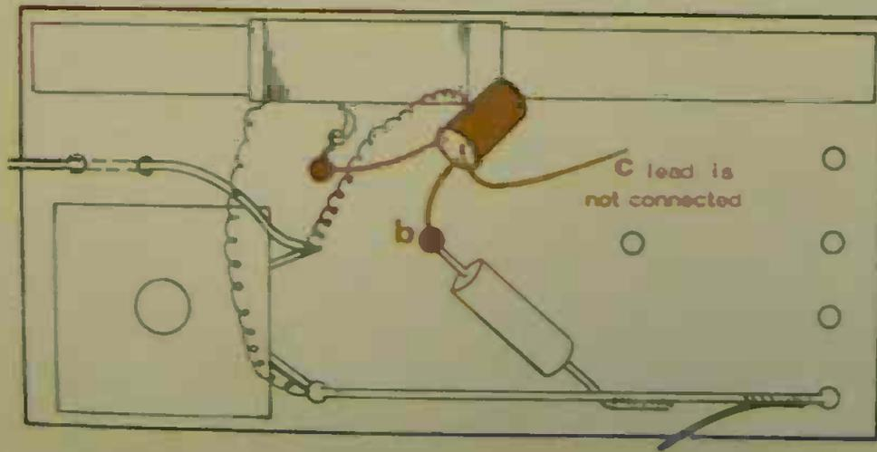
A transistor can work like a diode, using just two of its connections—the (e) or emitter and (b) or base leads. The diagram opposite shows the complete circuit—the same as on pages 12/13 with a transistor used instead of a diode. The unused (c) lead of the transistor is twisted out of the way.
