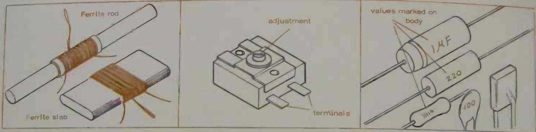
1. **TUNING COILS** consist of fine enamelled wire wound many times round a **FERRITE ROD** or **FERRITE SLAB**. You can buy these ready-made, or wind tuning coils yourself (see pages 8 and 9).
