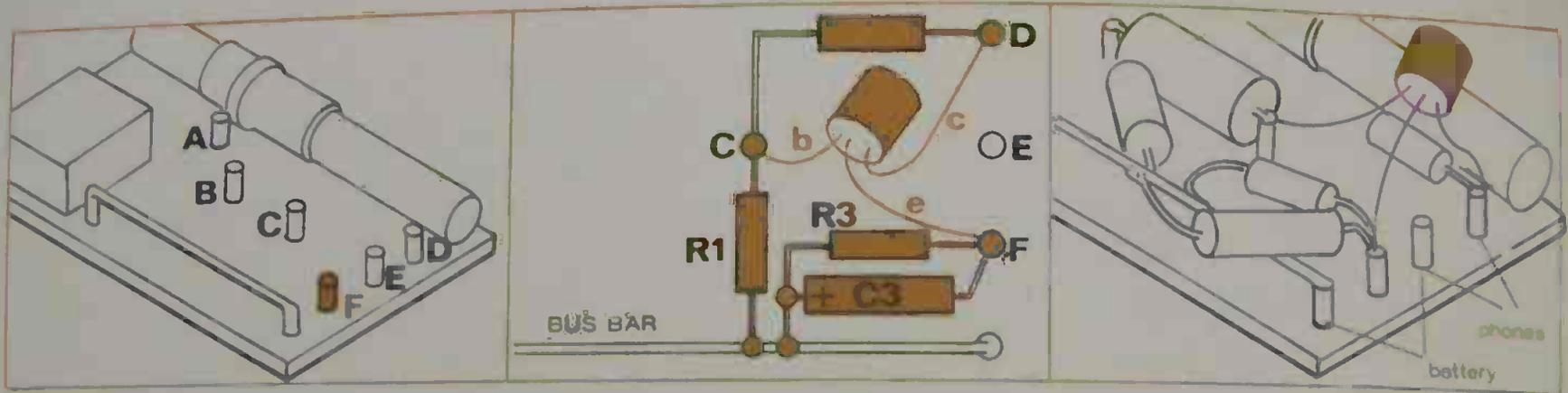
1. The circuit panel is made up as previously, but with the hole not used (F) also fitted with a 6BA terminal screw. There are now six terminal points, A, B, C, D, E and F.
