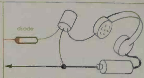
9. Using a diode as the detector, followed by a transistor for amplification of the 'sound signal', even better results can be obtained, because the transistor can be selected to work best with 'sound wave' frequencies. Again a battery is required.
