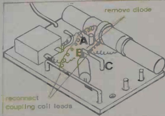
4. Remove the diode and disconnect the coupling coil leads taken to terminal A in the circuit on page 18. Reconnect this coupling coil lead to terminal B. This completes the modification to the 'front end' of the circuit.
