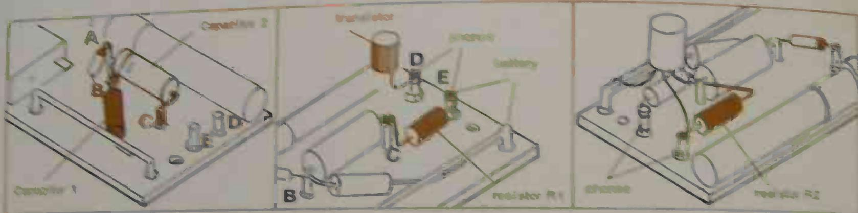
1. Assemble the panel with terminals A, B, C, D and E. Connect diode between terminals A and B (+ to A), capacitor 1 between terminals B and C (+ end towards B),
