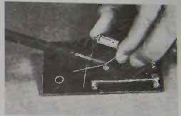
4. Technique for soldering 'bus bar' and component leads in place. Hold iron in place to heat up joint, then touch with solder, which should melt and run freely to complete joint.
