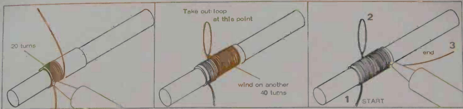
4. Secure the end of the 38s.w.g. wire with a dab of adhesive, leaving about 3" free. Then carefully wind 20 turns on to the paper sleeve, each turn tight up against the one before it.
