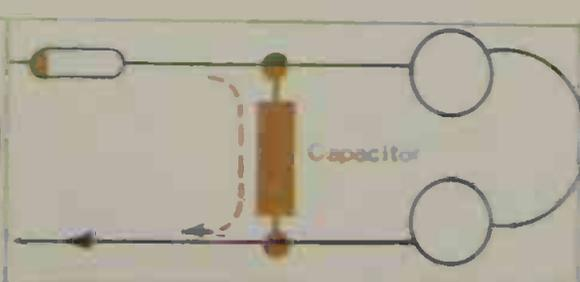
6. To improve the 'listening signal' a capacitor connected across the phones by-passes any stray 'radio' signal which has got past the diode. This makes the 'listening signal' easier to hear.
