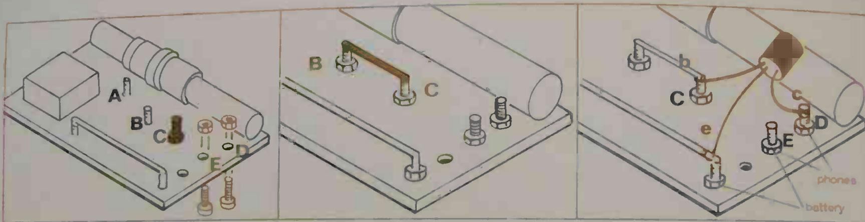
1. To accommodate the additional transistor circuit, three more terminal points are required on the panel. These are provided by fitting 6BA screws in holes C, D and E. Secure with nuts.
