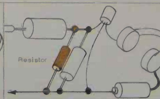
12. Finally, as well as a capacitor by-passing stray radio frequencies and 'noise' to the return, a resistor connected in parallel with the capacitor can further improve reception.
