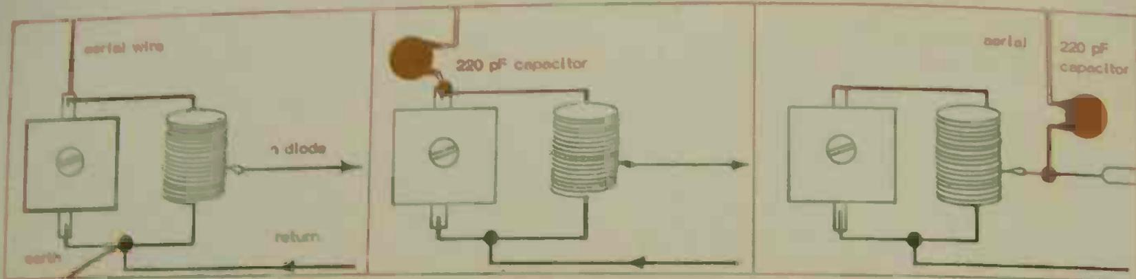
The point at which the aerial coil is tapped to feed the diode detector has an important effect. For best results, this should be towards the return line or 'earth' side of the circuit.
