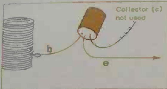
7. A transistor can work as a detector, just like a diode, using only the b (base) and e (emitter) connections. In such cases the 'sound wave' content of the original radio signal is passed on in the form of a minute fluctuating direct current.
