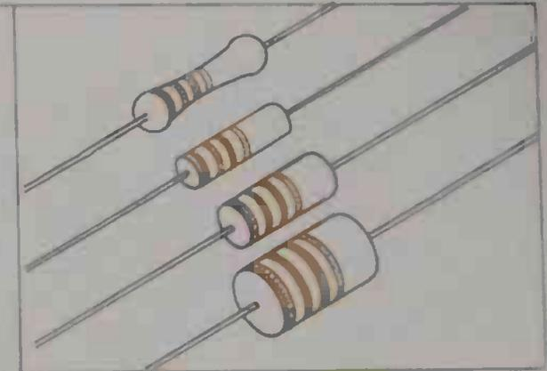
6. RESISTORS are another important component. They are usually cylindrical in shape with connecting leads emerging from each end. Resistor values are marked by coloured rings.
