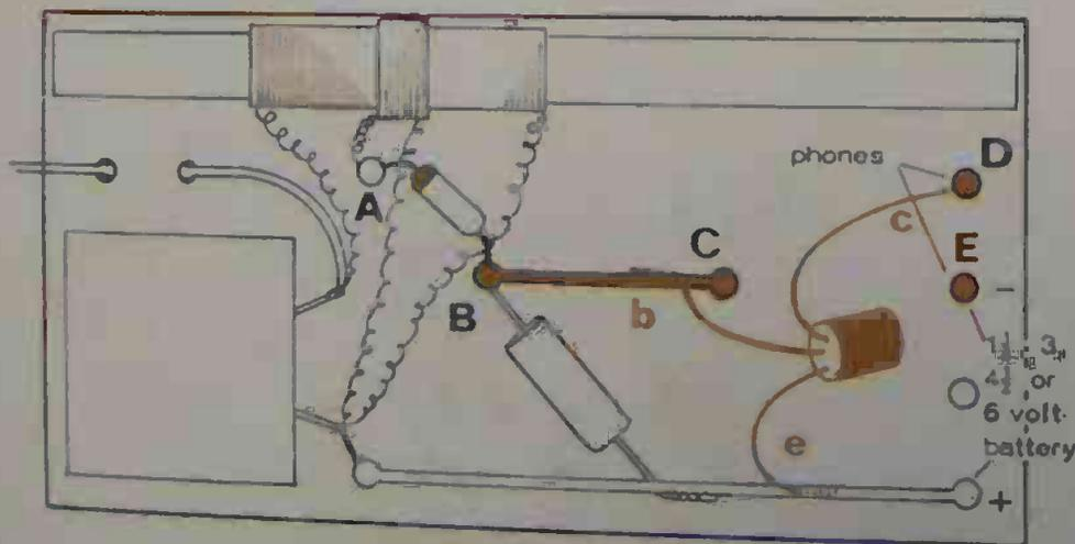
This circuit is a basic crystal set (with diode), with the addition of a transistor to work as an *amplifier* to boost the strength of the signal received (photograph, far right). This time all three leads to the transistor are connected and a battery is needed to power the transistor.
