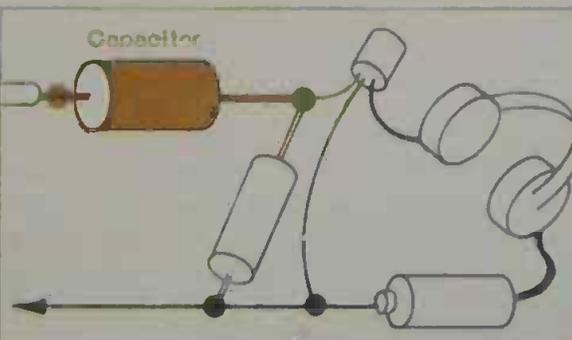
11. Another way of filtering out unwanted signal components is to connect the diode (detector) to the transistor (amplifier) via a capacitor. This usually improves signal quality.
