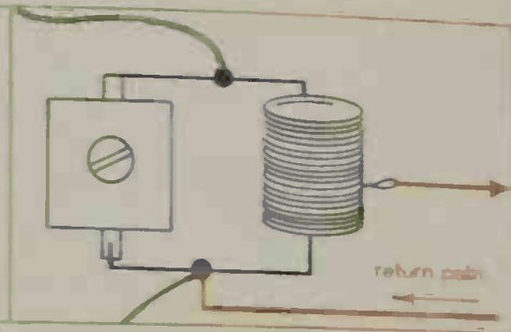
3. This means that when the aerial circuit is tuned to a particular frequency it can pass on a magnified signal at that frequency, whilst other signals received by the aerial are so weak that they become negligible by comparison.
