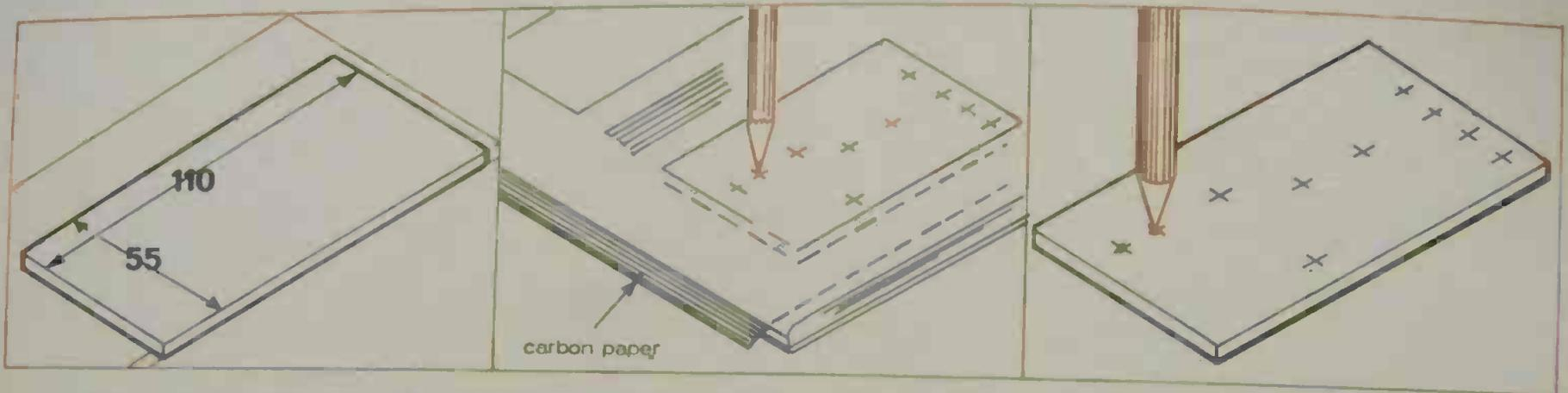
1. Mark out a rectangle 110 mm by 55 mm wide on a sheet of Paxolin and cut out carefully with a hacksaw. Smooth the edges with sandpaper, or a file.
