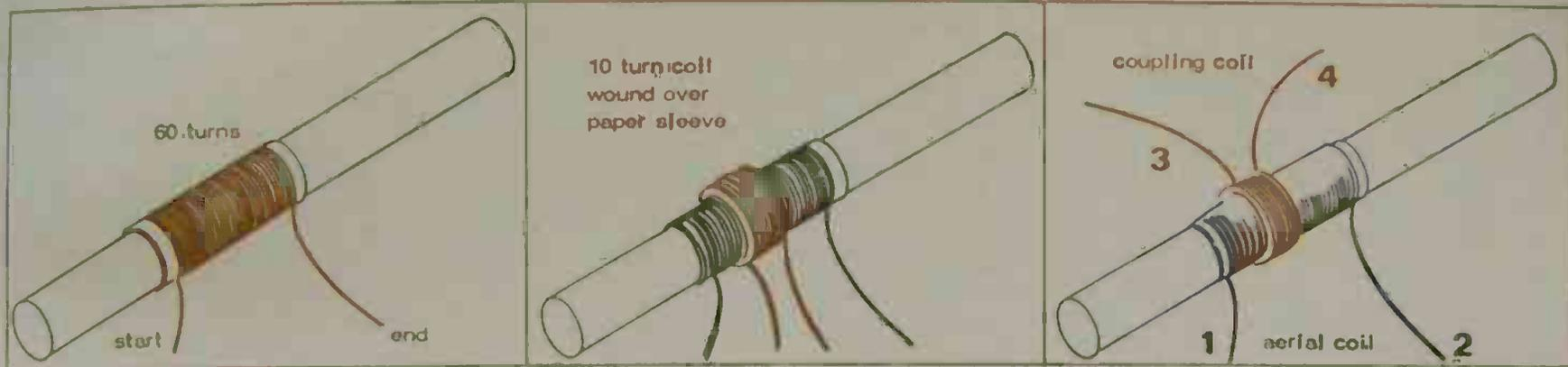
1. Make a paper sleeve to fit a ferrite rod, as on pages 8/9, and wind on a 60-turn coil of 38 s.w.g. wire with no tapping point. Secure the start and end with cement.
