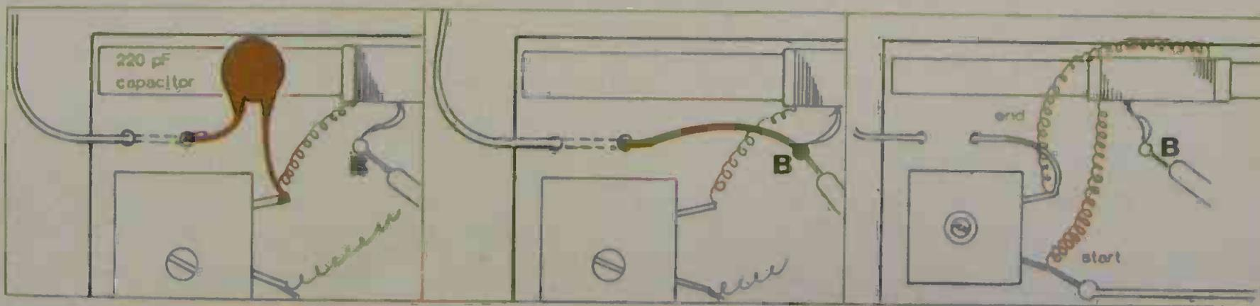
Here is a simple way of improving the efficiency of your aerial. Disconnect the aerial wire from the tuning capacitor terminal and solder to one lead of a 220 pF capacitor. Connect the other lead of this capacitor to the tuning capacitor terminal.
