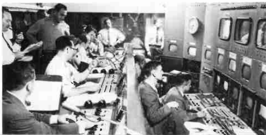
In one of NBC's TV studios, a single coordinator can view material picked up by various cameras and can switch from one to another to keep pace with developments. (Below)
