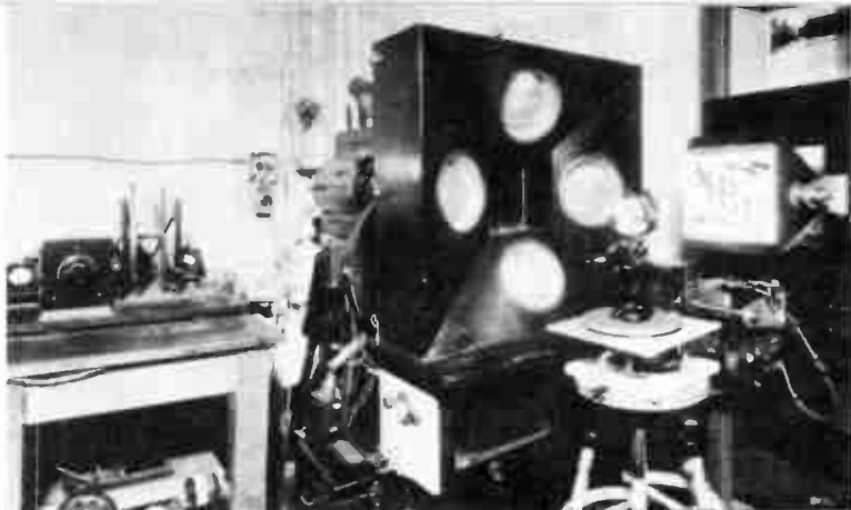
Felix the Cat made a television debut in the late twenties, whirling for hours on a hand-wound phonograph as engineers experimented with early pickup devices.
