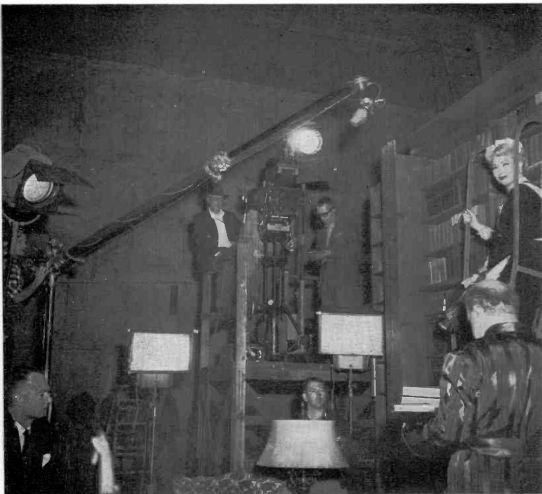
FIGURE 5. TV FILM TAKE. To take a high-angle shot, the camera has been placed on a platform. Lighting shown consists of two fill-lamps, center, and fresnel lamps, left and top, with "barn door" shutters. The boom mike can be moved from side to side, extended or retracted, and raised or lowered. (Photo courtesy of CBS Television)
