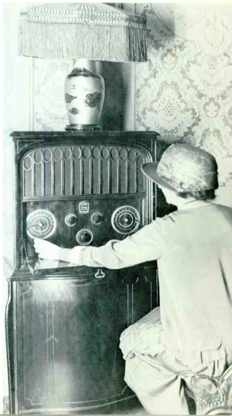
The "Radiola Super VIII," an RCA Super-Heterodyne receiver of 1925. This high-receptivity receiver revolutionized radio.
