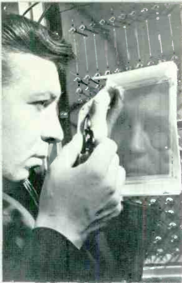
An RCA computer scientist inspects an experimental memory device which can store a quarter-million bits of information when immersed in liquid helium.
