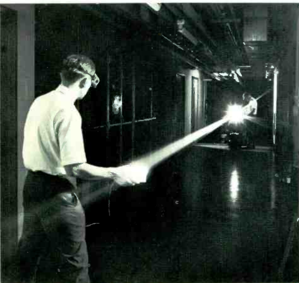
An argon gas laser built for the National Aeronautics and Space Administration to track space vehicles is tested at the David Sarnoff Research Center.
