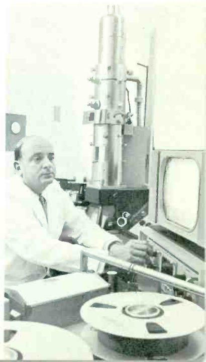
An electron microscope, used with a television set that displays the specimen under observation, is a key research tool at New York's Lenox Hill Hospital.
