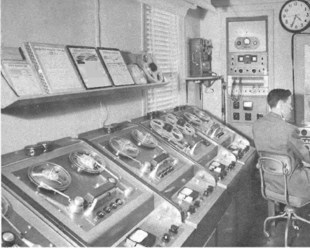
Mr. Herbert W. Armstrong broadcasts The WORLD TOMORROW from the modern studios of the campus at Ambassador College in Pasadena. Mr. Norman Smith sits at the controls. He directs the "dubbing" of hundreds of tape recordings on the precision Ampex recording equipment.
