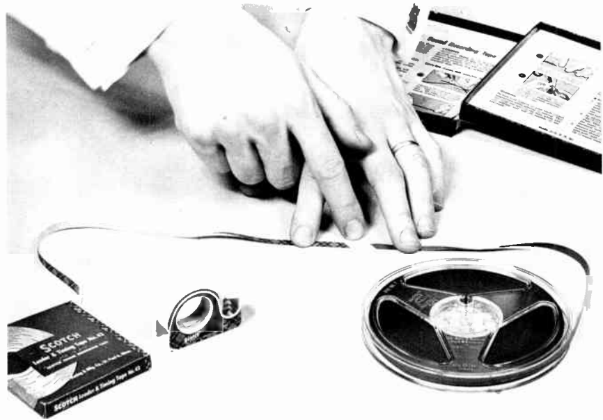
Figure 5-20 Attaching Leader to Recorded Tape Courtesy Minnesota Mining & Mfg. Co.
