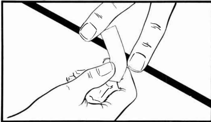
Figure 5-15 Applying the Splicing Tape Courtesy Minnesota Mining & Mfg. Co.
