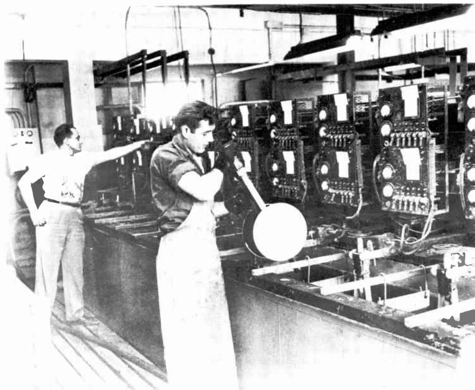
Figure 5-7 From Master To Mother To Stamper
