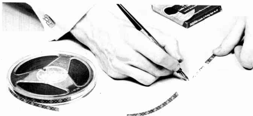
Figure 5-23 Marking Recording Information on Leader Courtesy Minnesota Mining & Mfg. Co.
