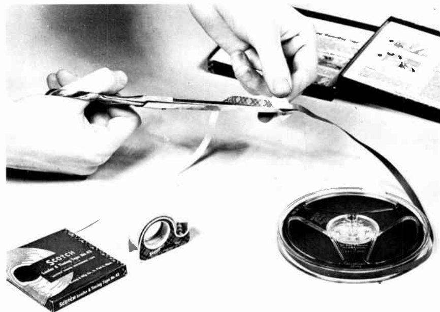
Figure 5-21 Trimming Off Excess Splicing Tape Courtesy Minnesota Mining & Mfg. Co.
