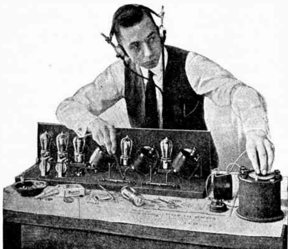
Fig. 71. Showing the Five Tube "Neutrodyne" Receiver Being Adjusted for Complete Neutralization.
