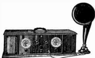
Fig. 77. Modern Super-Heterodyne Receiver Showing two Control Handles.
