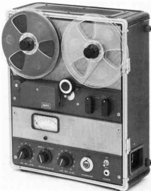
Fig. 6: Portable AC-operated broadcast-type tape recorder. Ampex 602.
