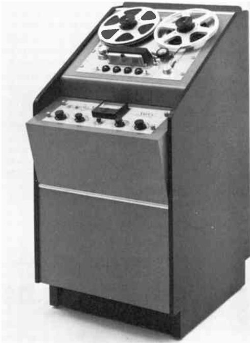
Fig. 5: Console-mounted tape recorder for studio use. Note large 10½" reels. Ampex 351.
