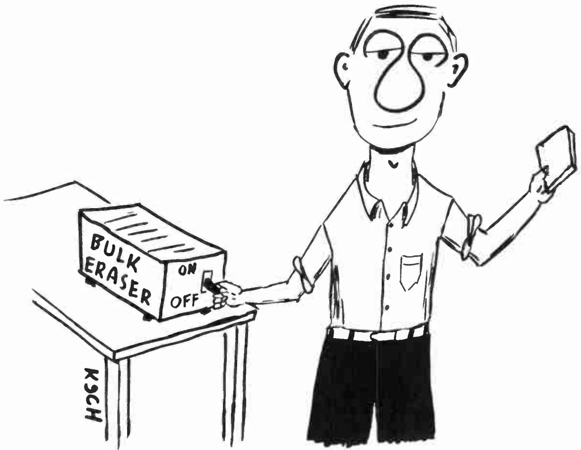
Fig. 2-11. Using bulk erasers. A bulk tape eraser can wipe out all program material on a cart, cassette, or reel of tape in a matter of seconds. Be sure to hold the tape away from the eraser while turning it on and off. It's also a good idea to keep other tapes, watches (both electronic and mechanical), and magnetic-striped credit cards away from the bulk eraser at all times.
