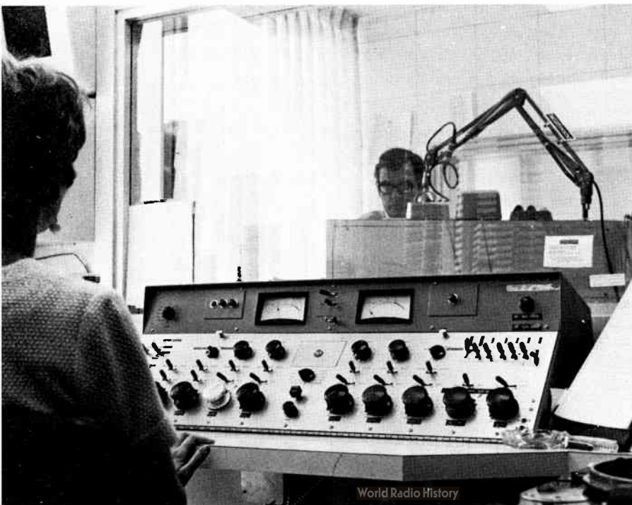
Figure 30. Control room and announce booth at KNBR-AM and FM , San Francisco. Announcer Dave Niles speaks into an RCA 77-DX ribbon microphone, while engineer Diane Smithem operates an RCA BC-7 console. (Courtesy KNBR )
