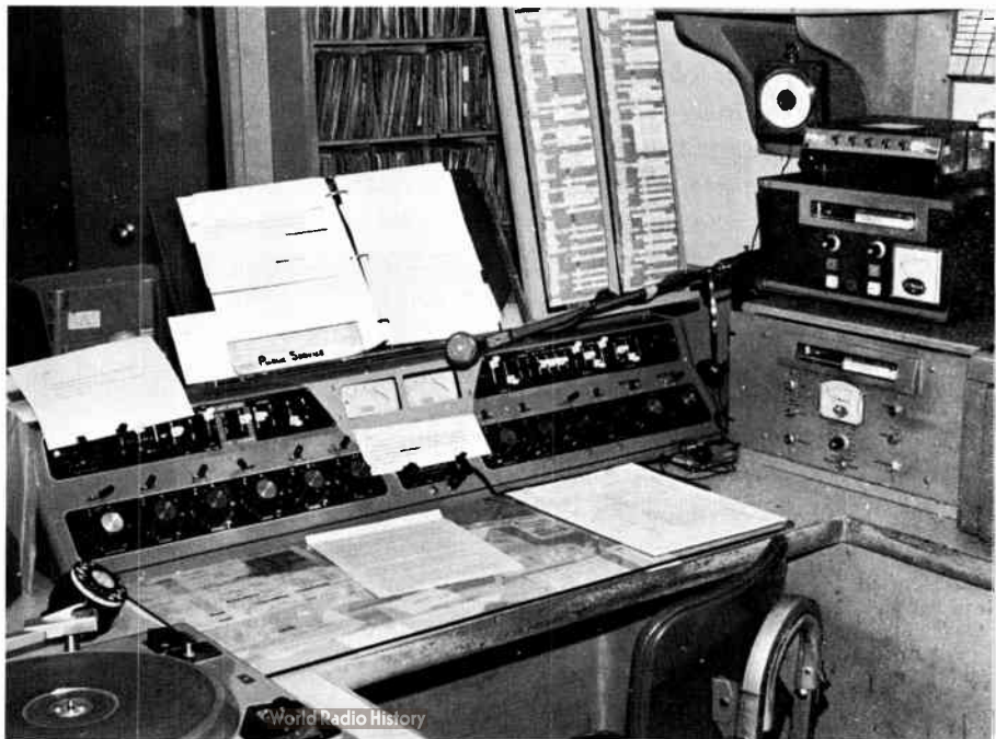
Figure 27. Typical control-room arrangement for combo operation. Equipment includes a Gates Dualux audio console, an E-V 665 dynamic microphone, a Gates turntable, and a Gates Spot Tape cartridge unit. (Courtesy KTIM-AM and FM, San Rafael, California)
