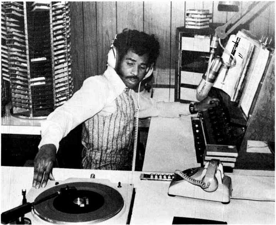
Figure 28. Combo operator at work. Tony King, disc jockey at KSOL-AM, San Francisco, operates a Sparta console, a QRK turntable, and an RCA 77-DX ribbon microphone. (Courtesy KSOL)
