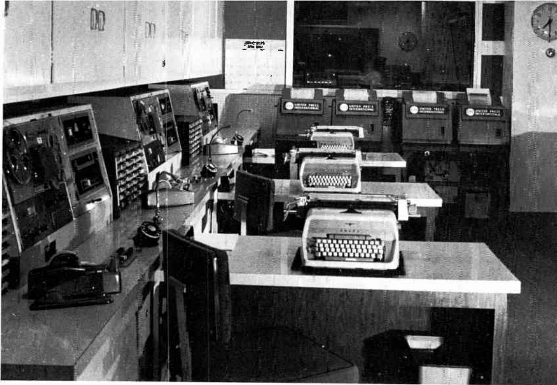
Figure 24. News “nests” at KNEW-AM, Oakland, California. Each nest includes tape and tape-cartridge machines, a microphone for recording news stories, telephone lines to receive reports from the field or to interview newsmakers, and a typewriter. (Courtesy KNEW)
