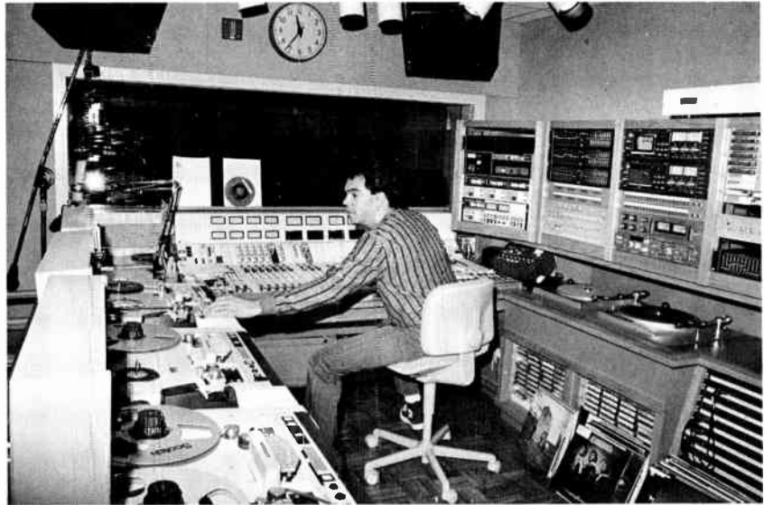
FIGURE 4.7 Production Director Albert Lord operates an ABX-34 production console, Technics turntables, Tomcat tape cart machines, Tascam cassette machines, Otari reel-to-reel tape recorders, and Sennheiser 441 microphones. (Courtesy Albert Lord and KFRC, San Francisco)
