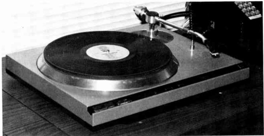
FIGURE 4.5 A Technics professional turntable and tone arm. (Courtesy KTIM, San Rafael, California)
