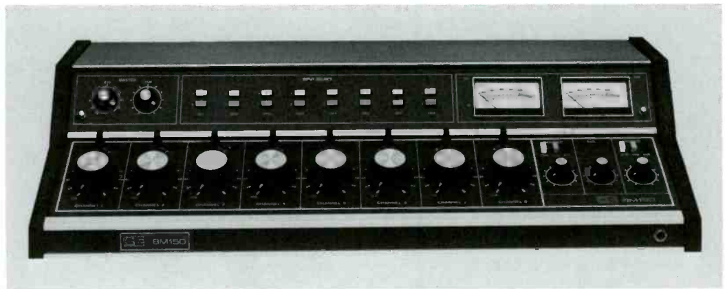
FIGURE 9.8 Eight-mixer ("pot") monaural console. Courtesy Broadcast Electronics.
