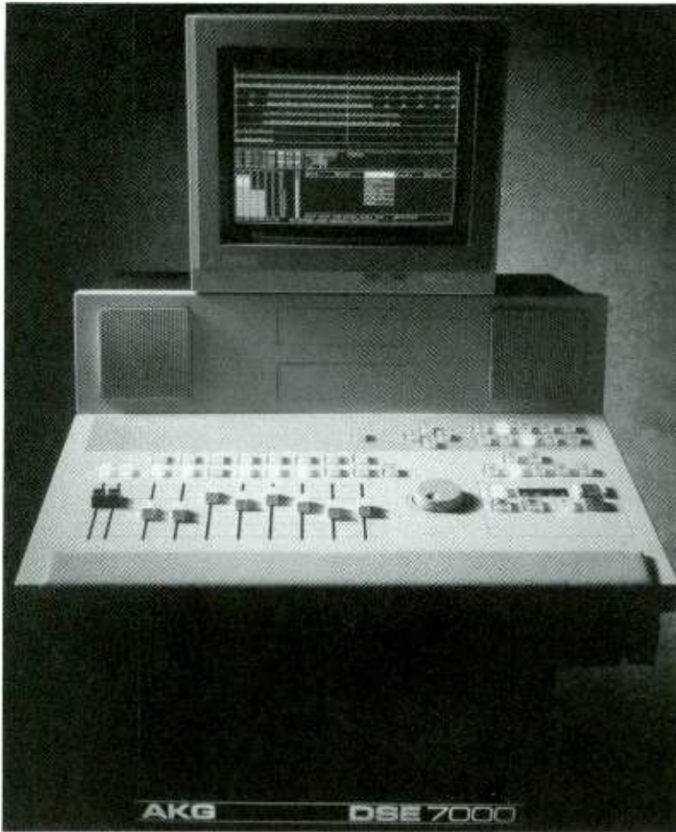
FIGURE 9.31 Digital audio workstations mark a new era in radio production mixing, editing, and storage. Courtesy AKG.
