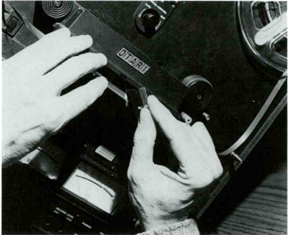
FIGURE 9.29C Make a diagonal cut with a single-edge razor. Use a sharp razor to avoid an uneven cut.
