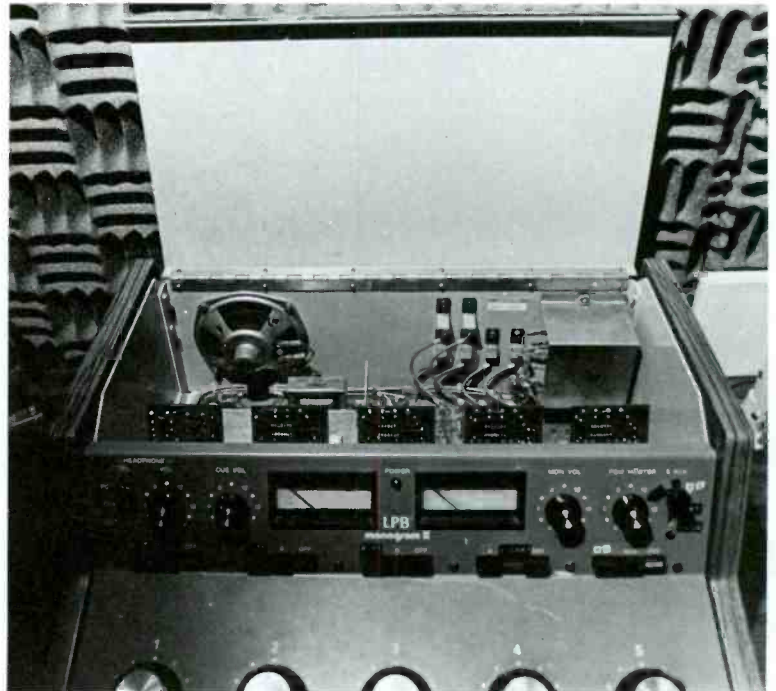
FIGURE 9.9 Cue speaker within console permits producer to set up elements for audio processing. Courtesy LPB.
