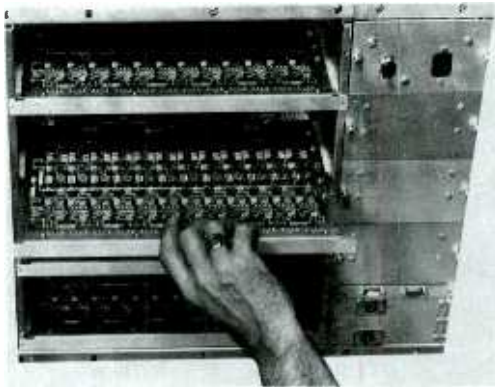
FIGURE 10.22 The luxury of solid-state electronics—pull out the bad, put in the good. Courtesy IGM.
