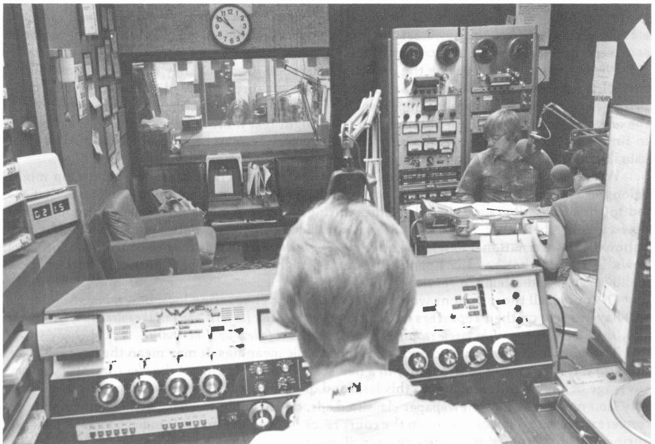
Figure 13-2. A radio broadcast engineer monitors voice levels at the master control board during a live in-studio interview.
