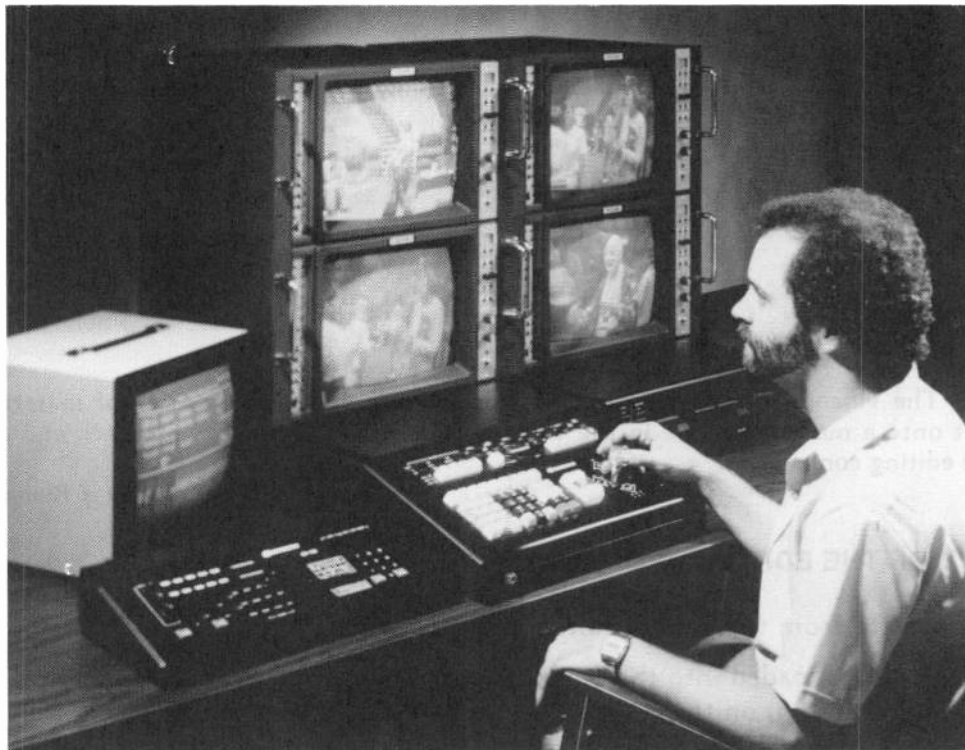
Figure 10-1. A videotape editor previews scenes at an editing console before making a final edit. Three of the four television monitors allow the operator to preview material from three separate videotape recorders during special effects editing, necessary for example when three scenes are to be connected through dissolves, or when editing A-B-C roll packages. The fourth monitor shows scenes from the master tape.
