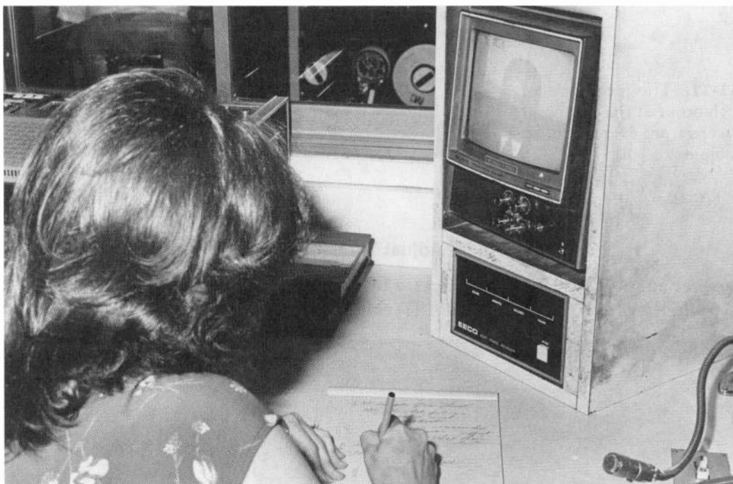
Figure 11-13. A reporter selects sound bites from a field tape and enters her selections on a “shot sheet” or edit decision list. Note the edit code reader that displays an SMPTE time code in the extreme upper left hand corner of the TV monitor.
