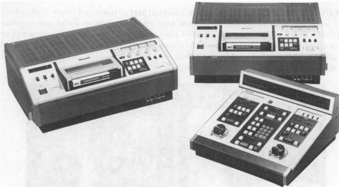
Figure 10-2. The videotape cassette editing system allows electronic transfer of material from the playback unit onto a master cassette in the videotape recorder. Both VTR playback and recorder are slaved to the editing control unit.
