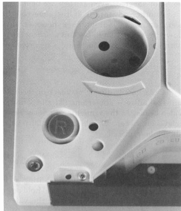
Figure 11-16. The red record button must be in place before the videocassette can be used for recording.
