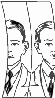
FIG. 67.—The effect of phase displacement, when vertical scanning is in use.
