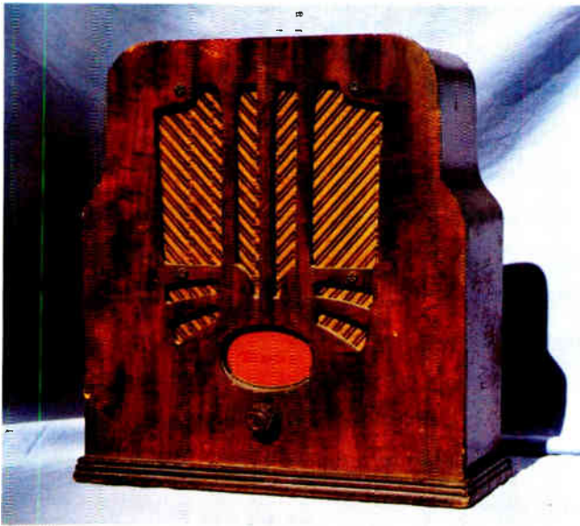
Philco "Teleflash" from the mid thirties. Not actually a radio; the cabinet contains an audio amplifier and a speaker. It was wired to telephone lines and may have been used for news reports or horse racing play-by-play. Photo by Michael Prossie.
