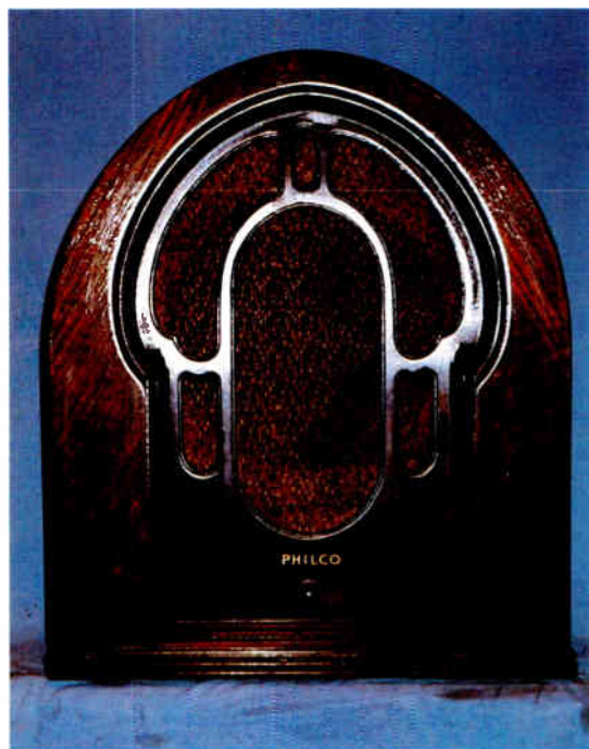
Extension speaker for use with Philco receivers, from 1932. Photo by Michael Prossie.
