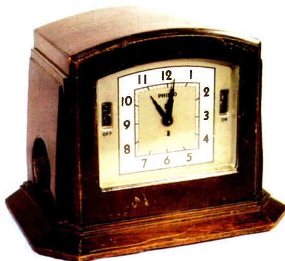
Model A clock timer, which could be set to turn your radio on and off at preset times. Photo by Ron Boucher.
