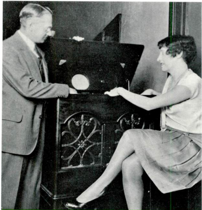
In 1929, Dr. V. K. Zworykin demonstrated the first electronic television receiver using the Kinescope, or picture tube, which he developed together with the famed Iconoscope, "eye" of the camera.
