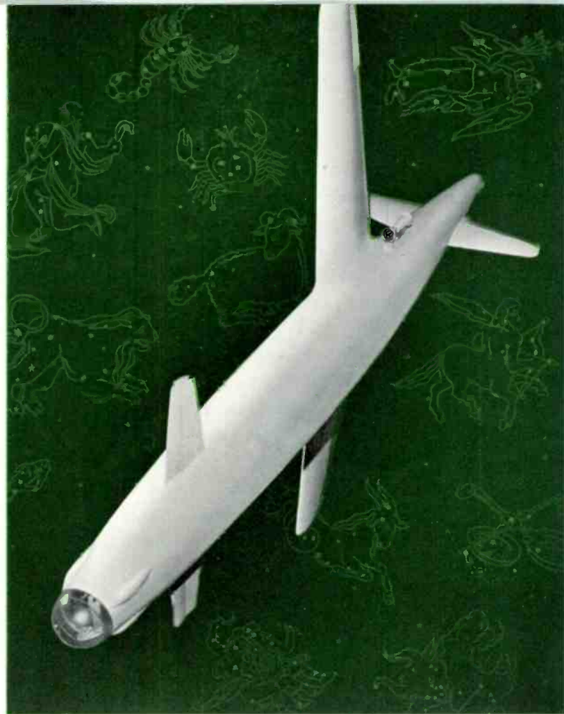
One of the Navy's flying weapons which employs television "eyes" to guide it to the target.
