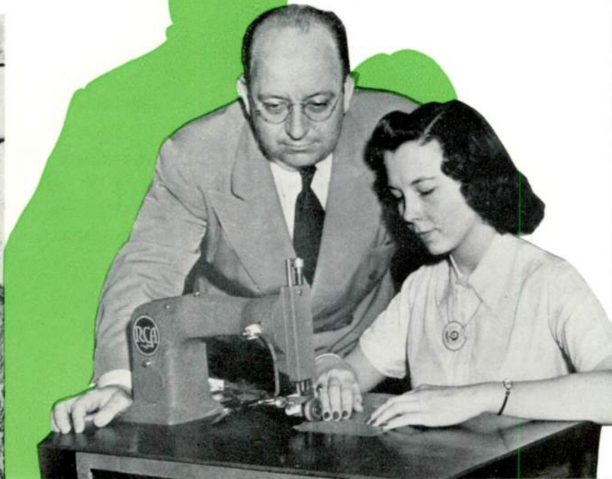
Radio sewing machine developed during the war stepped-up production and usage of thermoplastic garb.
