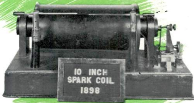
Spark transmitter which played an important role in the early evolution of wireless.
