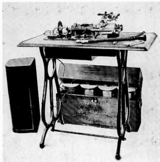
Edison battery-operated "Spectacle" phonograph of 1889 was mounted on a sewing machine stand. Box contained four wet cells (Edison-Lalande) to supply about five amperes current to the DC motor. (Edison National Historic Site Museum.)
