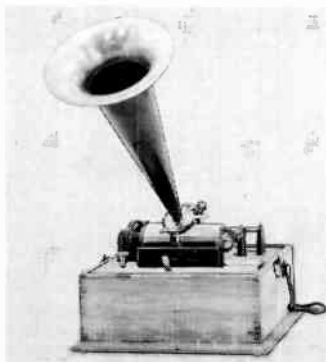
Edison "Standard" phonograph of 1897 had an interchangeable recorder or reproducer. The latter could be adjusted to track the record grooves. Built-in shaver removed thin coating from cylinder for re-use. (O. Read collection.)
