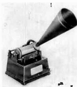
Edison "Gem" phonograph of 1898. First of four compact models. Played the two-minute brown wax cylinder. Knob turned to control speed of governor and moved in and out for braking. (O. Read collection.)
