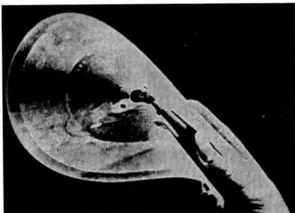
Fig. 30-1. The virtually indestructible PVC foil disc used in the video disc process invented by Teldec.
