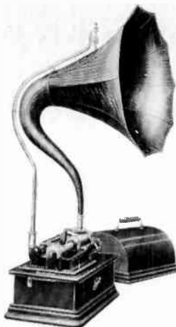
Edison "Home" phonograph of 1911 had an open-ended mandrel. The machine played both two- or four-minute records by means of a turnover Type O reproducer. Proper gear pitch was selected by a manual gear changer. (Clark-Welch Collection.)
