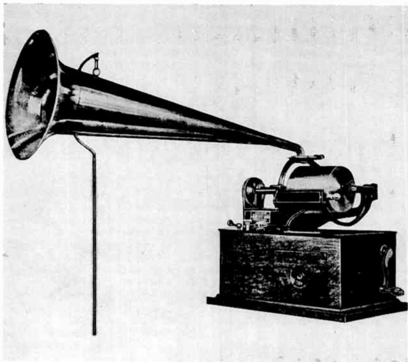
Fig. 12-1. The Edison Concert phonograph played 5-inch wax records. Stepped-up surface speed produced higher frequencies.
