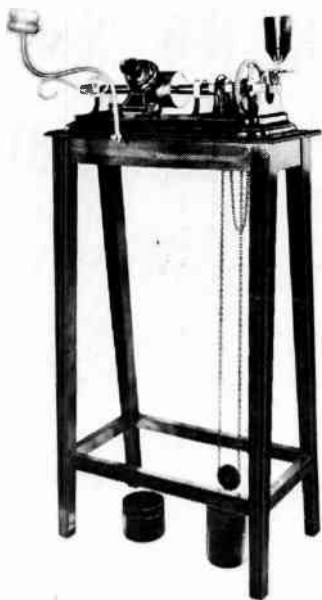
Edison Tinfoil Phonograph, built by the London Stereoscopic Company in London—probably by Charles Stroh. It was made in 1878 and was the first commercial phonograph having a motor (gravity type) and a governor. (Electric & Musical Industries, Limited Museum—Hayes, Middlesex, England.)
