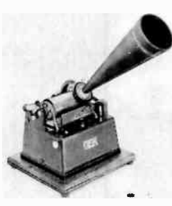
Edison "Gem" phonograph, 1901, with improved spring motor and start-stop-regulating device. A gear-change attachment (added later) reduced rotation speed of feed screw so that four-minute records could be played. (O. Read collection.)
