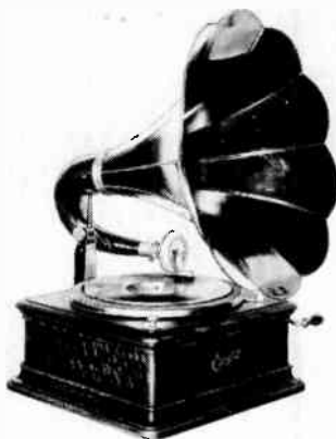
Edison Disc phonograph, made in 1911. Horn had a continuous taper from reproducer to bell. The mica-diaphragmed reproducer is positioned to respond to vertically-cut records. (Edison National Historic Site Museum.)
