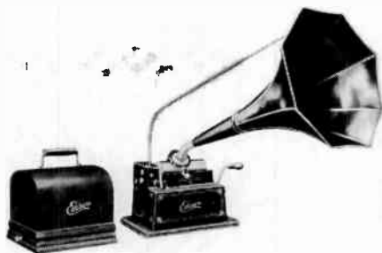
Edison "Gem" phonograph, 1908, played both two- and four-minute records, using a Type K combination reproducer and a Fireside horn supported by a crane. (Edison National Historic Site Museum.)
