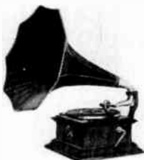
The "Victor II" of 1902 had extra-heavy single spring, a ten-inch turntable, and was furnished with black-japanned steel horn having a 13 3/4-inch bell. It sold for $32.50 with choice of Concert or Exhibition sound box. (Victor 1908 catalogue.)
