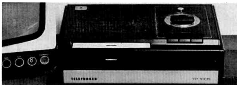
Fig. 30-3. The TED Videodisk player Model TP 1005. (Photo courtesy of Telefunken/Teldec.)
