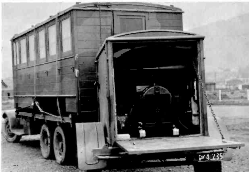
The NBS Middle East Recording Unit. The van woodwork was built by New Zealand Railways, shipped to Egypt and fitted to a Leyland bus chassis.
