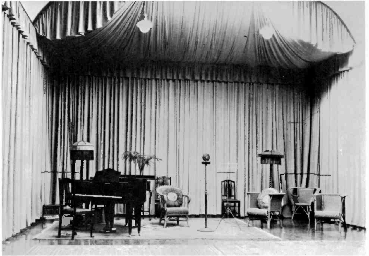
The new IYA studio, France Street, Auckland, 1926. The tent-like drapes on ceiling and walls were an attempt to stop undesirable echoes from getting into the microphone and spoiling the sound.
