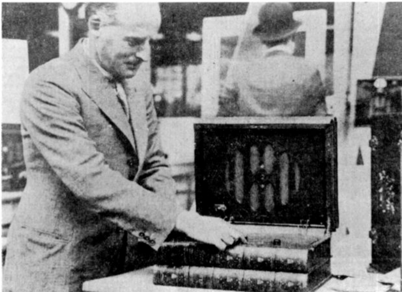
One of the earliest portable radios available in New Zealand, described as ' . . . a five valve portable radio set, self-contained including antenna, batteries and loudspeaker, which may be called the "Library Set". It is built in the form of folio volumes.'
