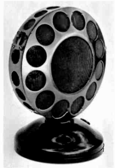
Typical carbon microphone used by radio stations during the 1920s.
