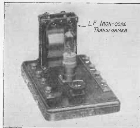
Fig. 89.—Photograph of Low-frequency Panel with Iron-core Transformer.
