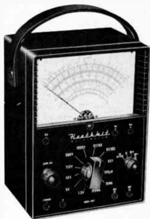
Fig. 403. Volt-ohm-milliammeter constructed from a kit. (Heath Co.)
