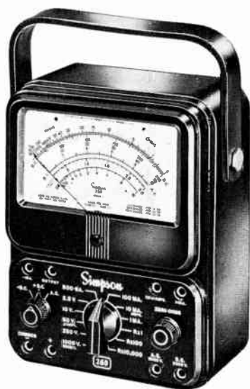
Fig. 506. Typical vom in the larger-size group. (Simpson Electric Co.)
