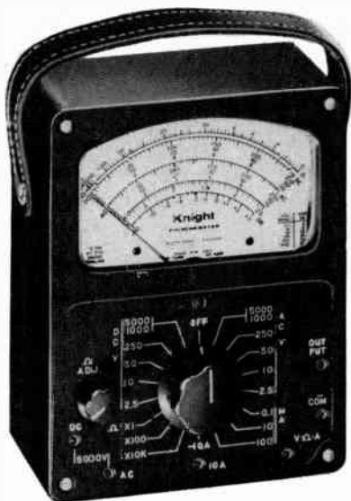
Fig. 416. This is a vom having a sensitivity of 20,000 ohms per volt. It was constructed from a kit. (Allied Radio)
