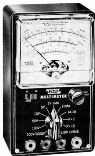
Fig. 516. Typical kit-type multimeter available in wired form. (Electronic Instrument Co.)
