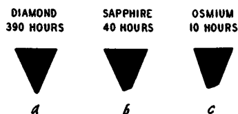
Fig. 1005-a, -b, -c. The diamond stylus has a much longer playing life than other types of needles. Although more expensive, it should be used to protect record grooves against damage by easily worn styli.
