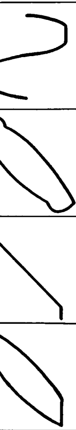
Fig. 709. These waveforms, illustrated at the top half of page 111, are forms of in-phase distortion.
