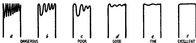
Fig. 602-a to f. Ringing is indicated by a damped wave superimposed on the d.c. level of a square wave.
