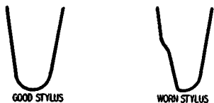
Fig. 1001. It is often difficult to detect needle wear, particularly without the use of a magnifying glass. Sharp reflections when the needle is held up to the light indicate flats. Uniform light reflection shows that there is no perceptible wear.
