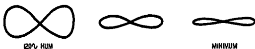
Fig. 1301. Forms of 120-cycle hum as seen on the face of a scope. This is the frequency of power-supply ripple in the output of a full-wave rectifier.
