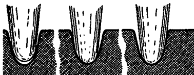
Fig. 1006. For proper sound reproduction, the needle should sit in a perpendicular fashion in the groove. Any tilting to left or right will increase distortion and record wear.
