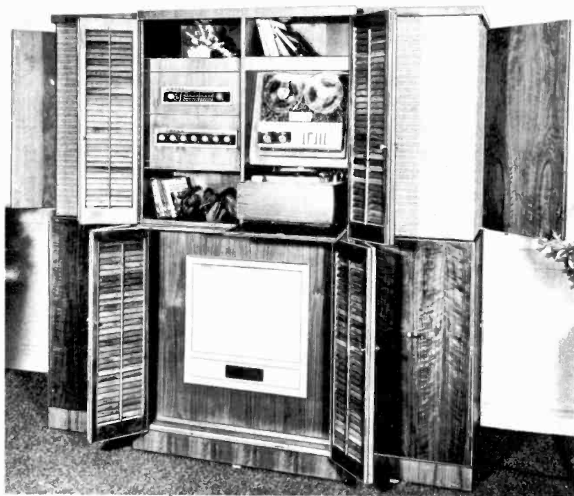
Fig. 1009. In this installation integration has been carried to the point where the cabinetry has been designed for the equipment used. (Courtesy Bell Sound Systems Inc.)
