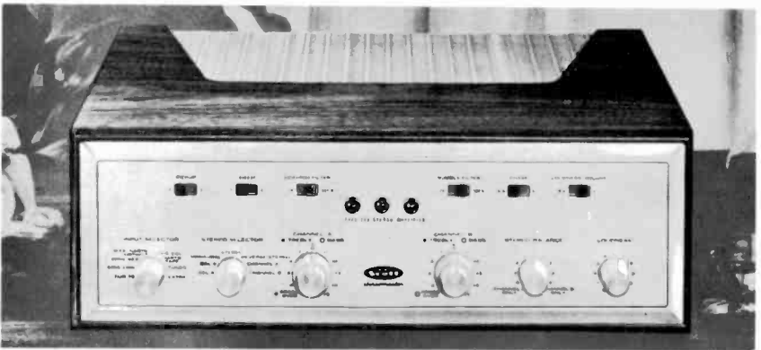
Fig. 1008 (continued). An integrated stereo amplifier which provides 20 watts output on each channel. (Courtesy H. H. Scott, Inc.)
