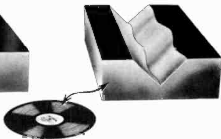
Fig. 410. A stereo groove containing only right-channel modulation.
