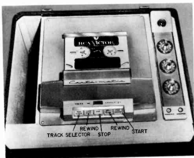
Fig. 613. The RCA tape magazine in place on a special tape machine.
