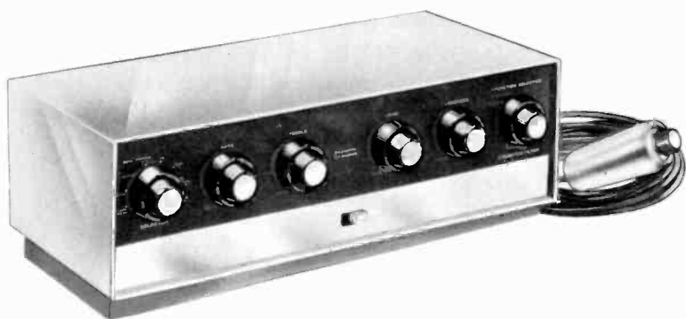
Fig. 805. To balance the stereo system from a normal listening position some control amplifiers include a balance control at the end of a long cable.
