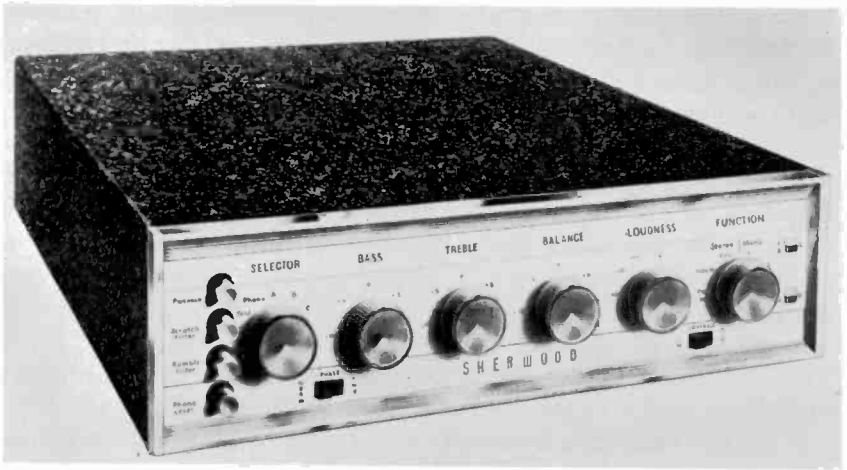
Fig. 1008. This integrated stereo amplifier features pancake construction. (Courtesy Sherwood Electronic Labs., Inc.)
