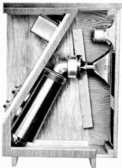
Fig. 919. An internal view of the Stereon. This horn-loaded unit is designed for use with a full-range speaker system. (Courtesy Electro-Voice, Inc.)
