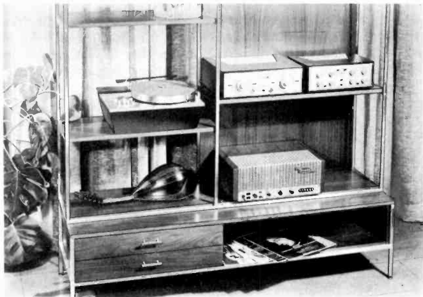
Fig. 1010. The problems of heat and wiring can be solved by using an open installation of the type shown. (Courtesy H. H. Scott, Inc.)
