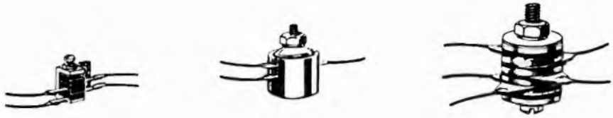
Fig. 6-1. Typical copper oxide instrument rectifiers.
