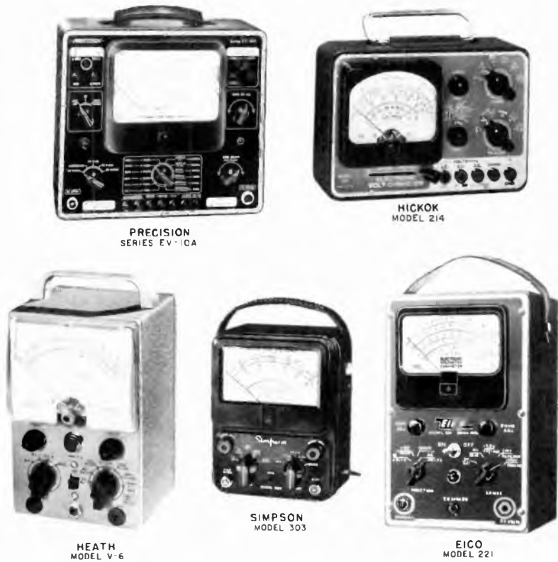
Fig. 10-3. Photographs of typical, modern vacuum-tube voltmeters. (Note: The above photos are reproduced through the courtesy of the manufacturers indicated.)
