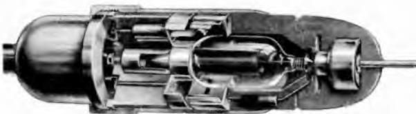
Fig. 9-18. Cross-sectional view of a Hewlett-Packard r-f and high-frequency probe used for measurements up to 1,000 mc.
