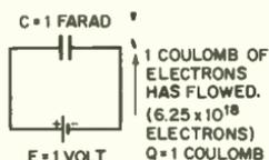
Fig. A-1. One volt causes a flow of  $6.25 \times 10^{18}$  electrons in a one-farad circuit.
