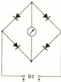
**The basic full-wave bridge rectifier circuit.**
