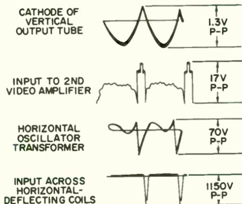
with a peak voltage of 1.5 volts. Many types of nonsinusoidal waveforms are encountered in TV receiver circuits. Fig. 4 shows some typical waveforms, with their normal peak-to-peak voltages.
