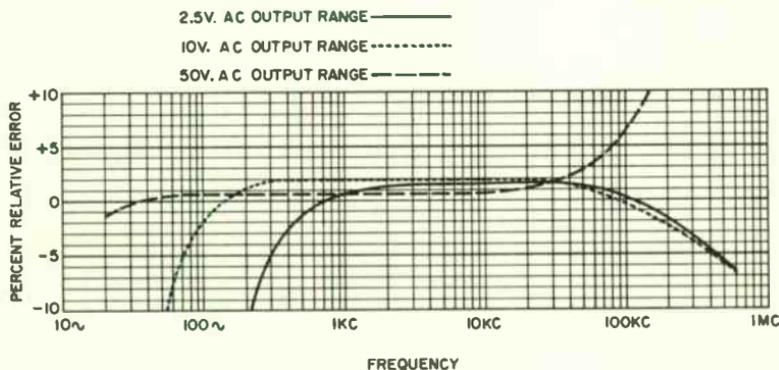
**Accuracy for output measurements with a typical VOM.** (Courtesy of Simpson Electric Co.)
