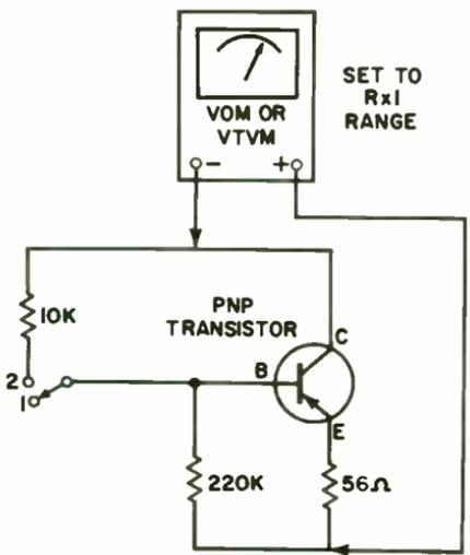
**Ohmmeter test of a transistor.**
