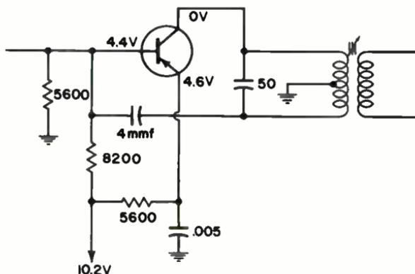
**(A) Zero-emitter voltage can be caused by shorted 4-mmf capacitor.**
