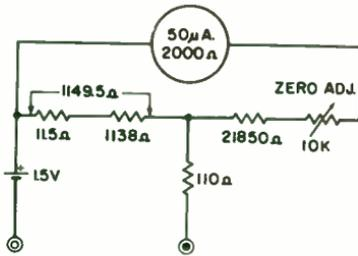
(C) A 110-ohm resistor is switched in on the R  $\times$  100 range to compensate for the resistance of the test leads.
