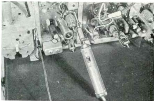
A polarity-reversing probe for a VOM. (Courtesy of Futuromic Co.)
