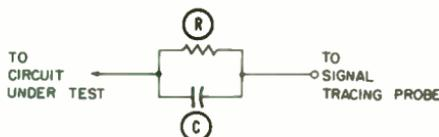
Wide-band voltage divider for signal-tracing probe.
