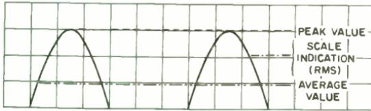
**Output of half-wave rectifier.**
