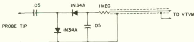
A peak-to-peak signal-tracing probe for a VTVM.
