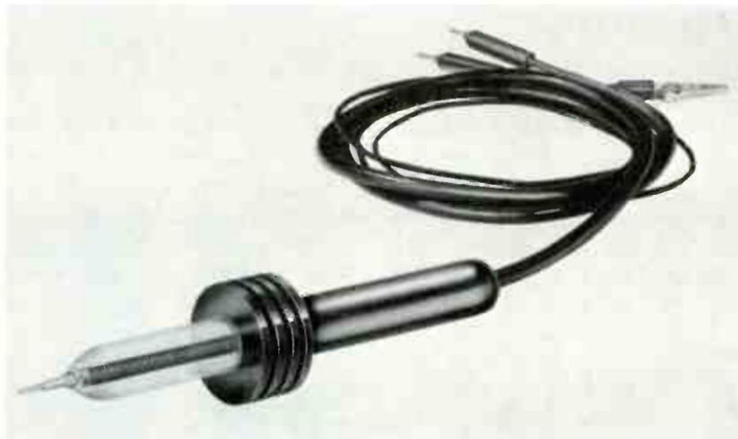
A high-voltage DC probe. (Courtesy of Precision Apparatus Co.)
