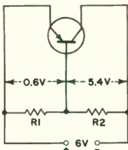
(B) Biasing with one battery and a voltage divider.
