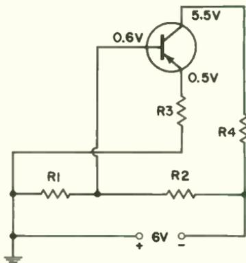
(C) Positive end of battery is grounded.
