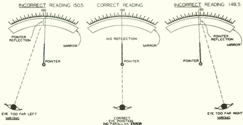
Using the antiparallax mirror. (Courtesy of B&K Manufacturing Co.)
