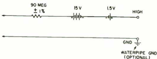
Circuit for a VTVM high-ohms probe.
