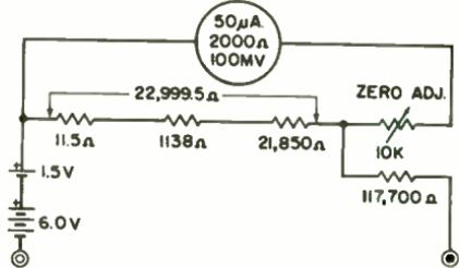
(D) A 117,700-ohm resistor is switched in on the R  $\times$  10,000 range to compensate for the resistance of the test leads.
