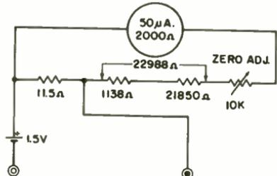
(B) Nominal circuit on R  $\times$  1 range includes resistance of test leads (not shown).
