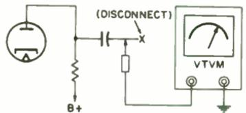
**Test setup for more sensitive test.**
