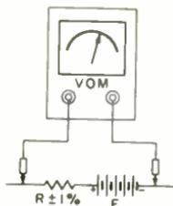
**(A) Measuring battery voltage.**
