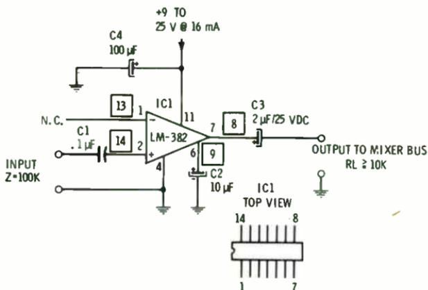
**Dual low-noise microphone preamplifier.**
