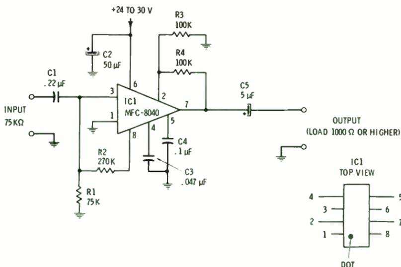
**High-gain microphone preamplifier.**
