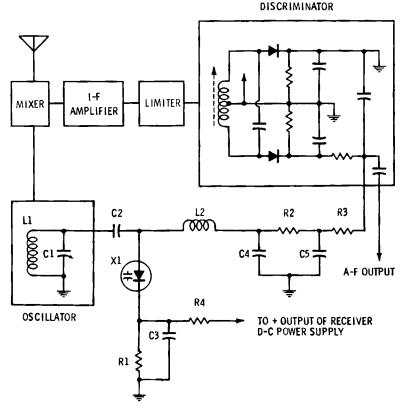
Fig. 3-4. Afc applied to an f-m receiver.
