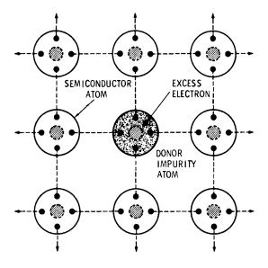
Fig. 1-3. Atoms in N-type semiconductor crystal lattice.
