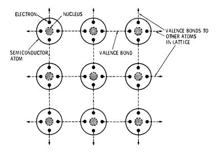
Fig. 1-2. Atoms in intrinsic semiconductor crystal lattice.
