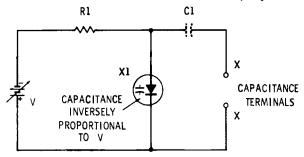
Fig. 2-1. D-c control of a varactor.
