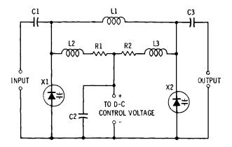
Fig. 7-4. Voltage-tuned pi filter.
