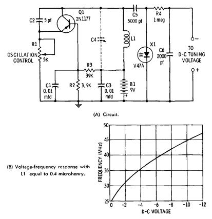
Fig. 4-2. Voltage tuning of low-powered transistor oscillator.
