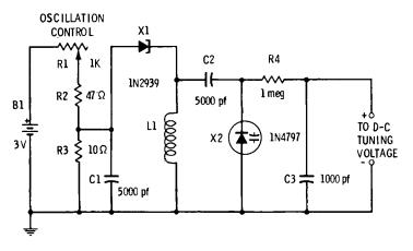
Fig. 4-3. Voltage tuning of tunnel-diode oscillator.
