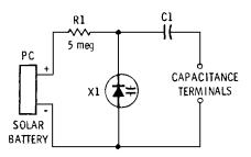
Fig. 7-8. Light-controlled capacitor.
