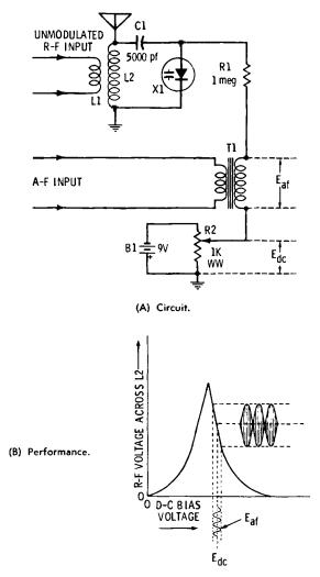
Fig. 4-8. Amplitude modulator.
