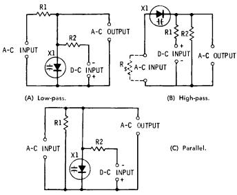
Fig. 2-7. Varactor in RC tuned circuits.
