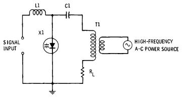
Fig. 5-1. The basic varactor amplifier.
