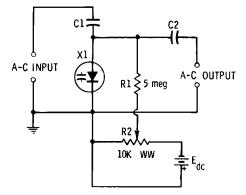
Fig. 7-7. Capacitive potentiometer (attenuator).
