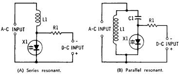
Fig. 2-6. Varactor-tuned LC circuits.
