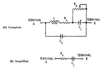
Fig. 1-7. Varactor equivalent circuit.
