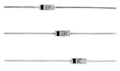
Courtesy TRW Semiconductors Fig. 1-10. Small-size varactors (TRW PG333).
