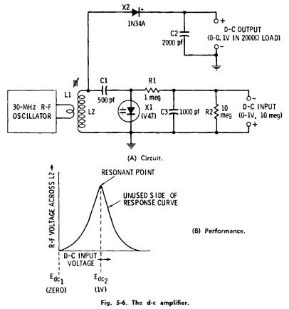
signals, this circuit provides a current gain of 500, power gain of 50, and voltage gain of 0.1. In its transformation of high input resistance (10 megohms) to low output resistance (2000 ohms) at power gain and voltage loss, it resembles a d-c cathode follower and is useful as such whenever its 10:1 voltage reduction can be tolerated.
