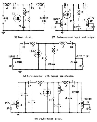
Fig. 4-6. Typical tripler circuits.
