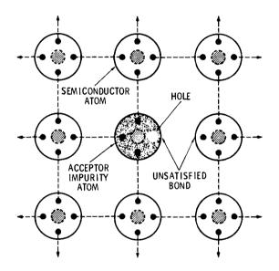
Fig. 1-4. Atoms in P-type semiconductor crystal lattice.
