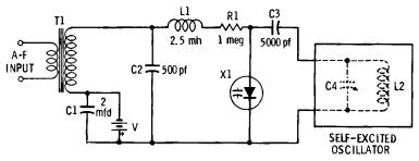
Fig. 4-7. Frequency modulator.
