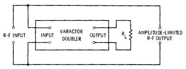
Fig. 7-2. Microwave-limiter circuit.
