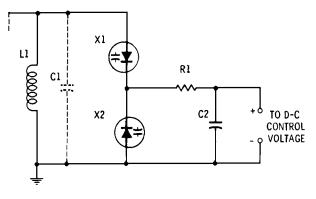
Fig. 3-2. A balanced-varactor tuned circuit.
