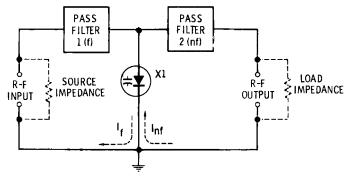
Fig. 2-8. Varactor frequency multiplier.
