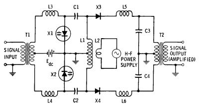
Fig. 5-3. Push-pull varactor amplifier.
