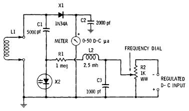
Fig. 6-1. Absorption wavemeter.
