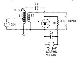
Fig. 7-6. Ultrahigh-resistance switch.
