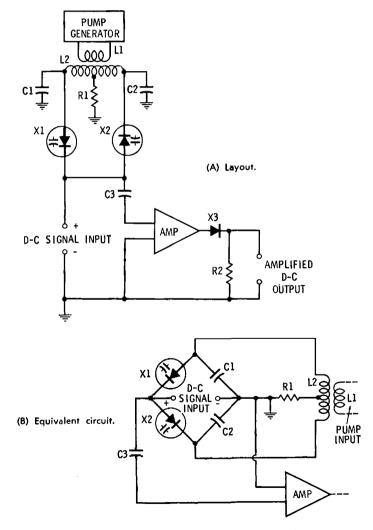
Fig. 6-5. Varactor signal converter for an instrument amplifier.
