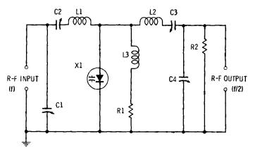
Fig. 7-1. Frequency-divider circuit.
