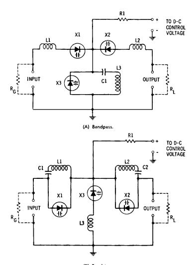
(B) Bandstop.Fig. 7-3. Wave filters.
