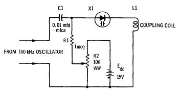
Fig. 6-3. A harmonic intensifier for frequency standard.
