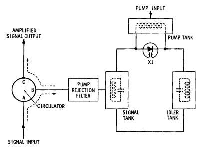
Fig. 5-5. Parameter amplifier with idler.
