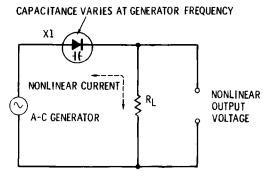
Fig. 2-2. Elementary a-c varactor circuit.
