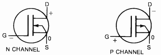
(B) MOSFETs (Depletion type—reverse bias reduces current.)
