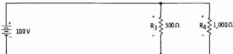
Two unequal resistances in parallel with a voltage source.
