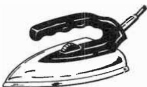
MOST ELECTRIC IRONS HAVE CONTROLS THAT REGULATE THE AMOUNT OF HEAT DEVELOPED BY THE HEATING ELEMENT (WIRE).
