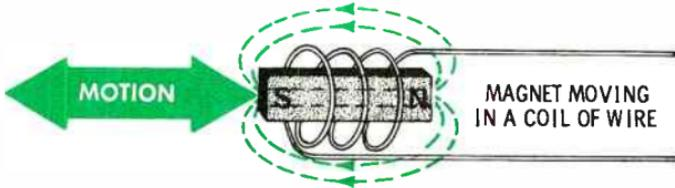
Inducing a current in a coil of wire.
