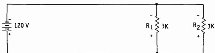
Two equal resistances in parallel with a voltage source.
