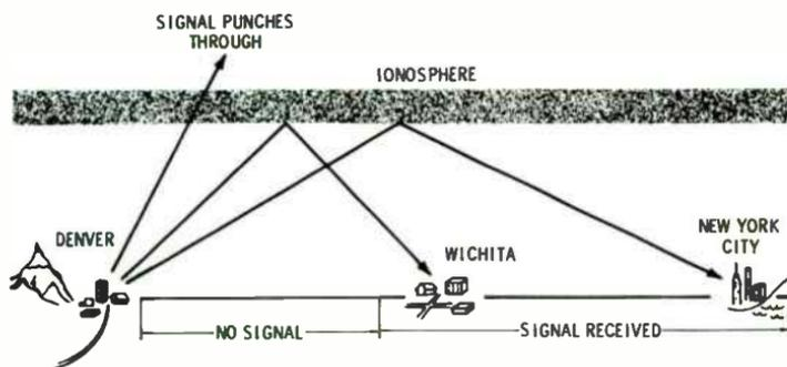
Fig. 1-4. Skip effect on 40-meter band.
