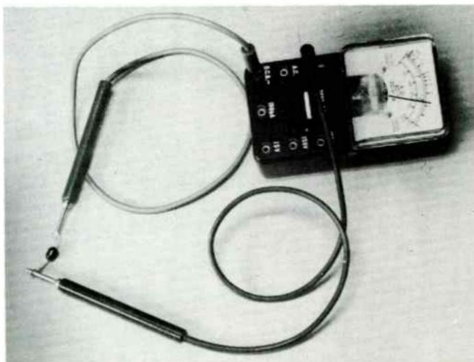
Fig. 4-6. Checking front-to-back ratio of a diode.
