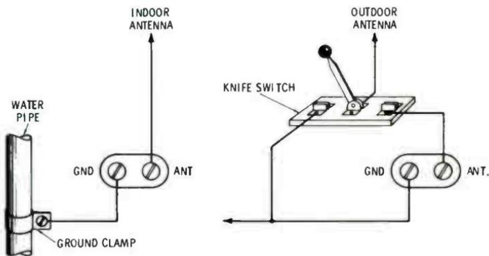
Fig. 3-2. Connections for single-wire antenna.
