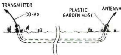
Fig. 10-13. Running coaxial cable underground.
