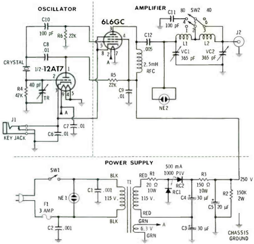
Fig. 6-9. Schematic diagram of the transmitter.
