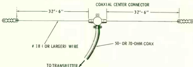
Fig. 10-7. The 40- and 15-meter antenna.
