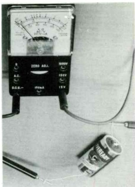
Fig. 4-10. Measuring battery voltage.
