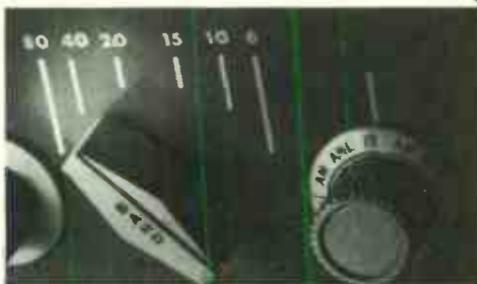
Fig. 3-6. Bands specified on the panel.
