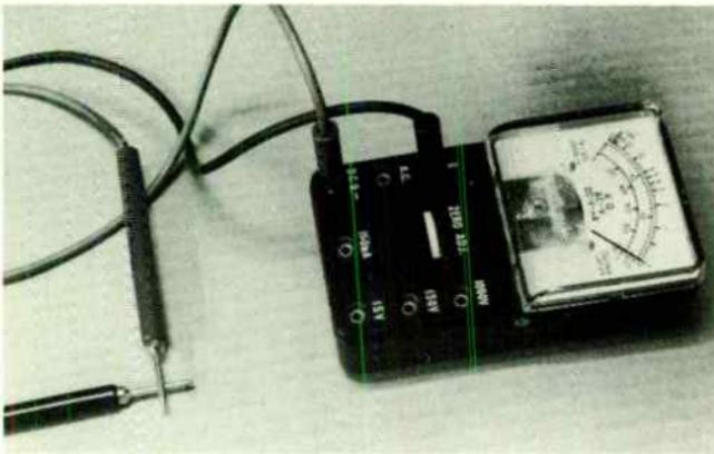
Fig. 4-3. Preparing meter for resistance measurements.
