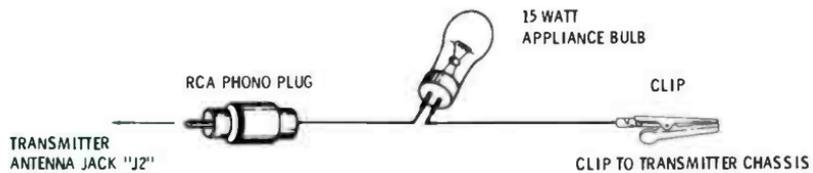
Fig. 6-10. Dummy antenna construction.
