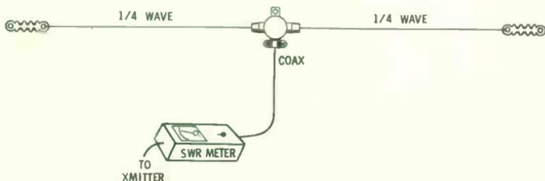
Fig. 10-5. Hookup for an swr meter.
