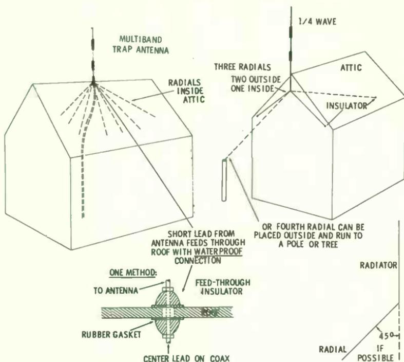
Fig. 10-12. Radials can be inside attic.
