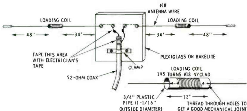
Fig. 10-9. Three-band antenna using loading coils.
