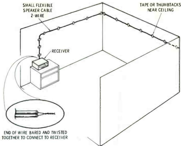
Fig. 3-1. A temporary room antenna.
