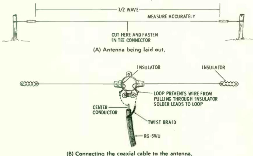
Fig. 10-3. Constructing a dipole.
