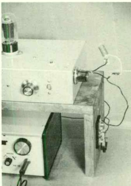
Fig. 9-2. Antenna switch mounted on base.
