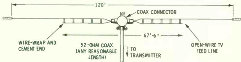
Fig. 10-8. Novice-band antenna for 80, 40, and 15 meters.
