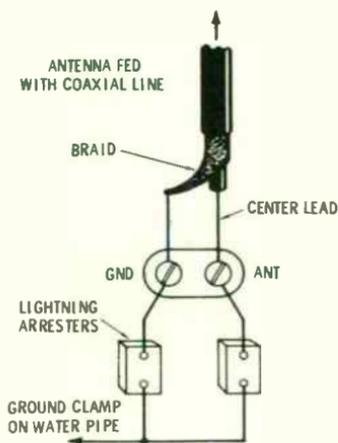
Fig. 3-3. Connections for coaxial-cable antenna.
