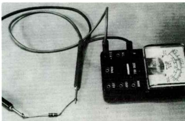
Fig. 4-4. Checking the resistance of a resistor.
