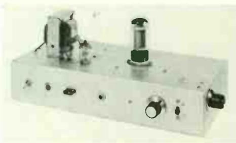
Fig. 5-4. A homemade transmitter.
