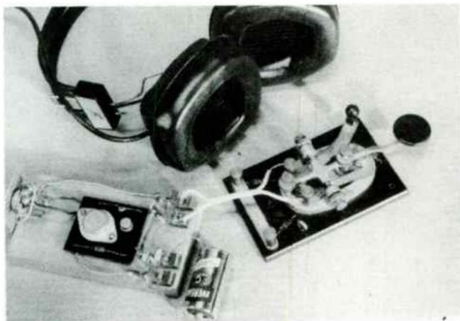
Fig. 8-2. Hookup for using headphones as output.
