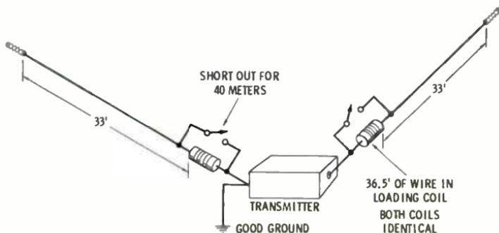
**Fig. 9-8. A short 80-meter antenna.**
