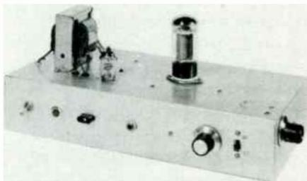
Fig. 6-1. A very simple 25-watt transmitter.
