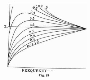
term m will be a positive number between zero and one, and its value governs the characteristics of the filter.
