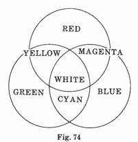
The three additive primaries used in color television are shown in Fig. 74. From the illustration we can see that by mixing colors in certain proportions, we can obtain the following:
