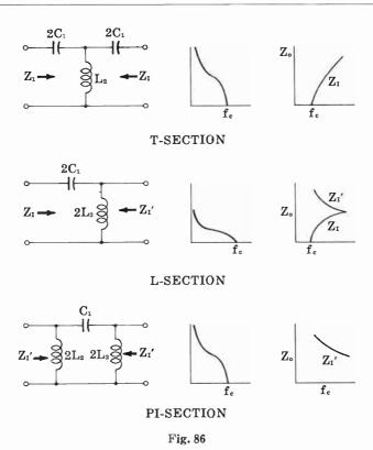
and L sections, and the capacitors in the L and pi sections, are equal to one-half the computed value.
