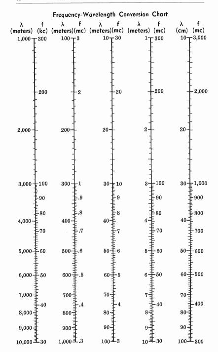
known value (either frequency or wavelength) on one of the scales, and then read the corresponding value from the opposite side of the scale.
