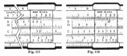
The A and B scales, which are identical, are located on the upper portion of the body and slide. The A and/or B scales are used with the C and/or D scales for finding the square or square root of a number.
