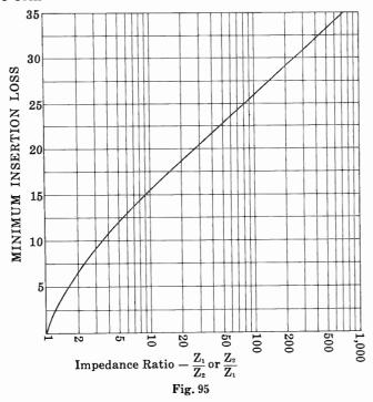
The four steps in the design of a pad are: (1) Determine the type of network required. (2) If impedances are unequal, calculate the ratio of input to output impedance (or output to input impedance) and refer to Fig. 95 for the minimum loss value. (3) From Table XXV find the value of K for the desired loss. (4) Calculate the resistor values, using the following formulas.
