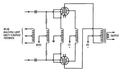
Fig. 5-21. McIntosh Pentafilar winding arrangement.
