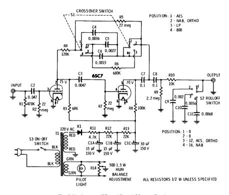
Fig. 5-43. A preamplifier with variable equalization.
