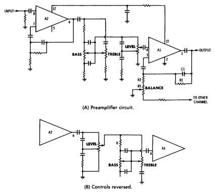
Fig. 5-49. Single-channel preamplifier using one half of integrated circuit.
