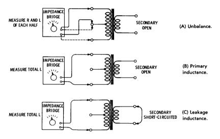
Fig. 5-9. Simple tests on output transformers.
