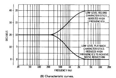
Fig. 4-69. Dolby B processing in Harman-Kardon CAD5 tape deck.
