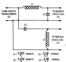
Fig. 6-29. A filter-type divider circuit, formulas, and sample calculation.
