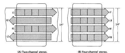
Fig. 3-12. Track arrangements on four-track open-reel tape.
