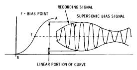
Fig. 4-65. Mixing and applying recording and bias signals.
