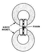
Fig. 4-76. Construction of a velocity microphone.
