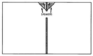
Fig. 8-19. Placement of speakers in adjoining rooms.
