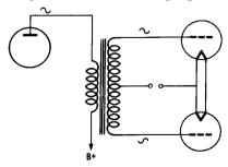
Fig. 5-30. Phase inversion with a transformer.
