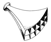
Fig. 6-19. A multicellular horn.
