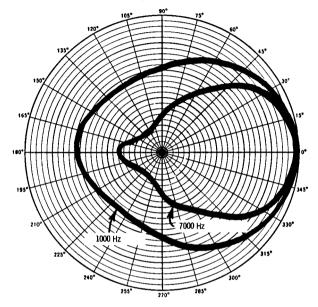
Fig. 4-75. Directivity of a dynamic microphone.
