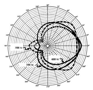
Fig. 4-79. Directivity of a dual-unit microphone.
