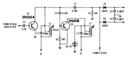
Fig. 4-59. Stereo indicator circuit in Knight Model KN-265.
