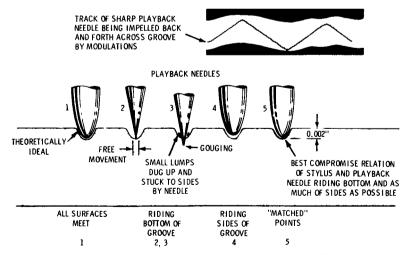
Fig. 4-1. Properly and improperly shaped playback needles.
