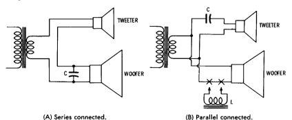
Fig. 6-27. Simple divider circuits employing single reactances.
