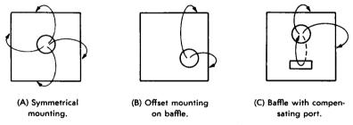
Fig. 7-2. Mounting a speaker on a flat baffle.
