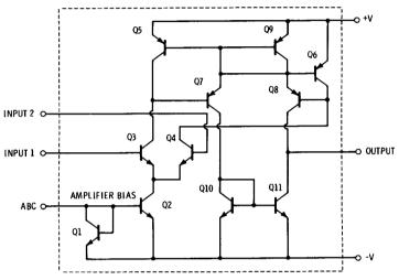
Fig. 4-31. Internal connections of integrated circuit.
