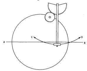
Fig. 4-11. Tracking error of tone arm.
