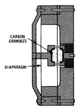
A carbon microphone generates a continuous hiss. This hiss is due to small variations in contact resistance which take place between the carbon granules.
