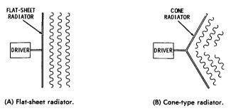
Fig. 6-7. Representation of two types of radiators.
