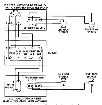
Fig. 8-13. Connection diagram for Stereo-4 decoder.
