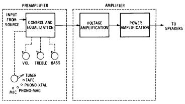
Fig. 5-52. Major divisions and functions of one channel in stereo amplifying system.
