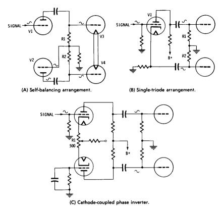
Fig. 5-31. Phase-inverter circuits.
