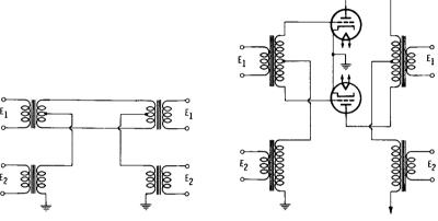
(A) Basic arrangement of transformers in phantom circuit.
