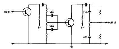
Fig. 5-42. Two-stage preamplifier with separate bass and treble controls.
