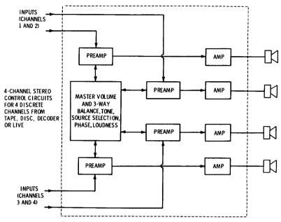
Fig. 5-54. Discrete four-channel arrangement (4-4-4).
