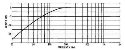
Fig. 7-19. Reduction in bass response in acoustic-suspension speakers.
