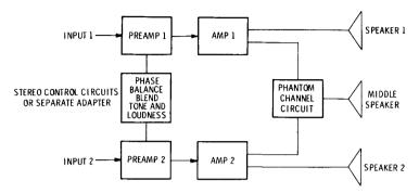
Fig. 5-53. How two amplifier controls are combined for stereo.
