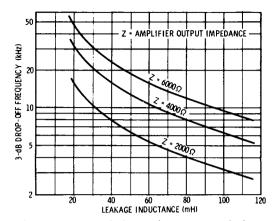
Fig. 5-11. Maximum leakage inductance versus highest response frequency.
