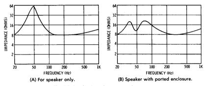
Fig. 7-7. Speaker impedance versus frequency.
