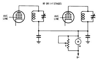
Fig. 4-33. A plate-current signal-strength meter.
