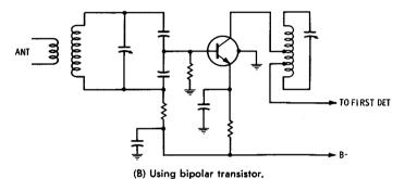
Fig. 4-38. Typical vhf rf amplifiers.
