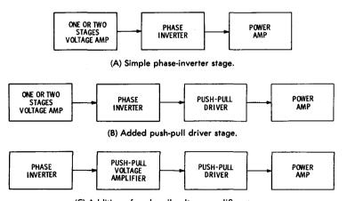
(C) Addition of push-pull voltage-amplifier stages.
