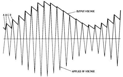
Fig. 4-27. Action of a detector circuit.
