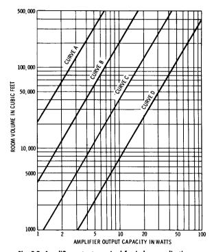
Fig. 8-2. Amplifier output required for indoor applications.
