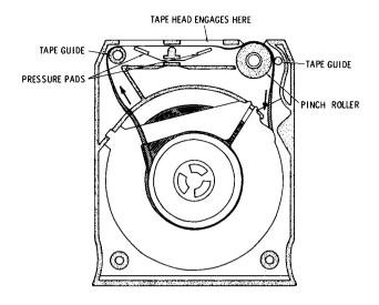
Fig. 3-13. Construction of a tape cartridge.
