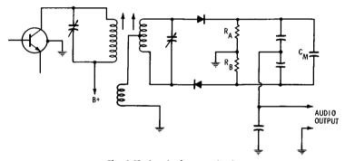
Fig. 4-48. A ratio detector circuit.
