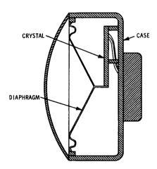
Fig. 4-73. Construction of a crystal microphone.
