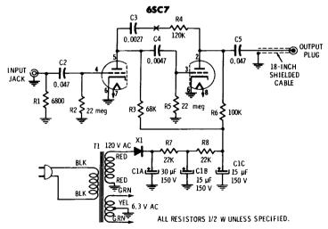
Fig. 5-41. A preamplifier with fixed equalization.
