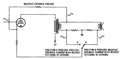
Fig. 5-34. One-stage voltage and current feedback circuit.
