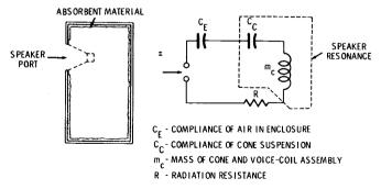
Fig. 7-4. Equivalent circuit of closed-box enclosure.
