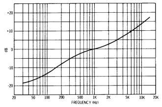
Fig. 5-3. RIAA recording curve.
