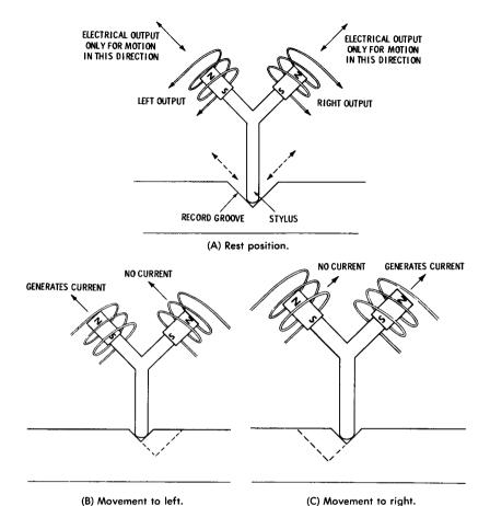
Fig. 3-6. Principle of operation of stereo phonograph cartridge.
