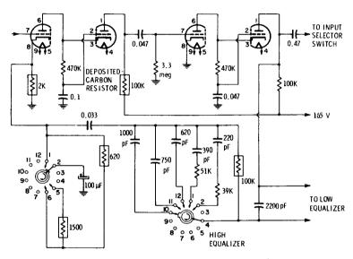
Fig. 5-46. Application of low-noise deposited-carbon resistors to reduce input-stage noise.
