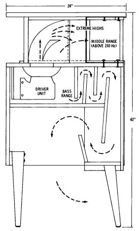
Fig. 7-14. Cross section of acoustic-labyrinth horn.
