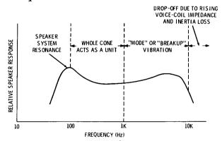
Fig. 6-10. Typical cone-radiator response curve.
