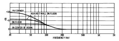
Fig. 7-22. Effects of room gain for different speaker placements.
