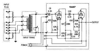
Fig. 5-37. A simple preamplifier circuit.
