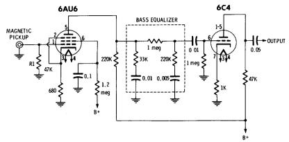
Fig. 5-44. A preamplifier with series equalization-attenuation.
