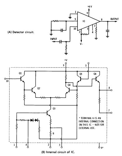
Fig. 4-26. Integrated-circuit a-m second detector.
