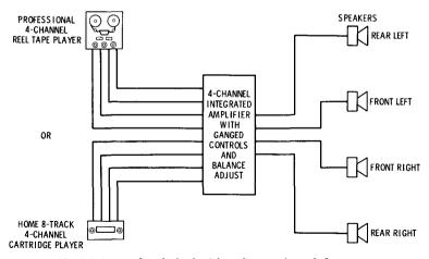
Fig. 8-9. System for playback of four discrete channels from tape.
