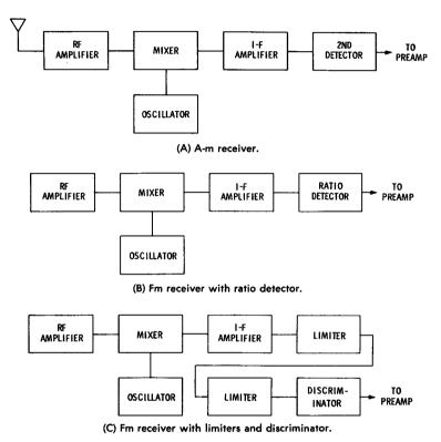
Fig. 4-37. Block diagrams of a-m and fm superheterodynes.
