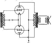
Fig. 5-16. Tetrode power amplifier
