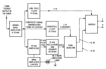
Fig. 4-58. Stereo multiplex with indicator-light takeoff before oscillator.
