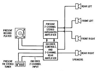
Fig. 8-14. Use of adapter-decoder-amplifier in 4-2-4 system.
