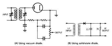
Fig. 4-25. Diode detectors.
