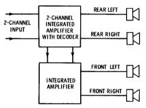
Fig. 5-58. Use of combination decoder and rear-channel amplifiers.
