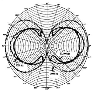
Fig. 4-77. Directivity of a velocity microphone.
