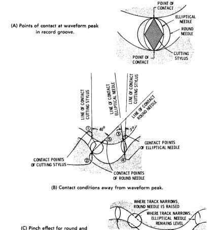
Fig. 4-2. Needle shape and performance.
