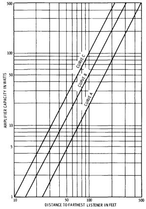
Fig. 8-3. Amplifier output required for outdoor applications.
