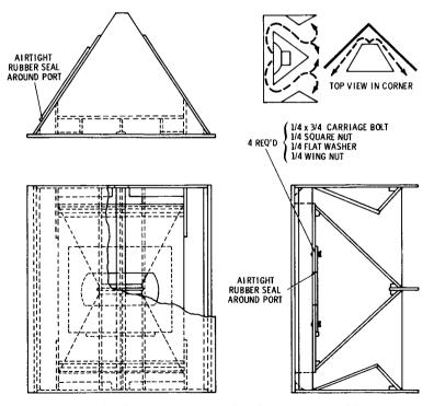
Fig. 7-11. Klipschorn arrangement used in Electro-Voice assemblage.
