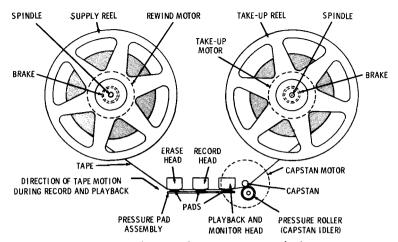
Fig. 4-63. Major parts of a tape-transport mechanism.
