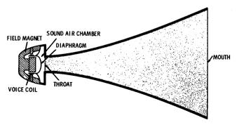
Fig. 6-4. Cross-sectional view of a horn-type reproducer.
