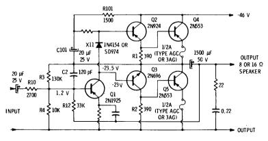
(D) Direct-coupled transistor power amplifier.
