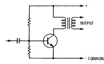
Fig. 5-13. Basic class-A transformercoupled transistor amplifier.
