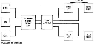
Fig. 5-55. Conversion of two-channel system to four-channel derived stereo (2-2-4).
