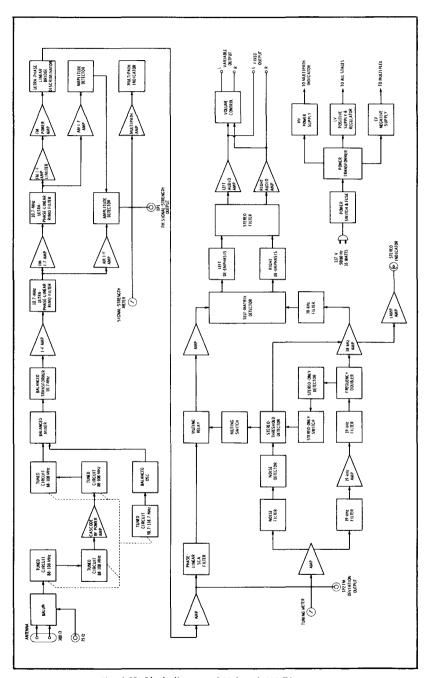
Fig. 4-62. Block diagram of McIntosh MR 73 tuner.
