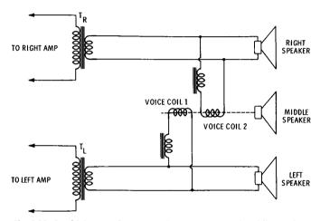
Fig. 8-22. Combining L and R outputs for a two-voice-coil middle speaker.
