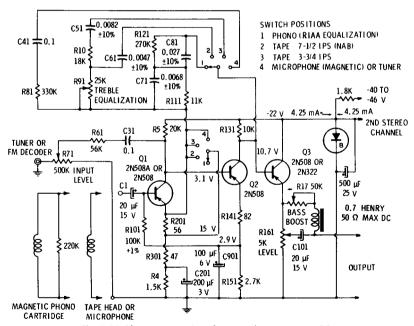
Fig. 5-45. Phono, tape, microphone, and tuner preamplifier.
