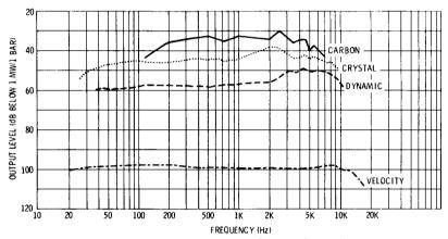
Fig. 4-70. Frequency-response curves for typical microphones.
