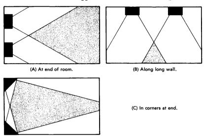
Fig. 8-20. Three ways of placing stereo speakers.
