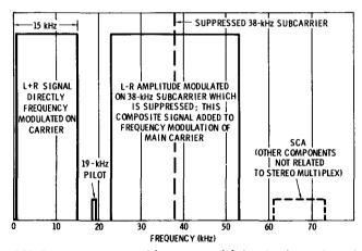
Fig. 4-55. Frequency spectrum of frequency-modulation signal on main carrier.
