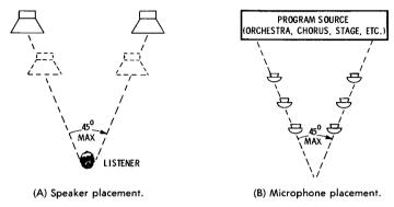
Fig. 3-1. Suitable locations for stereo speakers and microphones.
