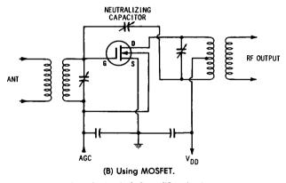
Fig. 4-24. Typical rf amplifier circuits.
