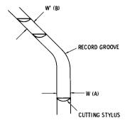
Fig. 3-9. Cause of the pinch effect.
