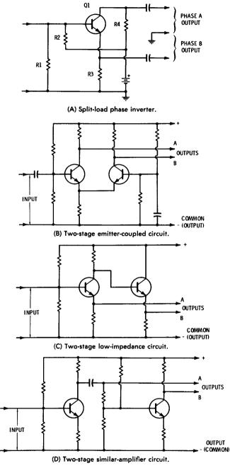
Fig. 5-32. Transistor phase-inverter circuits.
