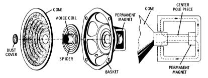
Fig. 6-3. Construction of a permanent-magnet speaker.
