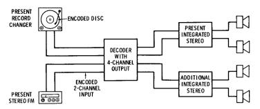
Fig. 8-12. Arrangement for reproduction from encoded discs, tape, or fm broadcasts.
