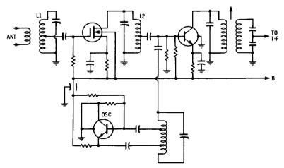
Fig. 4-39. Fm front end using MOSFET.
