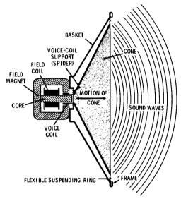
Fig. 6-2. Construction of a moving-coil dynamic speaker.
