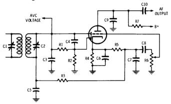
Fig. 4-29. Combined avc, second detector, and audio amplifier.
