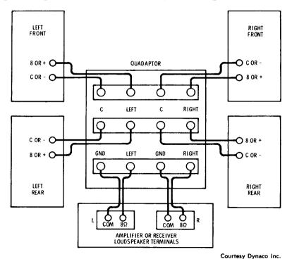
Fig. 8-11. Simplified connection diagram for Dynaco Quadaptor.
