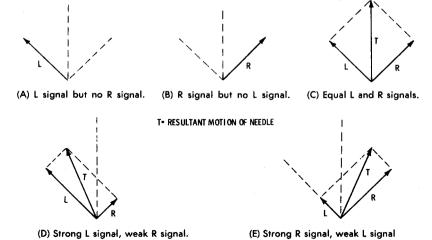
Fig. 3-7. Resultant motion for various combinations of L and R components.
