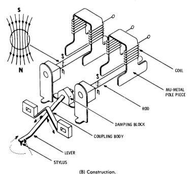
Fig. 4-7. A moving-magnet type of stereo pickup.
