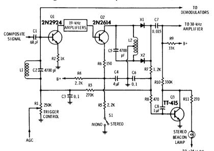
Fig. 4-61. Fisher Model 1249 beacon and automatic stereo circuit.
