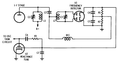
Fig. 4-35. An automatic-frequency-control circuit.
