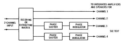
Fig. 5-57. Four-channel synthesized-sound system.
