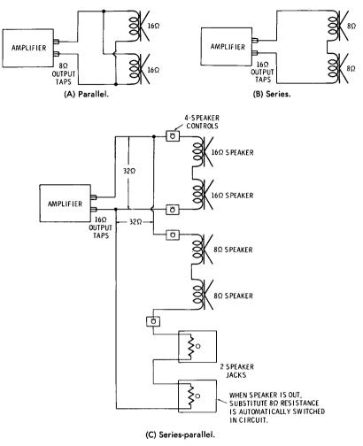
Fig. 8-27. Typical multiple-speaker connection circuits.
