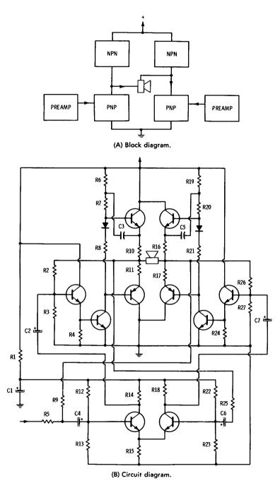
Fig. 5-26. Bridge-type audio amplifier.
