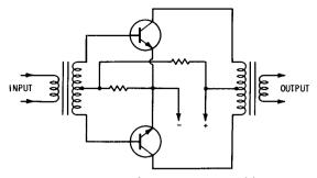
Fig. 5-14. Basic class-AB transistor amplifier.
