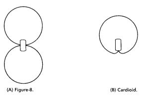
Fig. 3-2. Typical directional-microphone pickup patterns.
