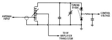
Fig. 4-42. Tuned circuit containing tuning diodes.
