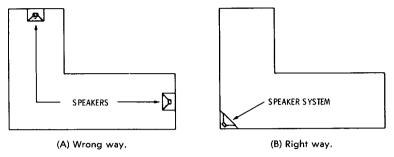
Fig. 8-18. Speaker placement in L-shaped room.
