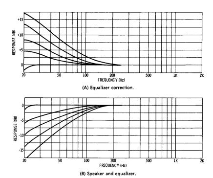
Fig. 7-23. Response curves for McIntosh equalizer.
