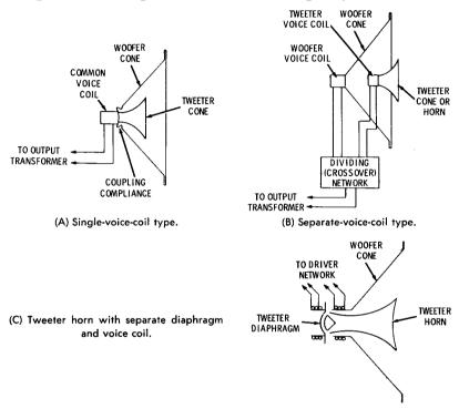
Fig. 6-22. Basic arrangements employed in coaxial speakers.
