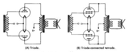
Fig. 5-15. Power-amplifier stages.
