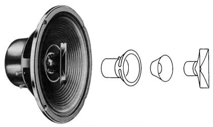
Fig. 6-26. A three-way coaxial speaker.
