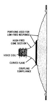
Fig. 6-20. Construction of a typical singlecone, extended-range speaker.
