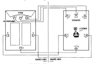
Fig. 2-1. An elaborate stereo system.
