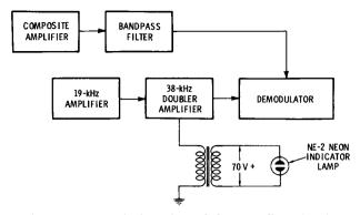
Fig. 4-57. Stereo multiplex indicator light (no oscillator circuit).
