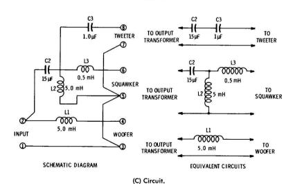
Fig. 6-30. Design features of a commercial three-way divider network.
