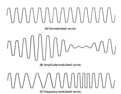
Fig. 4-36. Comparison of amplitude and frequency modulation.
