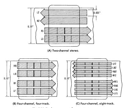
Fig. 3-16. Track arrangement for cassette tape.
