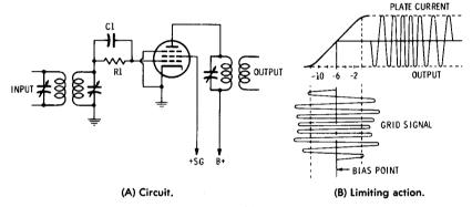
Fig. 4-44. A typical limiter circuit.
