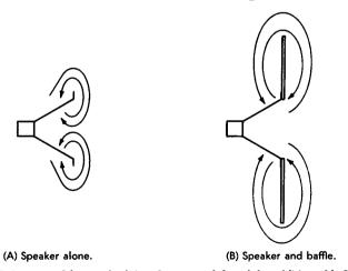
Fig. 7-1. Increase of front-to-back interference path length by addition of baffle.
