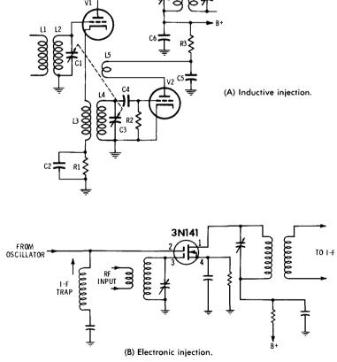
Fig. 4-20. Methods of injecting oscillator signal into mixer.
