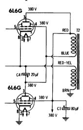
Fig. 5-23. Single-ended push-pull amplifier circuit.
