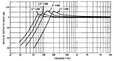
Fig. 6-8. Effect of cone size and resonance on low-frequency response.
