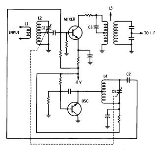
Fig. 4-19. Converter with separate mixer and oscillator.
