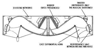
Fig. 7-30. Speaker arrangement in the enclosure of Fig. 7-29.
