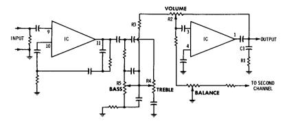
Fig. 5-50. Integrated-circuit preamplifier with feedback volume control.
