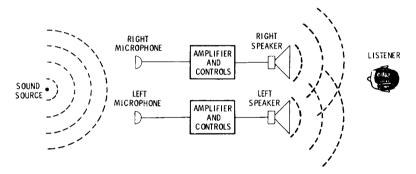
Fig. 2-3. Simple representation of the stereophonic principle.
