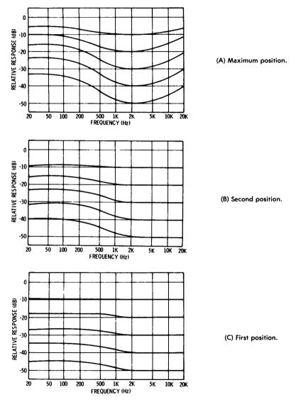
Fig. 5-48. Curves showing the frequency response of the amplifier of Fig. 5-47 corresponding to various positions of the loudness control.
