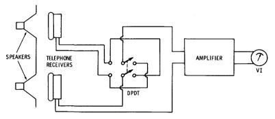
Fig. 8-32. Setup for determining speaker phasing.
