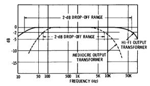
Fig. 5-7. Output-transformer response characteristics.
