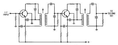
Fig. 4-22. Transistor i-f amplifier.
