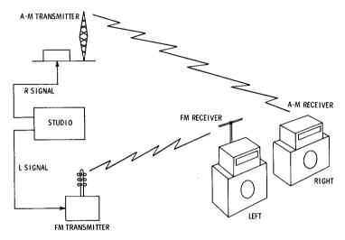
Fig. 3-17. Two-transmitter method for radio transmission of stereo signals.
