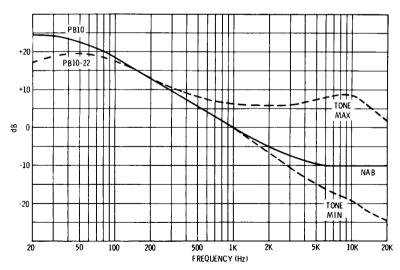
Fig. 5-39. Frequency response in series with head, for circuit shown in Fig. 5-38.
