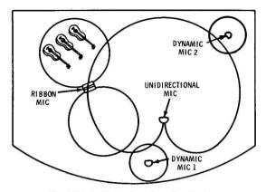
Fig. 4-82. Multiple-microphone installation.
