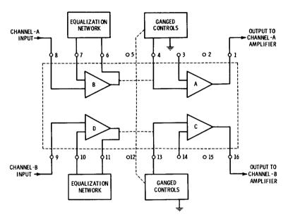
Fig. 5-51, Silicon monolithic integrated circuit for stereo preamplifier.
