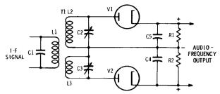
Fig. 4-46. A double-tuned discriminator circuit.
