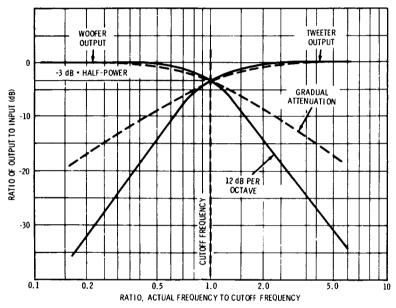
Fig. 6-28. Divider-network response curves.
