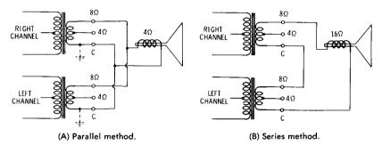
Fig. 8-28. Connection of stereo outputs for single-speaker monophonic operation.
