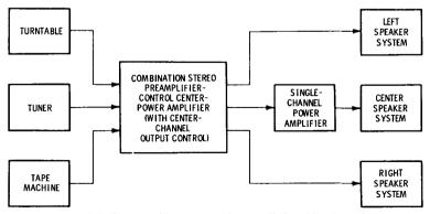
Fig. 8-8. Three-speaker output with controlled middle channel.
