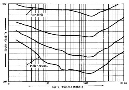
Fig. 1-1. Sound intensity required at different frequencies to produce uniform response in the sensory system of the ear.
