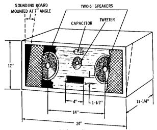
Fig. 7-8. Multiple-speaker arrangement.
