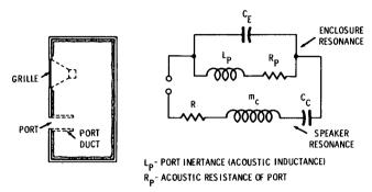
Fig. 7-5. The bass-reflex enclosure and its equivalent circuit.
