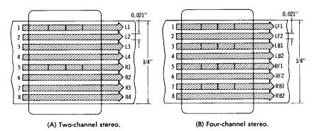
Fig. 3-14. Track arrangements for cartridge tape.
