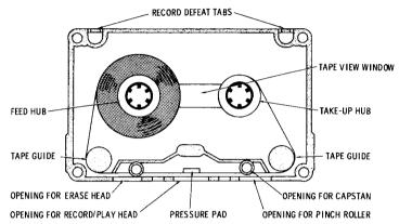
Fig. 3-15. Construction of a tape cassette.
