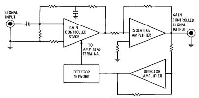
Fig. 4-32. Automatic-gain-controlled amplifier using integrated circuits.
