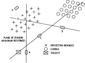
Fig. 4-81. Microphone placement plan.
