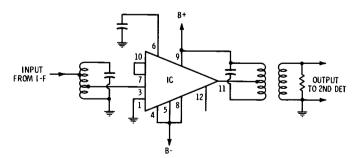
Fig. 4-45. Integrated-circuit limiter.
