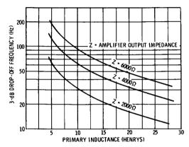
Fig. 5-10. Primary inductance required versus minimum response frequency.
