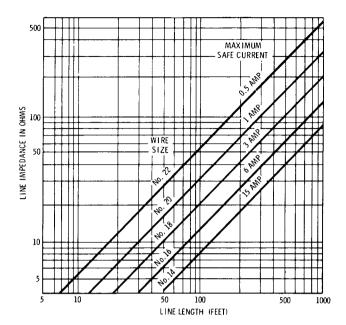
Fig. 8-30. Wire sizes for speaker lines.
