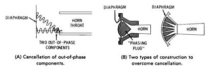
Fig. 6-16. Methods for overcoming out-of-phase cancellation of high-frequency components in the air chamber of a horn driver.
