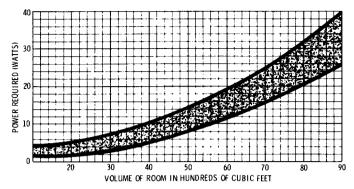
Fig. 8-1. Audio power required for various room sizes.
