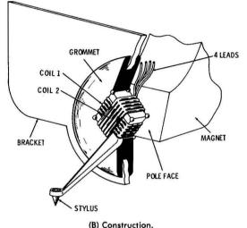
Fig. 4-8. The Grado moving-coil (dynamic) type of stereo pickup.
