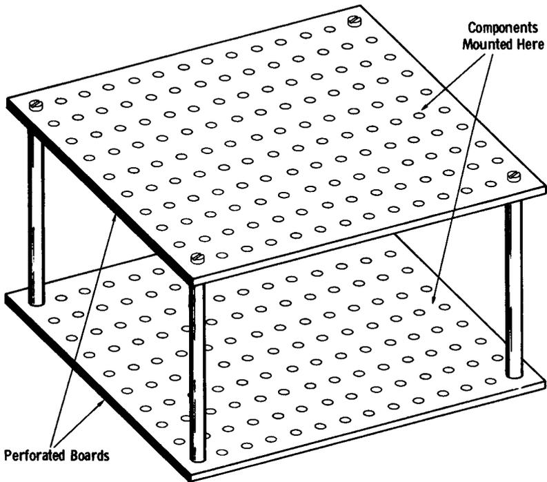
**Fig. 6-11. Stacked perforated board.**
