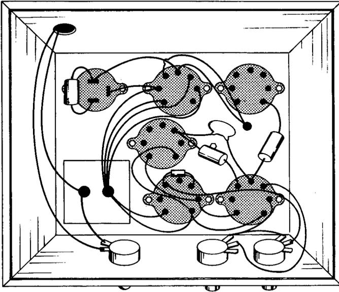
**Fig. 4-5. Example of component wiring.**
