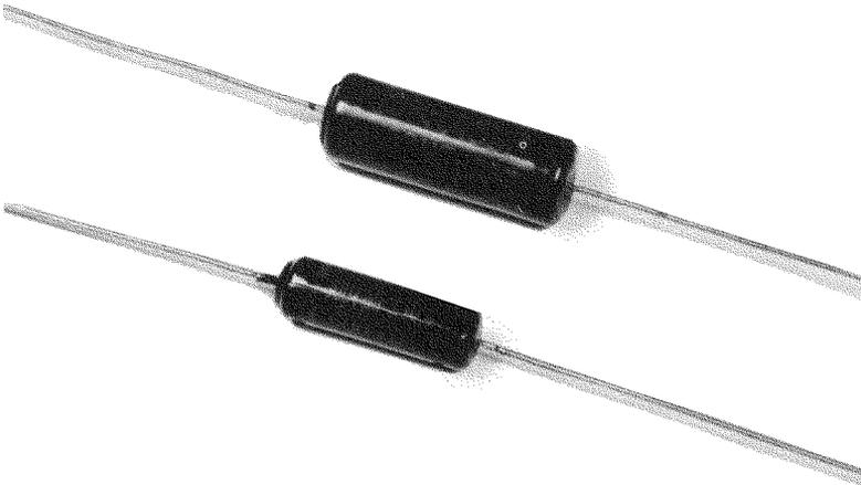
(B) Deposited-film resistor.
