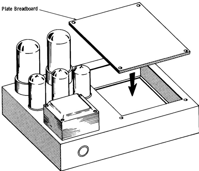
**Fig. 4-6. Integral power-supply breadboard.**
