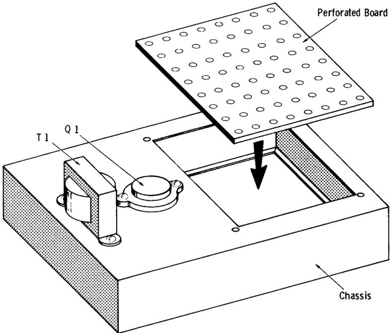
**Fig. 4-12. Integral power-supply breadboard.**
