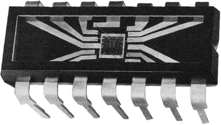
Fig. 6-13. Typical integrated circuits.
