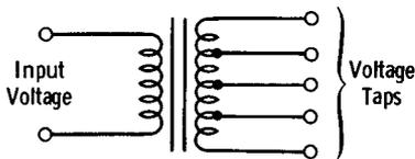
Fig. 3-18. Voltage-adjusting transformer.
