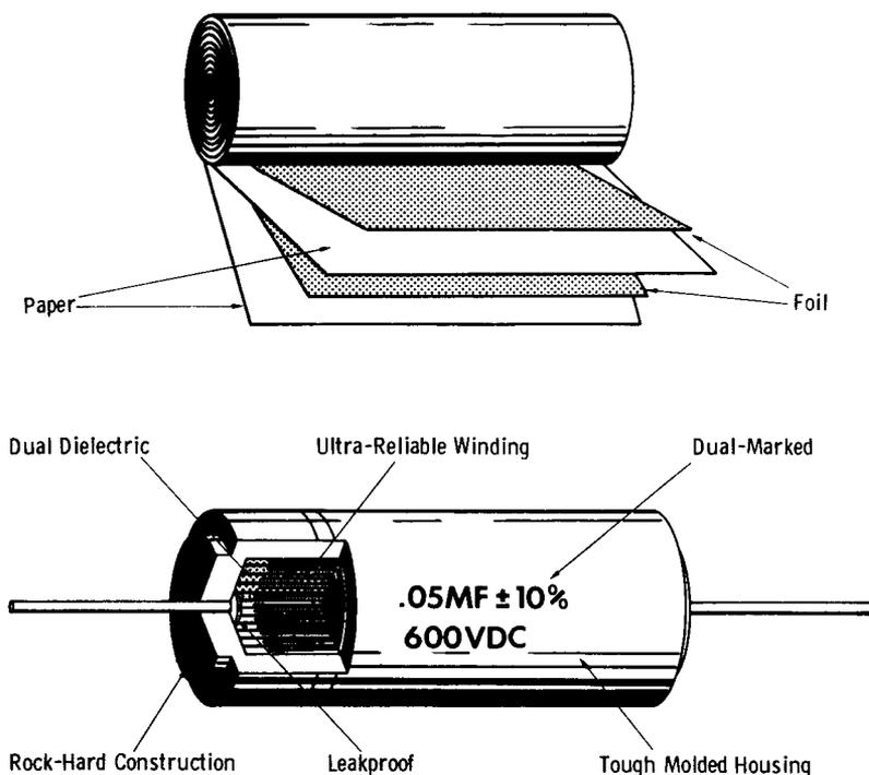
**Fig. 3-6. Paper tubular capacitor.**
