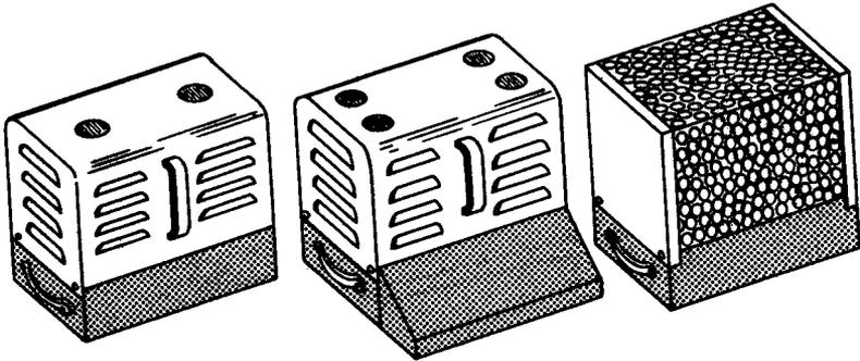
**Fig. 1-16. Amplifier foundations.**
