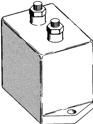
(C) High-capacitance mica capacitor.
