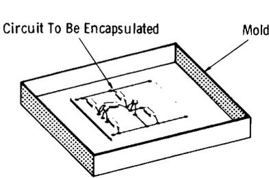
(A) Placing circuit in mold.
