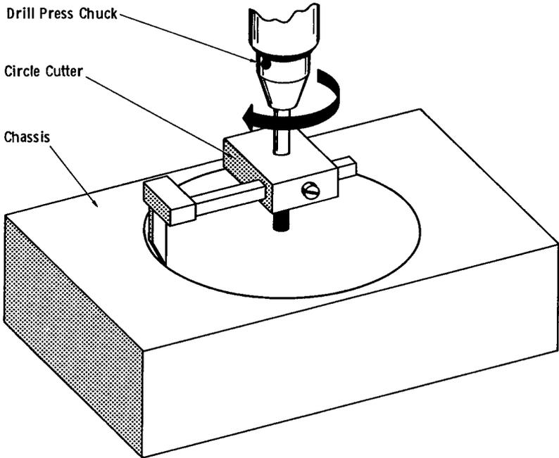
**Fig. 1-5. Operation of a circle cutter.**
