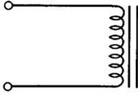
Fig. 3-22. Filter choke.
