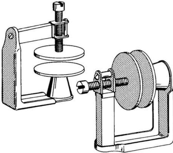
**Fig. 3-14. Neutralizing capacitors.**
