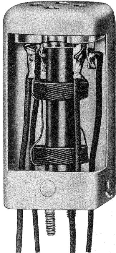
**Fig. 3-21. Intermediate-frequency (i-f) transformer.**
