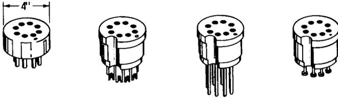
**Fig. 6-15. Sockets for integrated circuits.**
