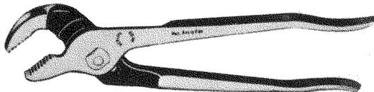
**Fig. 2-4 Tongue and groove pliers.**
