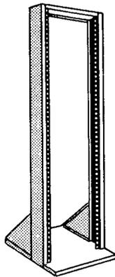
Rack panels are available in either steel or aluminum. Panel thickness may be either  $\frac{1}{8}$  inch or  $\frac{3}{16}$  inch.
