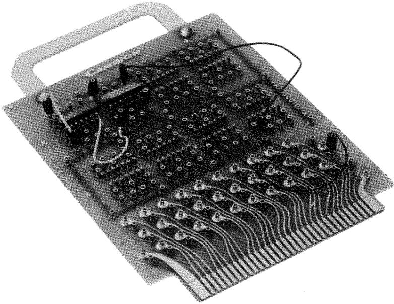
**Fig. 4-10. Commercial breadboard.**
