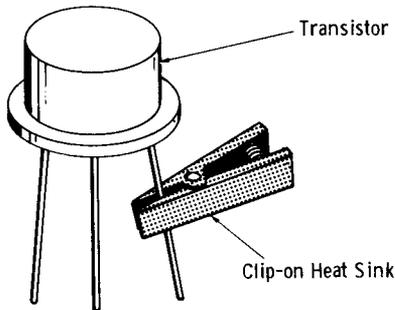
**Fig. 5-2. Clip-on lead heat sink.**
