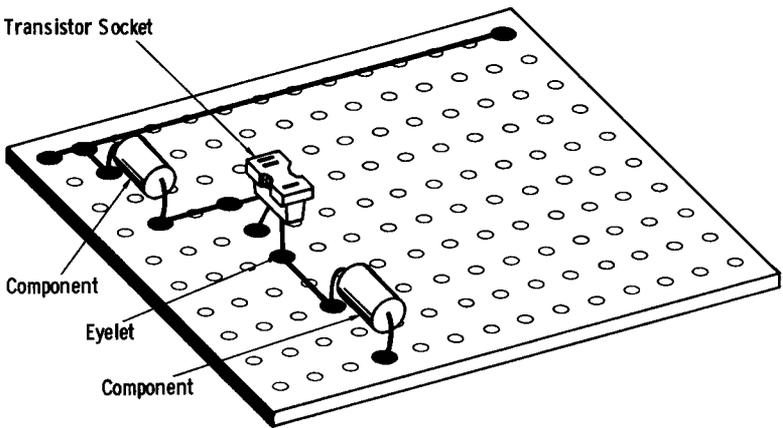
Fig. 4-8. Perforated-board breadboard.
