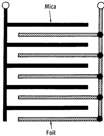
(A) Construction of a typical mica capacitor.
