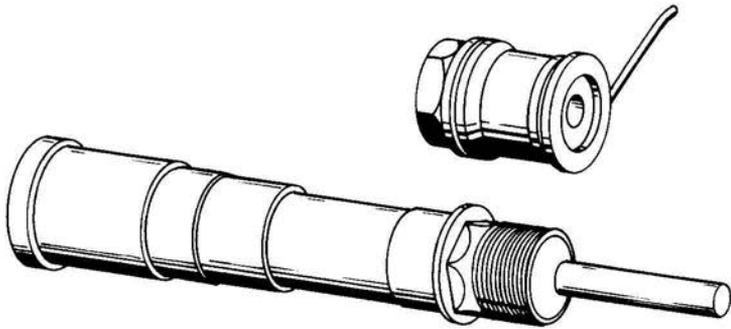
**Fig. 3-13. Piston capacitors.**
