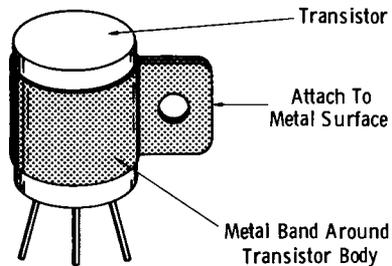
Fig. 5-6 shows a method of providing a heat sink for lower-power (250-500 milliwatt) transistors. A band of aluminum is fashioned to fit around the case of the transistor. The tab is then bolted to the metal chassis or other heat sink. Since the collectors of most of these small transistors are isolated from the case, no insulation is needed between the transistor case and band.
