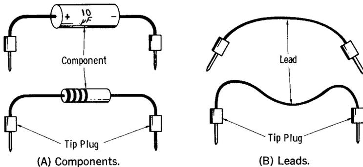
**Fig. 4-2. Tip plugs on component leads.**
