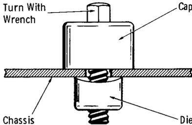
Fig. 1-3. Operation of a chassis punch.
