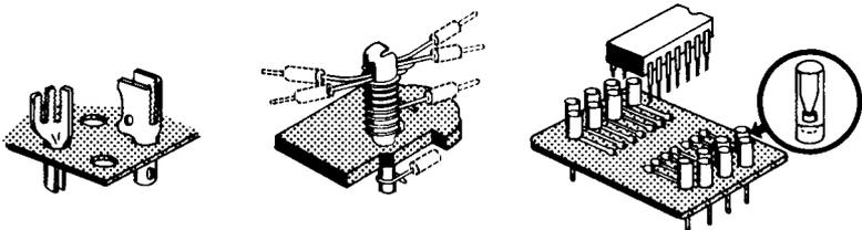
**Fig 4-11 Commercial breadboard components.**
