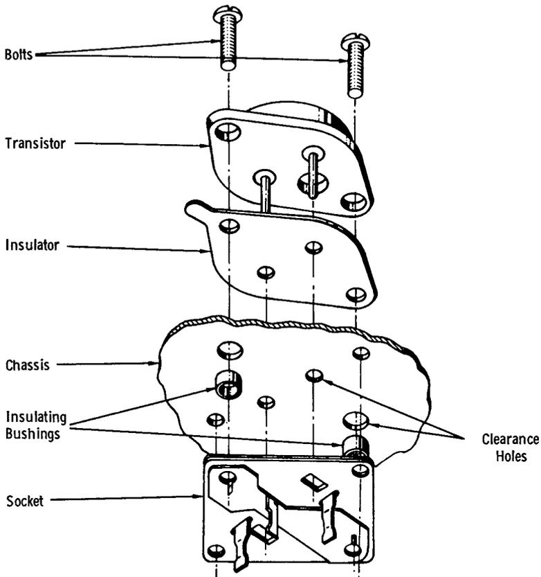
**Fig. 5-4. Method of power transistor mounting.**
