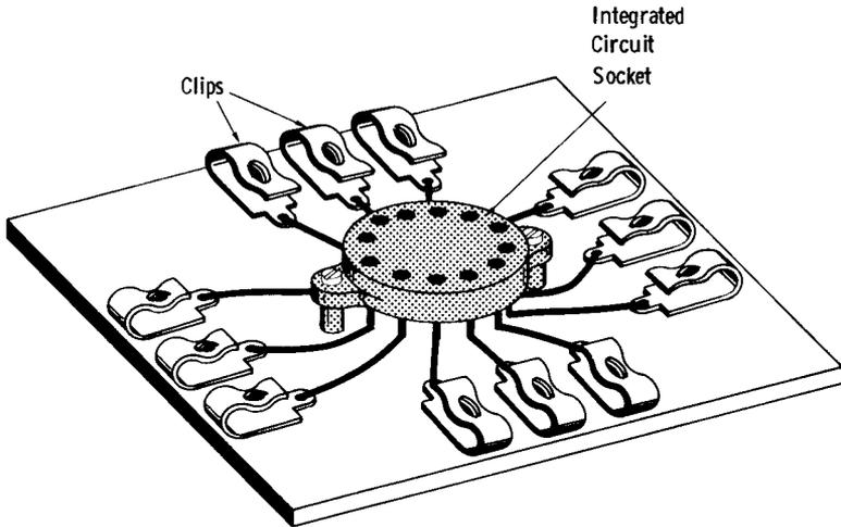
**Fig. 6-16. Mounting integrated circuit socket for experimental use.**
