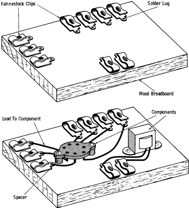
**Fig. 4-3. Wooden breadboards.**
