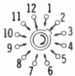
Fig. 7-10. A single-pole, 12-position wafer-switch symbol.
