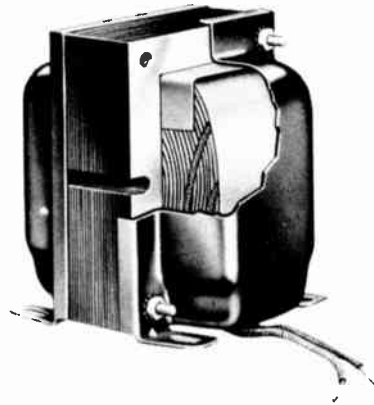
Fig. 4-5. Cutaway view of an iron-core transformer.
