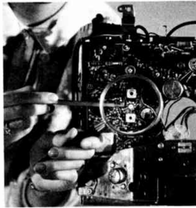
Fig. 9-17. An integrated circuit installed in a television receiver.
