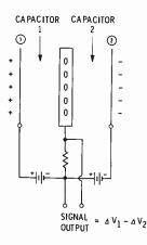
Fig. 3-18. A figure-eight condenser microphone. Operation is the same as in Fig. 3-16 except that capacitors 1 and 2 produce voltages across the resistor that are 180° out of phase with each other.
