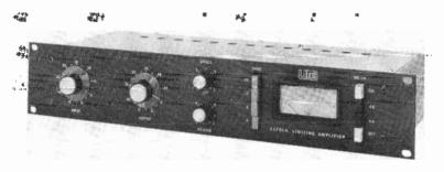
Courtesy United Recording Electronic Industries Fig. 5-35. The Universal Audio 1176LN.
