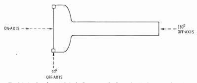
Fig. 3-5. A microphone axis is the line perpendicular to the diaphragm on the side exposed to the sound waves.
