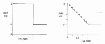
(A) Updating occurs once each second. The fade is encoded as a step change of 5 dB.
