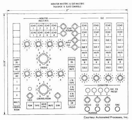
Fig. 6-19. The API monitor master control panel.
