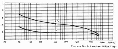
Fig. 5-53. Frequency response of decay time for BX20E.
