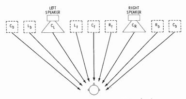
Fig. 13-12. The stereo stage created by a QS-encoded disc played in stereo.
