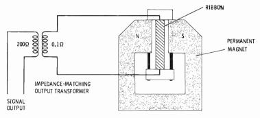
Fig. 3-8. The basic components of a ribbon microphone.
