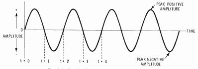
Fig. 2-1. Graph of waveform amplitude vs time.
