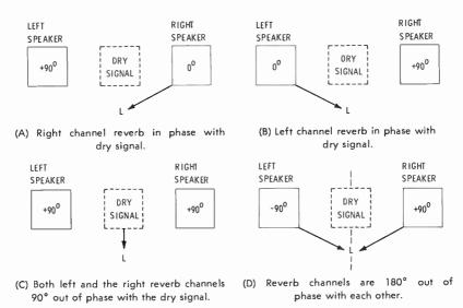
Fig. 5-46. The random phase relationship of the signals at the EMT plate outputs make the reverb appear to come from all directions.
