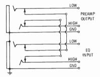
Fig. 6-3. Normalled jacks: the preamp output is normalled to the EQ input.
