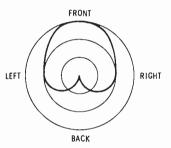
Fig. 3-2. A pressure-operated mike is sensitive to sound waves originating from any direction.
