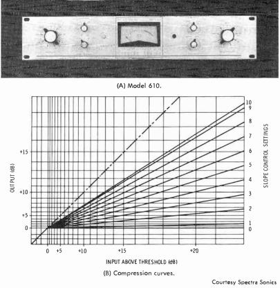
Fig. 5-38. The Spectra Sonics 610 Complimiter and compression curves.
