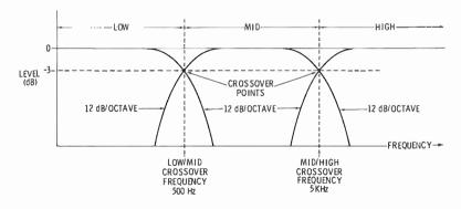
Fig. 8-4. Frequency response of a three-way crossover network with crossover frequencies of 500 Hz and 5 kHz.
