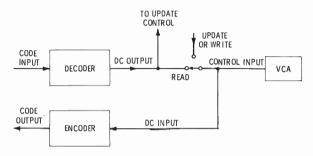
Fig. 11-10. The data for a function in the read mode is decoded and then re-encoded when recorded onto the other data track.
