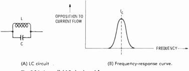
Fig. 5-14. A parallel LC circuit and frequency-response curve.
