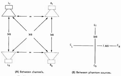
Fig. 13-4. Separation in the SQ system (with no logic or blending).
