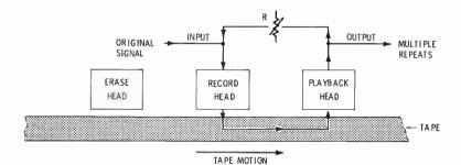
Fig. 5-58. Producing multiple repeats of a signal with a single playback head tape recorder.
