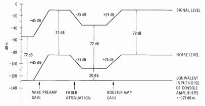
Fig. 3-23. Good console operating procedures do not degrade the signal-to-noise ratio.
