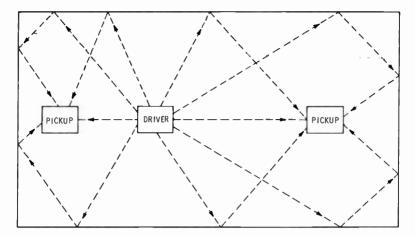
Fig. 5-44. The waves induced in the plate by the driver are reflected at the edges and converted into electrical signals by the pickups.
