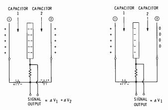
Fig. 3-16. An omnidirectional condenser Fig. 3-17. A cardioid condenser microphone. microphone diagram.
