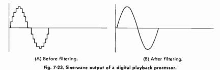
Since all signals below the threshold of the lowest quantization level are ignored, a type of noise called *quantization noise* is induced in the signal when it is in this range. This noise has a very grainy quality and can be reduced by increasing the number of digits used in the word, or it can be hidden by adding hiss to the original signal
