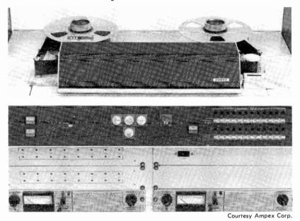
Fig. 4-27. The front panel of an Ampex MM1000 24-track recorder.
