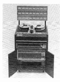
Courtesy Mincom Division, 3M Co. Fig. 4-36. The 3M M79/24, 24-track recorder. This machine is also available in 8and 16-track versions.
