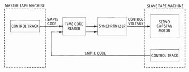
Fig. 10-10. Synchronizing two tape machines using the SMPTE code.
