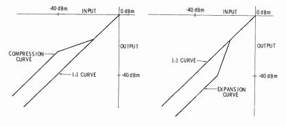
Fig. 7-5. The Dolby compression curve.
