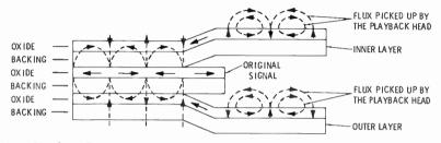
Fig. 4-25. The difference between print-through to the inner and outer layers of tape.
