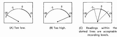
Fig. 6-15. VU meter readings.
