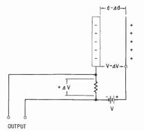
Fig. 3-14. If a sound wave decreases the plate spacing by  $\Delta$  d, the capacitance increases by  $\Delta$  C and the voltage across the plates falls by  $\Delta$  V.
