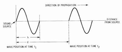
Fig. 2-2. Demonstrating velocity of a wave.
