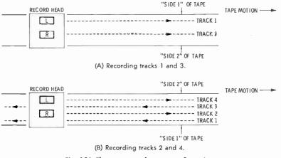
Fig. 4-20. The quarter-track stereo configuration.
