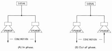
Fig. 8-5. Relative cone motion, speakers in phase and out of phase.
