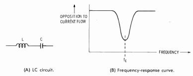
Fig. 5-15. A series LC circuit and frequency-response curve.
