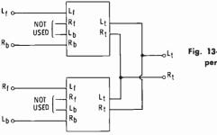
Fig. 13-8. Connecting two SQ encoders to permit encoding along the L<sub>7</sub>R<sub>b</sub> and R<sub>7</sub>L<sub>b</sub> diagonals.
