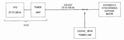
Fig. 5-64. Varying the speed of a hystersis synchronous motor.
