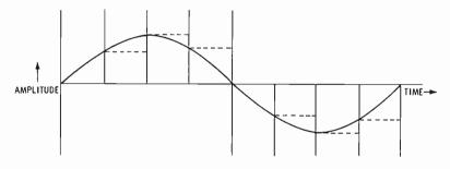
Fig. 7-21. The audio-signal amplitude is measured at each vertical line, and each measurement is converted into a binary word.
