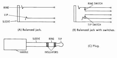
Fig. 6-5. Types of balanced jacks, and plug used with them.
