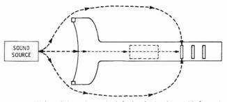
(B) Signal through port is shifted to be in phase with front signal.
