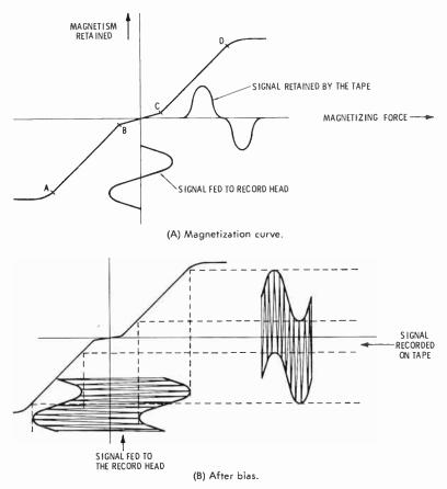
Fig. 4-14. Illustrating effect of biasing on recording linearity.
