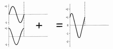
(C) The amplitudes of partially out-of-phase waves add in some places and subtract in others when mixed.
