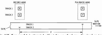
Fig. 4-17. If an overdub is attempted without the use of sel sync, the signal on track two will lag the original signal by a time equal to the distance (d), divided by the tape speed.
