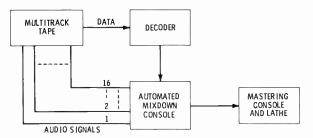
Fig. 11-12. Mastering a disc directly from a multitrack tape.
