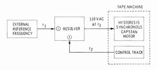
Fig. 10-3. Controlling tape speed with a resolver and a 60-Hz synchronous capstan motor.
