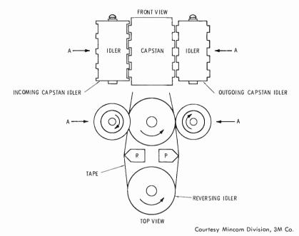
Fig. 4-4. Diagram of the capstan and capstan idlers used in 3M's "Isoloop" tape drive. The grooves make the incoming tape see a smaller capstan diameter than the outgoing tape.
