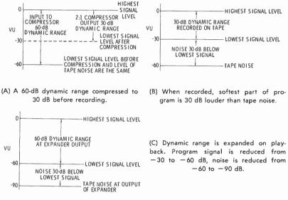
Fig. 7-19. Noise reduction in DBX system.
