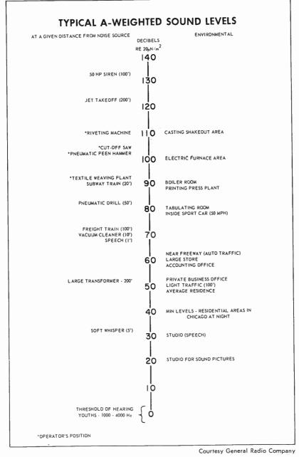
Fig. 2-18. Typical spls for common sounds. The reference level of 20  $\mu$ N/m<sup>2</sup> is equivalent to 0.0002 microbar (or 0.002 dynes/cm<sup>2</sup>).
