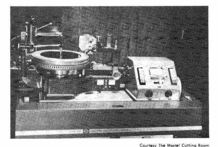
Fig. 12-4. The Neumann VMS-70 lathe front view.
