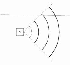
Fig. 1-7. Waves leave the sound source (\$) in an arc with angle  $\theta$ .
