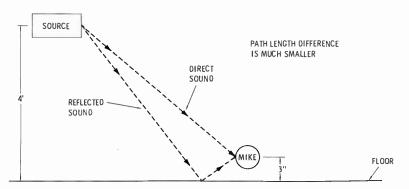
Fig. 3-26. Moving the distant mike toward the reflecting surface decreases the difference in path length and raises the lowest frequncy of cancellation.
