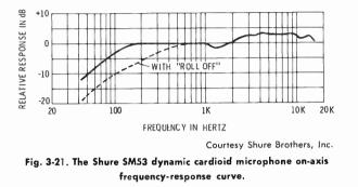
The next most significant specification is the *output impedance*. If the mike is not connected to the proper load, the frequency response and directional characteristics shown in the curves will be degraded.
