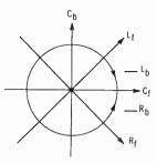
clockwise circle. The lengthwise motion of the groove under the stylus causes these two circular motions to form a double helix. Center-front information causes lateral stylus motion while center-back information causes vertical motion (Fig. 13-6).
