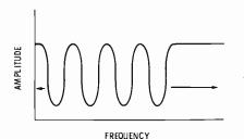
Fig. 5-68. The phasing effect creates a comb filter with variable dip frequencies.
