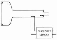
Fig. 3-11. A method of producing variable pickup patterns from a ribbon microphone using ports and an acoustical phase-shift network.
