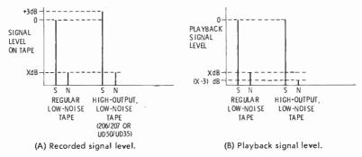
Fig. 4-21. Comparison of high-output, low-noise tape with regular low-noise tape.
