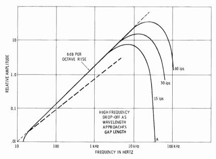
Fig. 4-9. The output of a playback head rises with frequency until the wavelength of the recorded signal approaches the gap length.
