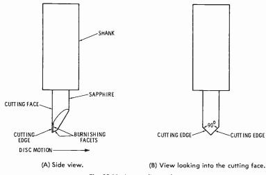
Fig. 12-11. A recording stylus.
