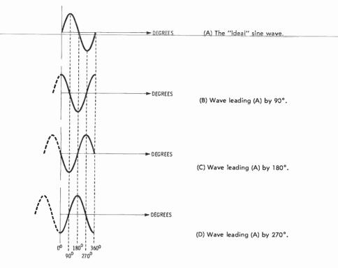
Fig. 2-5. Demonstrating phase relationships of sine waves.
