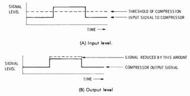
Fig. 5-29. The compressor reduces the level of the portion of the signal that exceeds the threshold.
