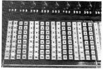
Courtesy Automated Processes, Inc. Fig. 6-11. The switching matrix on the 2824 console.
