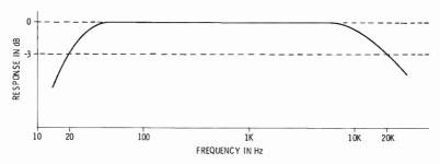
Fig. 4-13. A frequency-response curve with a 20-Hz lower cutoff frequency and a 20kHz upper cutoff frequency.
