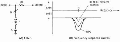
Fig. 5-17. A dip cut filter and frequency-response curves.
