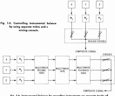
Fig. 1-6. Instrumental balance by recording instruments on separate tracks of multitrack tape.
