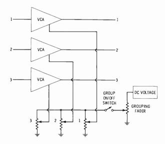
(C) Retaining separation by using VCAs and a grouping fader to control the level of the voltage fed to the individual dc control faders which in turn feed the VCA control inputs.
