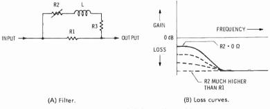
Fig. 5-9. A low-frequency shelf boost filter and loss curves.
