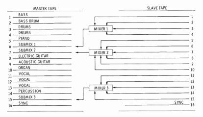
Fig. 10-6. Reducing the mixdown capacity requirements for interlocked tapes.
