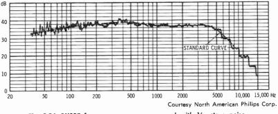
Fig. 5-54. BX20E frequency response measured with 1/3-octave noise.
