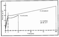
FIGURE 3. TENSILE PROPERTIES OF 11/2 MIL BACKING
