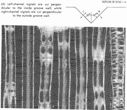
(B) A photomicrograph of grooves modulated with stereo program material.
