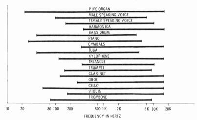
Fig. 5-23. Frequency ranges of instruments.
