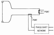
(A) Both ports are closed. The ribbon becomes a pressure-operated omnidirectional mike.
