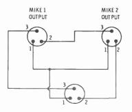
COMBINED SIGNAL OUTPUT TO MIKE PREAMP Fig. 3-28. Connecting two microphones in series. Pin 1 is ground, pin 2 is the high signal output, and pin 3 is the low signal output.
