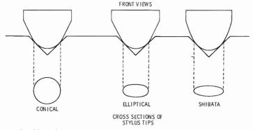
Fig. 12-18. Groove contact for the conical, elliptical, and Shibata styli.
