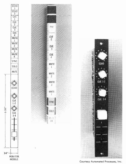
Fig. 6-18. The multitrack monitor mixer used on the API Model 2824 console.
