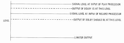
Fig. 7-13. The tape output is fed to the Dolby playback processor at too high a level.
