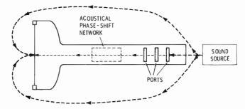
(A) Signals arrive at front and rear of the diaphragm.
