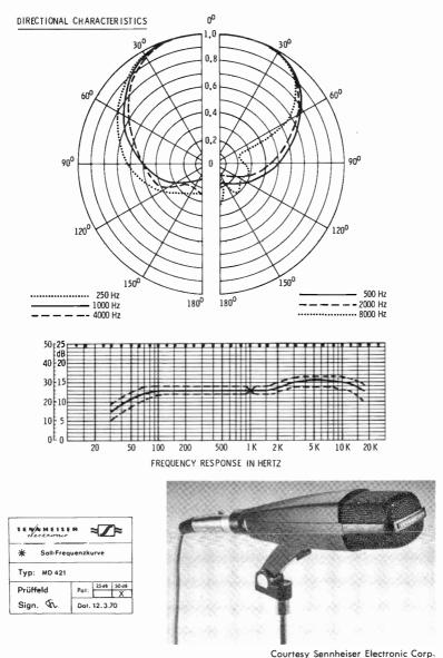
Fig. 3-29. The Sennheiser MD421 microphone.
