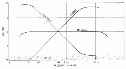
Fig. 4-11. The basic EQ used for magnetic recording.
