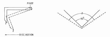
(A) Cutting at increased depth causes groove angle greater than 90°.
