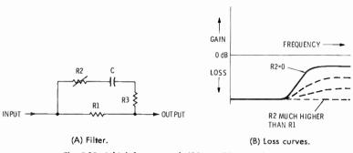
Fig. 5-10. A high-frequency shelf boost filter and loss curves.
