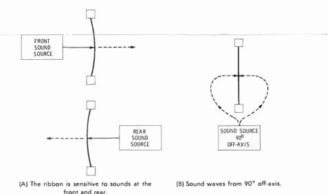
Fig. 3-9. Sound sources on-axis and 90° off-axis at a ribbon mike.
