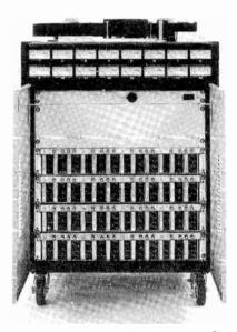
Courtesy Mincom Division, 3M Co. Fig. 4-32. The 3M M56 8-track recorder with remote control unit. Courtesy Ampex Corp.
