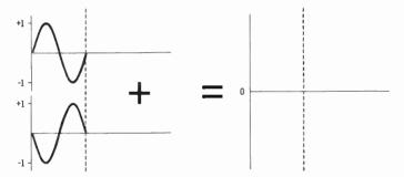
(B) Waves of equal amplitude cancel completely when mixed 180° out of phase.
