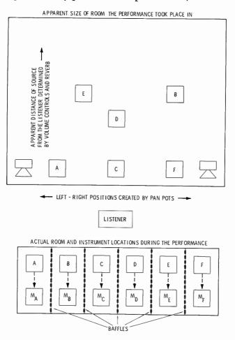
Fig. 1-12. Close-miked instruments A through F can be made to appear as if they originate from various locations in an imaginary stage behind and between the stereo speakers.
