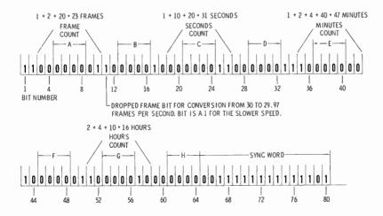
Fig. 10-7. The location of the 80 bits in the SMPTE digital word.
