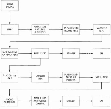
Fig. 1-3. The recording chain.
