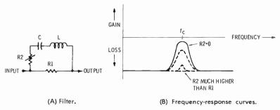
Fig. 5-16. A peak boost filter and frequency-response curves.
