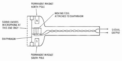
Fig. 3-1. The components of a dynamic microphone.
