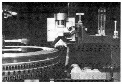
Courtesy The Master Cutting Room Fig. 12-7. Neumann SX-68 cutter head.
