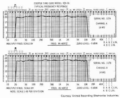
Fig. 5-63. Cooper Time Cube frequency-response curves.
