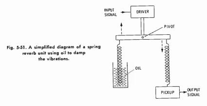
the propagation velocity of the waves in the springs and by the multiple reflections that occur both when the waves hit the oil and when a wave reaches the junction of two springs. The height of the oil in the tube determines the decay time of the unit. As the height of the oil rises, damping increases and the decay time decreases. The decay time in this type of unit usually remains fixed because draining and refilling the tube with oil is a messy job.
