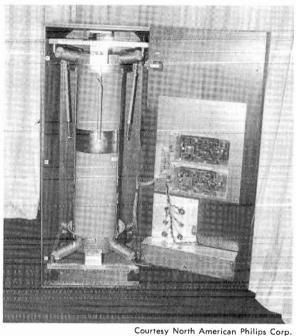
Fig. 5-52. The AKG BX20E reverberation unit (interior view).
