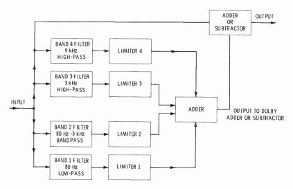
Fig. 7-8. Block diagram of the filter/limiter networks.
