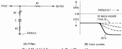
Fig. 5-11. A high-frequency shelf cut filter and loss curves.
