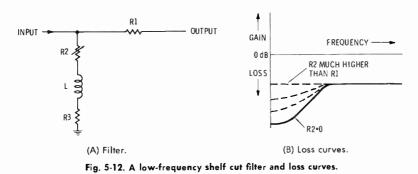
Low-frequency shelf cut is achieved simply by substituting an inductor for the capacitor (Fig. 5-12A). Fig. 4-12B shows loss curves for the network.
