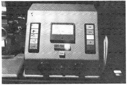
Courtesy The Master Cutting Room Fig. 12-5. The Neumann VMS-70 lathe pitch controller.
