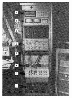
Courtesy The Master Cutting Room Fig. 12-21. The Neumann SP-172 Program Controller.
