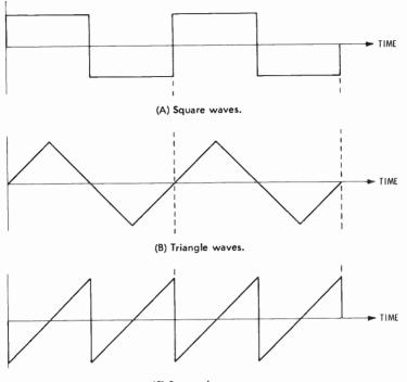
(C) Sawtooth waves. Fig. 2-3. Simple waveforms.
