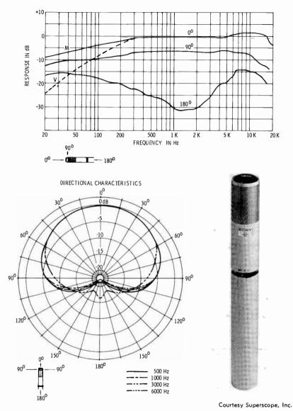
Fig. 3-30. The Sony ECM-22 electret condenser microphone.
