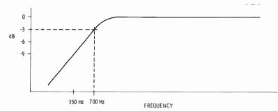
Fig. 5-19. A 700-Hz, high-pass filter with a slope of 6 dB per octave.
