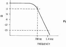
Fig. 5-20. A 700-Hz, low-pass filter with a slope of 12 dB per octave.
