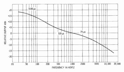
Fig. 12-20. The RIAA disc playback equalization curve.
