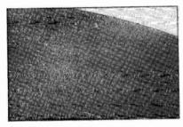
HOURE 1. ENLARGED VIEW OF DUST CONTAMINATION ON A REEL OF TAPE.
