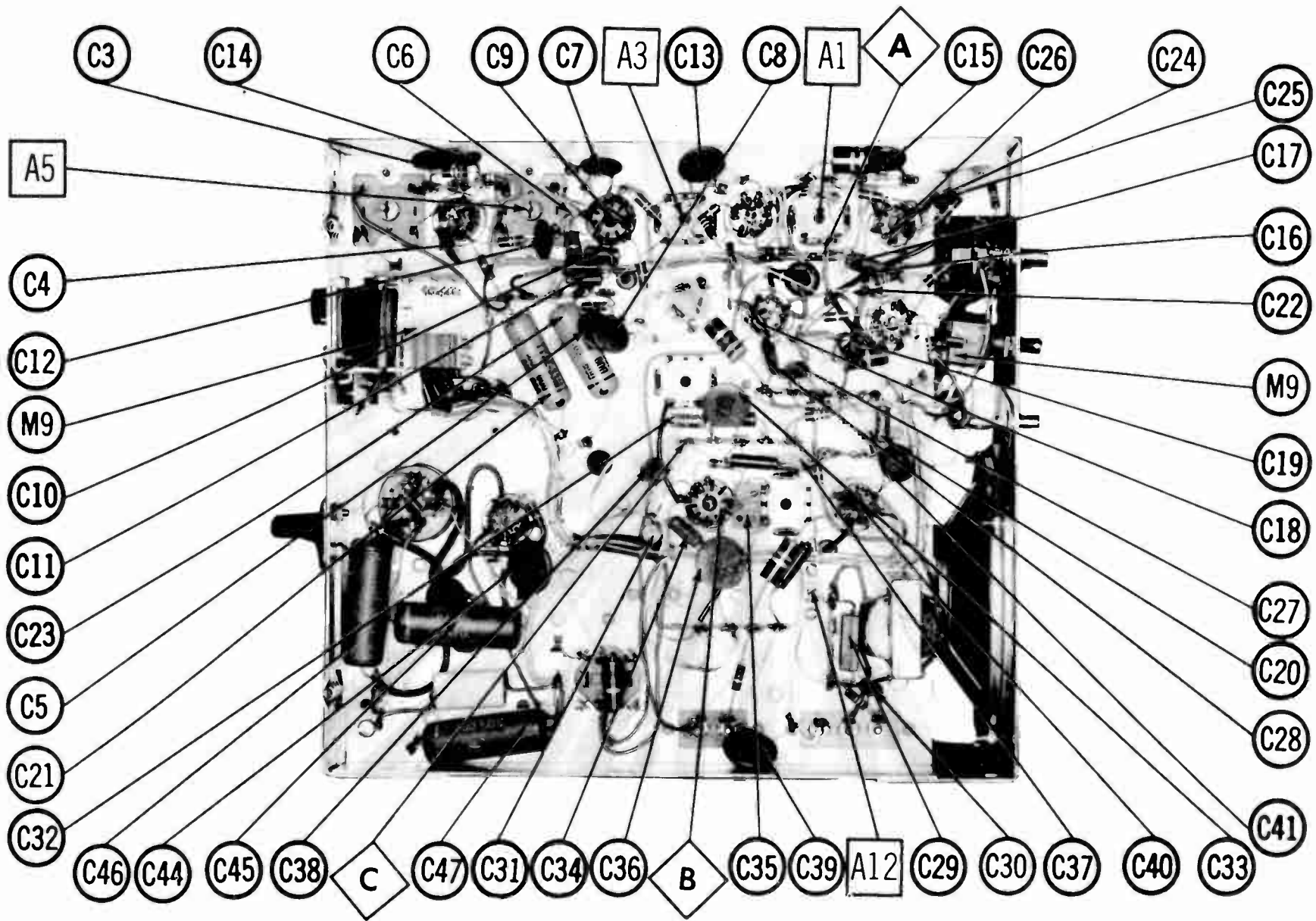
CHASSIS-BOTTOM VIEW-ALIGNMENT, CAPACITOR & MISC. IDENT.
